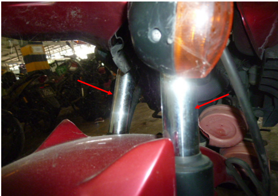
Photo 21 shows the front forks of the Motorcycle. The front forks were observed to be bent inwards as a result of the accident (arrowed). We were hence not able to conduct any tests on the steering system of the Motorcycle.
