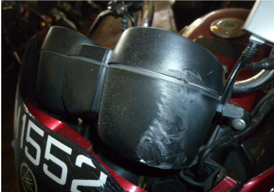
Photo 7 shows a closer view of the speedometer gauge which was amongst the body parts at the front body of the Motorcycle that had sustained damage as a result of the accident.
