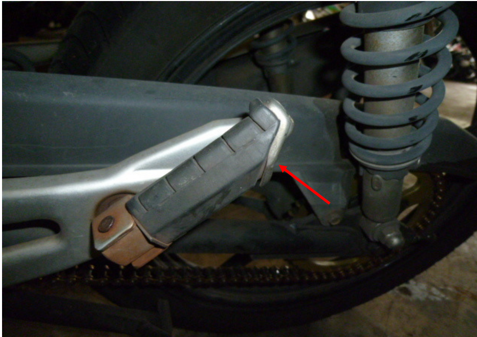
Photo 11 shows a closer view of the left pillion foot peg which was amongst the body parts of the Motorcycle that had sustained damage as a result of the accident (arrowed).
