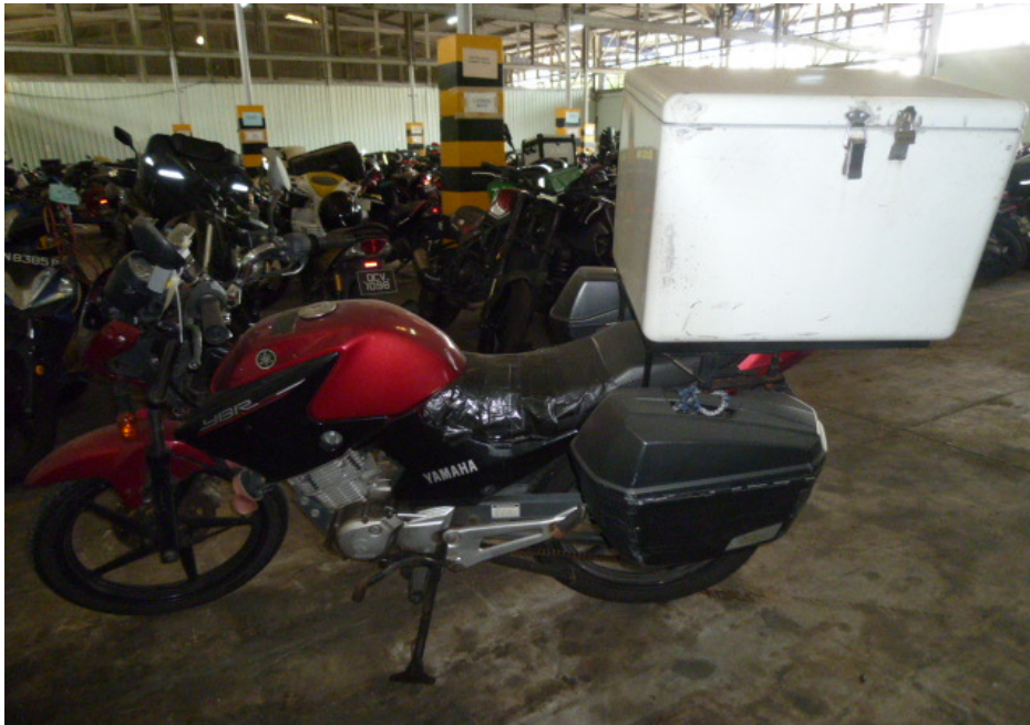
Photo 5 shows a general view of the left body of the Motorcycle at the time of our inspection. The Motorcycle had sustained damages all around. Body parts that were found to have been damaged include its headlight assembly, speedometer gauge, front fork assembly, front mudguard, left handlebar end, left side mirror, clutch lever, left cowling, left pillion foot peg, top box and side panniers, amongst others.
