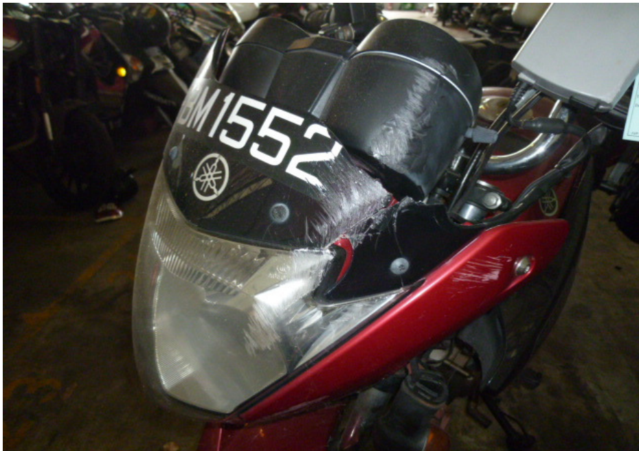
Photo 6 shows a closer view of the headlight assembly which was amongst the body parts at the front body of the Motorcycle that had sustained damage as a result of the accident.
