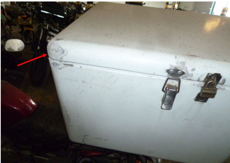
Photo 14 shows the top box of the Motorcycle which had sustained damage as a result of the accident (arrowed).
