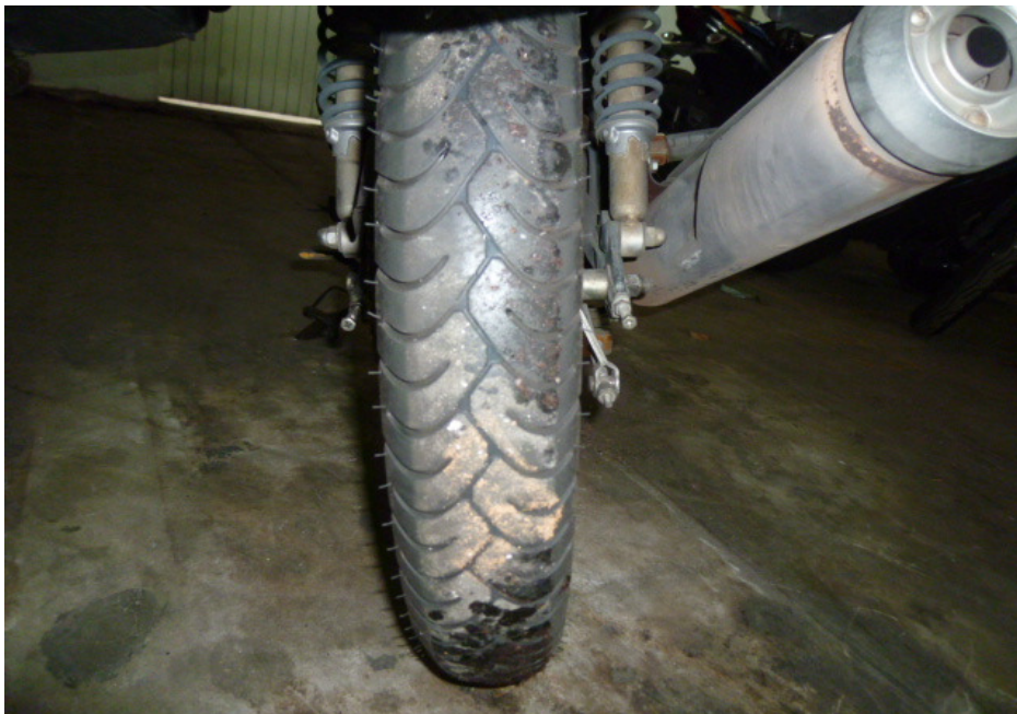
Photo 16 shows the condition of the Motorcycle's rear tyre. The pattern of the tread was clearly visible with remaining tread depth of approximately 2mm. We did not observe any tear, burst mark(s) and/or punctured hole(s) on the sidewalls as well as across the tread of the rear tyre.
