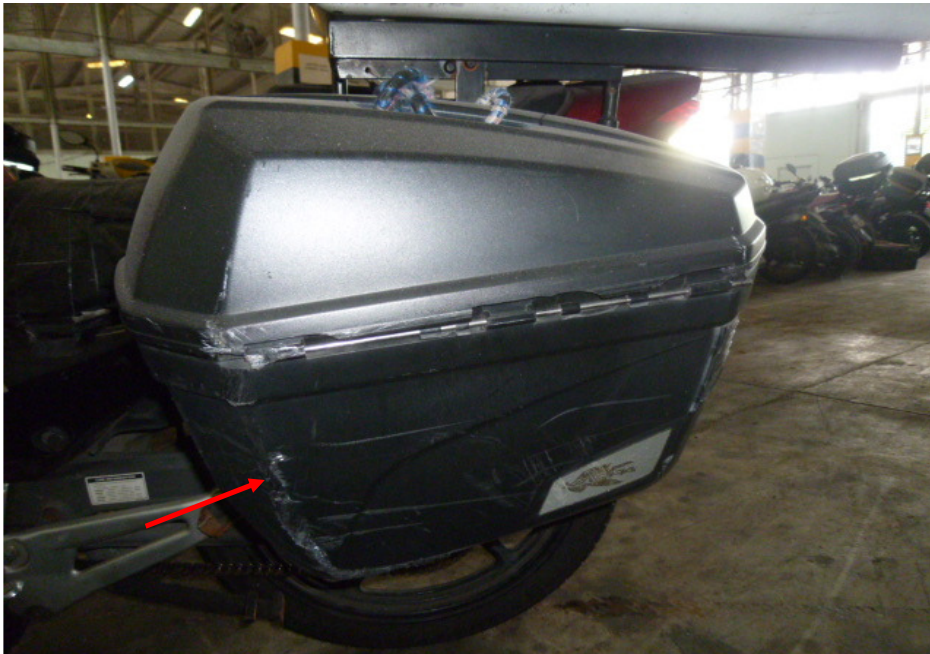
Photo 12 shows the left side pannier of the Motorcycle which had sustained damage as a result of the accident (arrowed).
