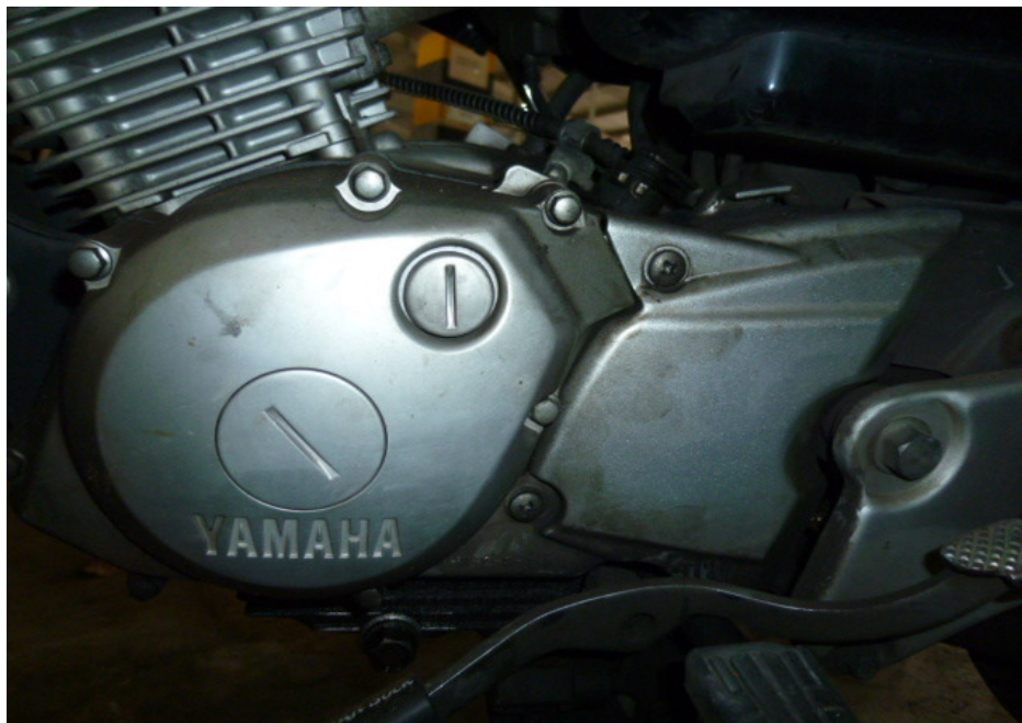
Photo 17 shows the left side of the engine of the Motorcycle at the time of our inspection. The various engine related parts and components were found to be intact with no visible damage. There was also no sign(s) or indication(s) of fluid leak observed around the left engine area of the Motorcycle.
