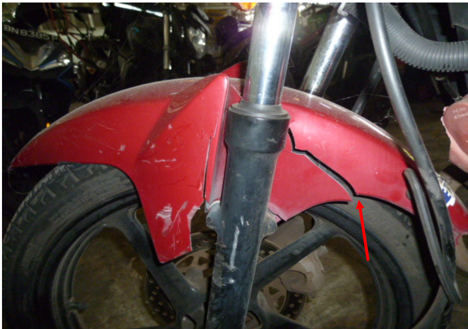
Photo 8 shows a closer view of the front mudguard which was amongst the body parts at the front body of the Motorcycle that had sustained damage as a result of the accident (arrowed).
