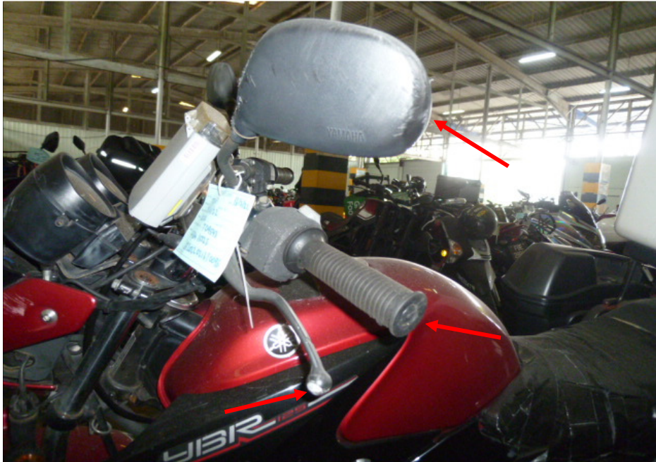
Photo 9 shows a closer view of the left side mirror, clutch lever and left handlebar end of the Motorcycle (arrowed). These parts were amongst the body parts of the Motorcycle which were damaged as a result of the accident.
