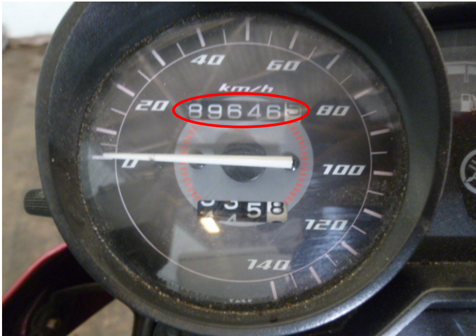
Photo 1 shows the speedometer gauge of the Motorcycle. The mileage of the Motorcycle at the time of our inspection was 89, 646km (circled).
