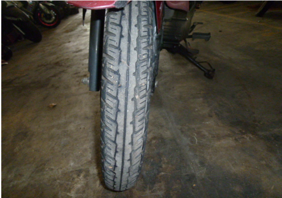
Photo 15 shows the condition of the Motorcycle's front tyre. The front tyre was observed to be in serviceable condition with remaining tread depth of approximately 2mm. There was no tear, burst mark(s) and/or punctured hole(s) on the sidewalls as well as across the tread of the front tyre.
