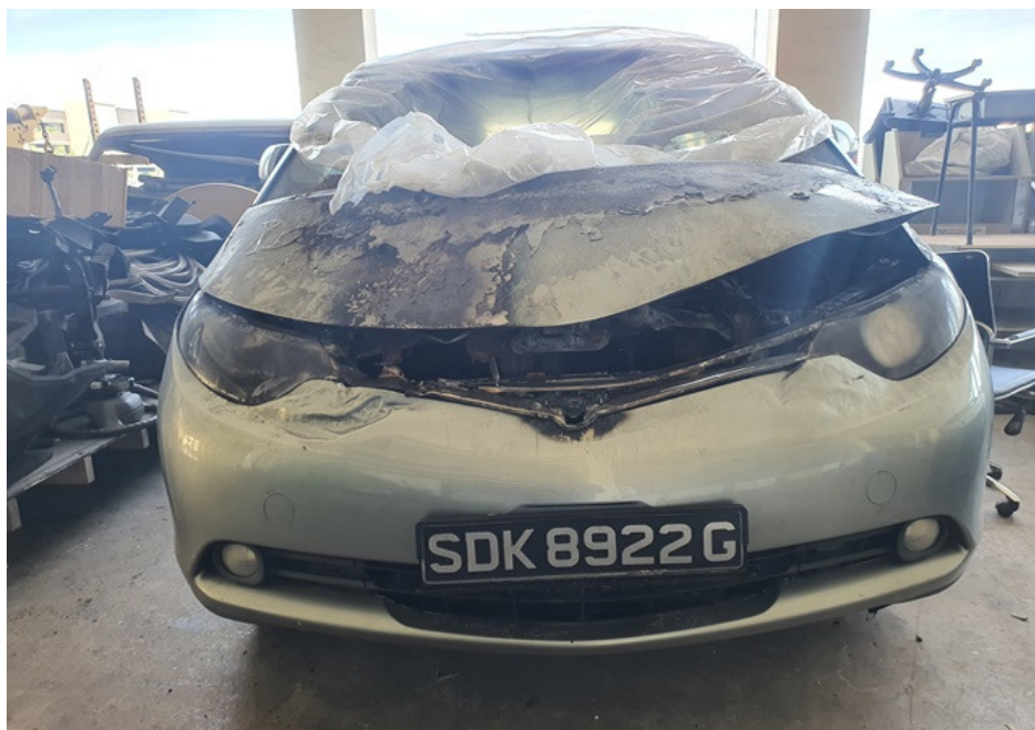
Photo 2 shows the general view of the frontal portion of the Insured Vehicle at the time of our inspection. The exterior body of the Insured Vehicle had sustained visible fire damage. This included its front windscreen, front bonnet, front bumper, headlights and side panels.
