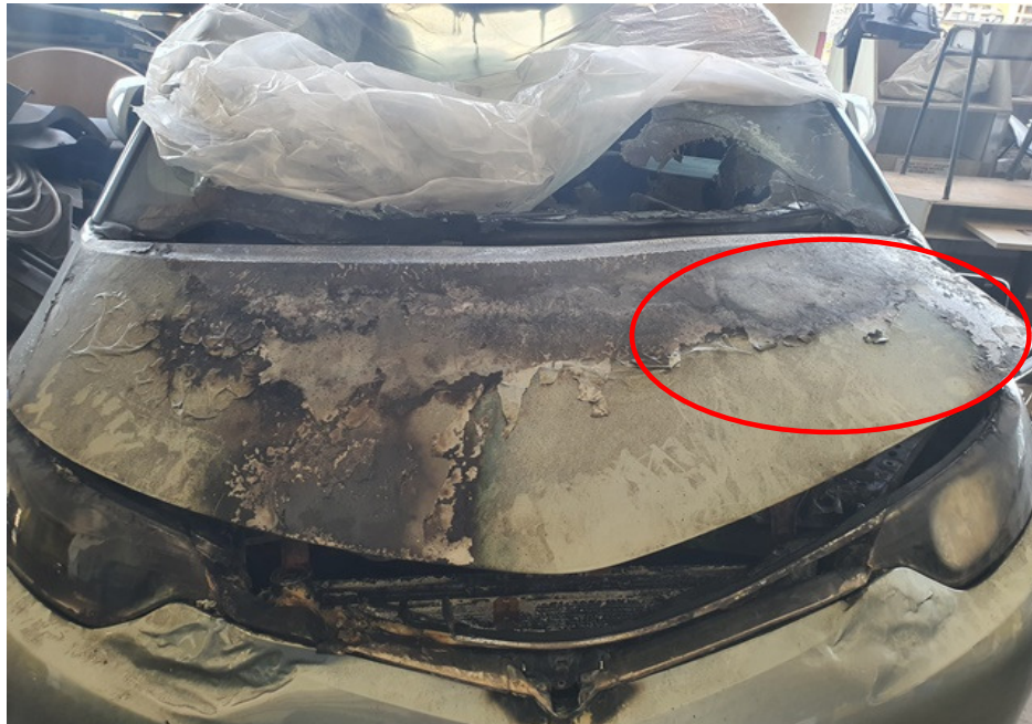
Photo 7 shows the burn pattern and whitish burn marks that were found on the left portion of the front bonnet of the Insured Vehicle (circled). Such whitish burn marks are a result of exposure to prolonged heat intensity, which may indicate where the fire had started. Rust would also begin to develop on these areas soon after the fire.
