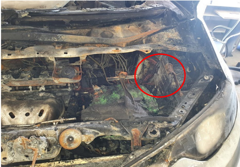
Photo 9 shows the burnt wirings around the left portion of the engine compartment which is in the immediate vicinity where the fire to the Insured Vehicle had likely started. We noticed greenish residue on several stretches of burnt wirings leading from the Engine Control Module (ECM) (circled). The presence of greenish residue indicates internal heating of copper wires, a sign of an electrical short circuit occurring.
