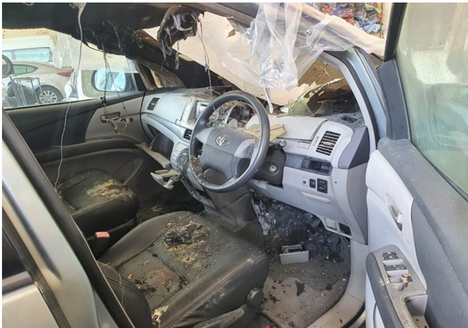
Photo 6 shows the interior compartment of the Insured Vehicle, which was observed to be severely affected by the fire.
