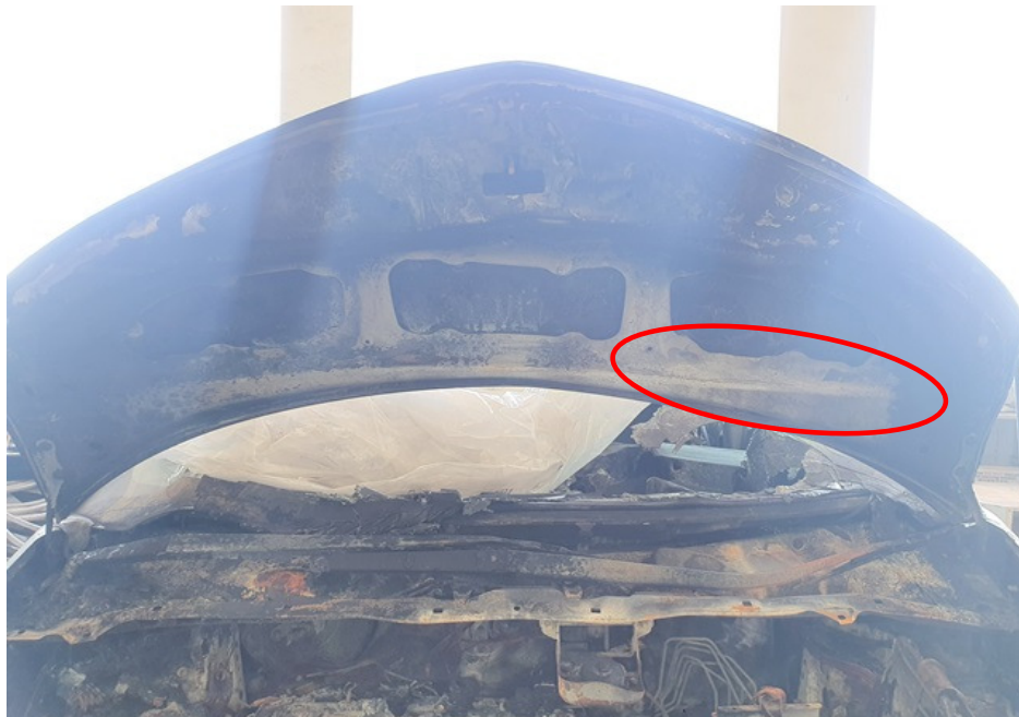
Photo 8 shows the rust that had developed on the underside of the front bonnet, around the left bottom portion (circled). The development of rust is an indication that this area was subjected to prolonged exposure to high heat intensity, which had caused the steel/metal material of the front bonnet to be exposed to natural environmental condition. Hence the fire to the Insured Vehicle can be determined to have originated towards the left portion of the engine compartment.
