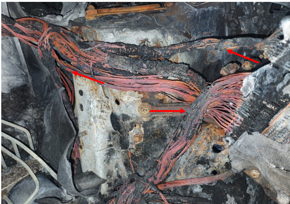
Photo 12 shows a close up view of the greenish residue found on several stretches of burnt wirings leading from the Engine Control Module (ECM) (red arrows). The presence of such greenish residue suggests occurrence of an electrical short circuit.
