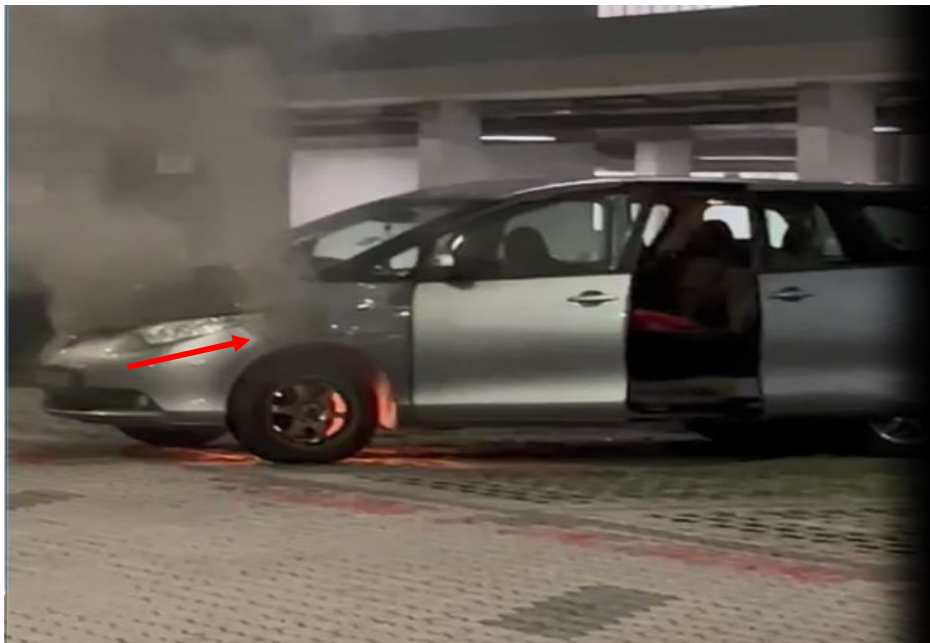
Photo 13 shows the Insured Vehicle on fire before the arrival of the SCDF. In general, the information that could be gathered from this photograph had corresponded to the events that were related to us by Ms Chua, which is the fire had started from the left rear portion of the engine compartment (arrowed).
