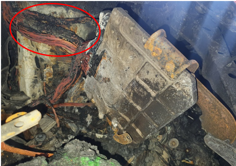
Photo 10 shows a closer view of the burnt wirings leading from the Engine Control Module (ECM). We noticed greenish residue on several stretches of the burnt wirings (circled). The greenish residue is normally left behind from oxidation as a result of chemical reaction involving the copper wires.
