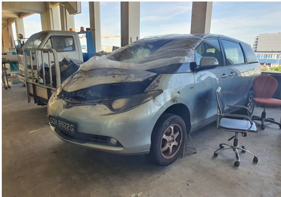
Photo 3 shows the general view of the left portion of the Insured Vehicle at the time of our inspection. The exterior body of the Insured Vehicle had sustained visible fire damage. This included its front windscreen, front bonnet, left headlight, front bumper and left front panel.
