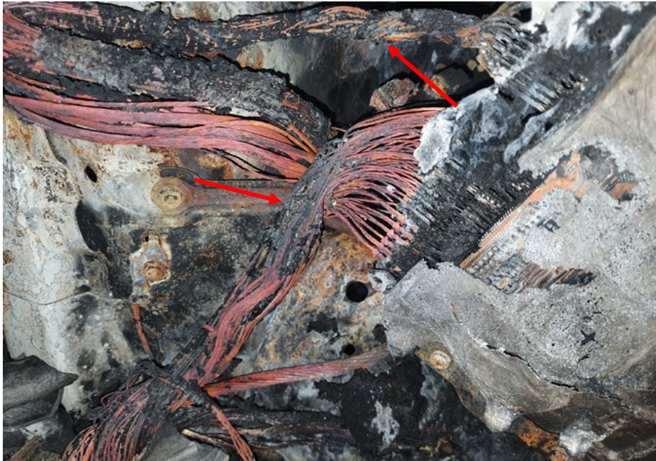
Photo 11 shows a close up view of the greenish residue found on several stretches of burnt wirings leading from the Engine Control Module (ECM) (red arrows). The presence of such greenish residue suggests occurrence of an electrical short circuit.
