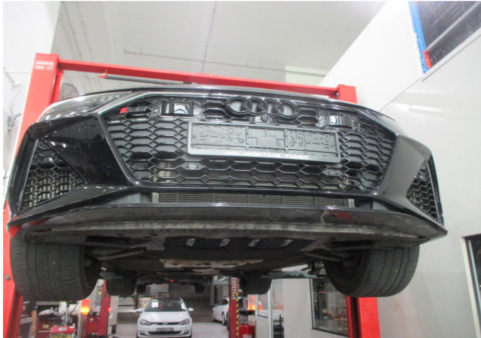
Photo 27 shows the Motor Car hoisted up for checks on its undercarriage. There was no sign(s) or indication(s) of fluid leakage and/or fluid stain(s) on the underside of the Motor Car. The undercarriage components of the Motor Car were also all observed to be intact and secured in an appropriate manner.
