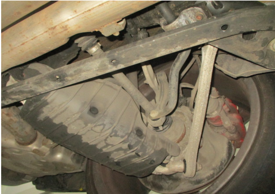
Photo 29 shows a general view of the control arms and linkages at the rear left wheel of the Motor Car. I did not observe any fluid leak and/or fluid stain on the underside of the Motor Car. All of the Motor Car's undercarriage components were observed to be intact and secured in an appropriate manner.
