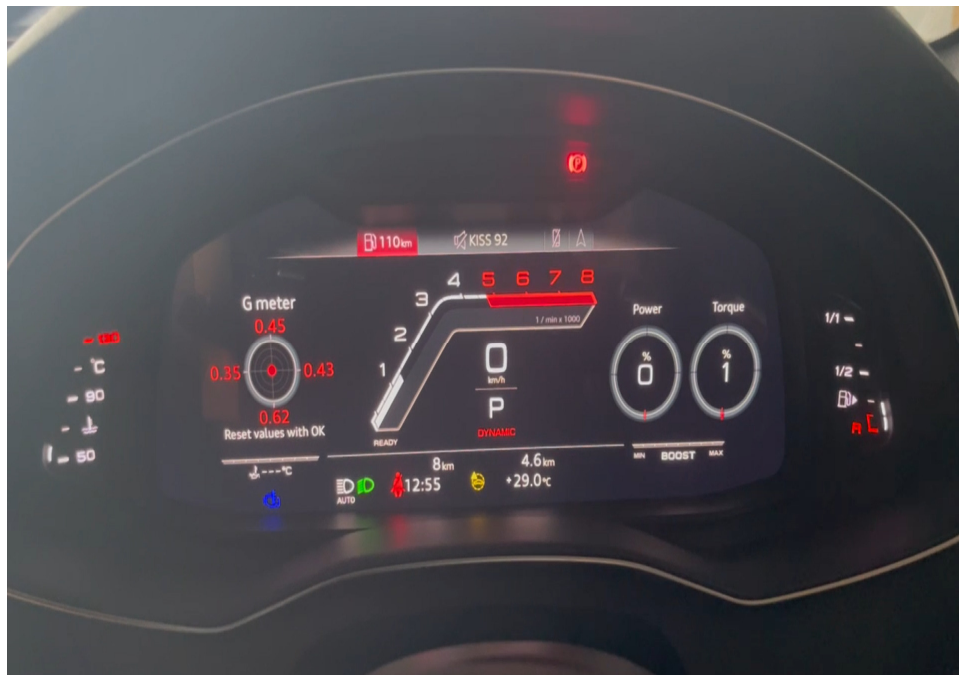
Photo 26 shows the respective warning lights no longer illuminated, indicating that there is no fault detected to the ABS, SRS, EPS, TPM and ESC systems of the Motor Car during the self-test. These electronic systems were hence in working condition at the time of my inspection.
