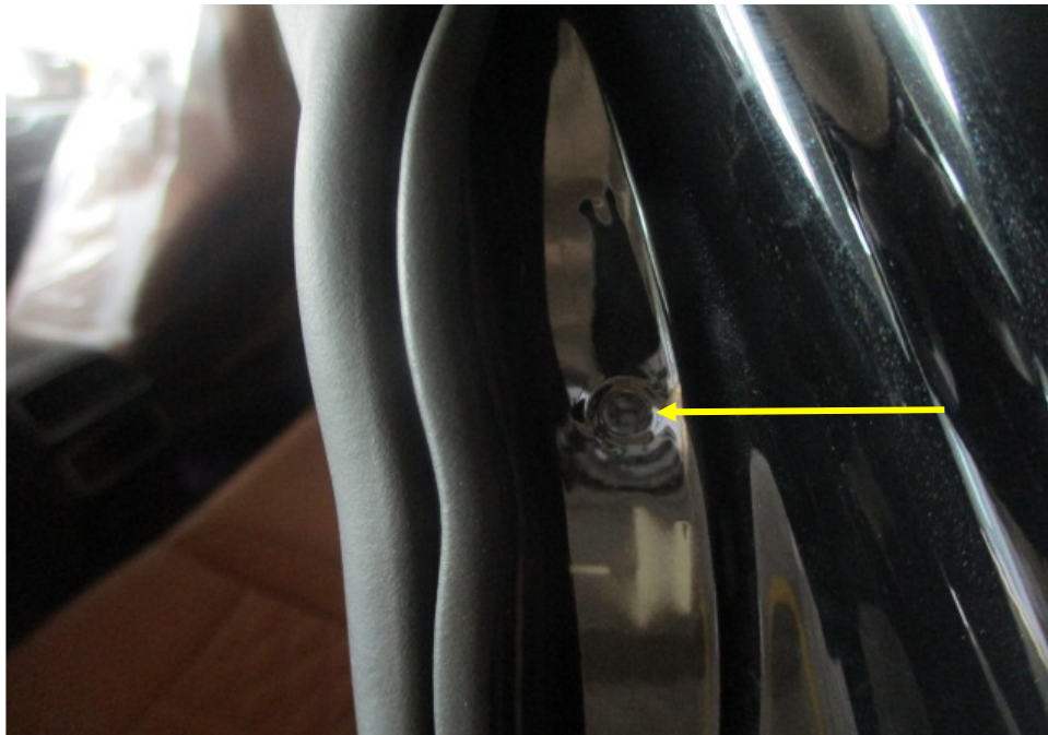
Photo 38 shows the left side "C" pillar of the Motor Car. I did not find any weld marks other than original spot weld marks (arrowed) on the left side "C" pillar of the Motor Car which, indicates that there was no re-welding works carried out. In general, I had found all the non-detachable body panels of the Motor Car to be originally fitted at the time of my inspection.
