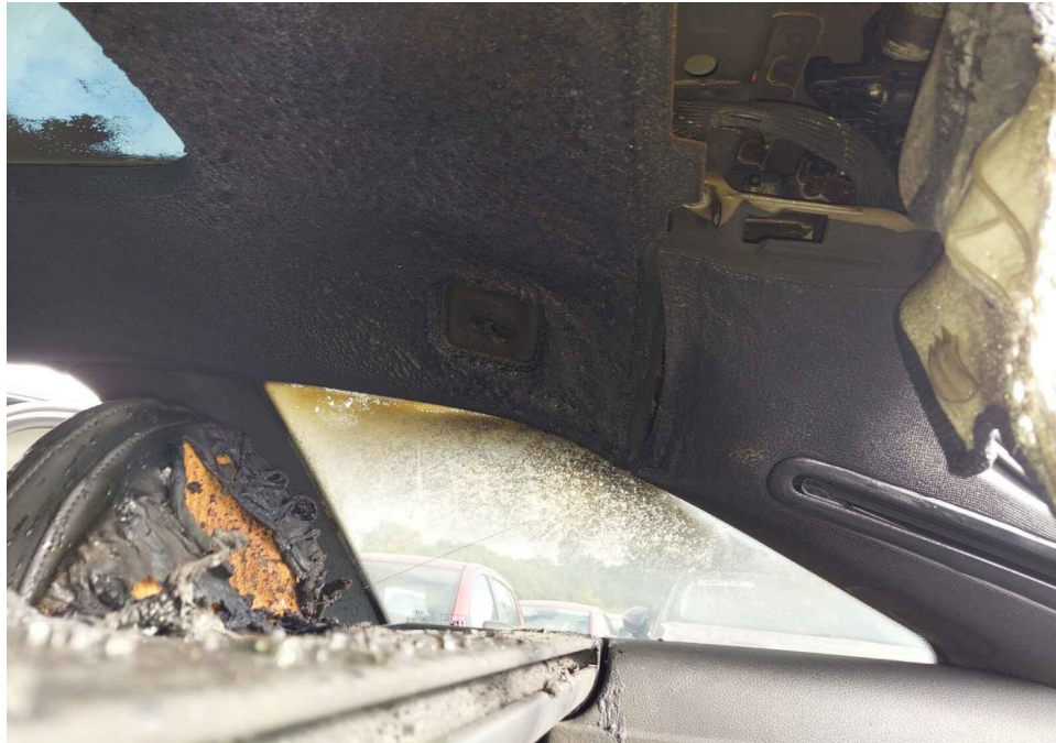
Photo 7 shows another view of the rear interior compartment of the Motor Car (photograph provided to me). Damage of fire/heat/smoke nature was seen to several parts and components within the interior compartment of the Motor Car. Parts and components affected had included the rear seats, roof upholstery, various inner trims, door windows, front windscreen and moon roof glass amongst others.
