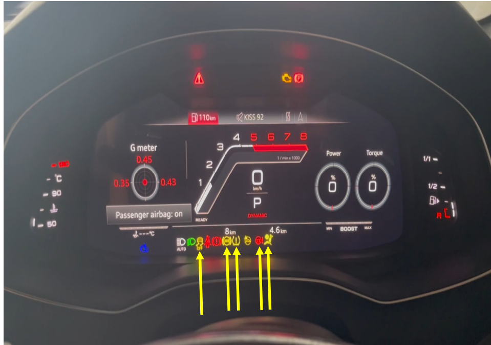
Photo 25 shows the warning lights for the various electronic safety features appearing on the instrument panel of the Motor Car during its self-test when the engine is cranked, in particular the ABS, SRS, EPS, TPM and ESC lights (arrowed).
