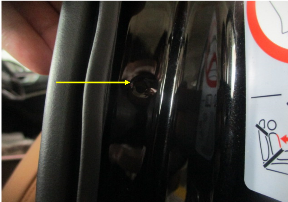
Photo 39 shows the left side "B" pillar of the Motor Car. I did not find any weld marks other than original spot weld marks (arrowed) on the left side "B" pillar of the Motor Car which, indicates that there was no re-welding works carried out. In general, I had found all the non-detachable body panels of the Motor Car to be originally fitted at the time of my inspection.
