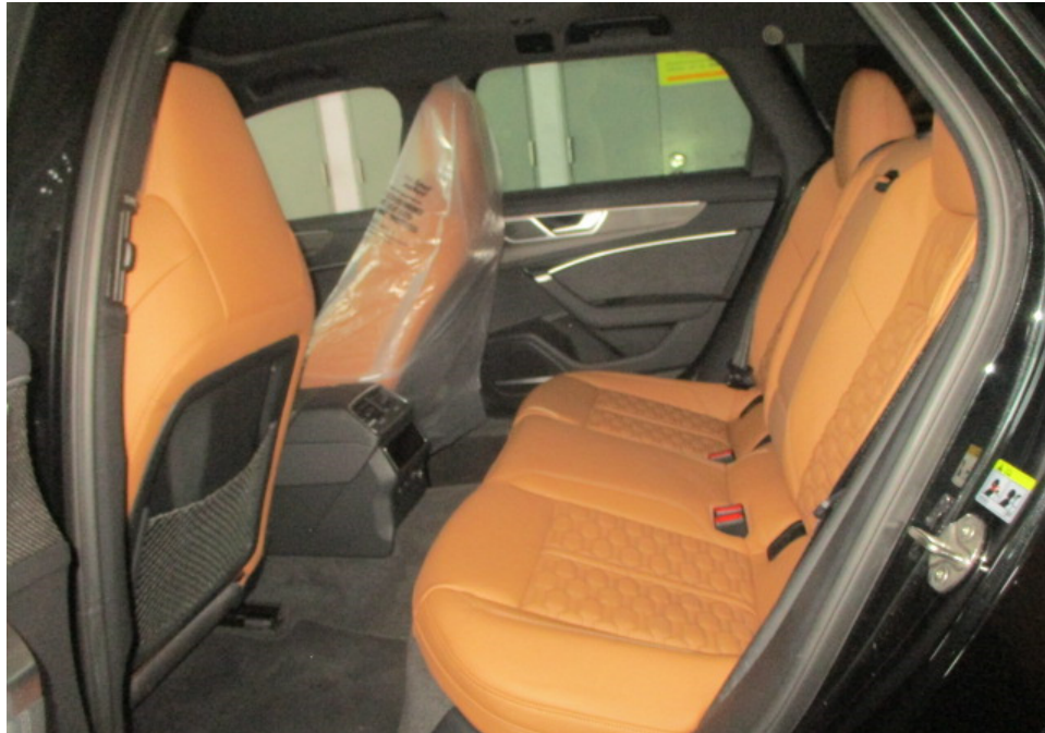
Photo 21 shows the front seats, rear seats, carpet and inner trims of the Motor Car. The various parts and components, inner trims, carpet and upholstery within the interior compartment were all observed to be intact and properly fitted. The repair/restoration works carried out to the damaged area of the Motor Car (refer to photograph 5 - 8 above) were reasonably adequate and in order.
