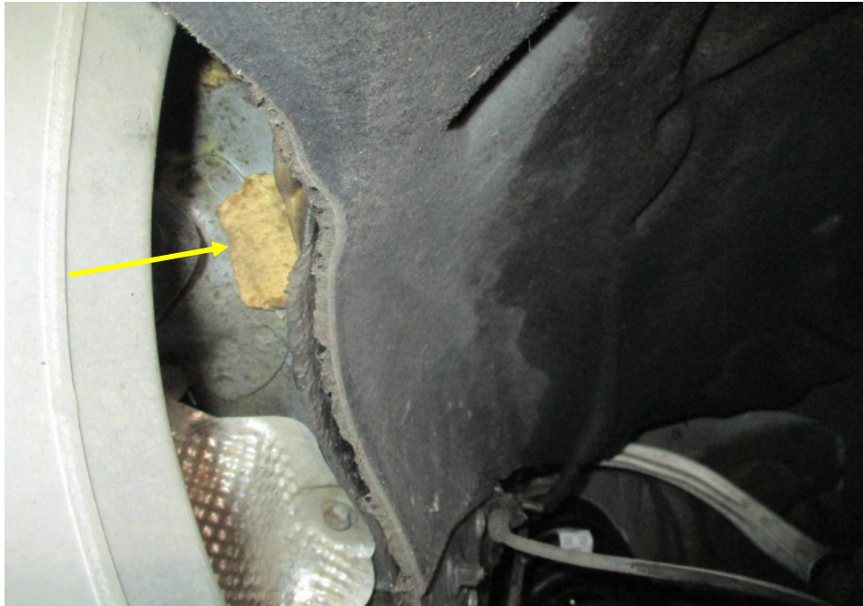
Photo 37 shows the chassis/structural body at the underside front right of the Motor Car. I did not find any weld marks other than original spot weld marks on the chassis/structural body of the Motor Car. The original factory sealant (arrowed) at the joints along the chassis/structural body was also untouched, indicating no work was done on the chassis/structural body of the Motor Car and that the chassis/structural body was originally fitted.
