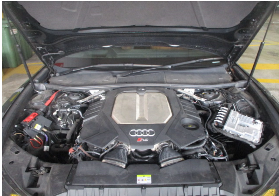
Photo 18 shows a general view of the engine compartment of the Motor Car at the time of my inspection. The various parts and components within the engine compartment were all observed to be intact and properly fitted. There was also no sign(s) or indication(s) of fluid leak and/or fluid stain found inside the engine compartment.
