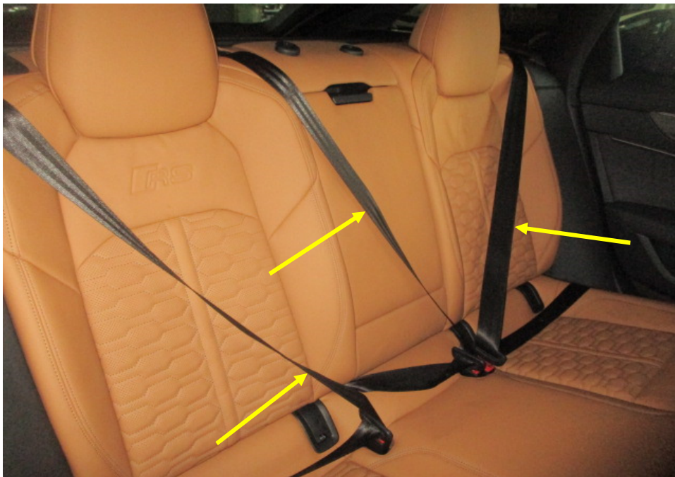
Photo 24 shows the rear seats of the Motor Car. All the seats of the Motor Car were secured via seat rails to the floorboard. They were also fitted with a retractable seat belt reel and a pre-tensioner. The seat belts (arrowed) were tested and were able to be fastened into the respective pre-tensions that were fitted on the side of each individual seat.
