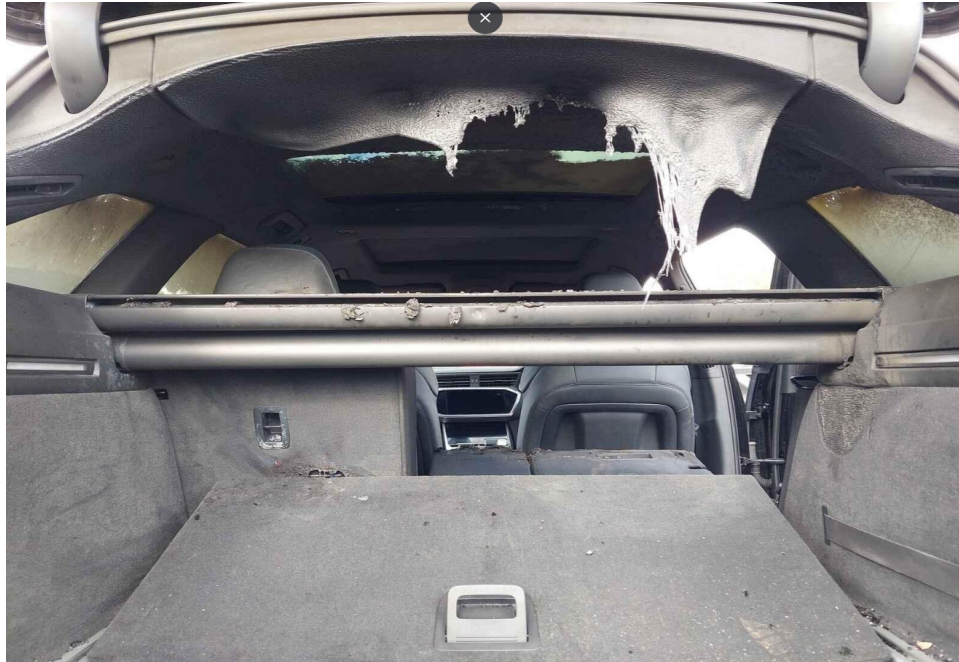
Photo 5 shows the rear interior compartment of the Motor Car (photograph provided to me). The photographs provided to me had showed damage of fire/heat/smoke nature to several parts and components within the interior compartment of the Motor Car. Parts and components affected had included the rear seats, roof upholstery, various inner trims, door windows, front windscreen and moon roof glass amongst others.
