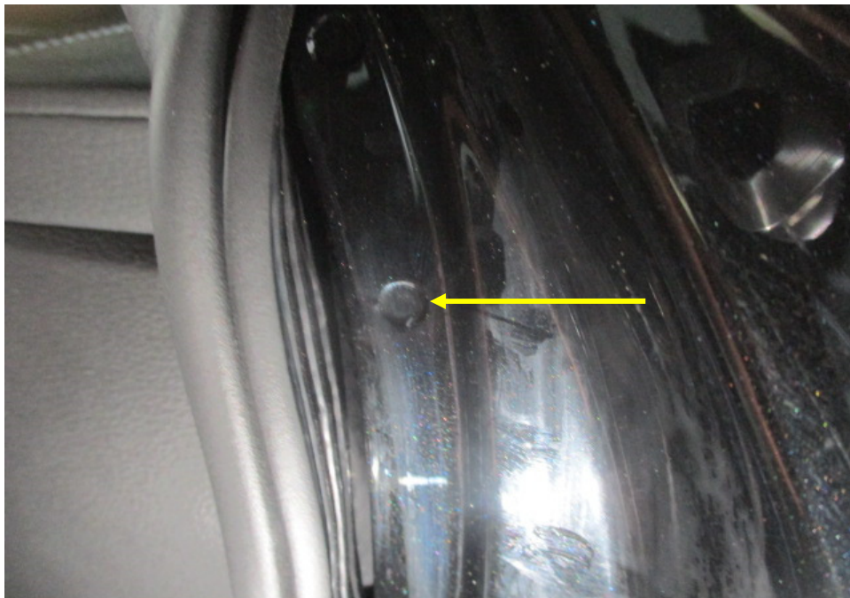
Photo 40 shows the right side "A" pillar of the Motor Car. I did not find any weld marks other than original spot weld marks (arrowed) on the right side "A" pillar of the Motor Car which, indicates that there was no re-welding works carried out. In general, I had found all the non-detachable body panels of the Motor Car to be originally fitted at the time of my inspection.
