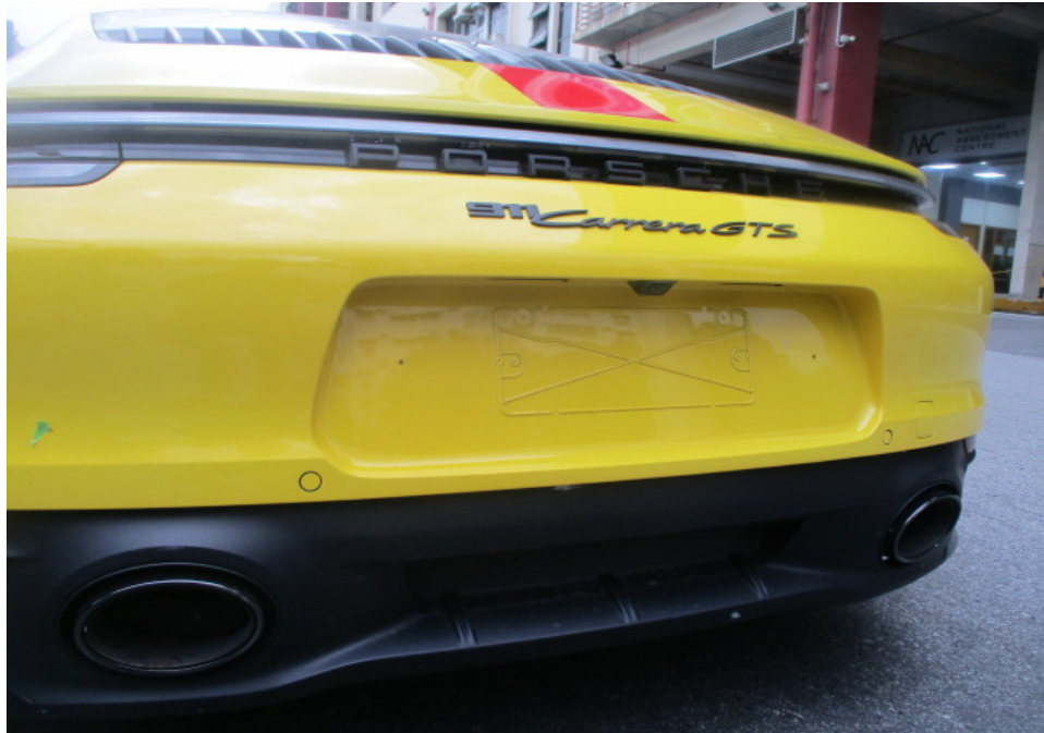
Photo 16 shows a closer view of the Motor Car's rear bumper, rear bumper lower cover, rear left exhaust garnish and rear centre lamp. The body parts at the rear portion of the Motor Car were visually examined and it was observed that the repair/restoration works carried out to the damaged area of the Motor Car (refer to photograph 3 & 4 above) were reasonably adequate and in order.
