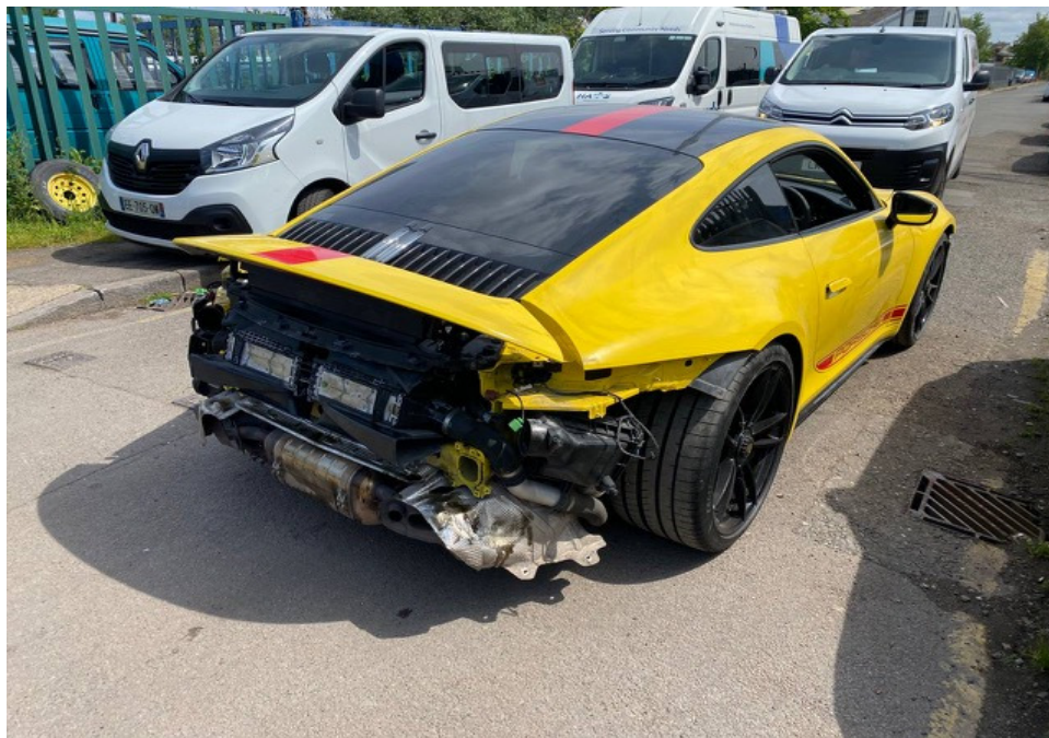
Photo 4 shows the rear right body of the Motor Car (photograph provided to me). The Motor Car's rear right taillamp, rear centre lamp, rear bumper and all its related parts and attachments like the rear bumper lower cover, rear bumper right bracket, rear bumper right reflector, rear bumper sensors and rear right exhaust garnish amongst others, were missing/dislodged/damaged.
