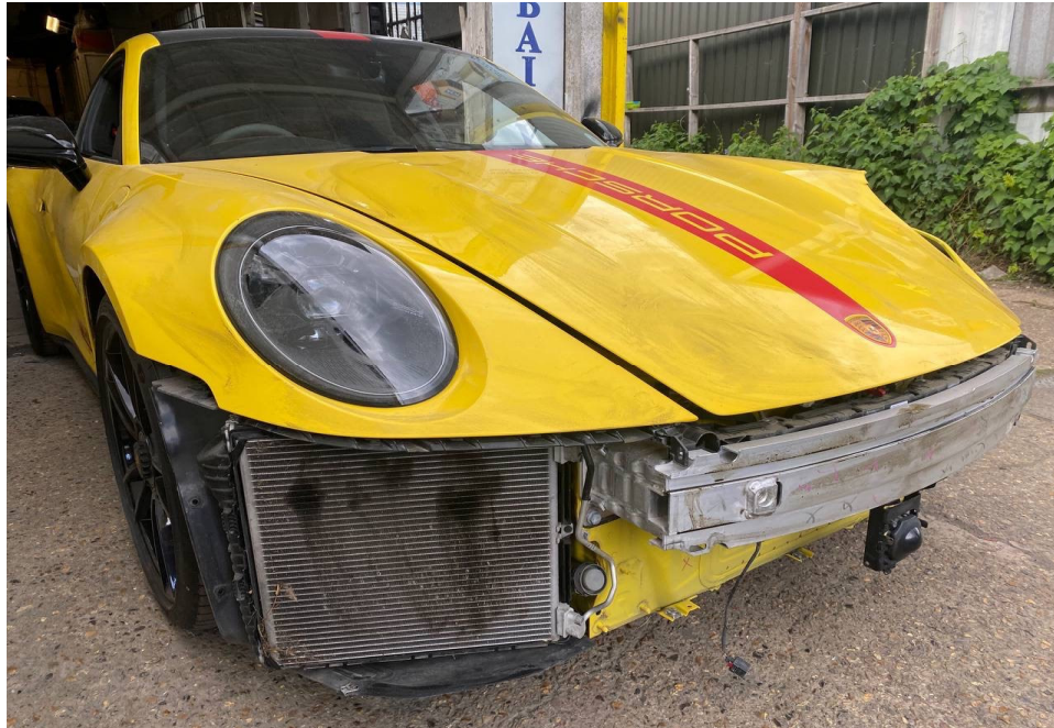
Photo 1 shows a general view of the front right body of the Motor Car (photograph provided to me). The Motor Car's front bumper and all its related parts and attachments like the front bumper lower lip, front bumper right lower grille, front bumper centre air guide, front bumper sensors, front bumper tow cover, front radar unit, front right day light, and front right signal lamp amongst others, were observed to be missing/dislodged/damaged.
