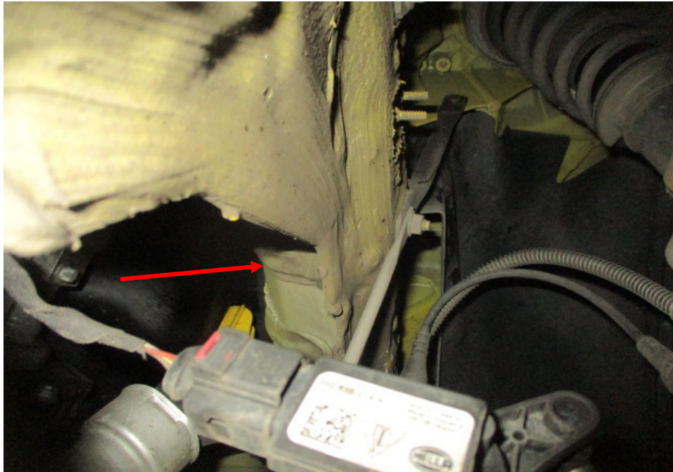
Photo 36 shows the chassis/structural body at the underside front right of the Motor Car. The original factory sealant (arrowed) at the joints along the chassis/structural body was observed to be untouched. In general, I had found no work was carried out on the chassis/structural body of the Motor Car. The chassis/structural body of the Motor Car was originally fitted.
