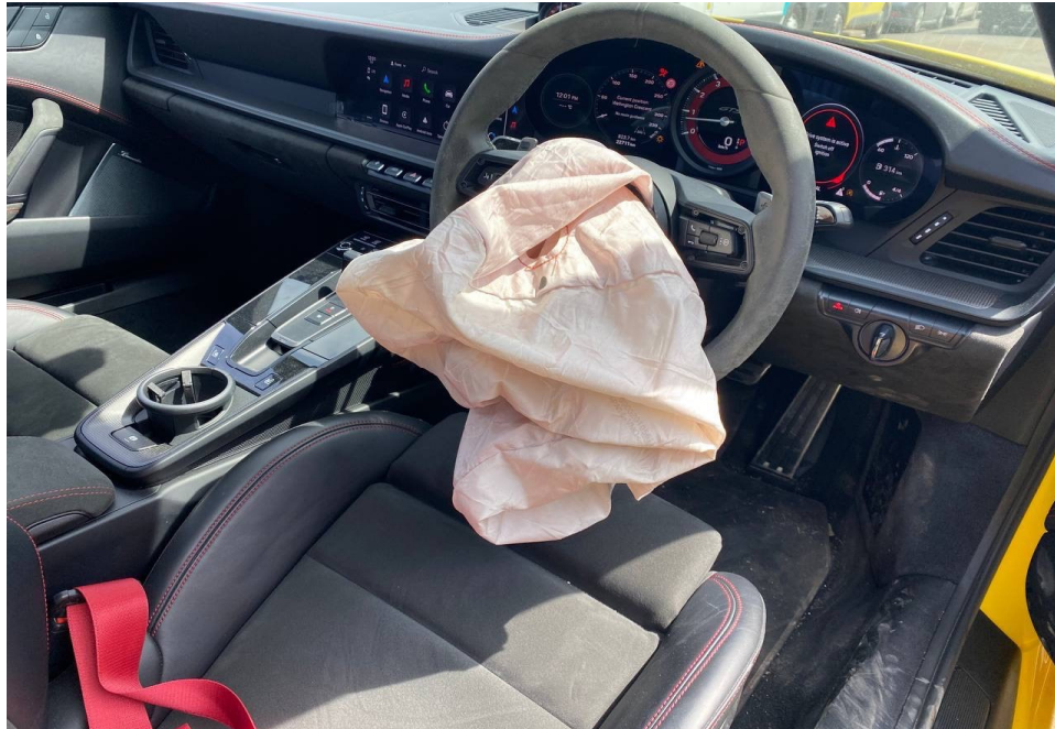
Photo 5 shows the interior compartment of the Motor Car (photograph provided to me). The various parts and components within the interior compartment were all intact and unaffected. The driver's airbag was deployed.
