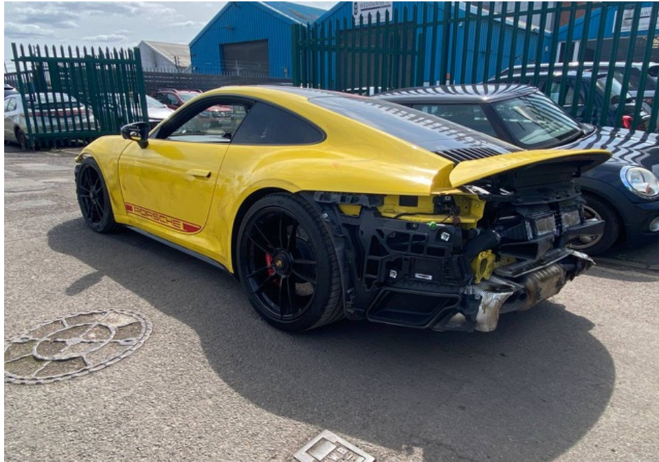
Photo 3 shows a general view of the rear left body of the Motor Car (photograph provided to me). The Motor Car's rear left taillamp, rear centre lamp, rear bumper and all its related parts and attachments like the rear bumper lower cover, rear bumper left reflector, rear bumper sensors, rear bumper tow cover and rear left exhaust garnish amongst others, were missing/dislodged/damaged.
