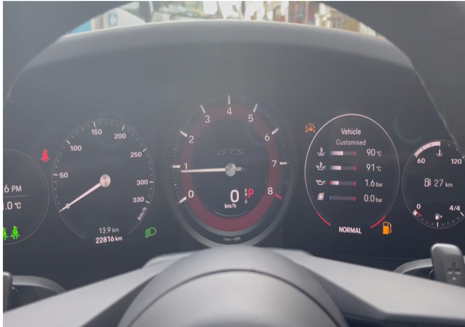
Photo 24 shows the respective warning lights no longer illuminated, indicating that there is no fault detected to the ABS, SRS, EPS, TPM and TCS systems of the Motor Car during the self-test. These electronic systems were hence in working condition at the time of my inspection.
