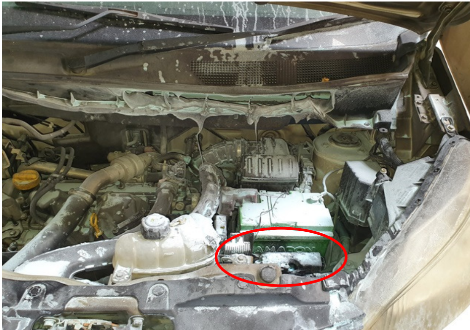
Photo 9 shows the burnt stretches of original factory fitted wirings near the radiator, which is in the immediate vicinity where the fire to the Insured Vehicle had likely started. Faint traces of greenish residue were found on some of the wirings (circled). The presence of such greenish residue suggests occurrence of an electrical short circuit.
