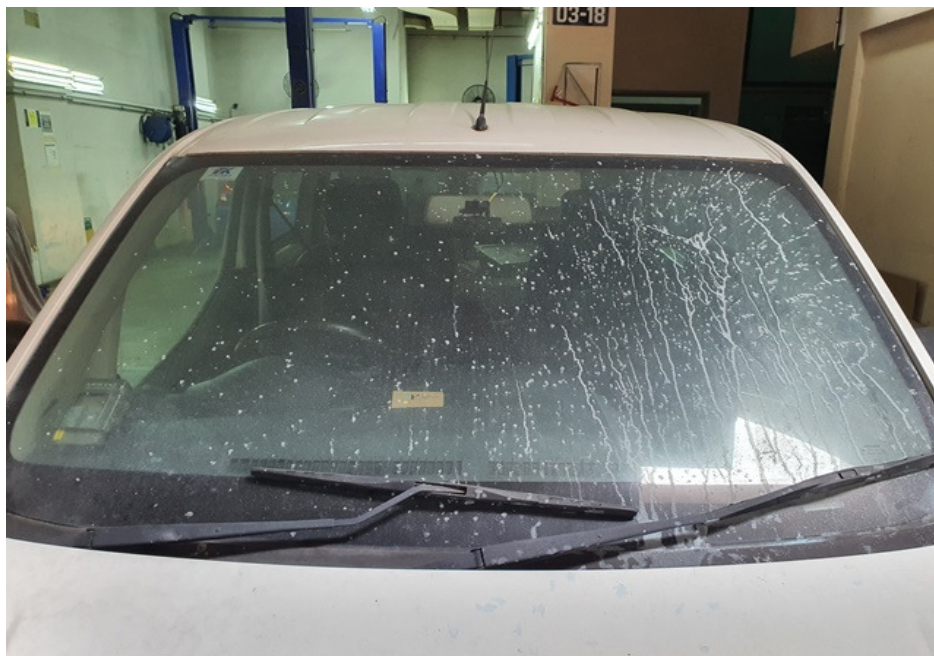
Photo 4 shows the general view of the front windscreen of the Insured Vehicle at the time of our inspection. The fire damage to the front windscreen of the Insured Vehicle was minimal.
