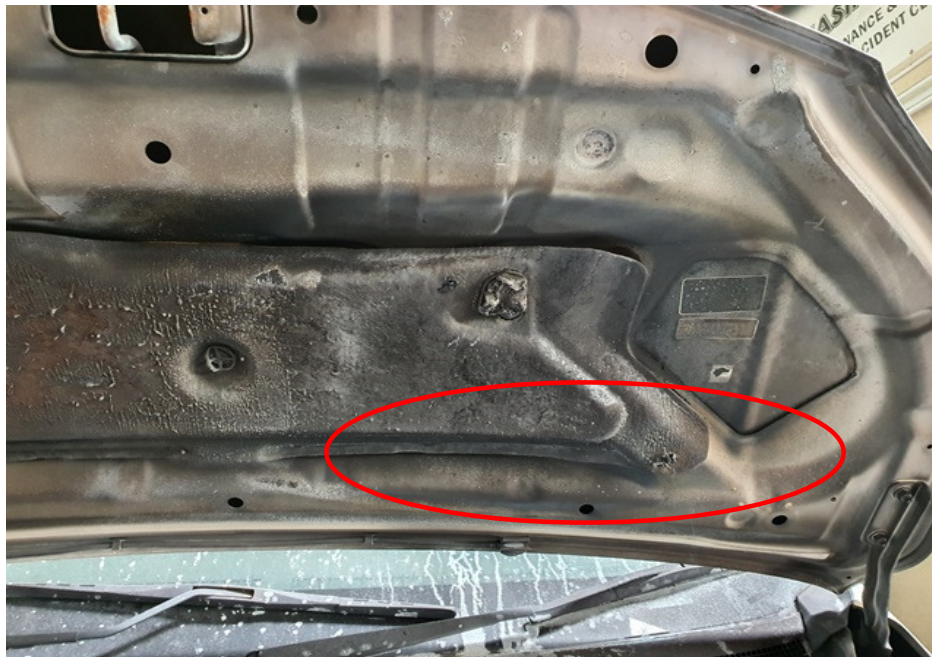
Photo 8 shows the rust that had developed on the underside of the front bonnet, around the left bottom portion (circled). The development of rust is an indication that this area was subjected to prolonged exposure to high heat intensity, which had caused the steel/metal material of the front bonnet to be exposed to natural environmental condition. Hence the fire to the Insured Vehicle can be determined to have originated towards the left centre portion of the engine compartment.
