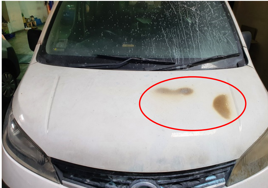
Photo 7 shows the burn pattern and whitish burn marks (circled) that were found on the left centre portion of the front bonnet of the Insured Vehicle. Such whitish burn marks are a result of exposure to prolonged heat intensity, which may indicate where the fire had started. Rust would also begin to develop on these areas soon after the fire.
