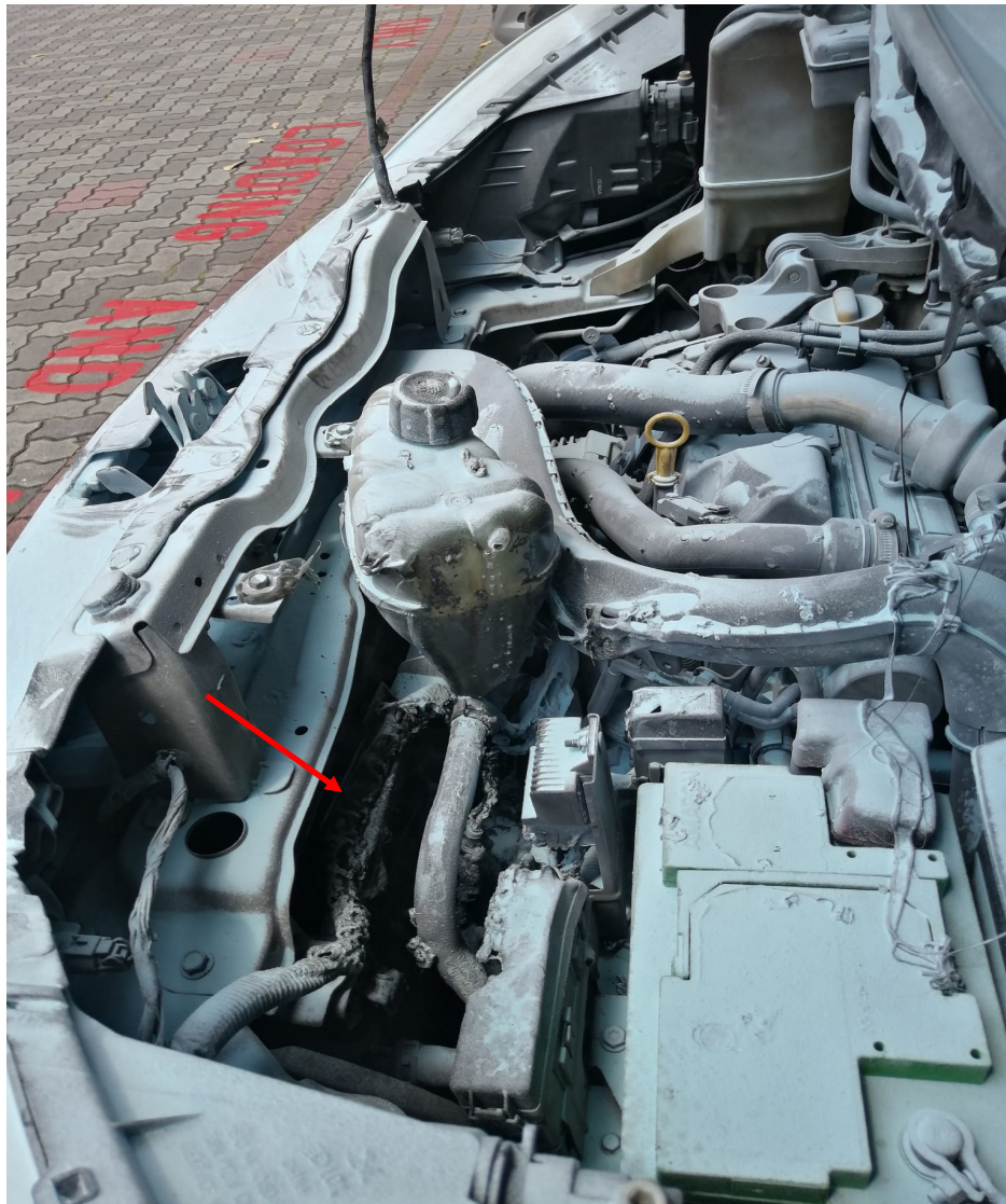
Photo 14 shows the engine compartment of the Insured Vehicle at the incident location post- incident. In general, the information that could be gathered from this photograph had corresponded to the events that were related to us by Mr Nathan, which is the fire to the Insured Vehicle had started from the left portion of the engine compartment (arrowed).
