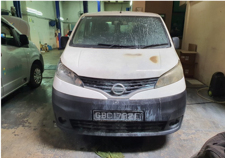
Photo 1 shows the general view of the frontal portion of the Insured Vehicle at the time of our inspection. The fire damage to the Insured Vehicle was confined to its frontal portion. Its front windscreen, front bonnet, front bumper and left front headlamp were amongst the body parts that were found to have been affected as a result of the fire.
