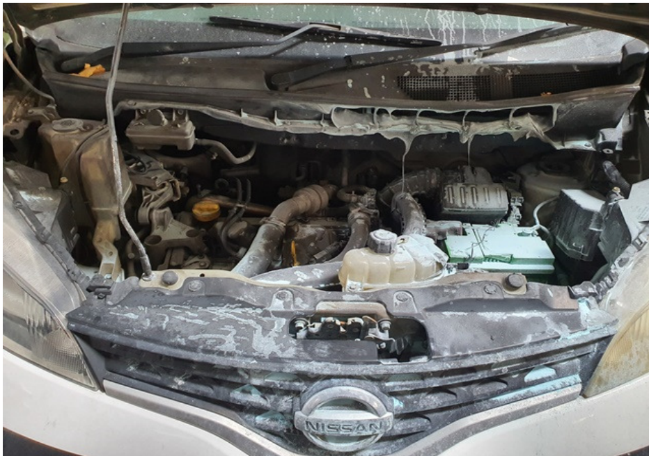
Photo 6 shows a general view of the engine compartment of the Insured Vehicle which was covered in fire extinguisher residue at the time of our inspection. Most of its engine components were found to have been affected as a result of the fire.
