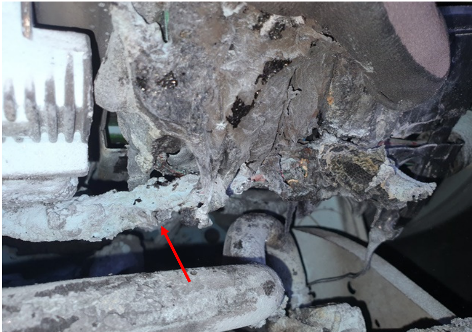
Photo 11 shows a close up view of the wirings under the fuse box of the Insured Vehicle which had partially melted (arrowed).
