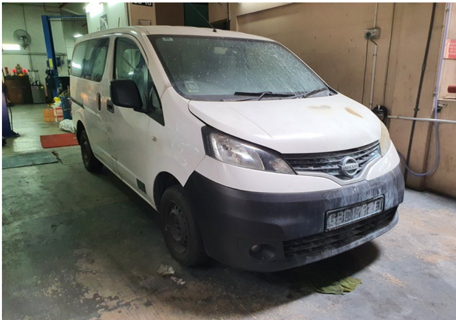
Photo 2 shows the general view of the right body of the Insured Vehicle at the time of our inspection. The fire damage to the Insured Vehicle was confined to its frontal portion. The right body was found to have been relatively unaffected by the fire.
