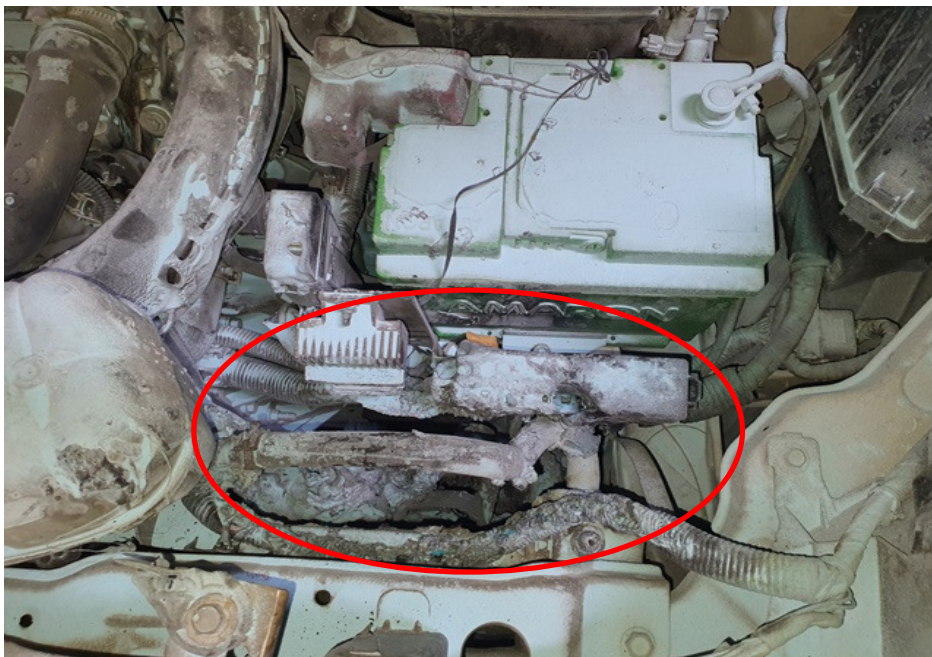
Photo 10 shows a closer view of the burnt stretches of original factory fitted wirings near the radiator, which is in the immediate vicinity where the fire to the Insured Vehicle had likely started (circled).
