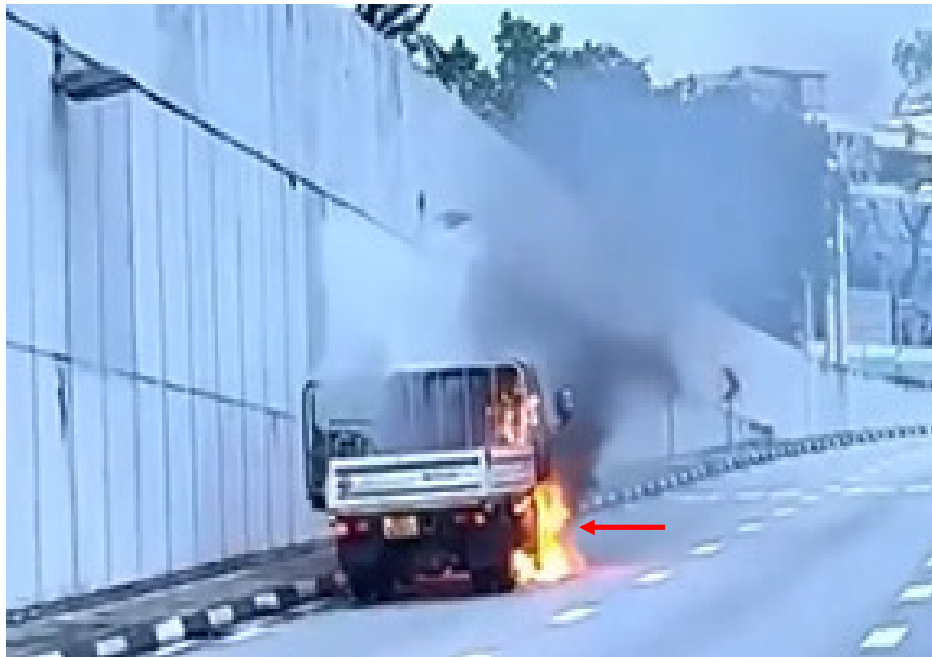
Photo 10 shows the Insured Vehicle on fire before the arrival of the SCDF. In general, the information that could be gathered from this photograph had corresponded to the events that were related to us by Mr Tay, which is the fire had started from the engine compartment (arrowed).
