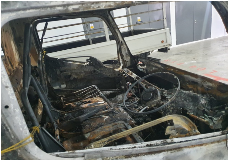
Photo 4 shows the interior compartment the Insured Vehicle at the time of our inspection. The interior compartment of the Insured Vehicle was severely affected by the fire.
