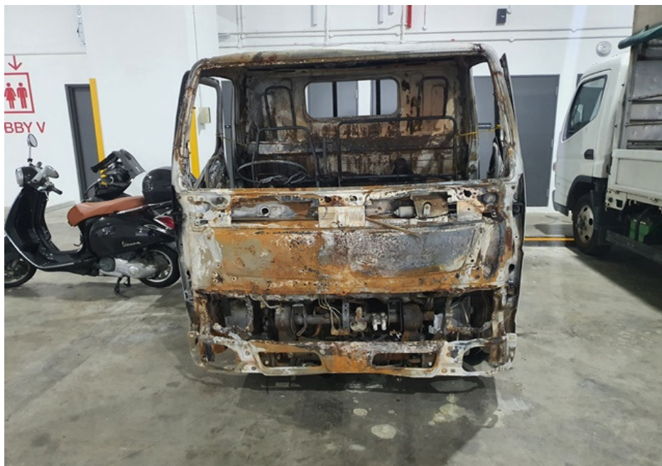
Photo 2 shows the frontal portion of the Insured Vehicle at the time of our inspection. The damage to the Insured Vehicle was confined to its frontal portion. The exterior body of the Insured Vehicle was relatively unaffected by the incident except for the frontal portion.
