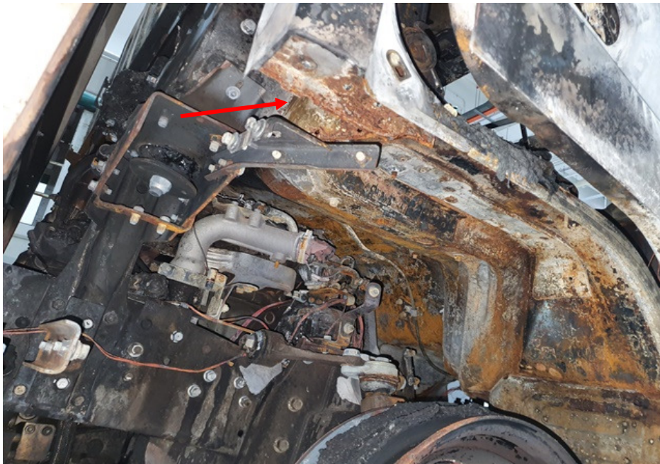
Photo 7 shows the rust that had developed on the underside of the cab of the Insured Vehicle (arrowed) which is an indication that the fire to the Insured Vehicle had originated from the engine compartment. The development of rust is an indication that the area was exposed to prolonged exposure to high heat intensity, which had caused the steel/metal material of the cab to be exposed to natural environmental condition.
