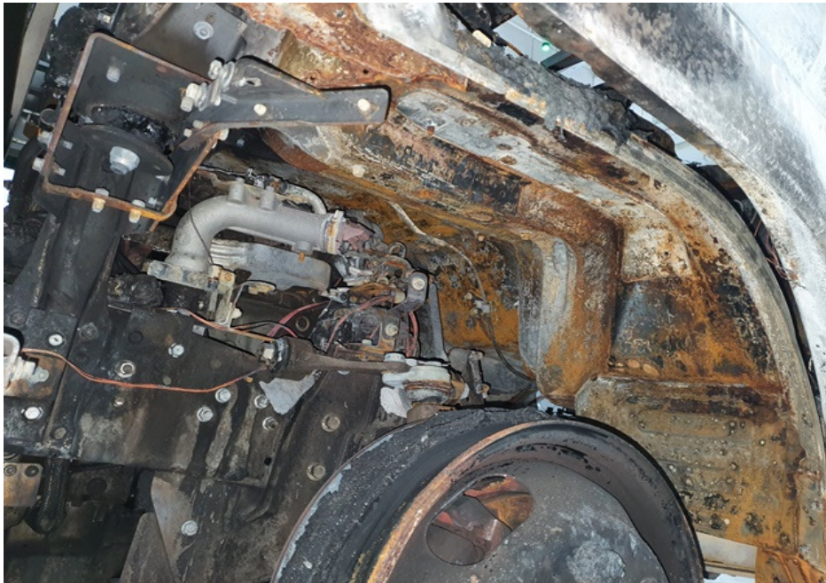
Photo 5 shows the engine compartment of the Insured Vehicle which is situated beneath the cab at the time of our inspection. The engine compartment of the Insured Vehicle was severely affected by the fire. Most of the components inside the engine compartment were found to be severely burnt and/or melted as a result of the fire.
