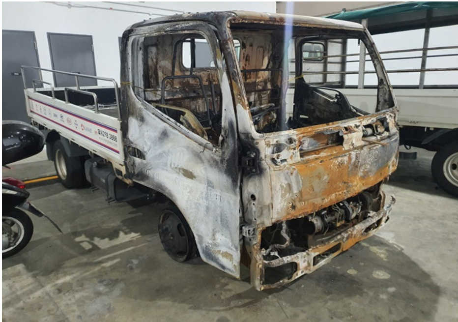
Photo 3 shows the right frontal portion of the Insured Vehicle at the time of our inspection. The exterior body of the Insured Vehicle was relatively unaffected by the incident except for the frontal portion.
