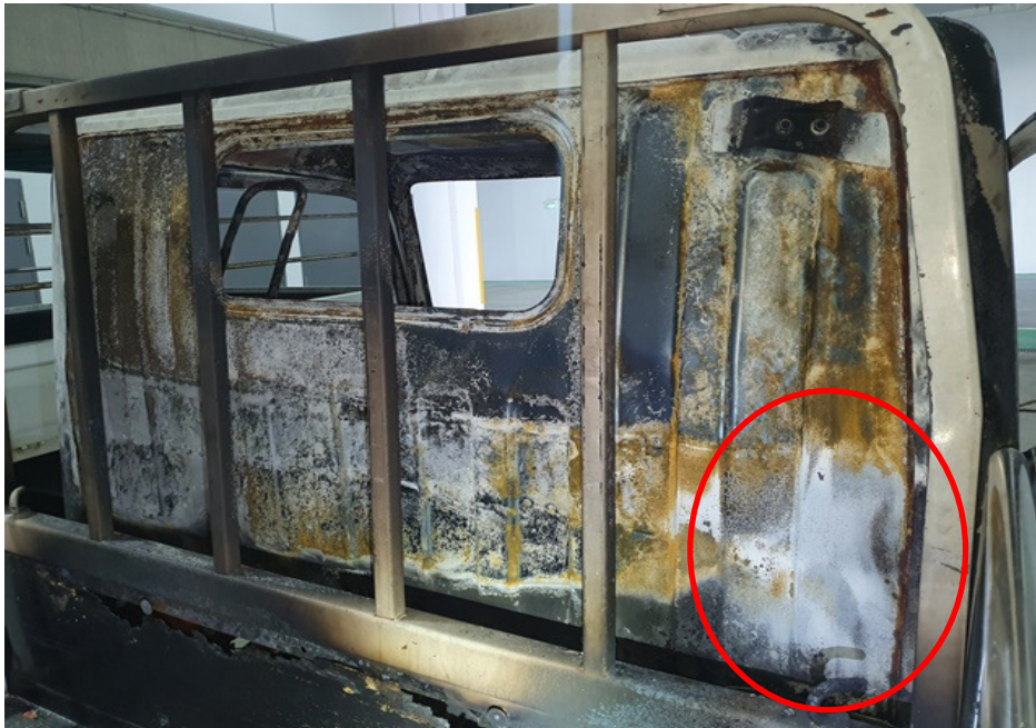
Photo 6 shows the whitish burn marks that were found on the rear right portion of the cab of the Insured Vehicle (circled). Such whitish burn marks are a result of exposure to prolonged heat intensity.
