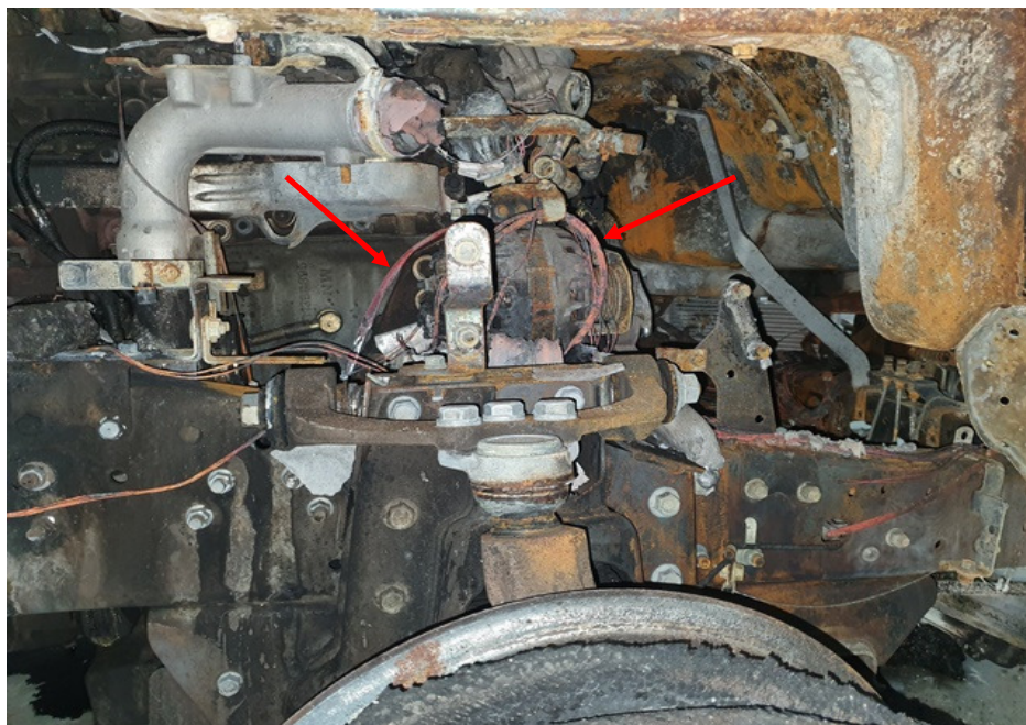
Photo 8 shows the wirings around the right side of the engine compartment, which is in the immediate vicinity where the fire to the Insured Vehicle had likely started. The wirings (red arrows) were found to have been burnt internally to its bare copper state, suggesting occurrence of an electrical short circuit.
