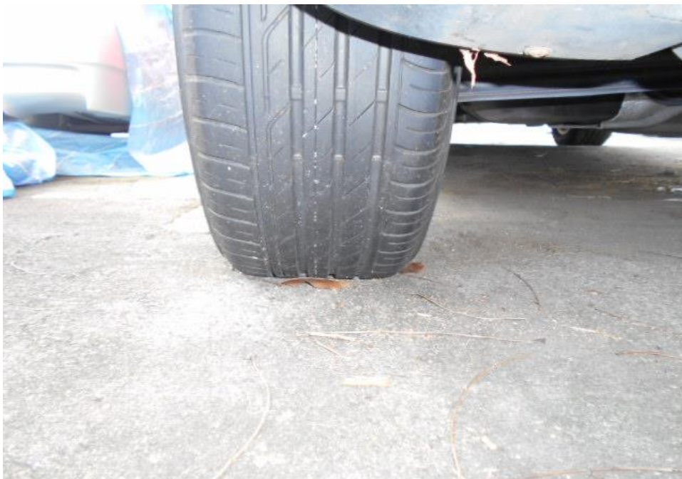
Photo 10 shows the condition of the rear left tyre of the Motor Car, which was observed to be in serviceable condition with remaining tread depth of approximately 6.2mm. The tyre was also observed to be sufficiently inflated for vehicular operation with no tear, cut or burst mark(s).
