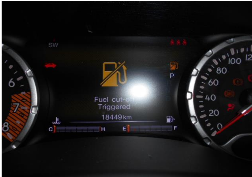
Photo 24 shows the Fuel cut-off Triggered warning lights illuminated on the instrument panel as a result of the accident, this had prevented me from starting up the Motor Car to conduct the automatic self-test of the functionality of its electronic operating systems like the ABS, TCS, SRS and etc.
