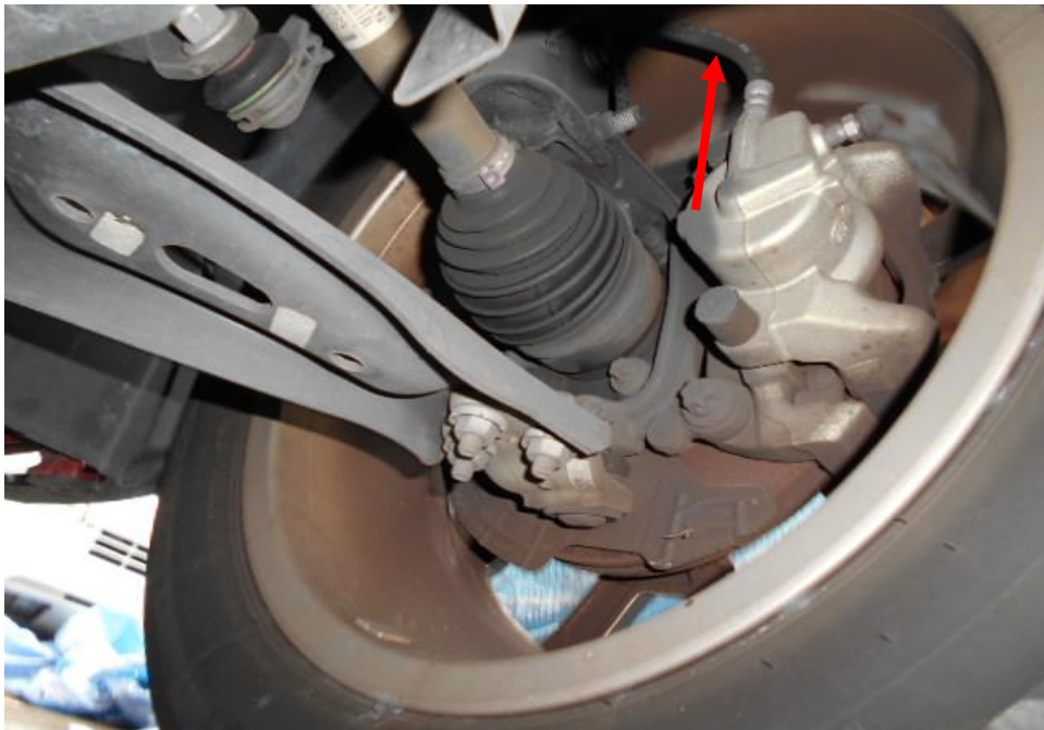
Photo 22 shows the brake hose/pipe (arrowed) at the front left wheel of the Motor Car. No leakage of brake fluid was observed. Visual examination of the various components of the braking system like the disc brake, brake booster, brake pedal etc. had revealed all to be intact and without visible damage.
