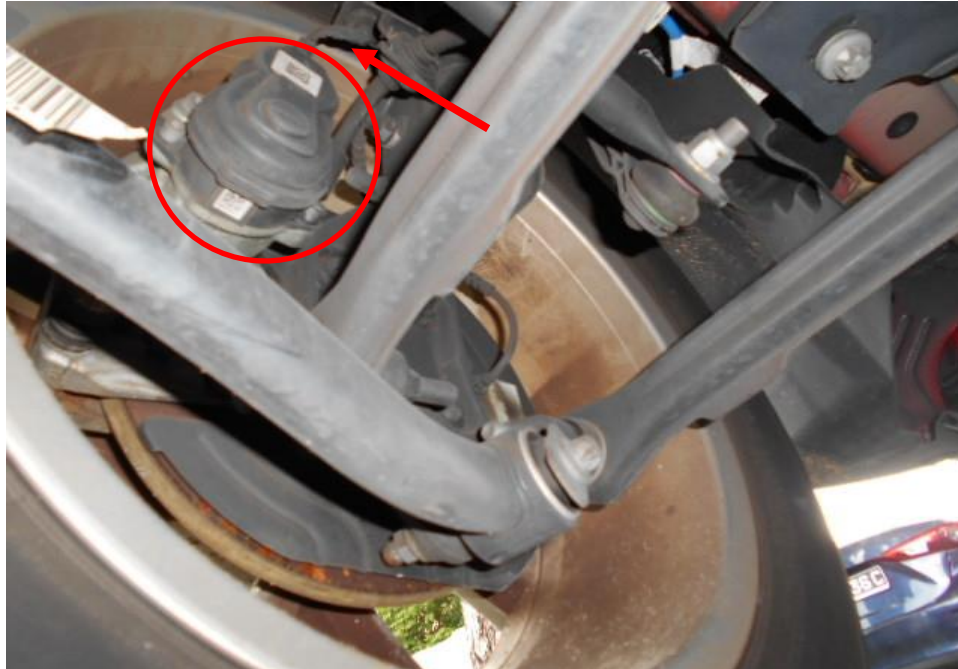
Photo 20 shows the brake hose/pipe (arrowed) at the rear left wheel of the Motor Car. No leakage of brake fluid was observed. Visual examination of the various components of the braking system like the brake caliper (circled), brake booster, brake pedal etc had revealed all to be intact and without visible damage.
