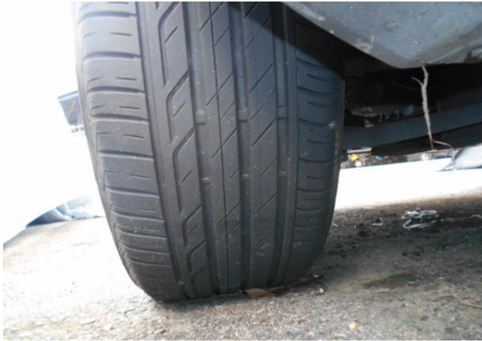
Photo 11 shows the condition of the front left tyre of the Motor Car, which was observed to be in serviceable condition with remaining tread depth of approximately 6.5mm. The tyre was also observed to be sufficiently inflated for vehicular operation with no tear, cut or burst mark(s).
