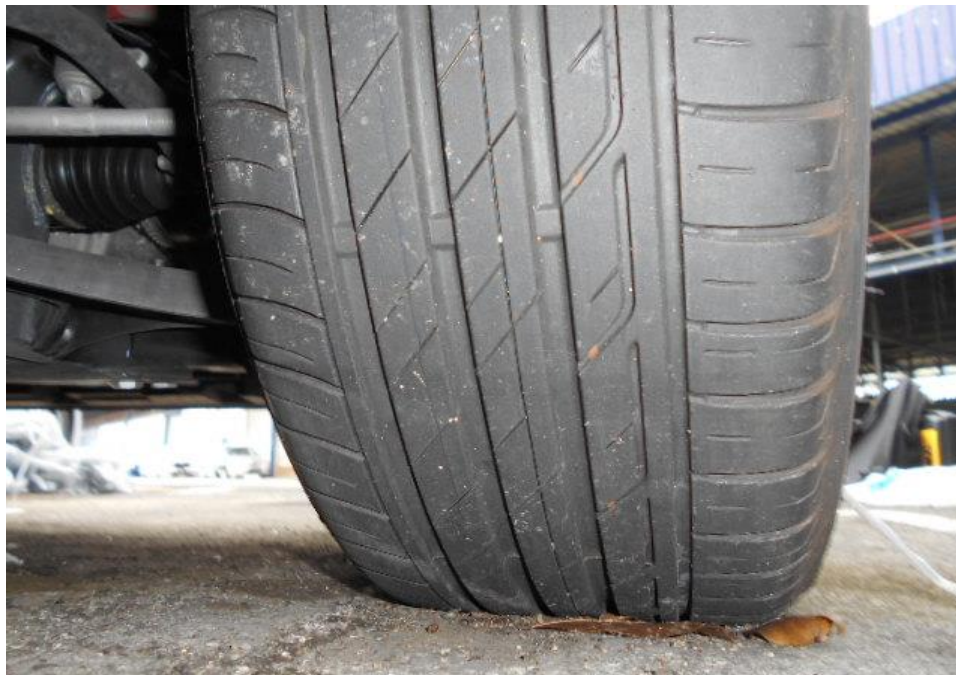
Photo 8 shows the condition of the front right tyre of the Motor Car, which was observed to be in serviceable condition with remaining tread depth of approximately 6.6mm. The tyre was also observed to be sufficiently inflated for vehicular operation with no tear, cut or burst mark(s).
