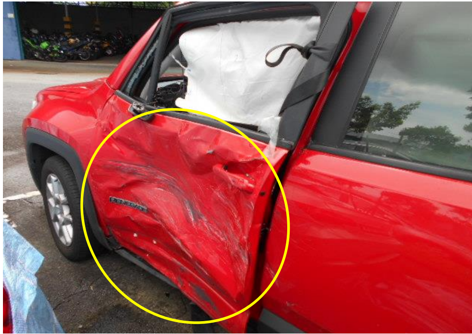
Photo 5 shows the close up view of the Motor Car's left body at the time of my inspection. The Motor Car was observed to have sustained damage at its left portion. Its left front door (circled) was damaged as a result of the accident.
