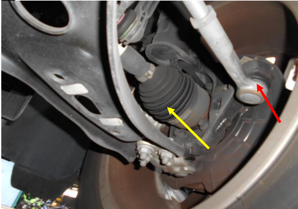
Photo 17 shows the various undercarriage components at the front right wheel of the Motor Car, in particular the steering tie rod (red arrow) and the driveshaft (yellow arrow). The various steering components were all found to be intact, suggesting that the steering system of the Motor Car was likely to be in serviceable condition at the material time of accident. There was also no sign of fluid stain observed on the various undercarriage components at the front right wheel of the Motor Car.
