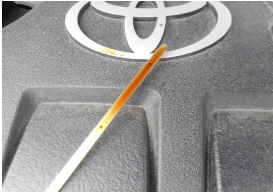
Photo 19 shows the engine oil dipstick of the Motor Car at the time of my inspection. The engine oil was observed to be of sufficient level and without any visible contamination.
