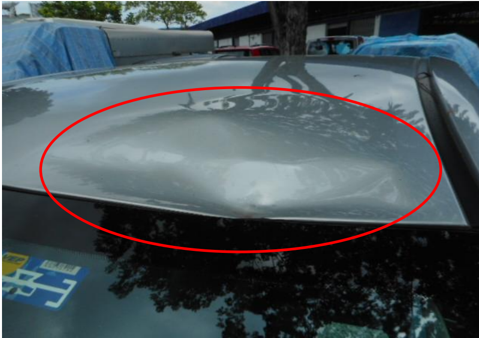
Photo 8 shows a close up view of the Motor Car's roof at the time of my inspection. The roof portion of the Motor Car was observed to have sustained damage. Its roof (circled) was amongst the body parts that were damaged as a result of the accident.
