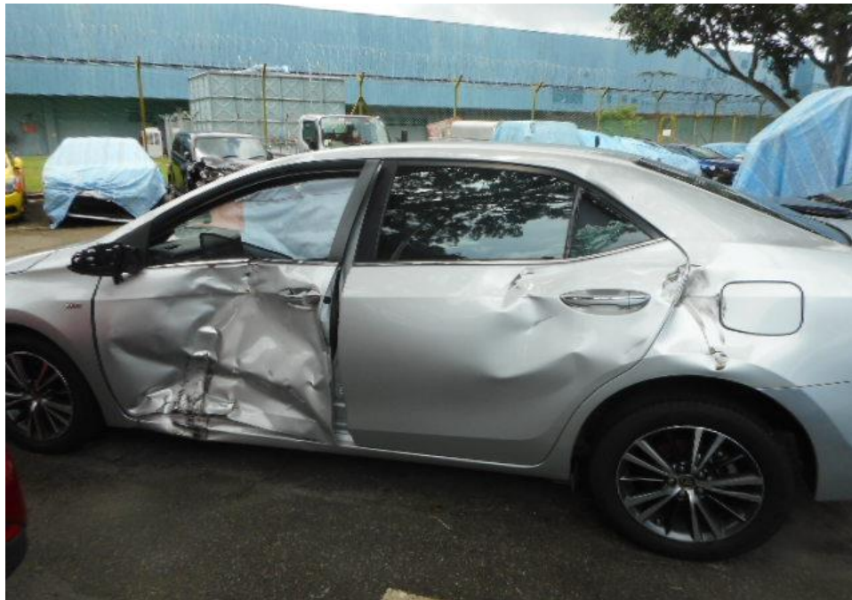
Photo 3 shows a general view of the Motor Car's left body at the time of my inspection. The left portion of the Motor Car was observed to have sustained damage. Its left rear view mirror, left doors, left side windscreen, left quarter body panel and its roof was amongst the body parts that were damaged as a result of the accident. The Supplemental Restraint System (SRS) was activated as a result of the accident.
