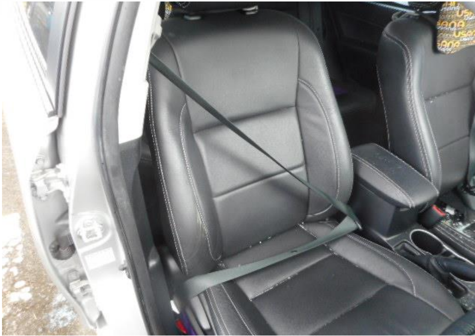
Photo 30 shows that the seat belt on the right seat was able to be fastened securely into the respective pre-tensioners that were fitted at the sides of each seat.
