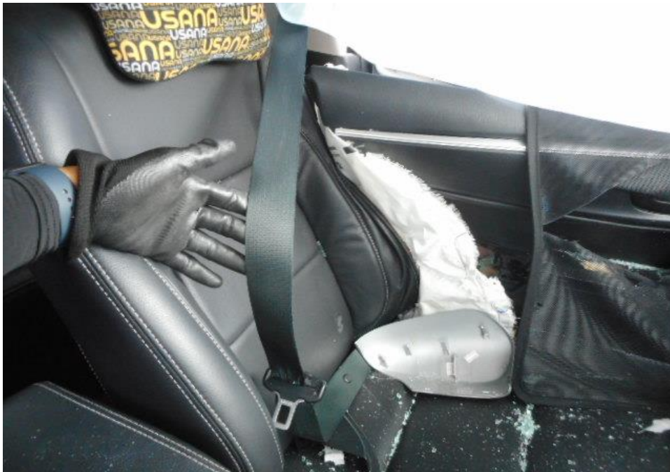
Photo 31 shows that the seat belt on the left seat was worn at the material time of accident as the safety pre-tensioners was activated at the moment of impact and caused the seat belt to be locked into the last position.
