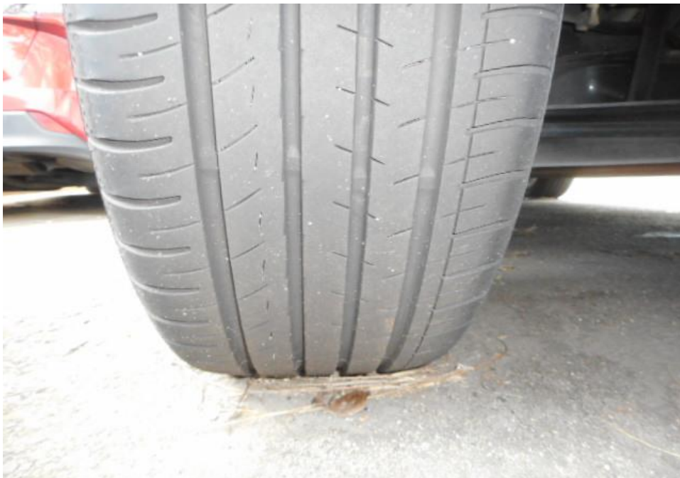
Photo 13 shows the condition of the rear left tyre of the Motor Car, which was observed to be in serviceable condition with remaining tread depth of approximately 4.6mm. The tyre, which was wrapped around alloy wheel rim, was also observed to be sufficiently inflated for vehicular operation. The 4 tyres of the Motor Car were wrapped around standard alloy wheel rims.
