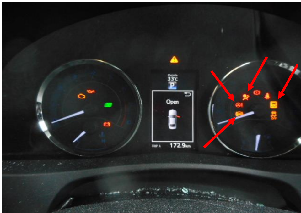
Photo 28 shows the warning light for Anti-Lock Brake System (ABS), Traction Control System (TCS), Electric Power Steering System (EPS), and Supplemental Restraint System (SRS) (arrowed) appearing on the instrument panel of the Motor Car during the self-test of its various electronic operating systems when its engine was cranked.
