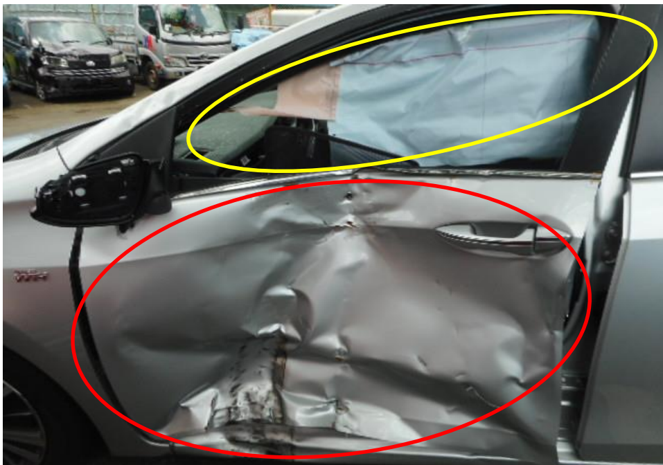
Photo 5 shows a close up view of the Motor Car's left body at the time of my inspection. The left portion of the Motor Car was observed to have sustained damage. Its left windscreen (yellow circle) and its left door (red circle) was the body parts that were damaged as a result of the accident.
