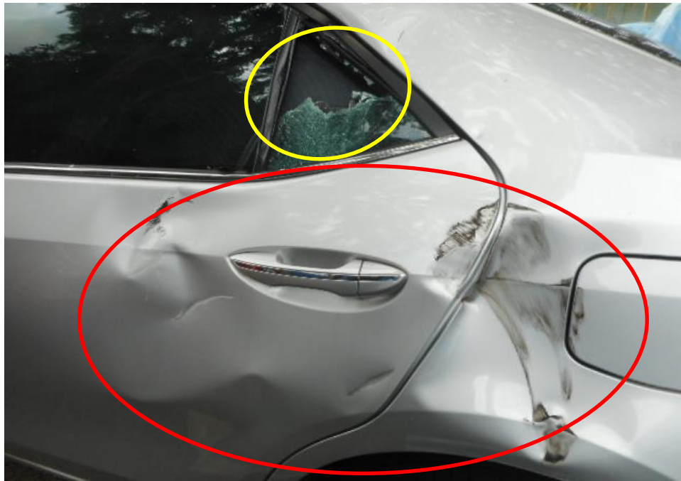
Photo 6 shows a close up view of the Motor Car's left body at the time of my inspection. The left portion of the Motor Car was observed to have sustained damage. Its left door, its left quarter body panel (red circle) and its left windscreen (yellow circle) and was the body parts that were damaged as a result of the accident.
