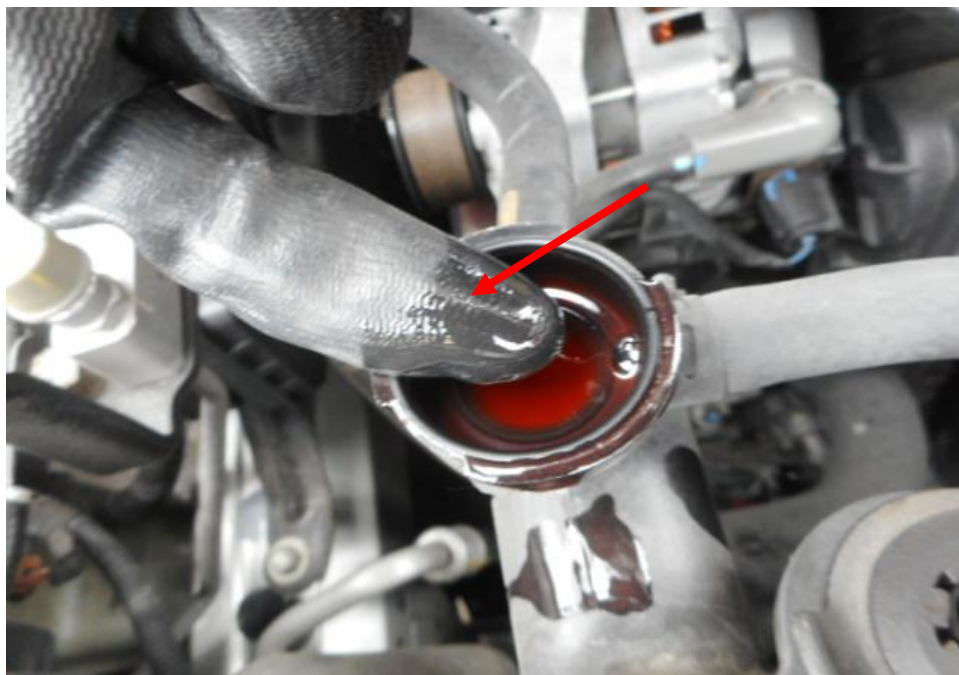
Photo 18 shows checks being carried out to the engine coolant of the Motor Car at the time of my inspection. The engine coolant was observed to be of sufficient level (arrowed) and without any visible contamination.
