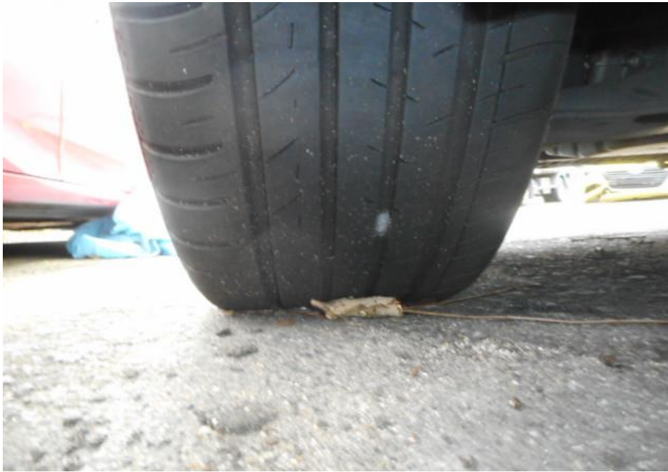
Photo 14 shows the condition of the front left tyre of the Motor Car, which was observed to be in serviceable condition with remaining tread depth of approximately 4.6mm. There was also no tear, cut or burst mark(s) on the outer and the inner sidewalls as well as across the tread of the Motor Car's 4 tyres.
