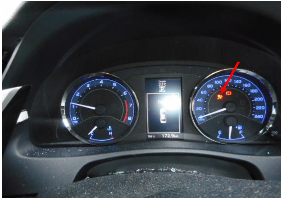
Photo 29 shows only the Supplemental Restraint System (SRS) remained illuminated on as due to the deployment of the Airbag as a result of the accident. No other warning lights illuminated on the instrument panel of the Motor Car after the engine was cranked. This would suggest that there was no abnormality to the electronic operating system of the Motor Car, like the ABS, TCS, EPS and etc.
