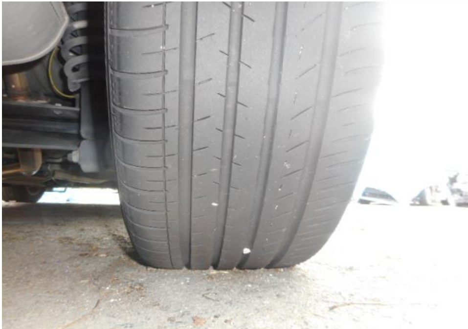
Photo 12 shows the condition of the rear right tyre of the Motor Car, which was observed to be in serviceable condition with remaining tread depth of approximately 5.2mm. The tyre was also observed to be sufficiently inflated for vehicular operation with no tear, cut or burst mark(s).
