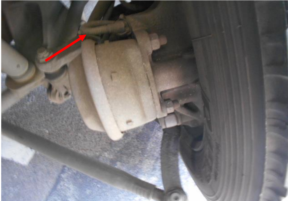
Photo 17 shows the brake pipe (arrowed) at the front right wheel of the Motor Bus. I did not observe any leakage of brake fluid at the time of my inspection of the Motor Bus. My static tests of the Motor Bus's braking system, along with my visual examination of the various mechanical components in the braking system, had indicated that there was no internal leakage of pressure/vacuum. Hence the braking system of the Motor Bus was likely to be in serviceable condition at the material time of accident.
