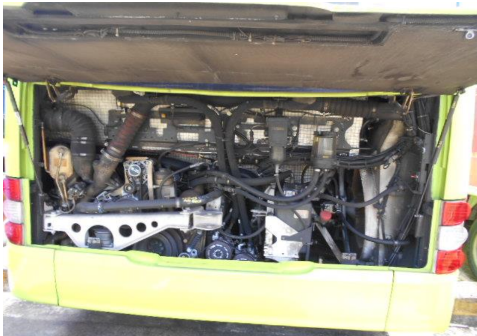
Photo 10 shows a general view of the Motor Bus's engine compartment, which was accessed by lifting the rear of the Motor Bus. The various parts and components inside the engine compartment were unaffected by the accident. There was also no sign(s) or indication(s) of fresh fluid leakage and/or fluid stain within the engine compartment
