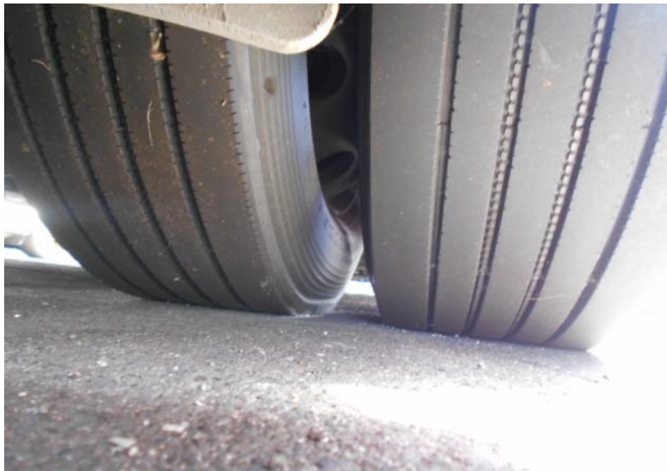
Photo 7 shows the condition of the rear right tyre of the Motor Bus, which was observed to be in serviceable condition with remaining tread depth of approximately 9.6mm. The tyre, which was wrapped around standard steel wheel rim, was also observed to be sufficiently inflated for vehicular operation.
