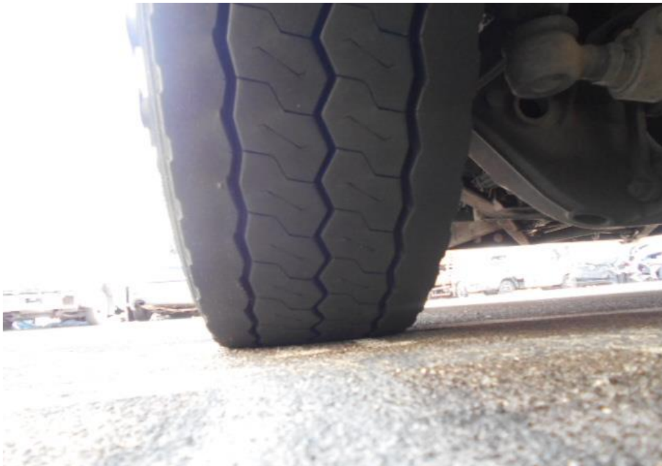
Photo 9 shows the condition of the front left tyres of the Motor Bus, which were observed to be in serviceable condition with remaining tread depth of approximately 12.6mm. There was also no tear, cut or burst mark(s) on the outer and the inner sidewalls as well as across the tread of the 6 tyres that were fitted on the Motor Bus.
