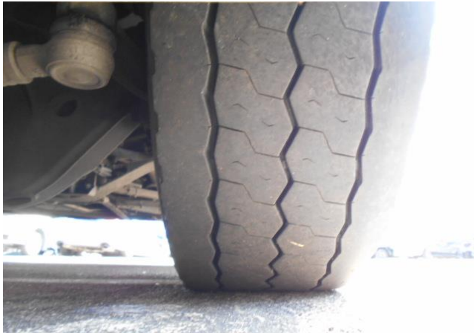
Photo 6 shows the condition of the front right tyre of the Motor Bus, which was observed to be in serviceable condition with remaining tread depth of approximately 13.2mm. The tyre, which was wrapped around standard steel wheel rim, was also observed to be sufficiently inflated for vehicular operation. There was no tear, cut or burst mark(s) on the outer and the inner sidewalls as well as across the tread of the 6 tyres that were fitted on the Motor Bus.
