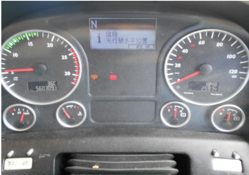
Photo 25 shows no warning lights illuminated on the instrument panel of the Motor Bus after the engine was cranked. This would suggest that there was no abnormality to the various electronic operating systems of the Motor Bus, like the TCS, ABS and etc.
