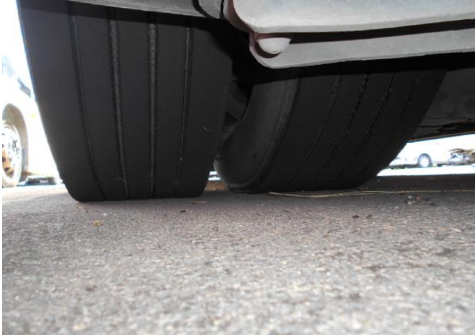
Photo 8 shows the condition of the rear left tyres of the Motor Bus, which was observed to be in serviceable condition with remaining tread depth of approximately 9.4mm. The tyres, which were wrapped around standard steel wheel rim, were also observed to be sufficiently inflated for vehicular operation. There was also no damage found on all 6 steel wheel rims of the Motor Bus.
