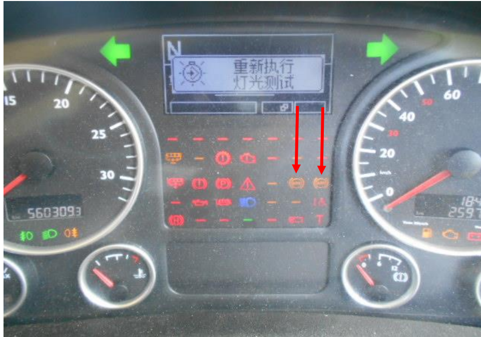
Photo 24 shows the warning light for Traction Control System (TCS) and Anti-Lock Braking System (ABS) appearing on the instrument panel of the Motor Bus during the self-test of its various electronic operating systems when its engine was cranked.
