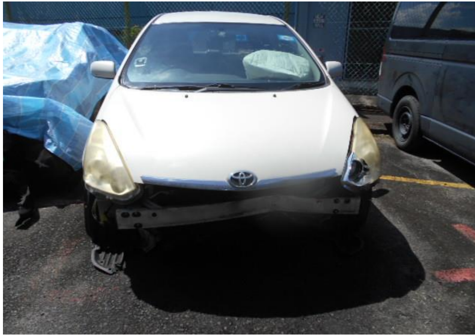
Photo 1 shows a general view of the Motor Car's front body at the time of my inspection. The front bumper which was observed to be missing, front windscreen, and front left headlamp was amongst the body parts that were damaged as a result of the accident. The Supplemental Restraint System (SRS) was activated as a result of the accident.
