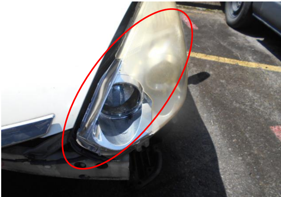
Photo 4 shows the close up view of the Motor Car's front body at the time of my inspection. The Motor car was observed to have sustained damage at its front portion. Its front left headlamp (circled) was damaged as a result of the accident.
