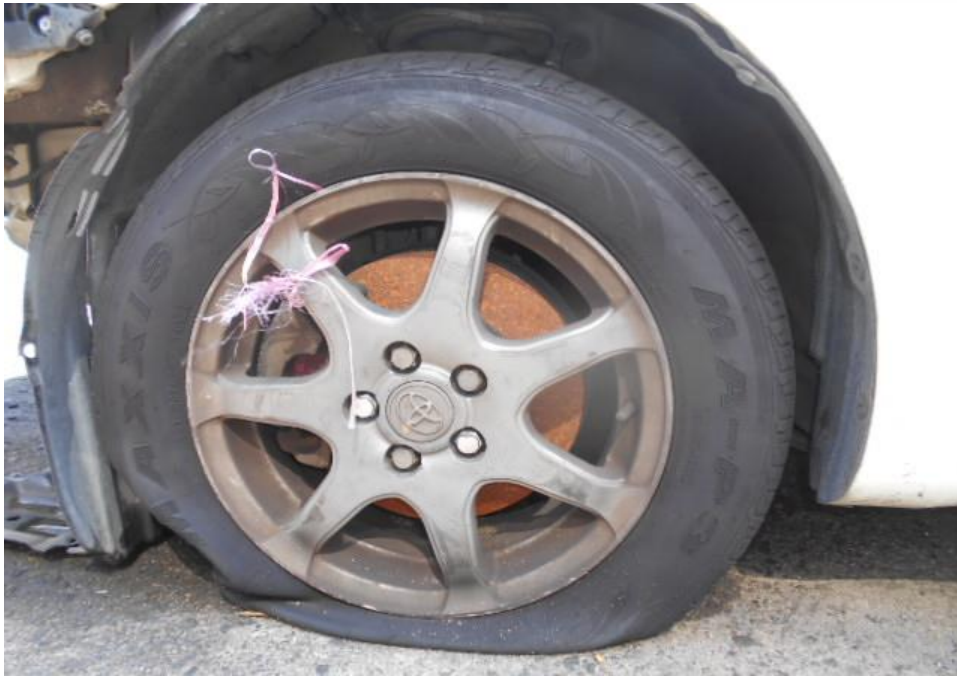
Photo 11 shows the condition of the front left tyre of the Motor Car, which was observed to be in unserviceable condition with remaining tread depth of approximately 5.9mm. The tyre was also observed to be deflated as a result of the damaged wheel rim as a result of the accident, however there was no tear, cut or burst mark(s) on the tyre.
