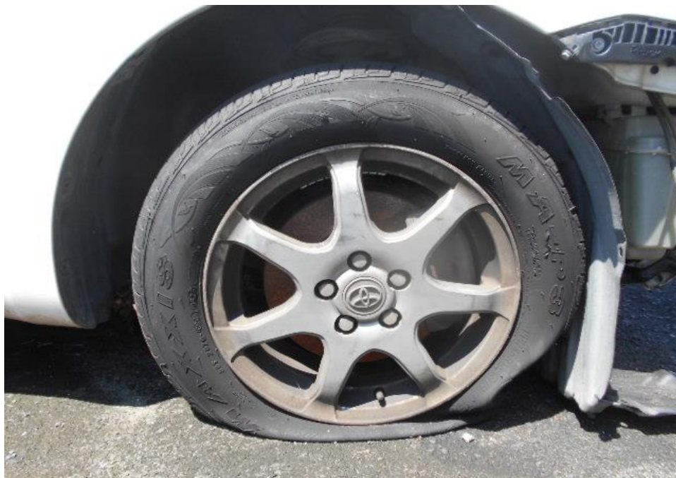
Photo 8 shows the condition of the front right tyre of the Motor Car, which was observed to be in unserviceable condition with remaining tread depth of approximately 5.8mm. The tyre was also observed to be deflated as a result of the damaged wheel rim as a result of the accident, however there was no tear, cut or burst mark(s) on the tyre.
