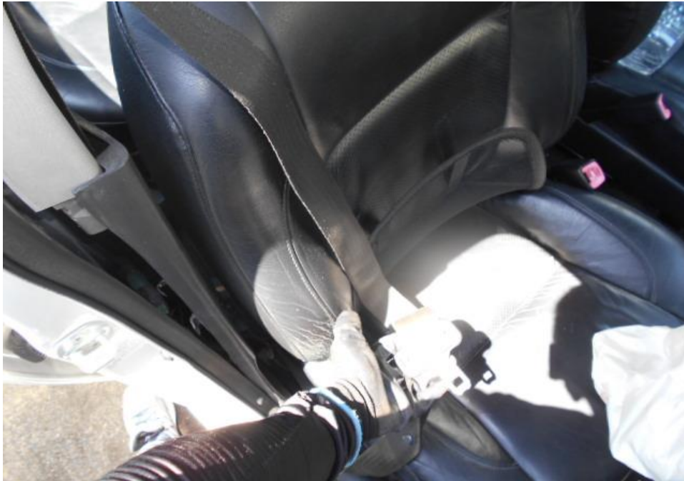
Photo 22 shows that the seat belt on the right seat was worn at the material time of accident as the safety pre-tensioners was activated at the moment of impact and caused the seat belt to be locked into the last position.
