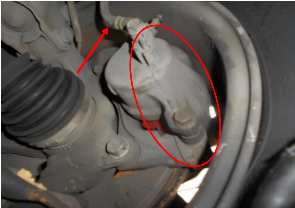
Photo 19 shows the brake hose/pipe (arrowed) at the front left wheel of the Motor Car. No leakage of brake fluid was observed. Visual examination of the various components of the braking system like the brake caliper (circled) had revealed to be intact and without visible damage.
