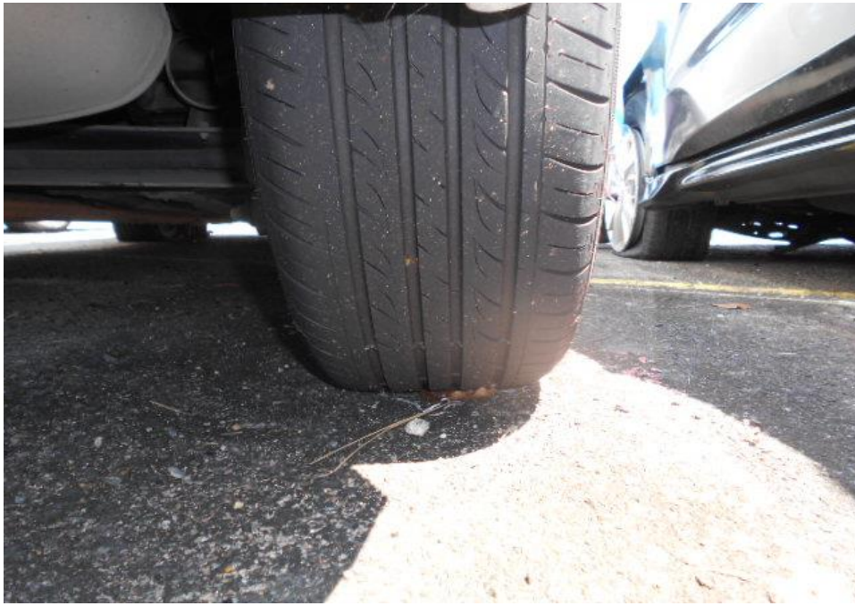
Photo 9 shows the condition of the rear right tyre of the Motor Car, which was observed to be in serviceable condition with remaining tread depth of approximately 5.9mm. The tyre was also observed to be sufficiently inflated for vehicular operation with no tear, cut or burst mark(s).
