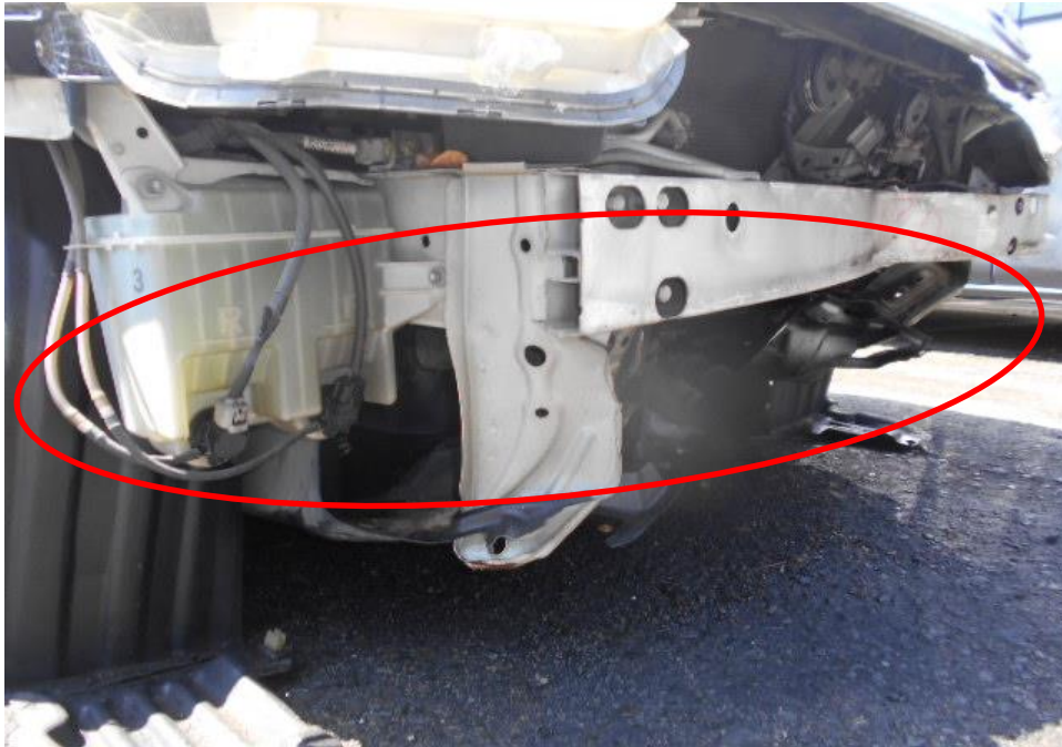
Photo 3 shows the close up view of the Motor Car's front body at the time of my inspection. The Motor car was observed to have sustained damage at its front portion. Its front bonnet (circled) was missing as a result of the accident.
