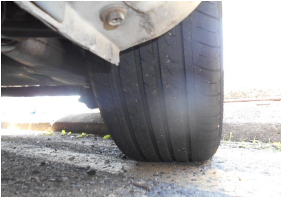
Photo 10 shows the condition of the rear left tyre of the Motor Car, which was observed to be in serviceable condition with remaining tread depth of approximately 5.1mm. The tyre was also observed to be sufficiently inflated for vehicular operation with no tear, cut or burst mark(s).
