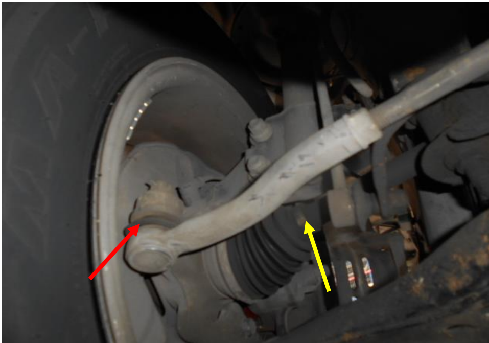
Photo 20 shows the various undercarriage components at the front right wheel of the Motor Car, in particular the steering tie rod (red arrow) and the driveshaft (yellow arrow). The various steering components were all found to be intact. There was also no sign of fluid stain observed on the various undercarriage components at the front right wheel of the Motor Car.
