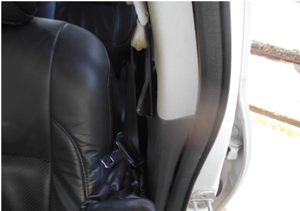
Photo 23 shows that the seat belt on the left seat as the safety pre-tensioners was activated at the moment of impact and caused the seat belt to be locked into the last position.
