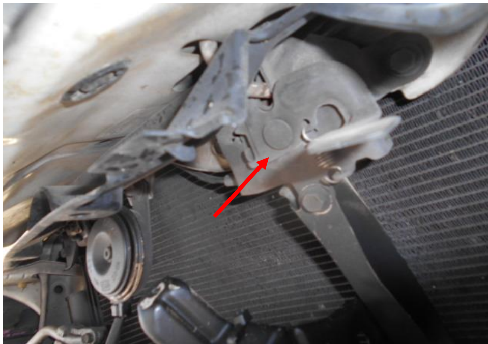
Photo 13 shows the close up view of the damaged front bonnet lock mechanism (arrowed) and the structure of the engine compartment of the Motor Car at the time of my inspection resulting it unable to open a result of the accident. (Unable to open)
