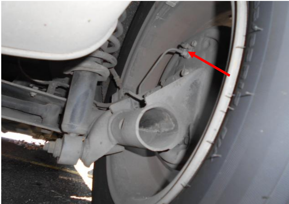
Photo 17 shows the brake hose/pipe (arrowed) at the rear right wheel of the Motor Car. No leakage of brake fluid was observed. Visual examination of the various components of the braking system like the brake drum to be intact and without visible damage.
