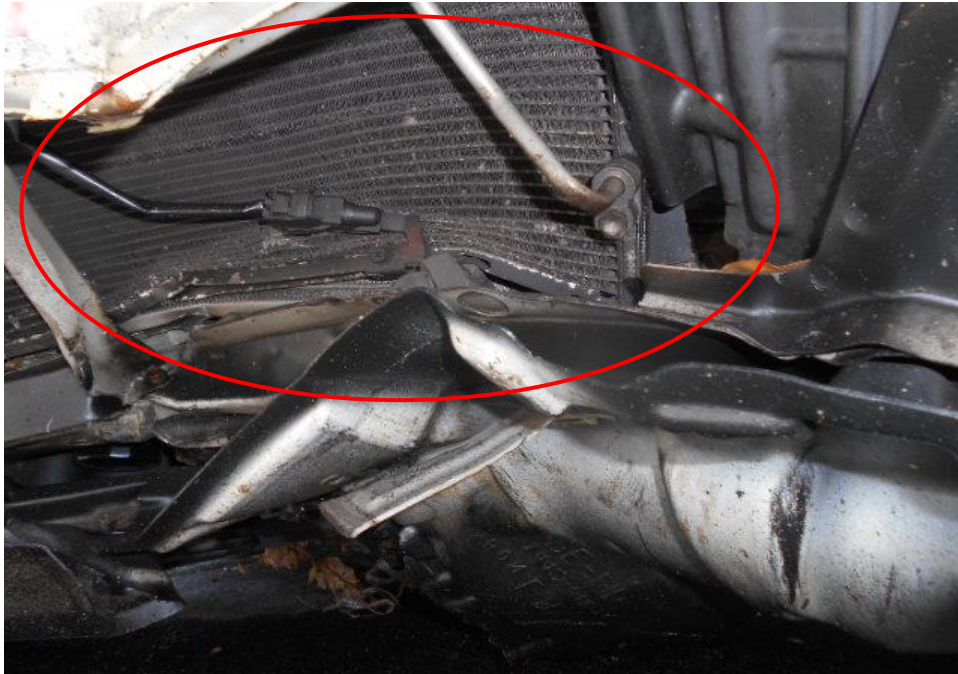
Photo 14 shows checks being carried out to the engine coolant of the Motor Car at the time of my inspection. The engine coolant radiator (circled) was damaged as a result of the accident.
