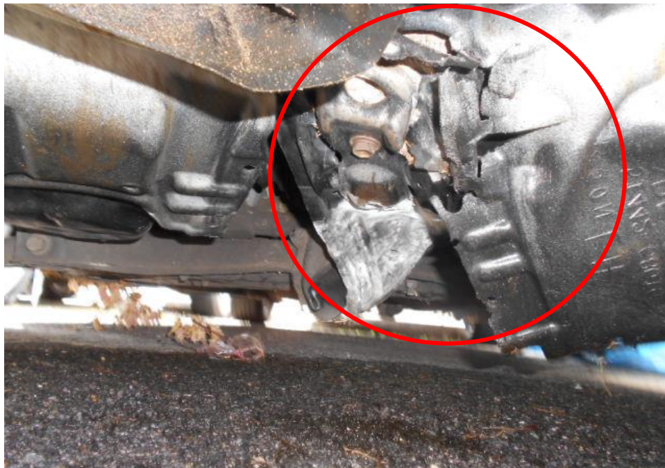
Photo 15 shows the undercarriage of the Motor Car, at the area where the engine housing and transmission housing are located. The transmission housing (circled) was observed to be damaged as a result of the accident, however I did not find any sign(s) or indication(s) of fluid leak and/or fluid stain(s) on the underside of the Motor Car.
