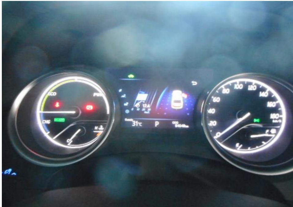
Photo 23 shows no warning lights illuminated on the instrument panel of the Motor Car after the engine was cranked. This would suggest that there was no abnormality to the electronic operating system of the Motor Car, like the ABS, EPS, TCS and SRS etc.
