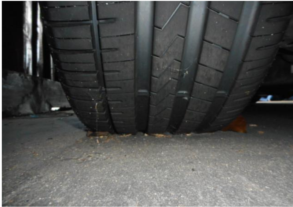
Photo 8 shows the condition of the rear left tyre of the Motor Car, which was observed to be in serviceable condition with remaining tread depth of approximately 7.5mm. The tyre, which was wrapped around alloy wheel rim, was also observed to be sufficiently inflated for vehicular operation. The 4 tyres of the Motor Car were wrapped around standard alloy wheel rims.
