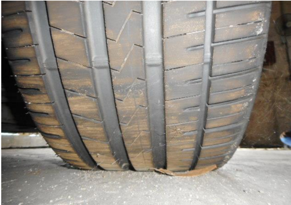
Photo 6 shows the condition of the front right tyre of the Motor Car, which was observed to be in serviceable condition with remaining tread depth of approximately 6.3mm. The tyre was sufficiently inflated for vehicular operation with no tear, cut or burst mark(s) on the outer and the inner sidewalls as well as across the tread. The 4 tyres of the Motor Car were wrapped around standard alloy wheel rims without any damage.
