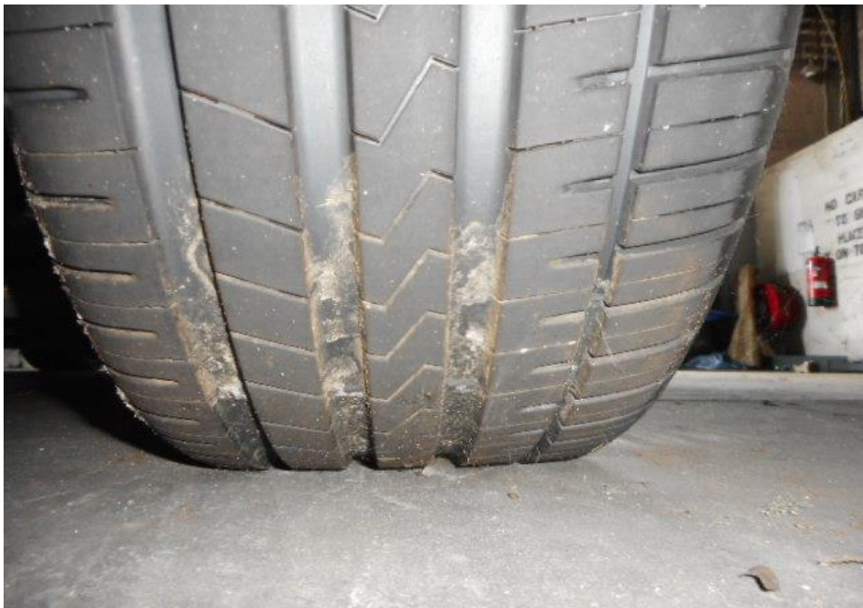
Photo 7 shows the condition of the rear right tyre of the Motor Car, which was observed to be in serviceable condition with remaining tread depth of approximately 6.9mm. The tyre was also observed to be sufficiently inflated for vehicular operation with no tear, cut or burst mark(s).
