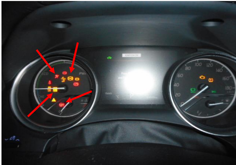
Photo 22 shows the warning light for Anti-Lock Brake System (ABS), Electric Power Steering System (EPS), Traction Control System (TCS) and Supplemental Restraint System (SRS) (arrowed) appearing on the instrument panel of the Motor Car during the self-test of its various electronic operating systems when its engine was cranked.
