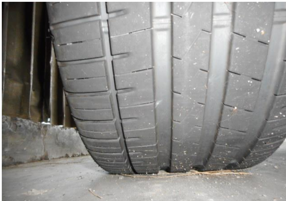
Photo 9 shows the condition of the front left tyre of the Motor Car, which was observed to be in serviceable condition with remaining tread depth of approximately 6.3mm. There was also no tear, cut or burst mark(s) on the outer and the inner sidewalls as well as across the tread of the Motor Car's 4 tyres.
