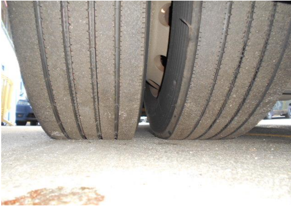
Photo 9 shows the condition of the rear left tyre of the Motor Bus, which was observed to be in serviceable condition with remaining tread depth of approximately 6.8mm. The tyre, which was wrapped around standard steel wheel rim, was also observed to be sufficiently inflated for vehicular operation.
