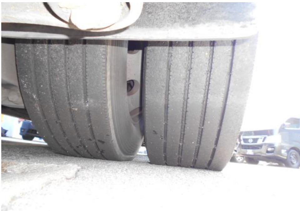
Photo 8 shows the condition of the rear right tyre of the Motor Bus, which was observed to be in serviceable condition with remaining tread depth of approximately 3.6mm. The tyre, which was wrapped around standard steel wheel rim, was also observed to be sufficiently inflated for vehicular operation
