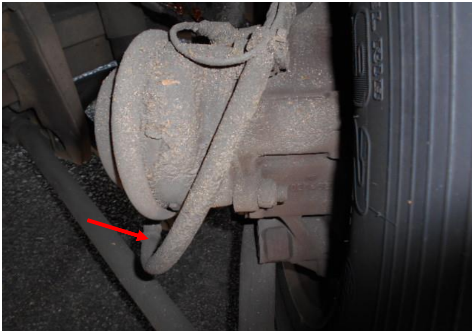
Photo 18 shows the brake pipe (arrowed) at the front left wheel of the Motor Bus. I did not observe any leakage of brake fluid at the time of my inspection of the Motor Bus. My visual examination of the various mechanical components of the braking system were generally intact and unaffected by the accident.
