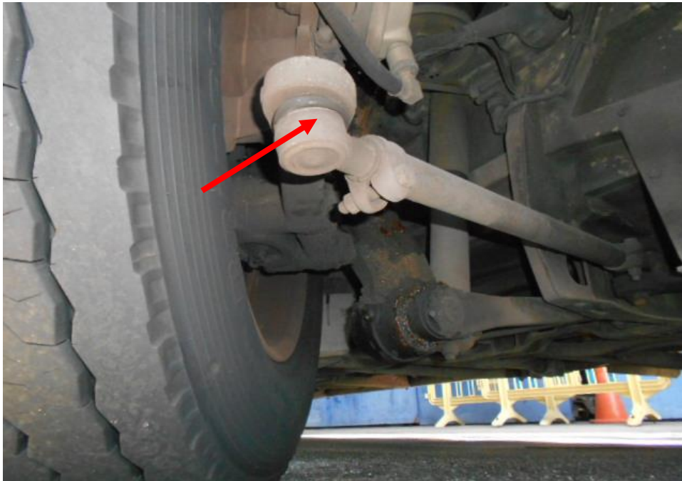
Photo 21 shows the various undercarriage components at the front left wheel of the Motor Car, in particular the steering tie rod end (arrowed). The various steering components were all found to be intact. There was also no sign of fluid stain(s) observed on the various undercarriage components.
