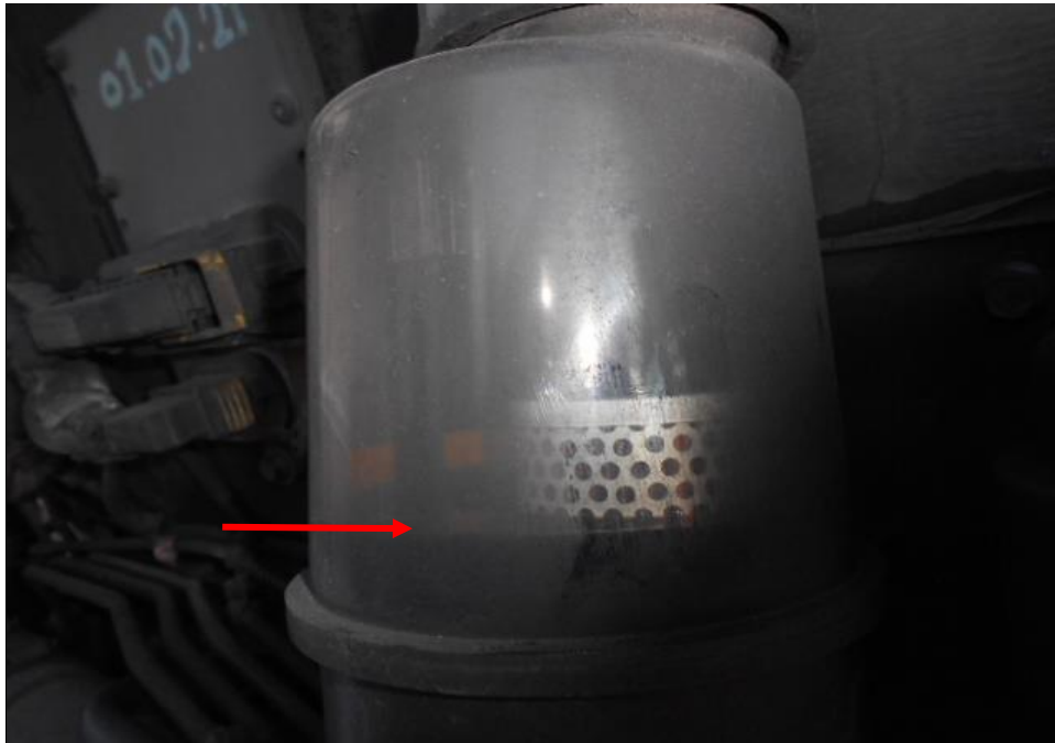
Photo 14 shows the power steering reservoir of the Motor Bus at the time of my inspection. The power steering was observed to be of sufficient level (arrowed) and without any visible contamination.
