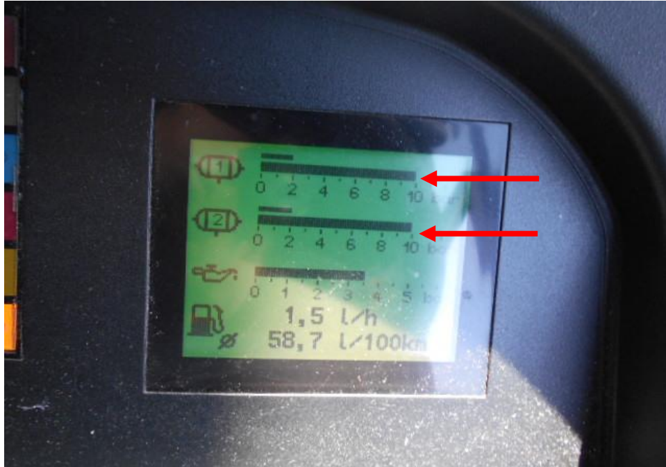
Photo 12 shows the air in the air brake cylinder of the Motor Bus at the time of my inspection. The air in the cylinder was observed to be of sufficient level & serviceable at the time of my inspection.
