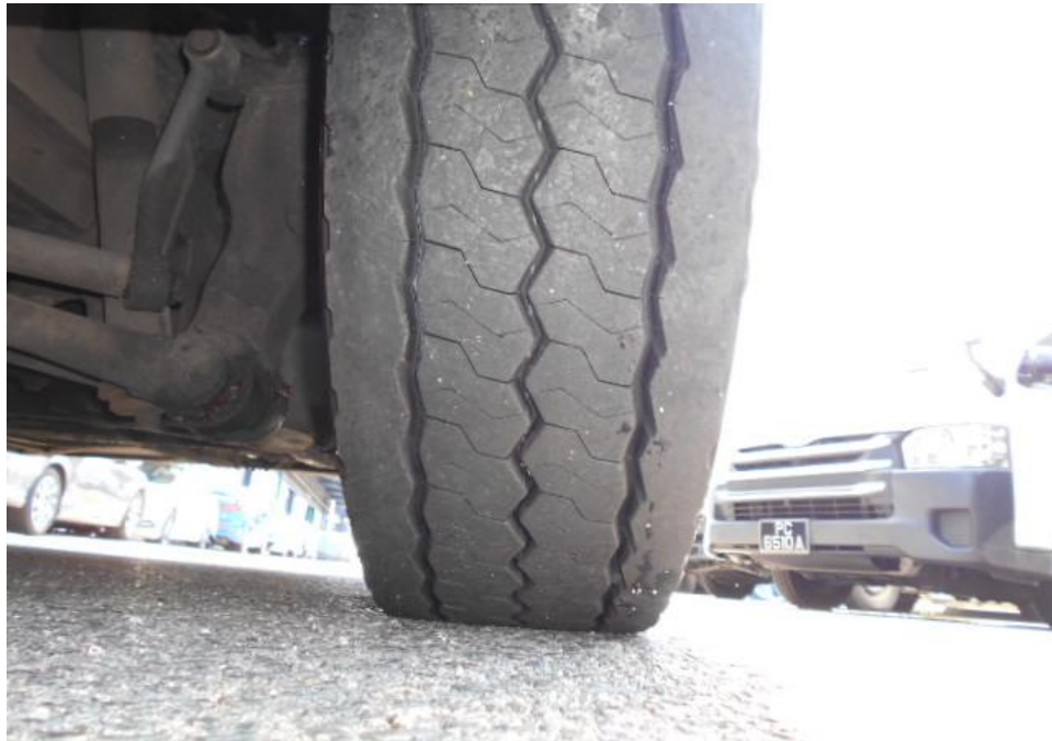
Photo 7 shows the condition of the front right tyre of the Motor Bus, which was observed to be in serviceable condition with remaining tread depth of approximately 16.4mm. The tyre, which was wrapped around standard steel wheel rim, was also observed to be sufficiently inflated for vehicular operation. There was no tear, cut or burst mark(s) on the outer and the inner sidewalls as well as across the tread of the 6 tyres that were fitted on the Motor Bus.
