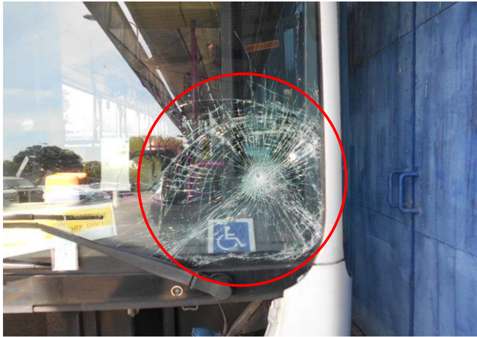
Photo 3 shows a close up view of the front body of the Motor Bus at the time of my inspection. The Motor Bus was observed to have sustained damages at its front portion. Its front windscreen (circled) was damaged as a result of the accident.
