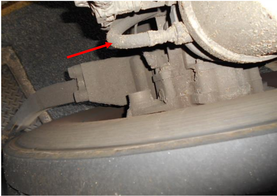
Photo 17 shows the brake pipe (arrowed) at the rear left wheel of the Motor Bus. I did not observe any leakage of brake fluid at the time of my inspection of the Motor Bus. My visual examination of the various mechanical components of the braking system were generally intact and unaffected by the accident.
