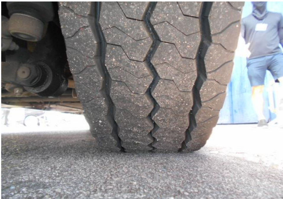
Photo 10 shows the condition of the front left tyre of the Motor Bus, which was observed to be in serviceable condition with remaining tread depth of approximately 12.7mm. The tyre, which was wrapped around standard steel wheel rim, was also observed to be sufficiently inflated for vehicular operation.
