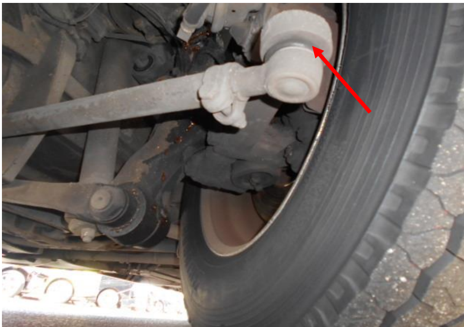
Photo 20 shows the various undercarriage components at the front right wheel of the Motor Car, in particular the steering tie rod end (arrowed). The various steering components were all found to be intact. There was also no sign of fluid stain(s) observed on the various undercarriage components.
