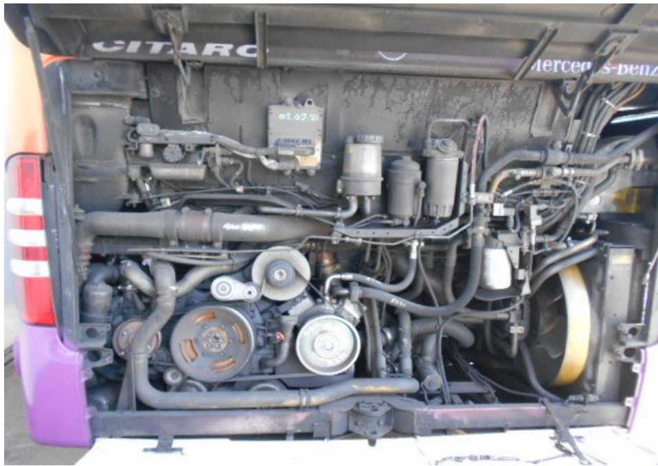
Photo 11 shows a general view of the Motor Bus's engine compartment, which was accessed by lifting the rear of the Motor Bus. The various parts and components inside the engine compartment were unaffected by the accident. There was also no sign(s) or indication(s) of fresh fluid leakage and/or fluid stain within the engine compartment.
