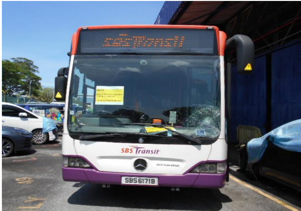
Photo 2 shows a general view of the front body of the Motor Bus at the time of my inspection. The Motor Bus was observed to have sustained damages at its front windscreen was observed to be damage at the time of my inspection.
