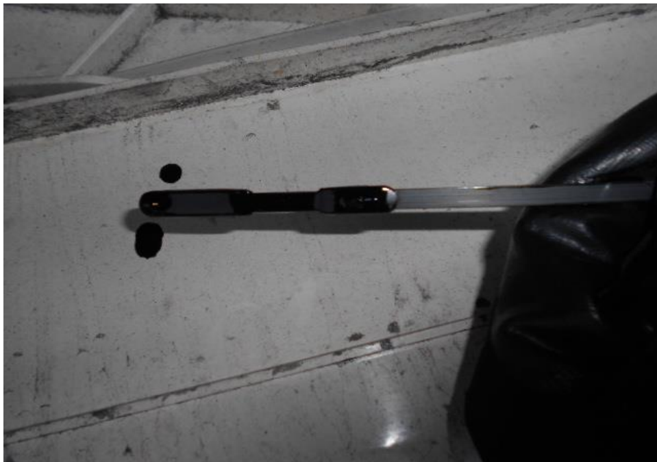
Photo 15 shows the engine oil dip stick of the Motor Bus at the time of my inspection. The engine oil was observed to be sufficient for operation and without any visible contamination.
