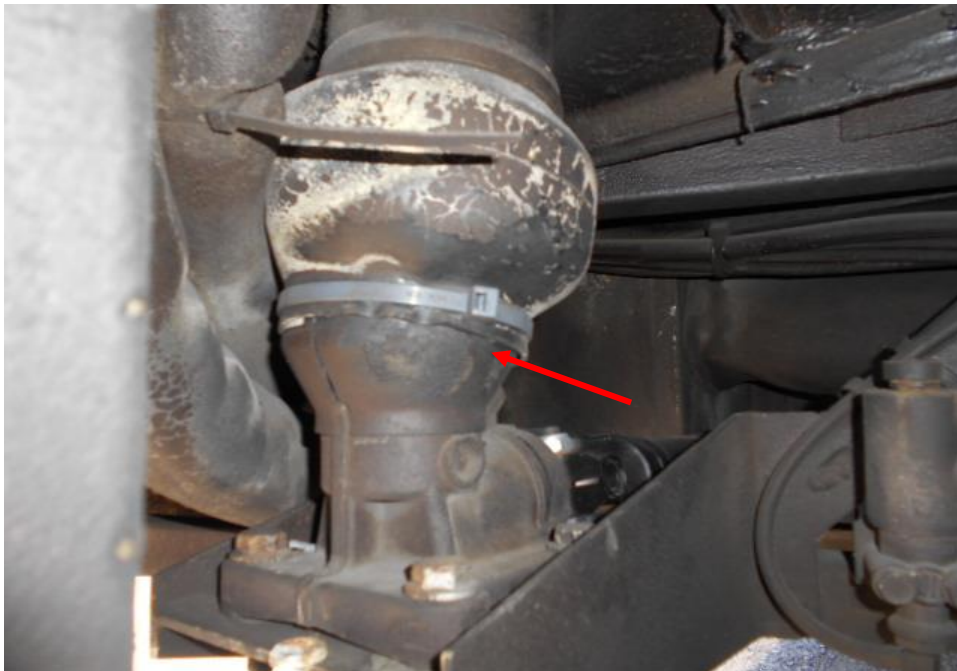
Photo 22 shows the steering box component (arrowed) at the undercarriage of the Motor Bus was found to be intact and without any visible damage. There was also no signs of fluid stain(s) observed on the various undercarriage components.
