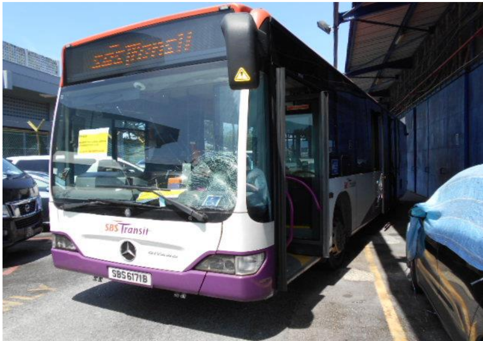
Photo 5 shows the general view of the left body of the Motor Bus at the time of my inspection. The Motor bus was observed to be intact and unaffected by the accident.
