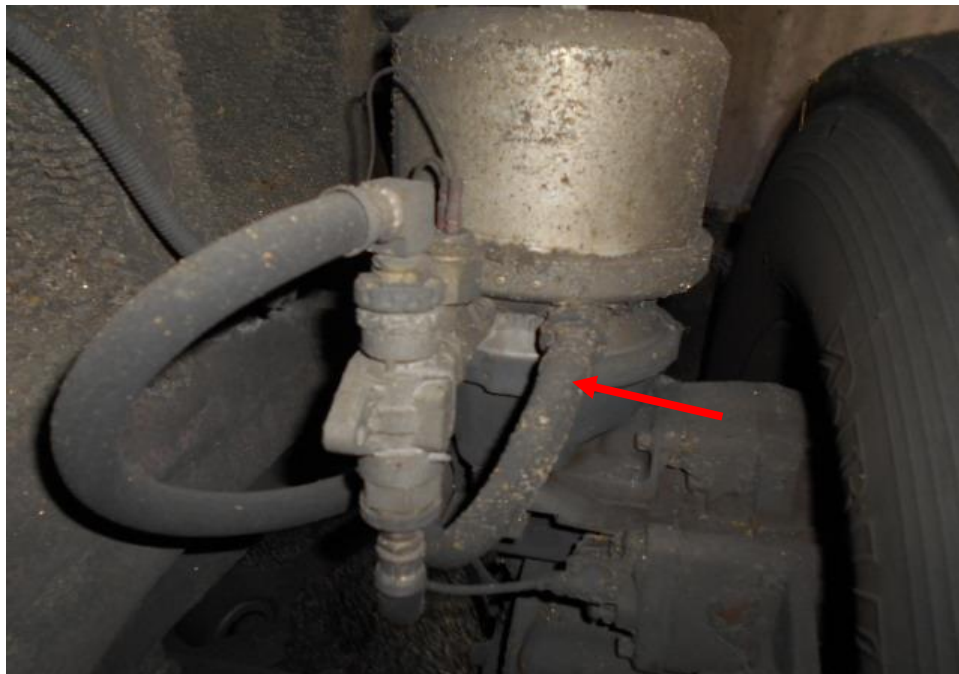
Photo 16 shows the brake pipe (arrowed) at the rear right wheel of the Motor Bus. I did not observe any leakage of brake fluid at the time of my inspection of the Motor Bus. My visual examination of the various mechanical components of the braking system were generally intact and unaffected by the accident.
