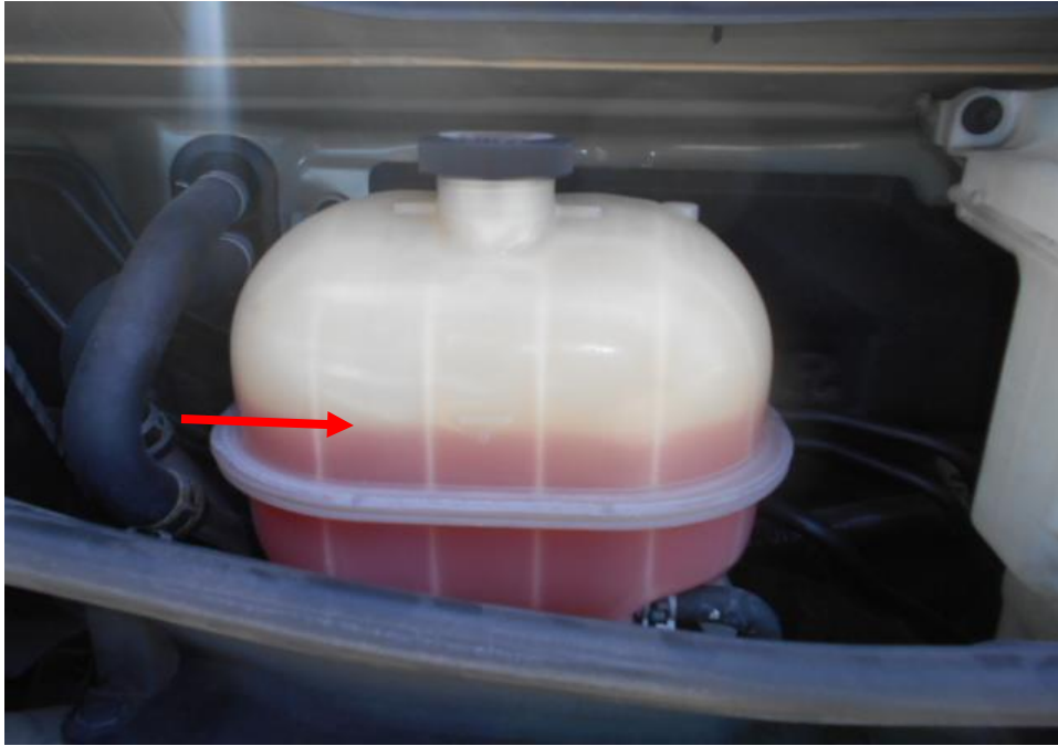
Photo 13 shows the engine coolant of the Motor Van at the time of my inspection. The engine coolant was observed to be of sufficient level (arrowed) and without any visible contamination
