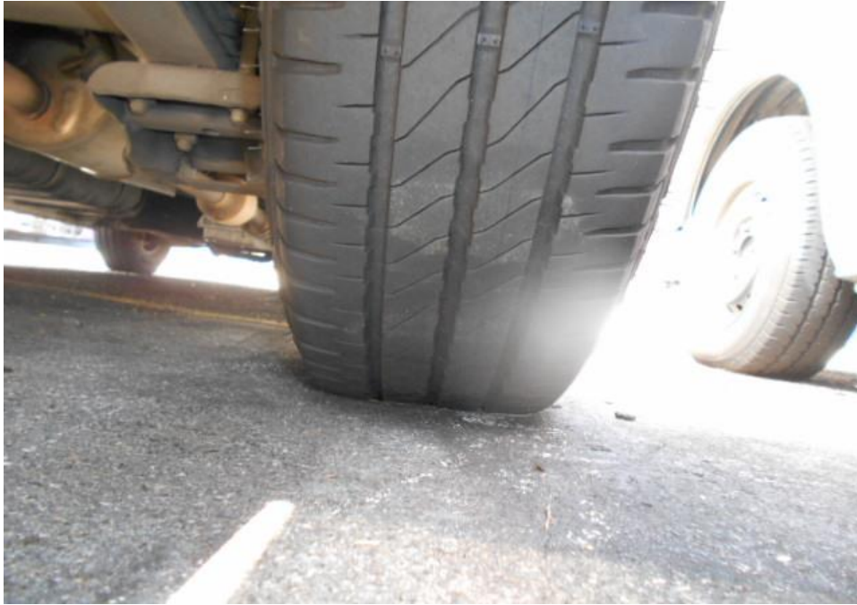
Photo 8 shows the condition of the rear right tyre of the Motor Van, which was observed to be in serviceable condition with remaining tread depth of approximately 4.5mm. The tyre, which was wrapped around standard steel wheel rim, it was observed to be sufficiently inflated for vehicular operation.
