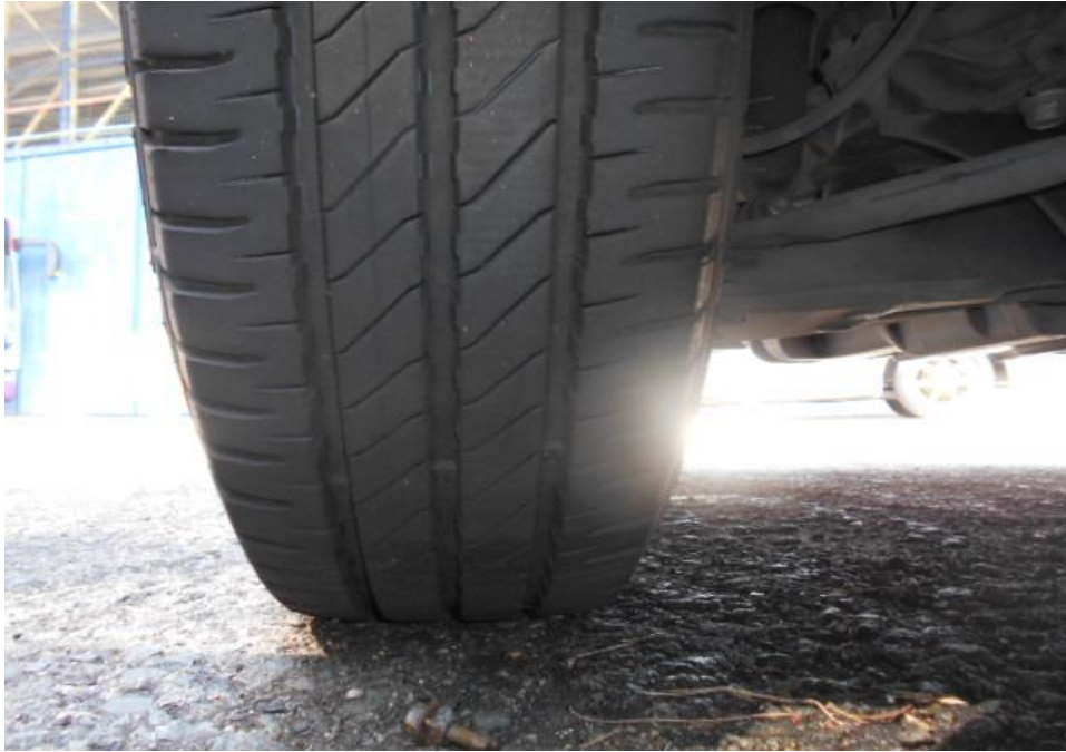
Photo 10 shows the condition of the front left tyres of the Motor Van, which were observed to be in serviceable condition with remaining, tread depth of approximately 7.4mm. There was also no tear, cut or burst mark(s) on the outer and the inner sidewalls as well as across the tread of the 4 tyres that were fitted on the Motor Van.
