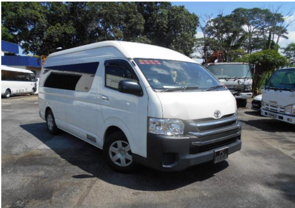
Photo 23 shows the front right wheel of the Motor Van turned to its full left. During my steering system test, I did not experience any abnormal free play and/or resistance when I had turned the steering wheel towards full left and full right. This would suggest that the steering system of the Motor Van was likely to be in serviceable condition at the material time of accident.
