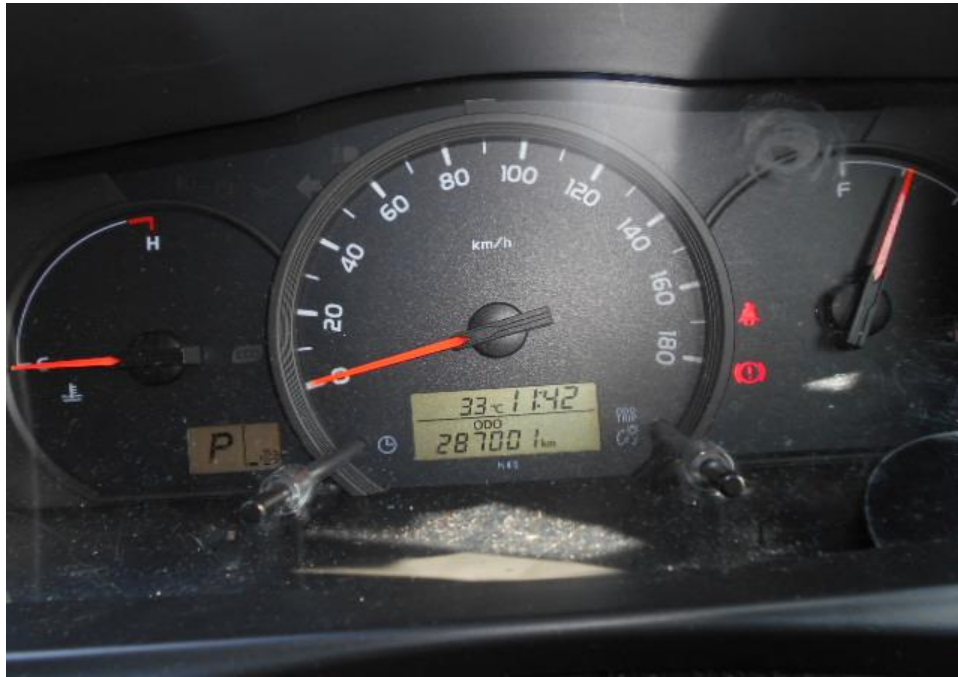
Photo 25 shows no warning lights illuminated on the instrument panel of the Motor Van after the engine was cranked. This would suggest that there was no abnormality to the electronic operating system of the Motor Van, like the ABS, TCS, SRS and etc.
