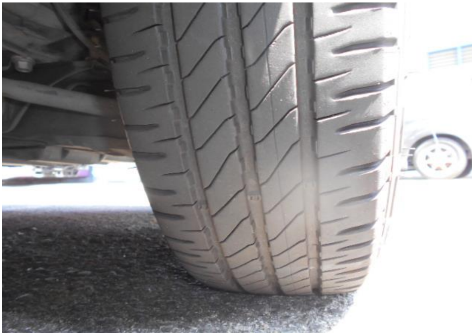
Photo 7 shows the condition of the front right tyre of the Motor Van, which was observed to be in serviceable condition with remaining tread depth of approximately 6.9mm. The tyre, which was wrapped around standard steel wheel rim, was also observed to be sufficiently inflated for vehicular operation. There was no tear, cut or burst mark(s) on the outer and the inner sidewalls as well as across the tread of the 4 tyres that were fitted on the Motor Van.
