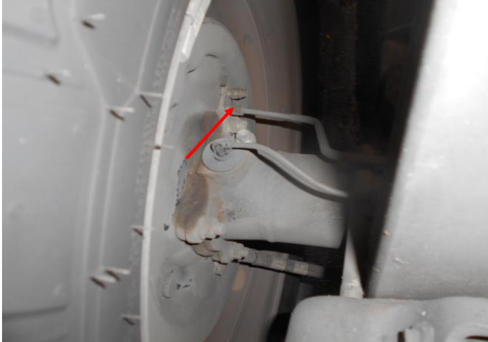
Photo 20 shows the brake pipe (arrowed) at the rear left wheel of the Motor Van. I did not observe any leakage of brake fluid at the time of my inspection of the Motor Van. My static tests of the Motor Van's braking system, along with my visual examination of the various mechanical components in the braking system had indicated that there was no internal leakage of pressure/vacuum. Hence the braking system of the Motor Van was likely to be in serviceable condition at the material time of accident.
