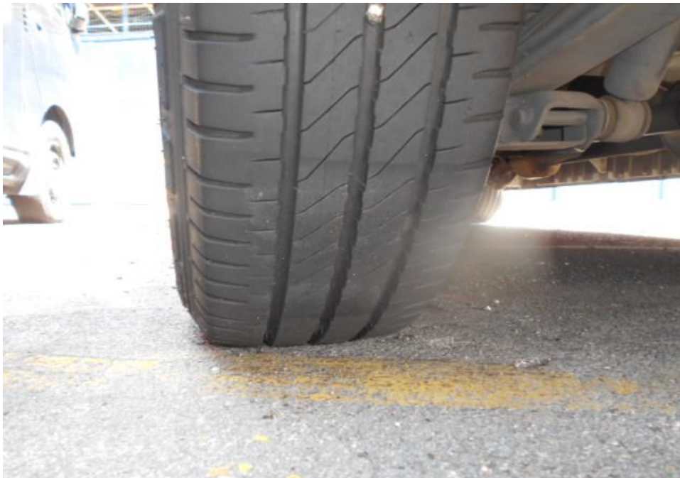
Photo 9 shows the condition of the rear left tyres of the Motor Van, which was observed to be in serviceable condition with remaining tread depth of approximately 4.18mm. The tyres, which were wrapped around standard steel wheel rim, were also observed to be sufficiently inflated for vehicular operation. There was also no damage found on all 4 steel wheel rims of the Motor Van.
