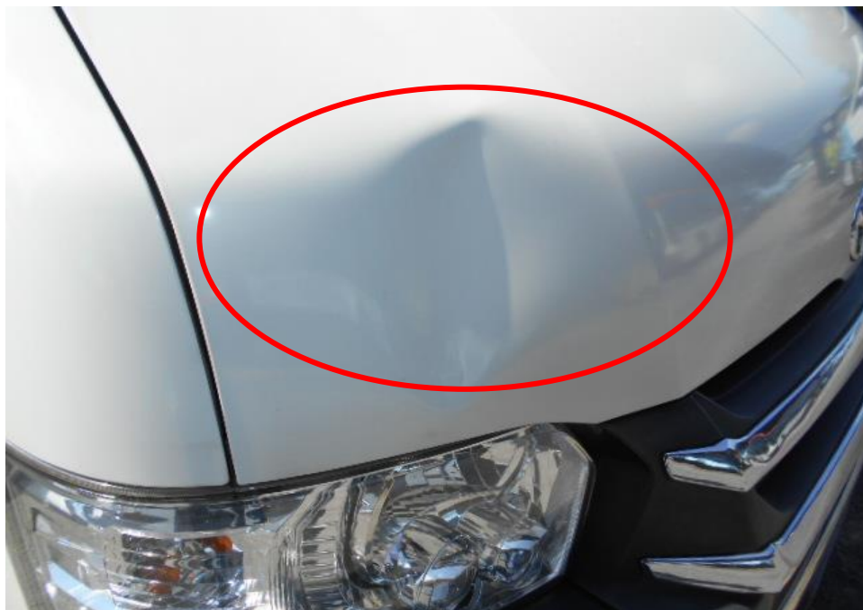
Photo 3 shows a close up view of the Motor Van's frontal portion at the time of my inspection. It appeared to have sustained damage at its frontal. Its front body panel (circled) was damage at the time of my inspection as a result of the accident.
