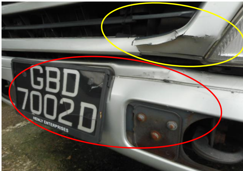
Photo 5 shows a close up view of the Motor Lorry's frontal portion at the time of my inspection. It appeared to have sustained damage at its frontal portion. Its front grille (yellow circle), front bumper and front number plate (red circle) was damage at the time of my inspection as a result of the accident.
