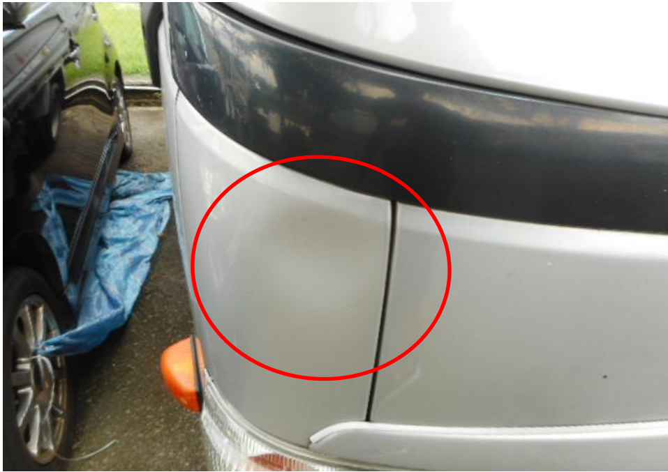
Photo 4 shows a close up view of the Motor Lorry's frontal portion at the time of my inspection. It appeared to have sustained damage at its frontal portion. Its front body panel (circled) was damage at the time of my inspection as a result of the accident.
