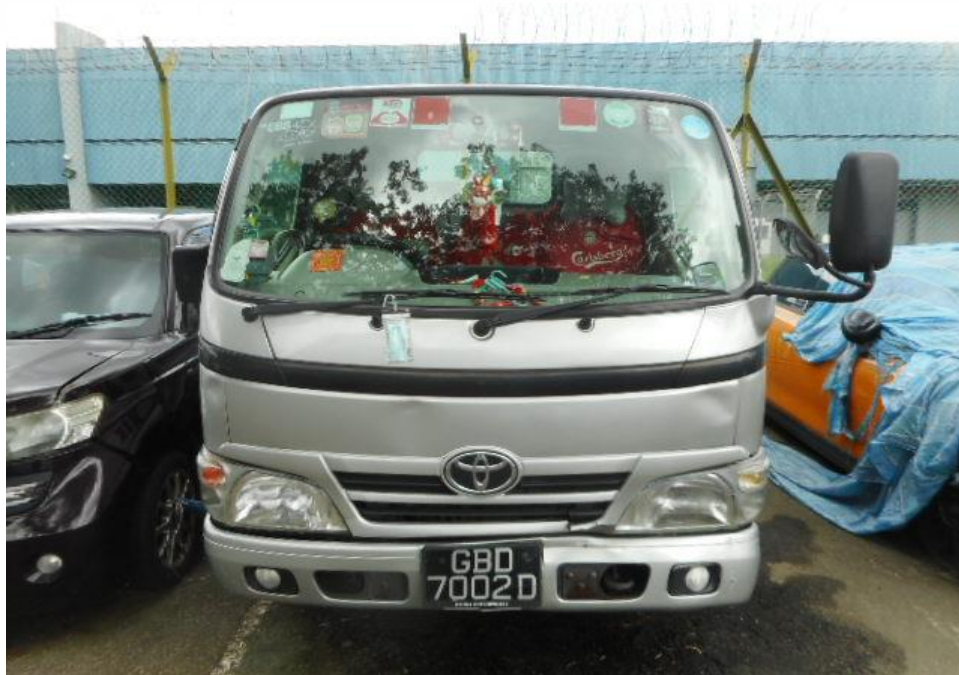
Photo 2 shows a general view of the Motor Lorry's frontal portion at the time of my inspection. It appeared to have sustained damage at its frontal portion. Its front body panel, front grille, front number plate and front bumper was damaged at the time of my inspection as a result of the accident.
