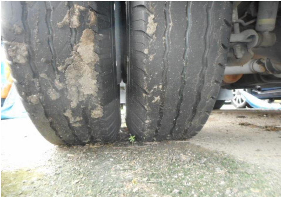
Photo 11 shows the condition of the rear left tyres of the Motor Lorry, which was observed to be in serviceable condition with remaining tread depth of approximately 1.7mm. The tyres, which were wrapped around standard steel wheel rim, were also observed to be sufficiently inflated for vehicular operation. There was also no damage found on all 6 steel wheel rims of the Motor Lorry.
