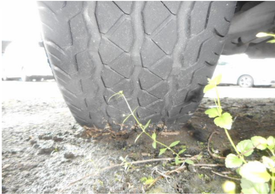
Photo 12 shows the condition of the rear right tyres of the Motor Lorry, which were observed to be in serviceable condition with remaining, tread depth of approximately 5.3mm. There was also no tear, cut or burst mark(s) on the outer and the inner sidewalls as well as across the tread of the 6 tyres that were fitted on the Motor Lorry.
