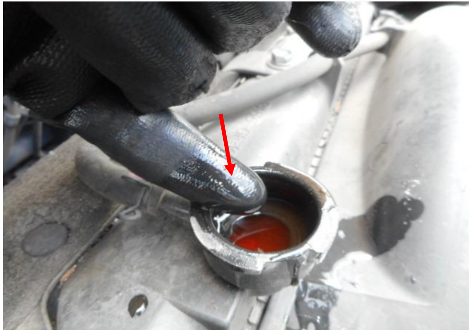
Photo 15 shows the engine coolant of the Motor Lorry at the time of my inspection. The engine coolant was observed to be of sufficient level (arrowed) and without any visible contamination.
