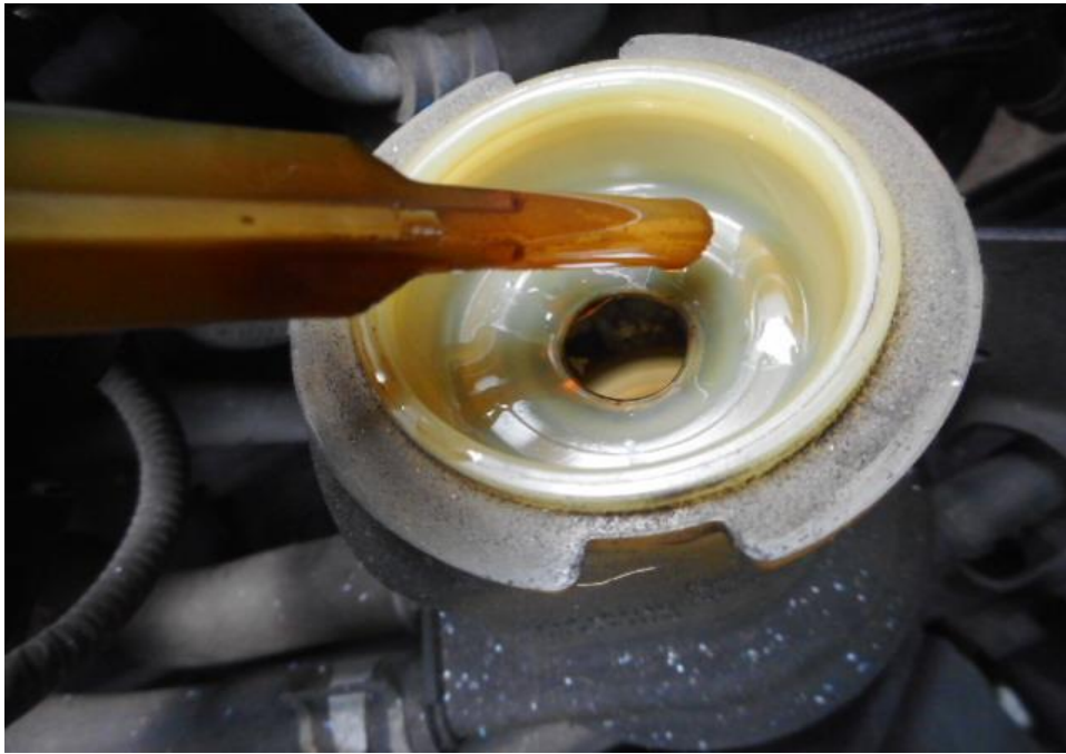
Photo 17 shows the power steering fluid dip stick of the Motor Lorry at the time of my inspection. The power steering fluid was observed to be of sufficient level and without any visible contamination.
