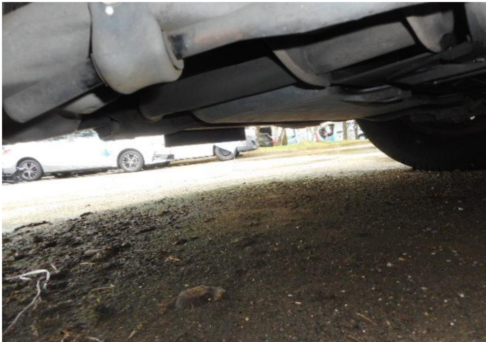
Photo 18 shows the undercarriage of the Motor Lorry, at the area where the engine housing and transmission housing are located at. We did not observe any leak and/or fluid stain(s) on the underside of the Motor Lorry.
