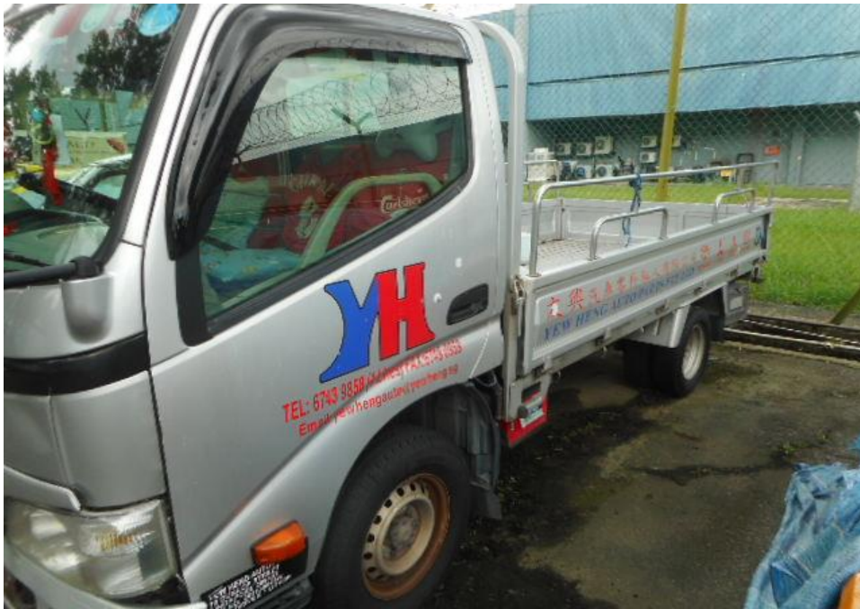
Photo 7 shows a general view of the left body of the Motor Lorry at the time of my inspection. The Motor Lorry was observed to be intact and unaffected by the accident.
