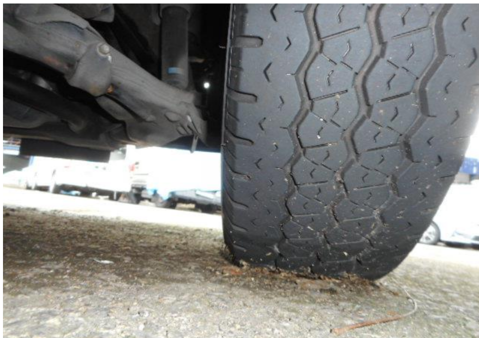
Photo 9 shows the condition of the front right tyre of the Motor Lorry, which was observed to be in serviceable condition with remaining tread depth of approximately 5.6mm. The tyre, which was wrapped around standard steel wheel rim, was also observed to be sufficiently inflated for vehicular operation. There was no tear, cut or burst mark(s) on the outer and the inner sidewalls as well as across the tread of the 6 tyres that were fitted on the Motor Lorry.
