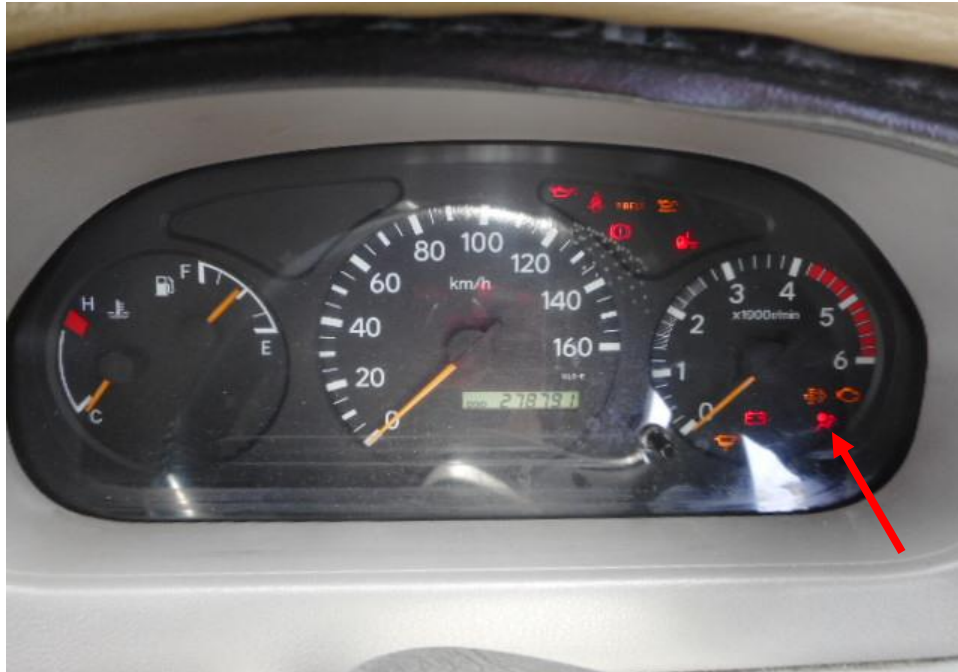
Photo 26 shows the warning light for Supplemental Restraint System (SRS) (arrowed) appearing on the instrument panel of the Motor Van during the self-test of its various electronic operating systems when its engine was cranked.
