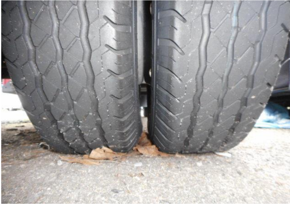
Photo 10 shows the condition of the rear right tyre of the Motor Lorry, which was observed to be in serviceable condition with remaining tread depth of approximately 3.3mm. The tyre, which was wrapped around standard steel wheel rim, it was observed to be sufficiently inflated for vehicular operation.
