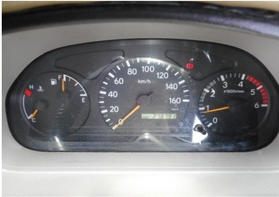
Photo 27 shows no warning lights illuminated on the instrument panel of the Motor Van after the engine was cranked. This would suggest that there was no abnormality to the electronic operating system of the Motor Van, like the SRS and etc.
