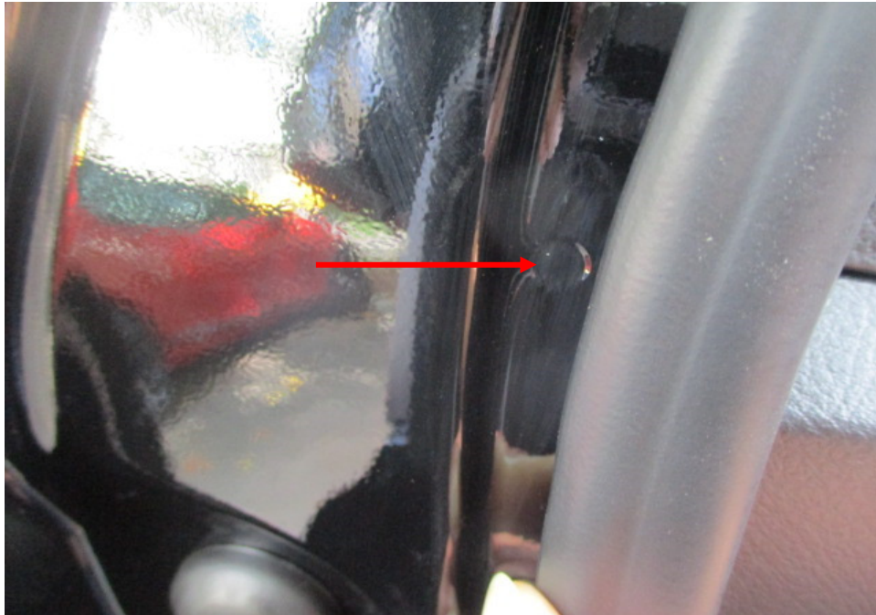
Photo 36 shows the left side "A" pillar of the Motor Car. I did not find any weld marks other than original spot weld marks (arrowed) on the left side "A" pillar of the Motor Car, which indicates that there was no re-welding works carried out. In general, I had found all the non-detachable body panels of the Motor Car to be originally fitted at the time of my inspection.
