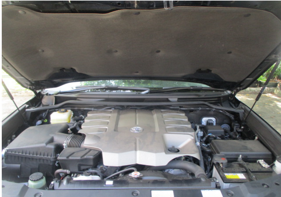
Photo 18 shows a general view of the Motor Car's engine compartment at the time of my inspection. The various parts and components inside the engine compartment were all observed to be intact and properly fitted. There was also no sign(s) or indication(s) of fluid leak and/or fluid stain found inside the engine compartment.
