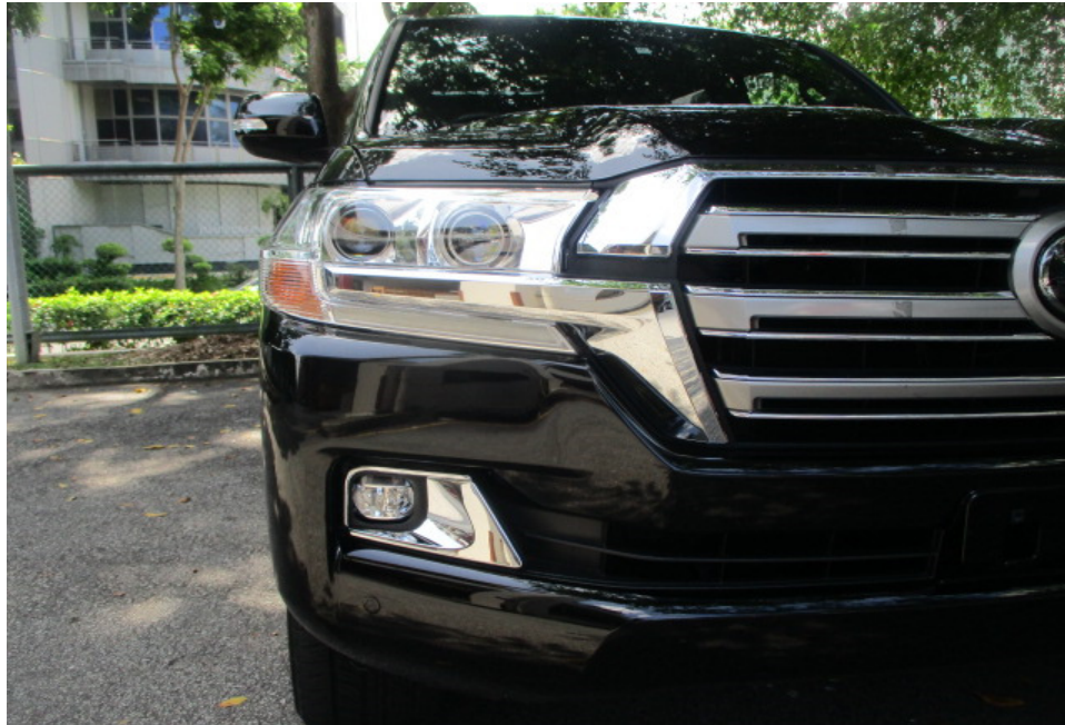
Photo 8 shows a closer view of the Motor Car's front bumper, front bumper right fog lamp cover, front bumper right fog lamp and front right headlamp. The body parts at the frontal portion of the Motor Car were visually examined and it was observed that the repair/restoration works carried out to the damaged area of the Motor Car (refer to photograph 1 - 3 above) were reasonably adequate and in order.
