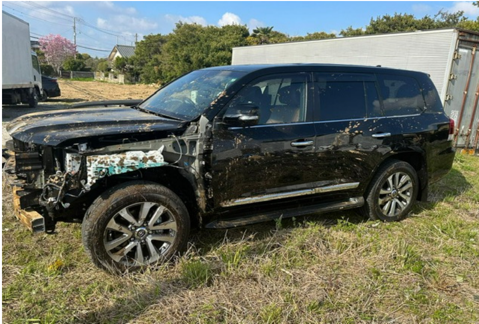
Photo 1 shows the front left body of the Motor Car (photograph provided to me). The photographs provided to me had showed the Motor Car's front left fender, front left blind spot mirror, front left headlamp, front bumper and all its related parts and attachments like the front bumper centre lower grille, front bumper sensors, front bumper left fog lamp cover and front bumper left fog lamp amongst others, missing/dislodged/damaged.
