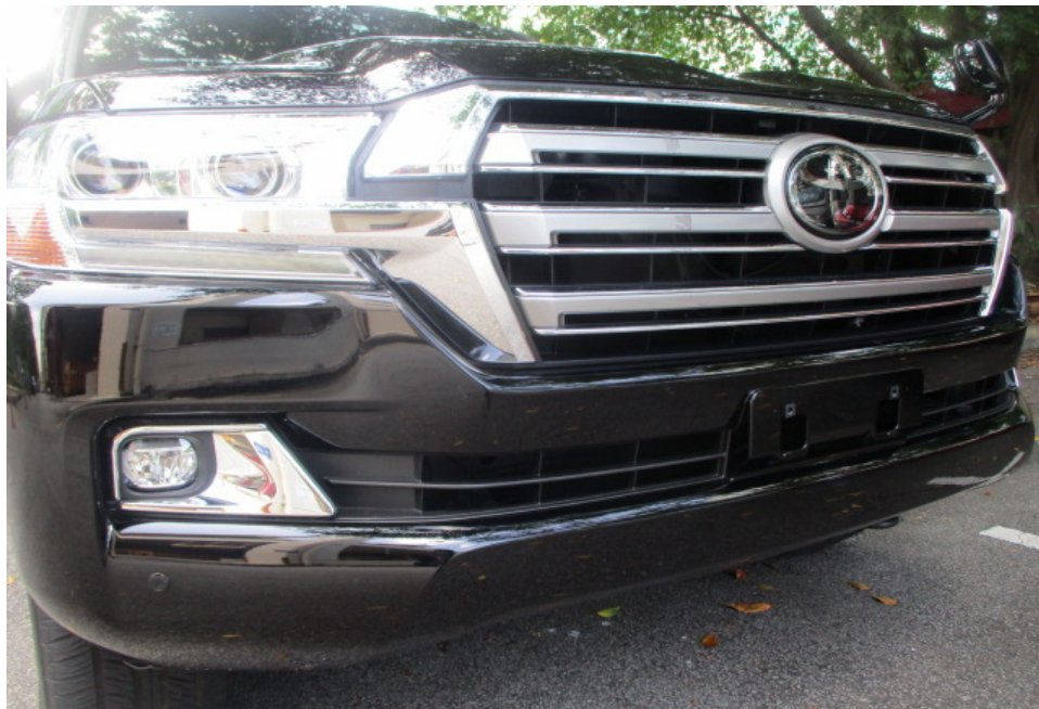
Photo 9 shows a closer view of the Motor Car's front bumper, front bumper left sensor, front bumper centre lower grille, front bumper right fog lamp cover, front bumper right fog lamp, front lower grille and front upper grille. The body parts at the frontal portion of the Motor Car were visually examined and it was observed that the repair/restoration works carried out to the damaged area of the Motor Car (refer to photograph 1 - 3 above) were reasonably adequate and in order.
