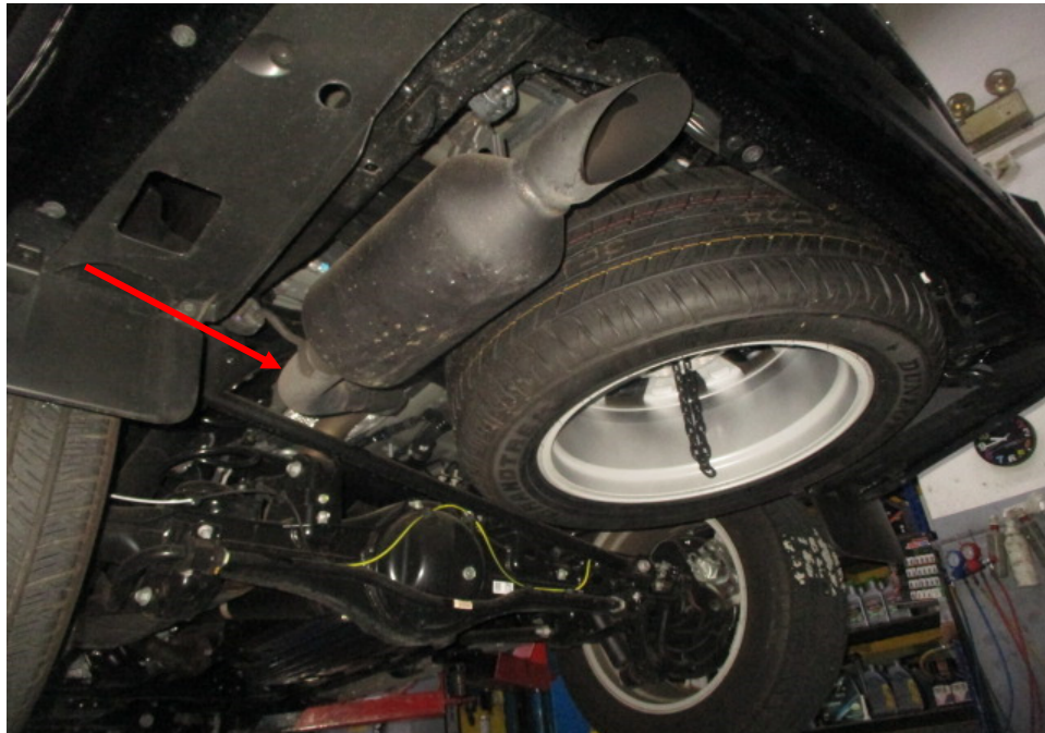
Photo 29 shows the rear section of the Motor Car's exhaust system. My examination of the Motor Car's exhaust system revealed no sign(s) or indication(s) of any cut or weld marks along its exhaust pipes (arrowed), on its rear muffler, on its centre resonator box and on its catalytic converters.
