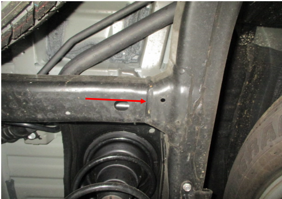
Photo 31 shows the chassis/structural body at the underside rear right of the Motor Car. I did not find any weld marks other than original spot weld marks on the chassis/structural body of the Motor Car. The original factory sealant (arrowed) at the joints along the chassis/structural body was untouched, indicating no work was done on the chassis/structural body of the Motor Car and that the chassis/structural body was originally fitted.
