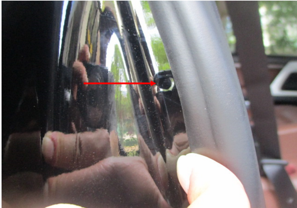
Photo 38 shows the right side "C" pillar of the Motor Car. I did not find any weld marks other than original spot weld marks (arrowed) on the right side "C" pillar of the Motor Car, which indicates that there was no re-welding works carried out. In general, I had found all the non-detachable body panels of the Motor Car to be originally fitted at the time of my inspection.
