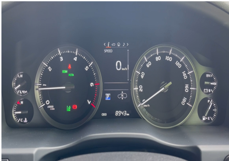
Photo 23 shows the respective warning lights no longer illuminated, indicating that there is no fault detected to the ABS, SRS, EPS and TCS systems of the Motor Car during the self-test. These electronic systems were hence in working condition at the time of my inspection.
