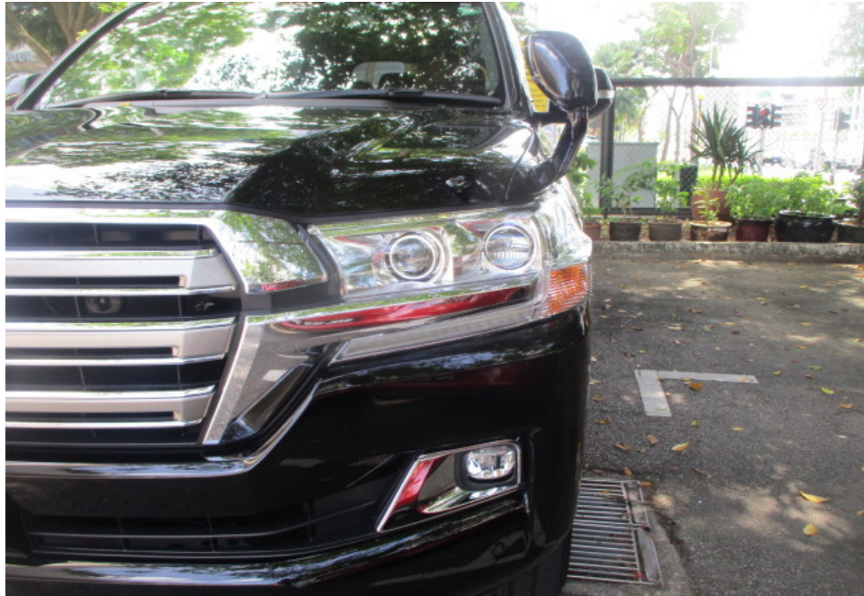
Photo 12 shows a closer view of the Motor Car's front bumper, front bumper left fog lamp cover, front bumper left fog lamp, front left headlamp and front left blind spot mirror. The body parts at the frontal portion of the Motor Car were visually examined and it was observed that the repair/restoration works carried out to the damaged area of the Motor Car (refer to photograph 1 - 3 above) were reasonably adequate and in order.
