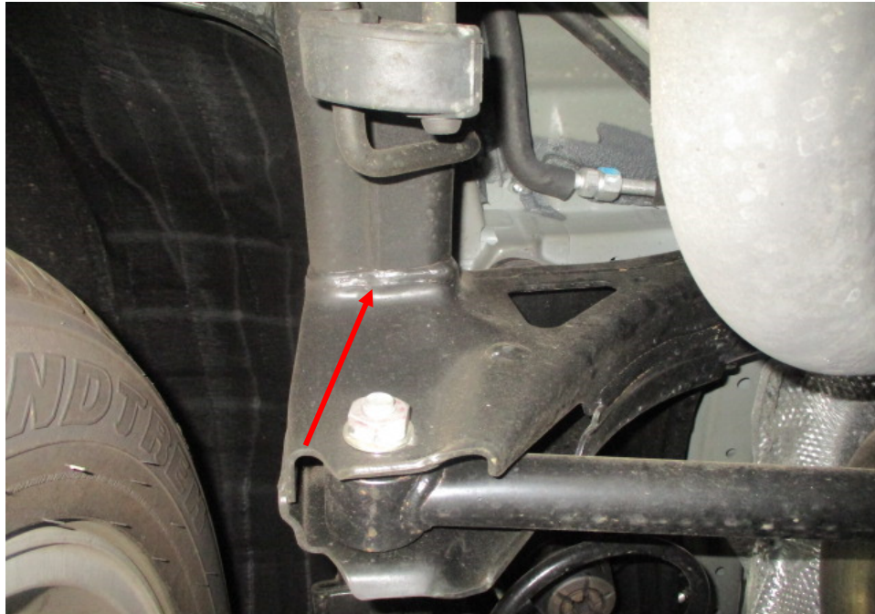
Photo 32 shows the chassis/structural body at the underside rear left of the Motor Car. I did not find any weld marks other than original spot weld marks on the chassis/structural body of the Motor Car. The original factory sealant (arrowed) at the joints along the chassis/structural body was untouched, indicating no work was done on the chassis/structural body of the Motor Car and that the chassis/structural body was originally fitted.
