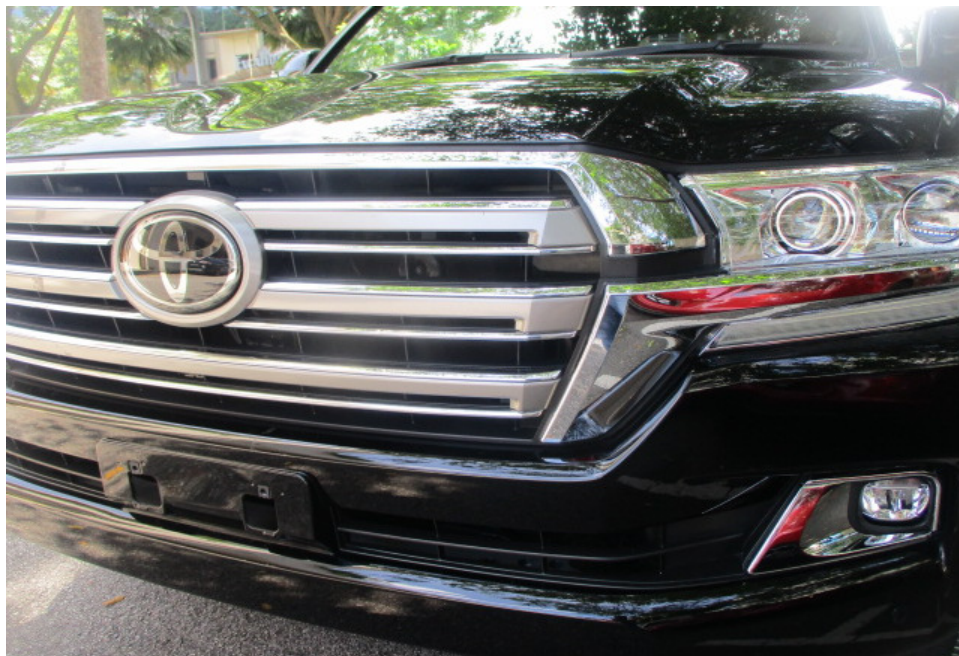
Photo 13 shows a closer view of the Motor Car's front bumper, front bumper centre lower grille, front bumper left fog lamp cover, front bumper left fog lamp, front lower grille, front upper grille and front emblem. The body parts at the frontal portion of the Motor Car were visually examined and it was observed that the repair/restoration works carried out to the damaged area of the Motor Car (refer to photograph 1 - 3 above) were reasonably adequate and in order.
