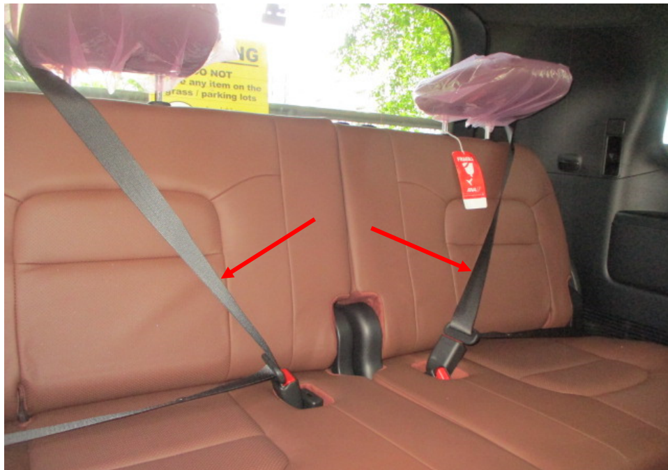
Photo 21 shows the rear seats at the 2 nd row of the Motor Car. All the seats of the Motor Car were secured via seat rails to the floorboard. They were also fitted with a retractable seat belt reel and a pre-tensioner. The seat belts (arrowed) were tested and were able to be fastened into the respective pre-tensions that were fitted on the side of each individual seat.
