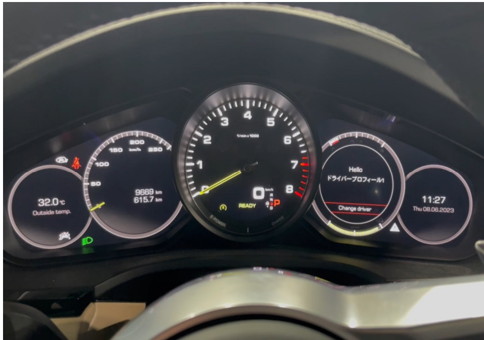
Photo 19 shows the respective warning lights no longer illuminated, indicating that there is no fault detected to the ABS, SRS, EPS, TPM and TCS systems of the Motor Car during the self-test. These electronic systems were hence in working condition at the time of my inspection.
