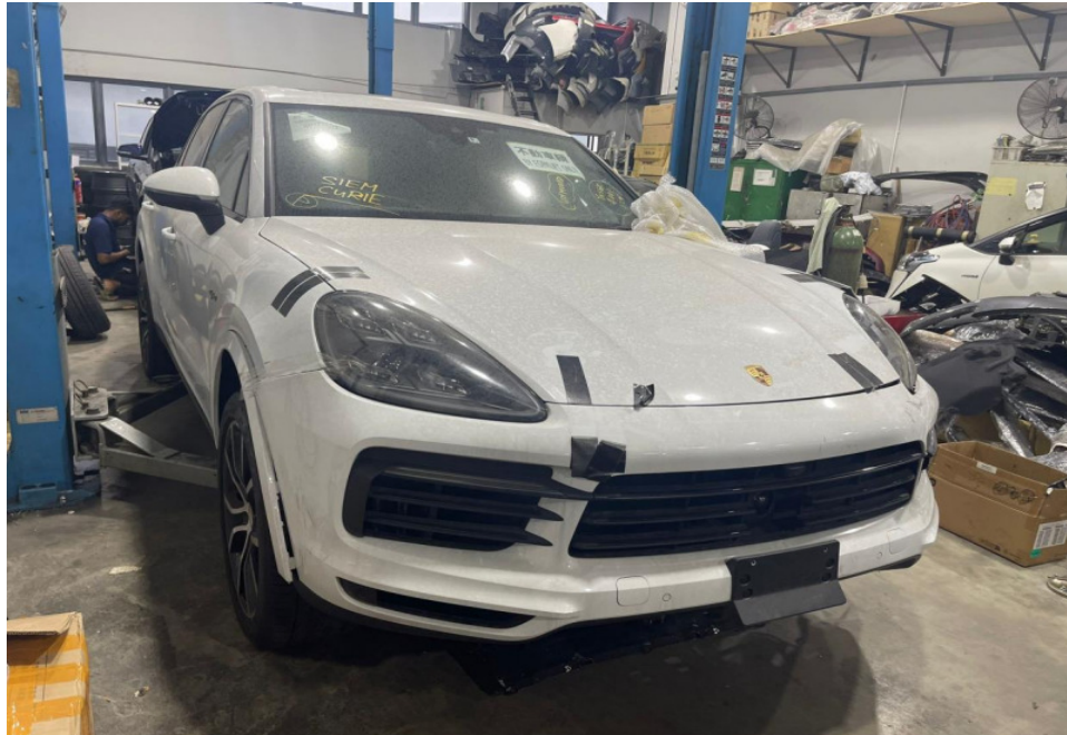
Photo 5 shows the front right body of the Motor Car (photograph provided to me). Apart for the left front portion, there was no physical damage observed to other areas of the Motor Car. The airbag(s) of the Motor Car was not deployed.
