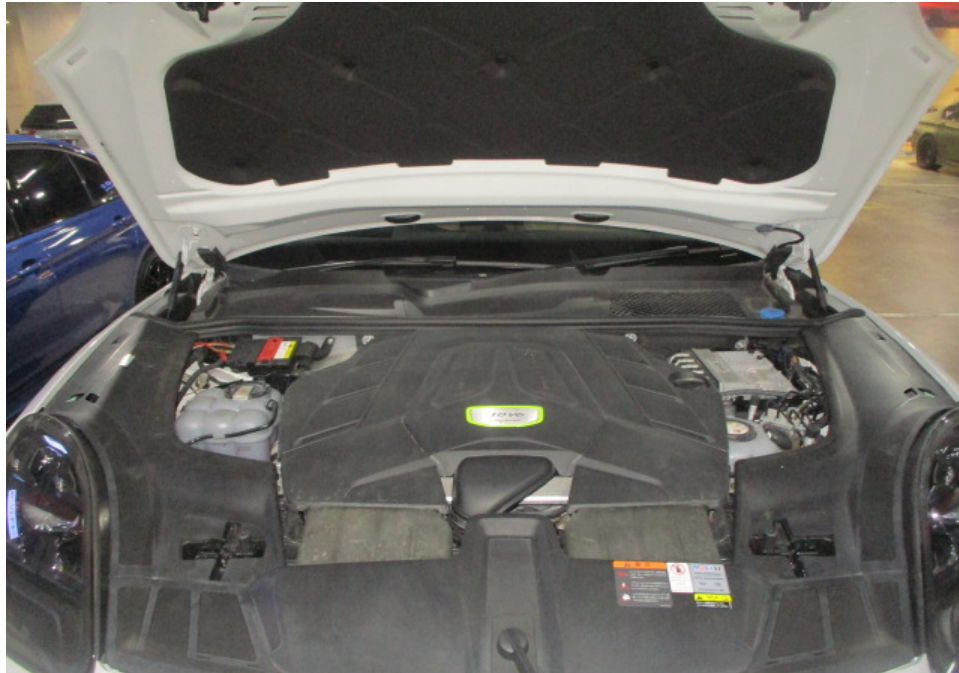
Photo 14 shows a general view of the engine compartment of the Motor Car at the time of my inspection. The various parts and components inside the engine compartment were all observed to be intact and properly fitted. There was also no sign(s) or indication(s) of fluid leak and/or fluid stain found inside the engine compartment.
