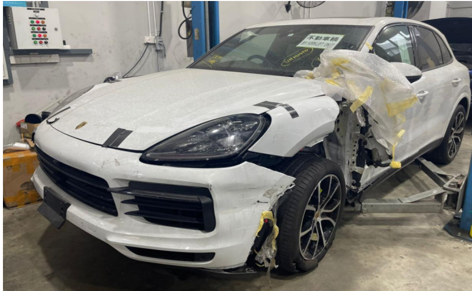
Photo 1 shows the front left body of the Motor Car (photograph provided to me). The photographs provided to me had showed damage to the left front portion of the Motor Car. The front bumper, front bumper lower cover, front bumper left bracket, front left fender, front left fender wheel arc garnish, front left fender inner shield, front left wheel rim, front left tyre, front left "A" pillar, front left door, front left door hinges and left side rocker panel garnish were amongst the body parts that were observed to have been damaged. The airbag(s) of the Motor Car was not deployed.
