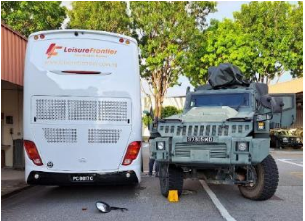
FIGURE B-1: Right side mirror and signal lights damaged
