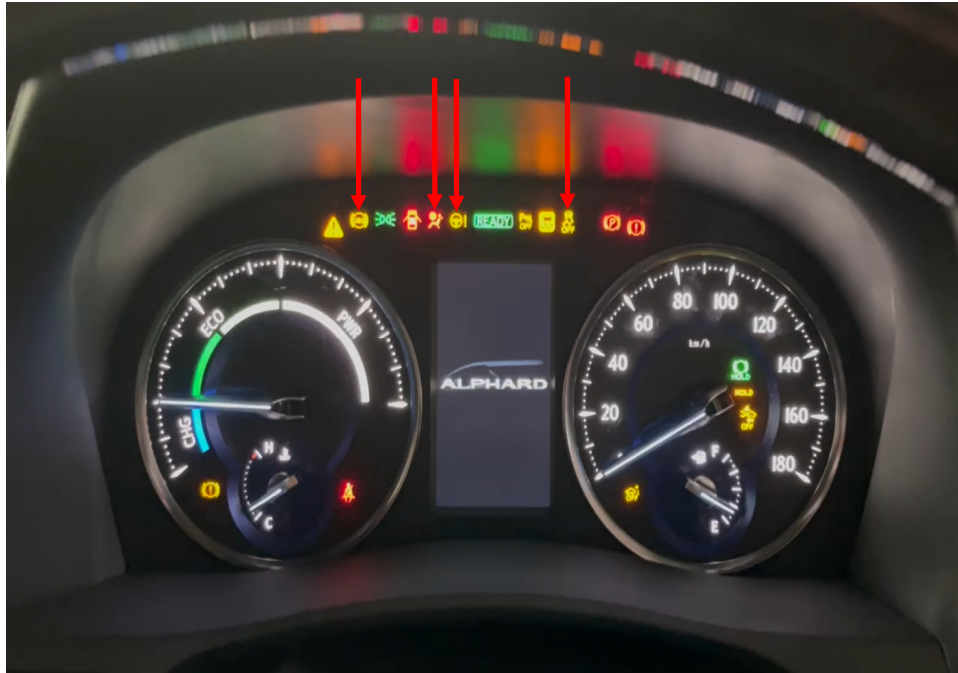
Photo 18 shows the warning lights for the various electronic safety features appearing on the instrument panel of the Motor Car during its self-test when the engine is cranked, in particular the lights for the ABS, SRS, EPS, VSC (arrowed) and the various collision prevention systems.
