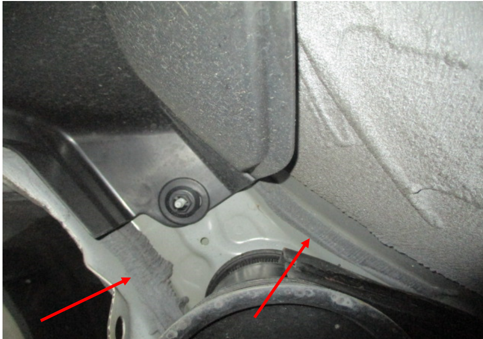
Photo 28 shows the chassis/structural body at the underside rear left of the Motor Car. The original factory sealant (arrowed) at the joints along the chassis/structural body was observed to be untouched. In general, I had found no work was carried out on the chassis/structural body of the Motor Car. The chassis/structural body of the Motor Car was originally fitted
