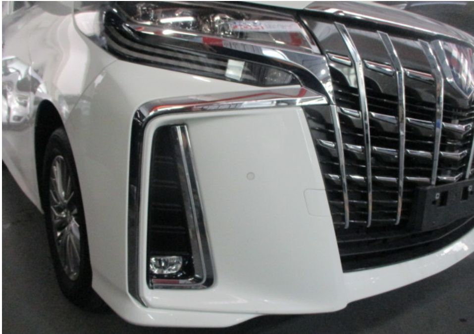
Photo 8 shows a closer view of the Motor Car's front bumper, front bumper right chrome moulding, front right fog lamp, front right headlamp and front right headlamp chrome moulding. The body parts at the front right portion of the Motor Car were visually examined and it was observed that the repair/restoration works carried out to the damaged area of the Motor Car (refer to photograph 1 & 2 above) were reasonably adequate and in order.
