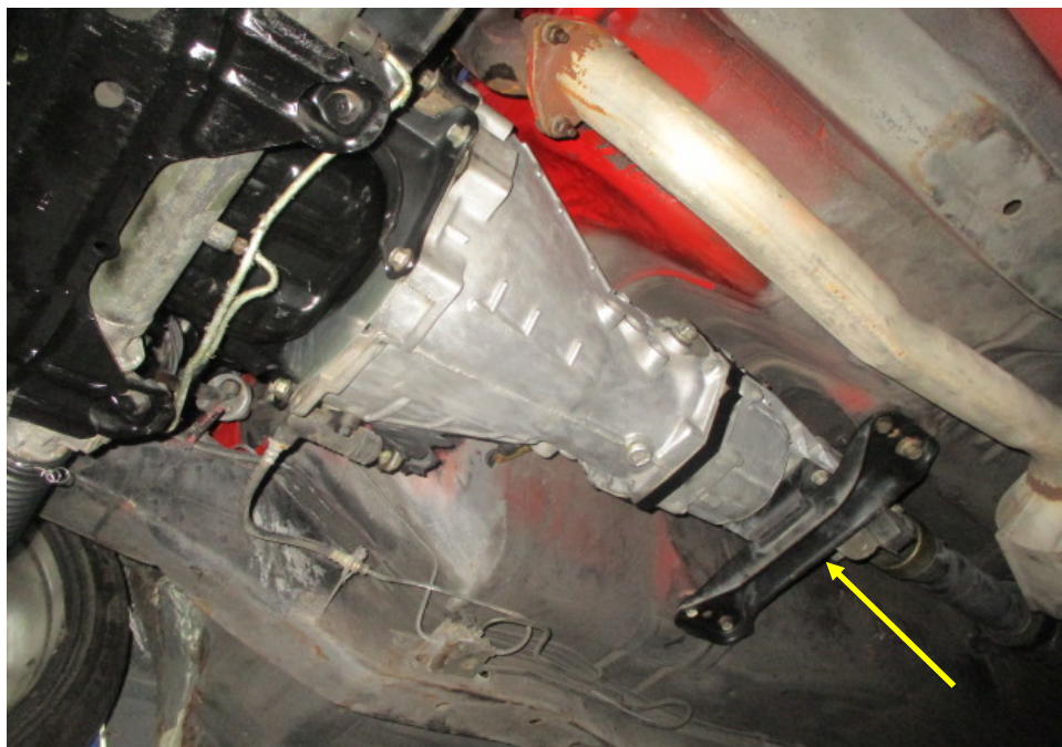
Photo 3 shows a general view of the bracket (arrowed) that was mounted to the underside of the Motor Car's floorboard, via bolts and nuts. The bracket supports the rear (output) side of the transmission assembly.
