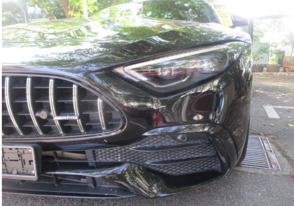
Photo 11 shows a closer view of the Motor Car's front bumper, front bumper left lower grille, front bumper left sensor and front left headlamp. The body parts at the frontal portion of the Motor Car were visually examined and it was observed that the repair/restoration works carried out to the damaged area of the Motor Car (refer to photograph 1 & 2 above) were reasonably adequate and in order.
