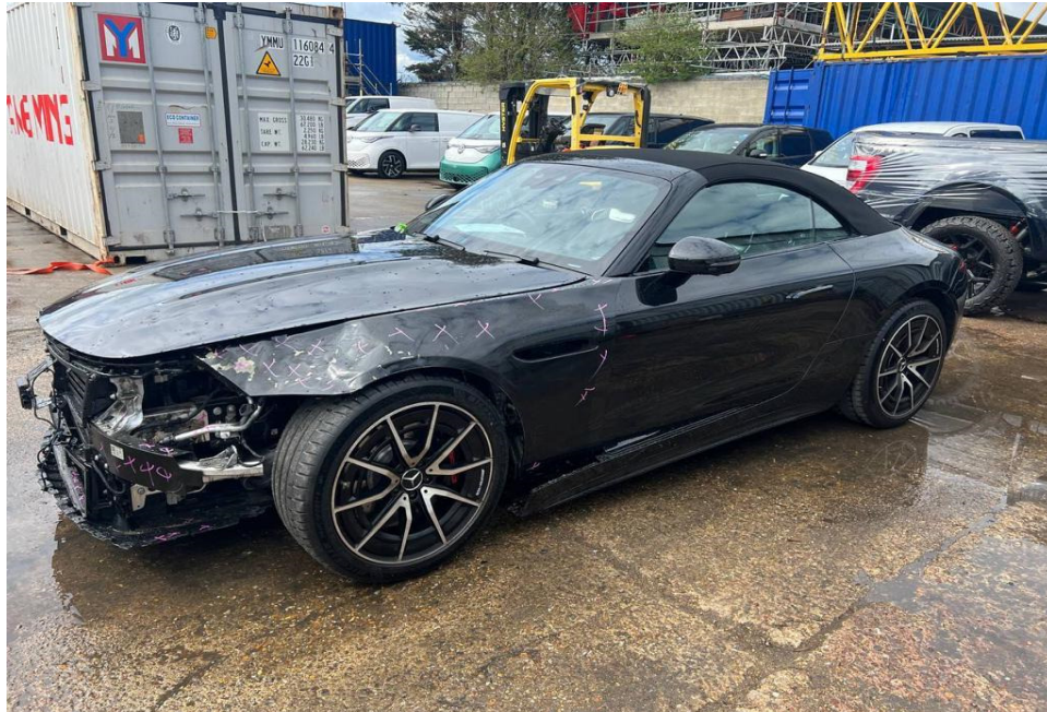
Photo 1 shows the front left body of the Motor Car (photograph provided to me). The Motor Car was observed to have sustained damage at its frontal portion. The front left fender and left side rocker panel garnish were amongst the body parts that were observed to have been damaged. The Motor Car's front bumper and all its related parts and attachments like the front bumper left lower grille and front bumper sensors amongst others, were also missing/dislodged/damaged.
