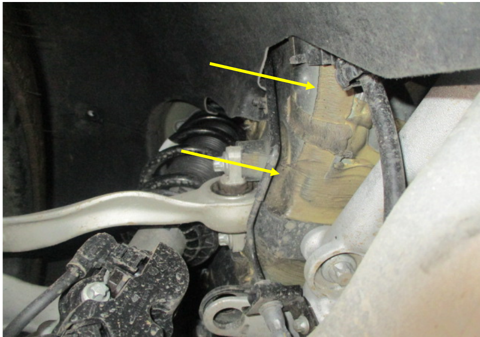
Photo 32 shows the chassis/structural body at the underside front left of the Motor Car. The original factory sealant (arrowed) at the joints along the chassis/structural body was observed to be untouched. In general, I had found no work was carried out on the chassis/structural body of the Motor Car. The chassis/structural body of the Motor Car was originally fitted.
