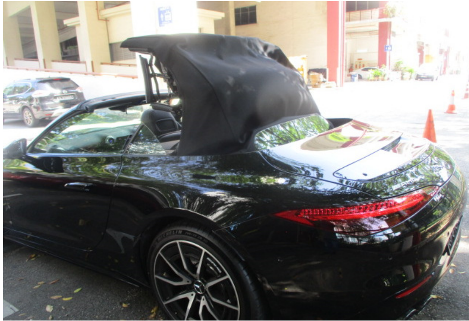
Photo 19 shows the Motor Car's soft top roof being tested. It was observed that as a safety feature, the soft top roof could only open and close when the Motor Car was in a stationary position or at low travelling speed. When opened, the soft top roof is completely folded into the rear compartment with no parts protruding out of the Motor Car's body. The soft top roof was also found adequately secured to the "A" pillar after closing.
