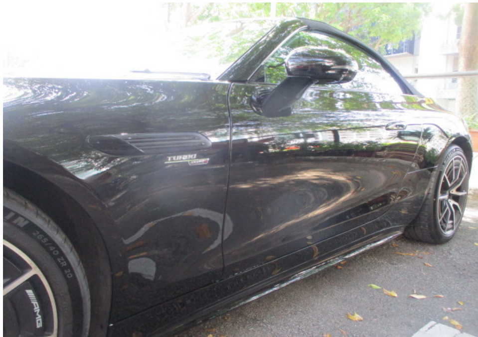
Photo 10 shows a closer view of the Motor Car's front left fender, front left door and left side rocker panel garnish. The body parts at the frontal portion of the Motor Car were visually examined and it was observed that the repair/restoration works carried out to the damaged area of the Motor Car (refer to photograph 1 & 2 above) were reasonably adequate and in order.
