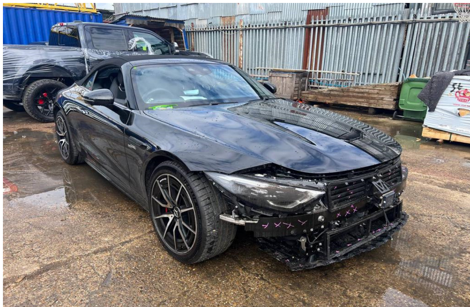
Photo 2 shows the front right body of the Motor Car (photograph provided to me). The Motor Car was observed to have sustained damage at its frontal portion. The front right headlamp was amongst the body parts that were observed to have been damaged. The Motor Car's front grille, front emblem, front number plate garnish, front bumper and all its related parts and attachments like the front bumper centre lower grille, front bumper right lower grille and front bumper sensors amongst others, were also missing/dislodged/damaged.
