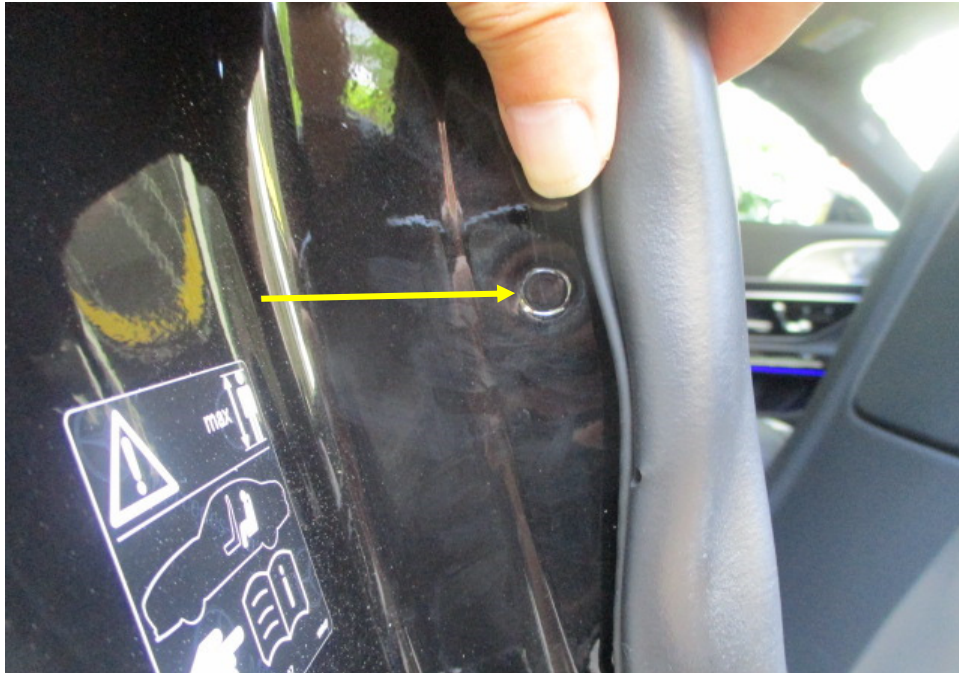
Photo 37 shows the right side rear body panel of the Motor Car. I did not find any weld marks other than original spot weld marks (arrowed) on the right side rear body panel of the Motor Car, which indicates that there was no re-welding works carried out. In general, I had found all the non-detachable body panels of the Motor Car to be originally fitted at the time of my inspection.
