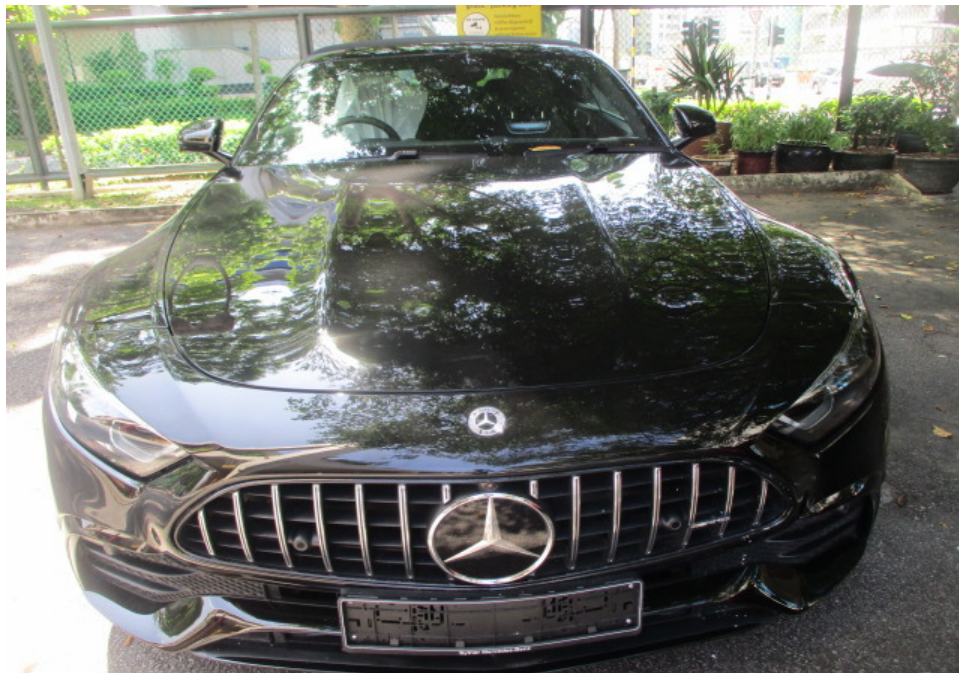
Photo 12 shows a closer view of the Motor Car's front bonnet, front grille and front emblem. The body parts at the frontal portion of the Motor Car were visually examined and it was observed that the repair/restoration works carried out to the damaged area of the Motor Car (refer to photograph 1 & 2 above) were reasonably adequate and in order.
