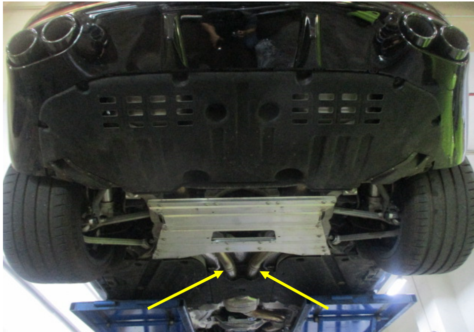
Photo 28 shows the rear section of the Motor Car's exhaust system. My examination of the Motor Car's exhaust system revealed no sign(s) or indication(s) of any cut or weld marks along its exhaust pipes (arrowed), on its rear muffler, on its centre resonator box and on its catalytic converter.
