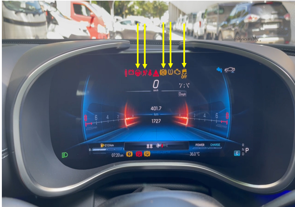
Photo 21 shows the warning lights for the various electronic safety features appearing on the instrument panel of the Motor Car during its self-test when the engine is cranked, in particular the ABS, SRS, EPS, TPM and TCS lights (arrowed).
