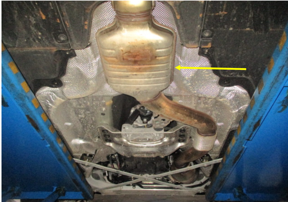
Photo 29 shows the front section of the Motor Car's exhaust system. My examination of the Motor Car's exhaust system revealed no sign(s) or indication(s) of any cut or weld marks along its exhaust pipes, on its rear muffler, on its centre resonator box (arrowed) and on its catalytic converter.
