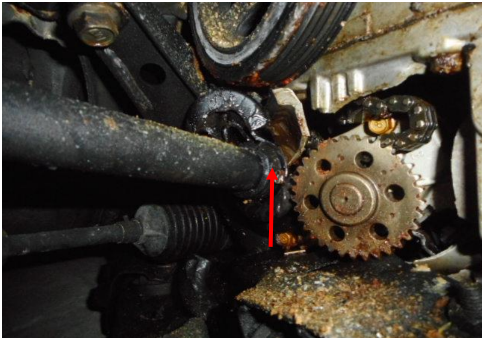
Photo 28 shows the various undercarriage components at the front right wheel of the Motor Car, in particular the driveshaft (arrowed) was observed to be damaged and broken off from the engine as a result of the accident.
