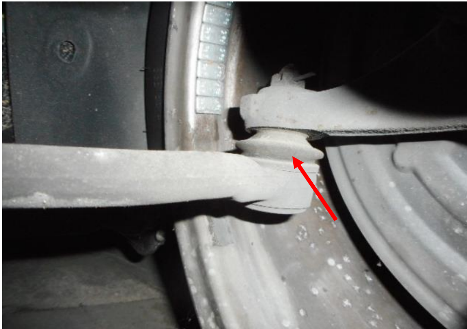
Photo 27 shows the various undercarriage components at the front left wheel of the Motor Car, in particular the steering tie rod (red arrow) and the driveshaft (yellow arrow). The various steering components were all found to be intact. There was also no sign of fluid stain observed on the various undercarriage components at the front left wheel of the Motor Car.
