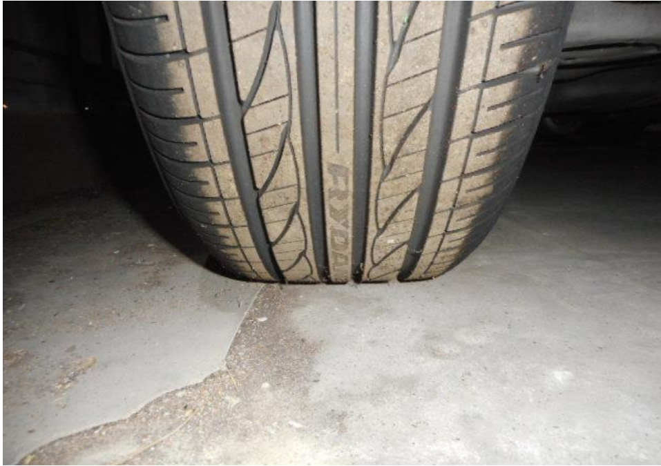
Photo 13 shows the condition of the rear left tyre of the Motor Car, which was observed to be in serviceable condition with remaining tread depth of approximately 6.9mm. The tyre was also observed to be sufficiently inflated for vehicular operation with no tear, cut or burst mark(s).
