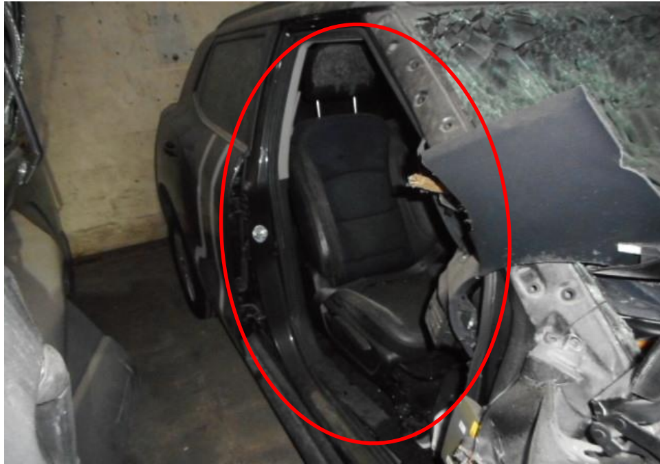
Photo 7 shows a general view of the Motor Car's right body at the time of my inspection. The right portion front right door (circled) was observed to be removed by SCDF for extraction purpose after the accident.
