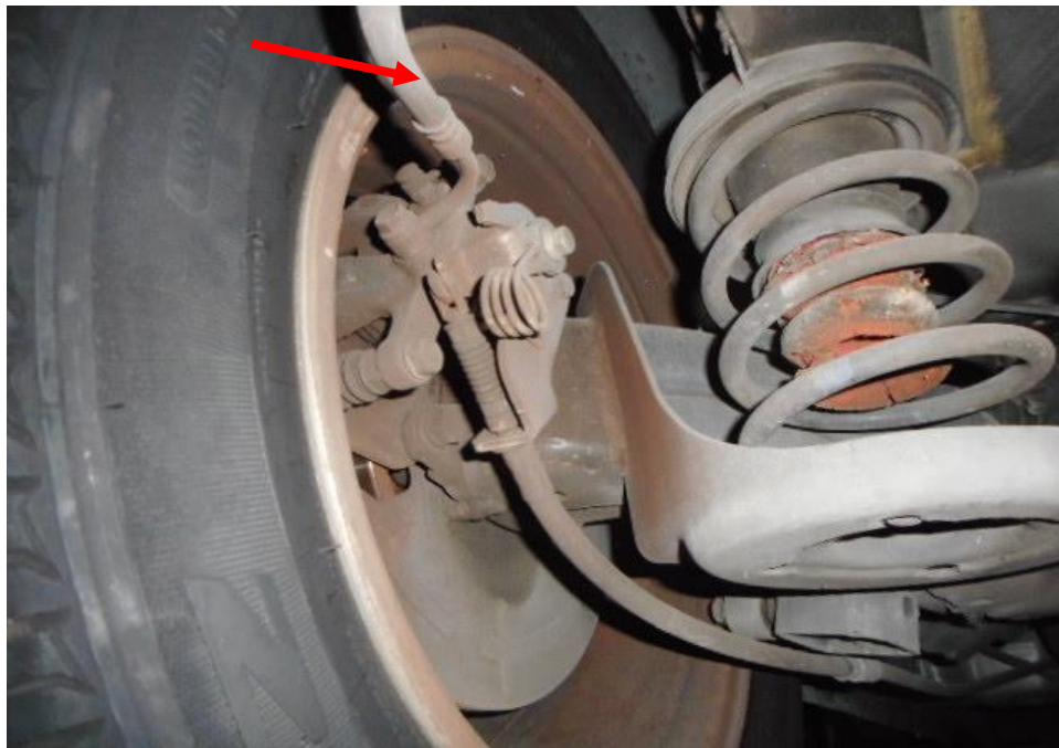
Photo 22 shows the brake hose/pipe (arrowed) at the rear left wheel of the Motor Car. No leakage of brake fluid was observed. Visual examination of the various components of the braking system like the brake caliper and etc had revealed to be intact and without visible damage.
