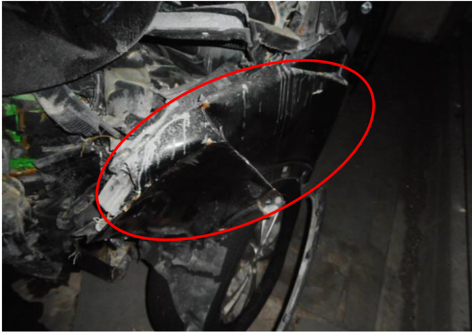
Photo 5 shows the close up view of the Motor Car's front body at the time of my inspection. The Motor Car was observed to have sustained damage at its front portion. Its front left fender (yellow circle) was damaged as a result of the accident.
