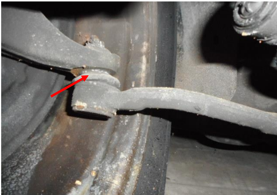
Photo 26 shows the various undercarriage components at the front left wheel of the Motor Car, in particular the steering tie rod (arrowed). The various steering components were all found to be intact.
