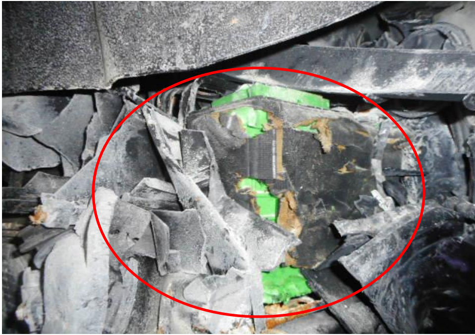
Photo 18 shows the close up view of the Motor Car's front body at the time of my inspection. The Motor Car was observed to have sustained damage at its front portion. Its ignition system battery (circled) was amongst the various components in the engine compartment were also damaged as a result of the accident.
