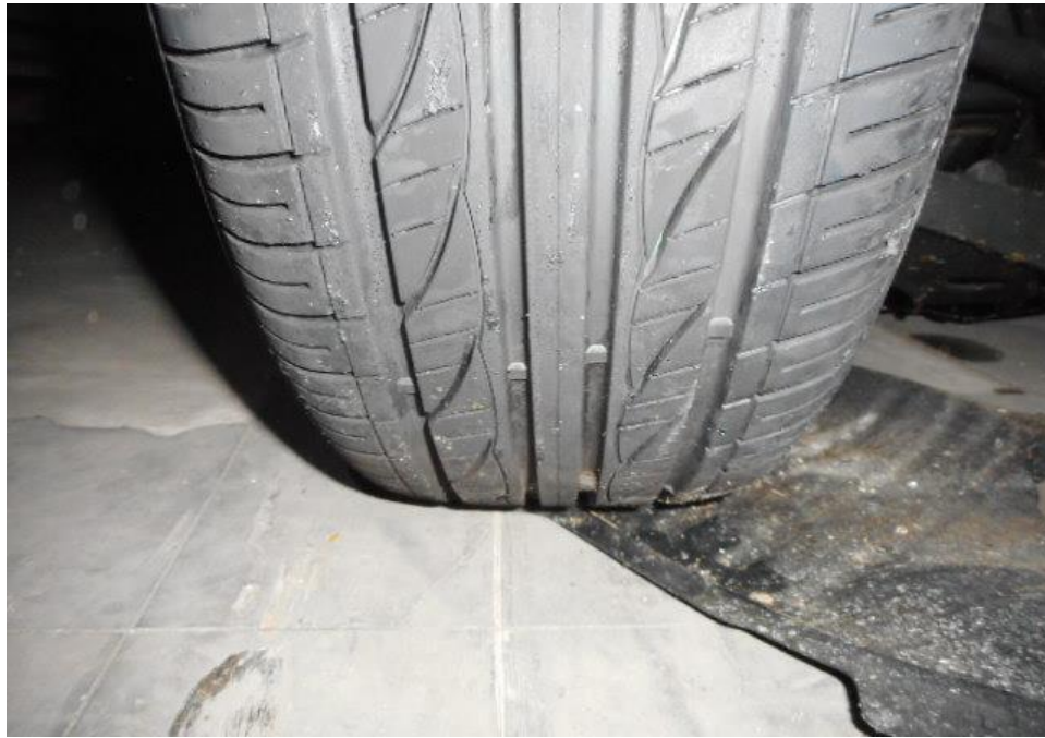
Photo 11 shows the condition of the front right tyre of the Motor Car, which was observed to be in serviceable condition with remaining tread depth of approximately 6.5mm. The tyre was also observed to be sufficiently inflated for vehicular operation with no tear, cut or burst mark(s).
