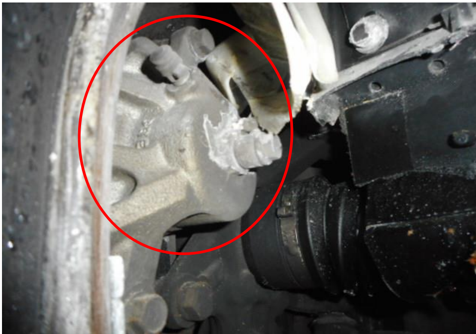
Photo 24 shows the close up view of the front right wheel rim and tyre, the viewing of the brake caliper and brake hose components at the front right wheel of the Motor Car was blocked due to the induced damages sustained to the engine and undercarriage component (circled) as a result of the accident.
