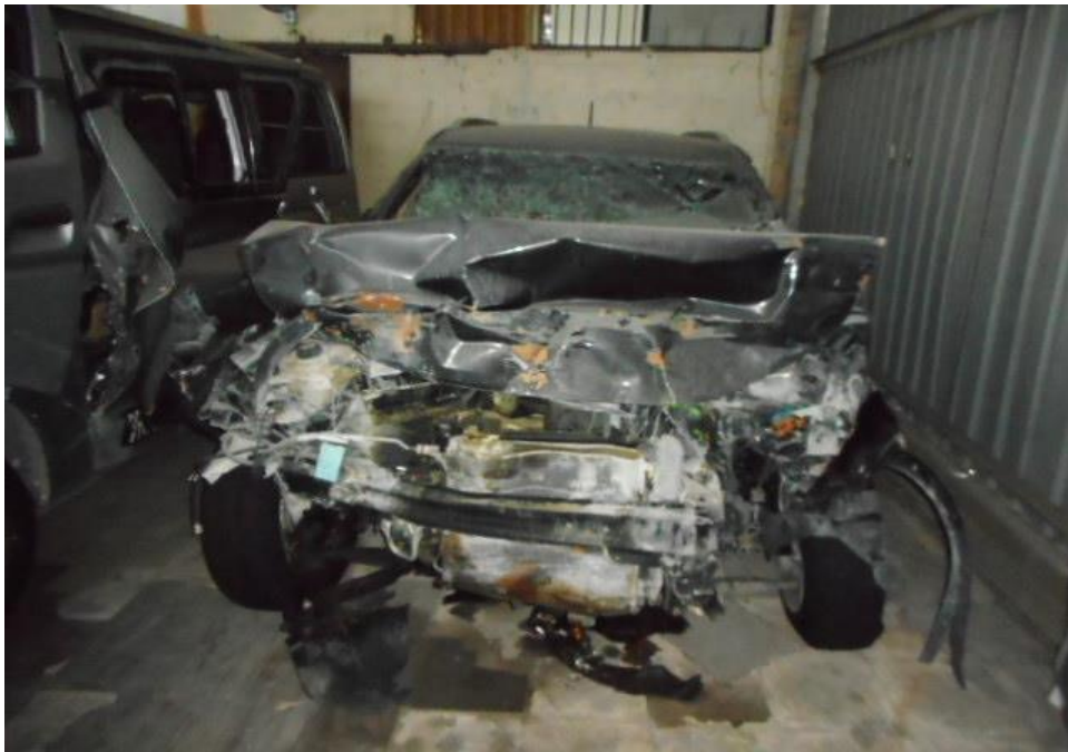
Photo 2 shows a general view of the Motor Car's front body at the time of my inspection. The Motor Car was observed to have sustained damage at its front portion. Its front windscreen, front bonnet, front bumper panel, front right and left fender was amongst the body parts and various engine components were also damaged as a result of the accident. The Supplemental Restraint System (SRS) was activated as a result of the accident.
