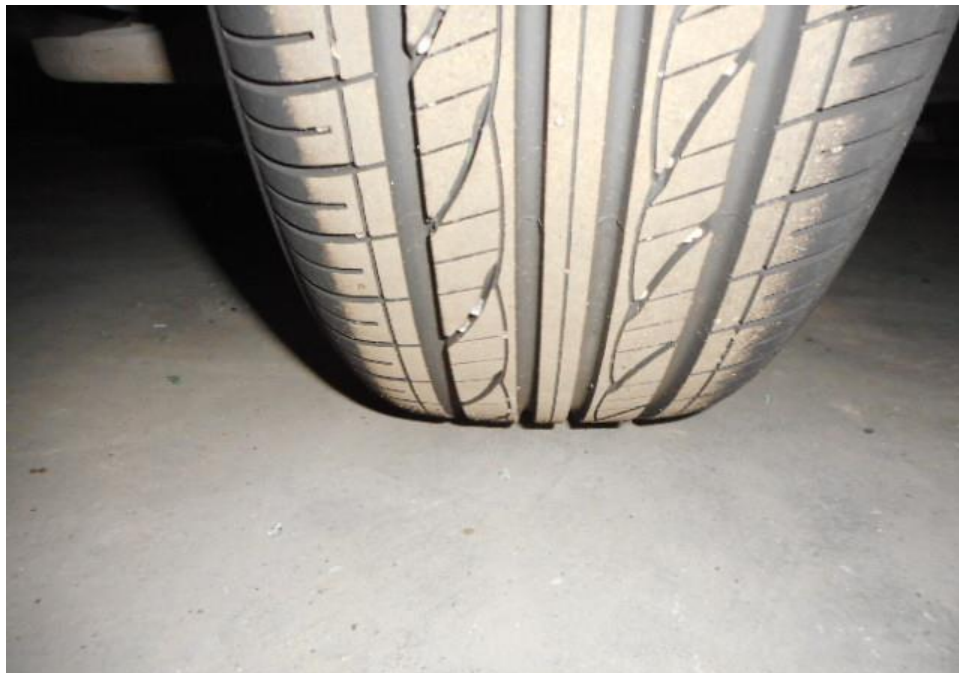
Photo 12 shows the condition of the rear right tyre of the Motor Car, which was observed to be in serviceable condition with remaining tread depth of approximately 6.5mm. The tyre was also observed to be sufficiently inflated for vehicular operation with no tear, cut or burst mark(s).
