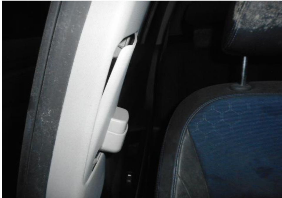
Photo 30 shows that the seat belt on the right seat was worn at the material time of accident as the safety pre-tensioners was activated at the moment of impact and caused the seat belt to be locked into the last position and the seat belt was cut for SCDF rescue extraction purposes.
