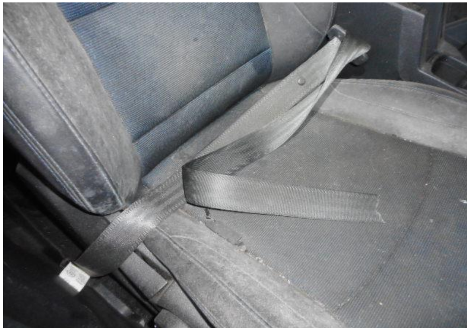
Photo 31 shows that the seat belt on the right seat was worn at the material time of accident as the safety pre-tensioners was activated at the moment of impact and caused the seat belt to be locked into the last position and the seat belt was cut for SCDF rescue extraction purposes.
