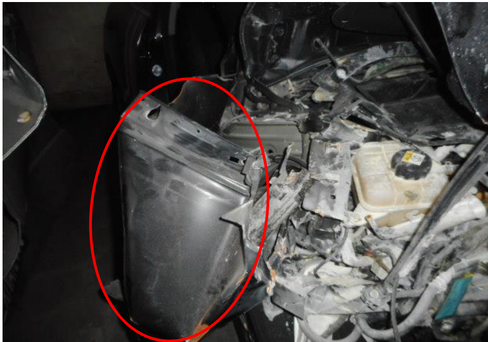
Photo 4 shows the close up view of the Motor Car's front body at the time of my inspection. The Motor Car was observed to have sustained damage at its front portion. Its front right fender (circled) was damaged as a result of the accident.
