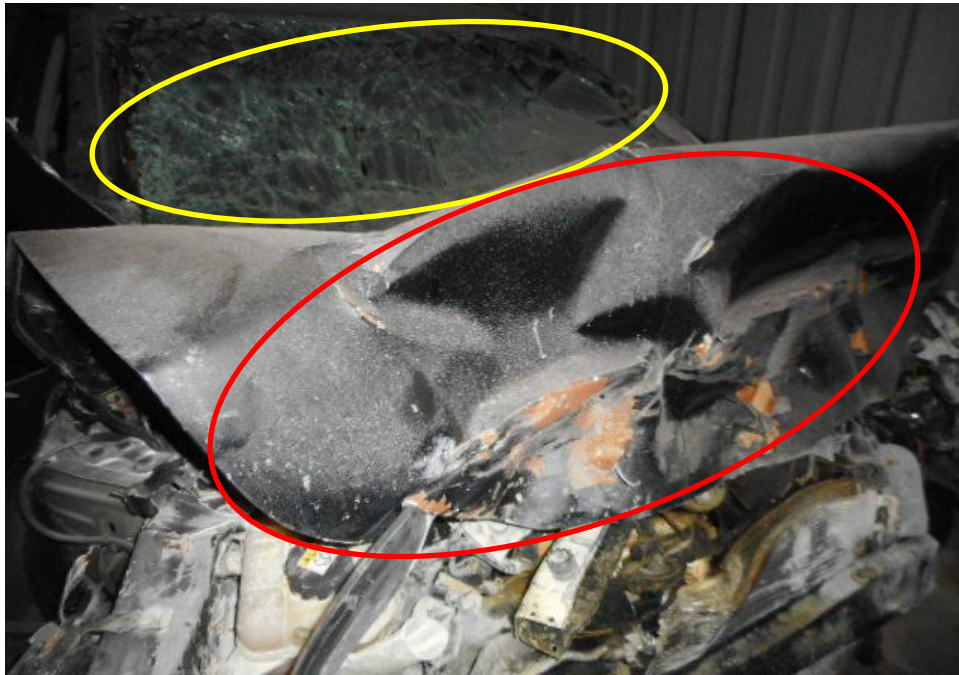
Photo 3 shows the close up view of the Motor Car's front body at the time of my inspection. The Motor Car was observed to have sustained damage at its front portion. Its front bonnet (red circle) and front windscreen (yellow circle) was damaged as a result of the accident.
