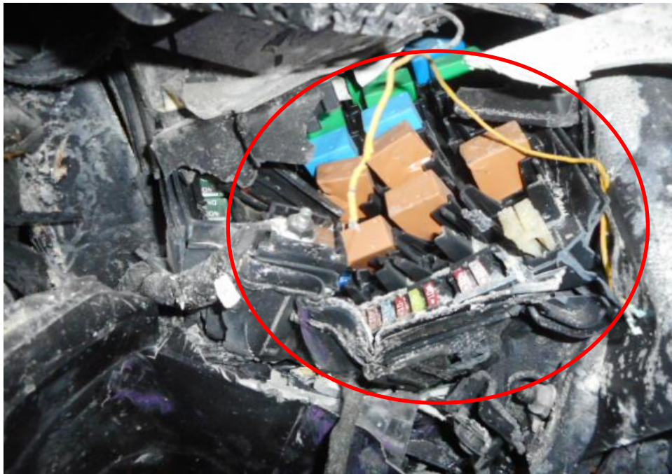
Photo 20 shows the close up view of the Motor Car's front body at the time of my inspection. The Motor Car was observed to have sustained damage at its front portion. Its electrical components (circled) was amongst the various components in the engine compartments were also damaged as a result of the accident.
