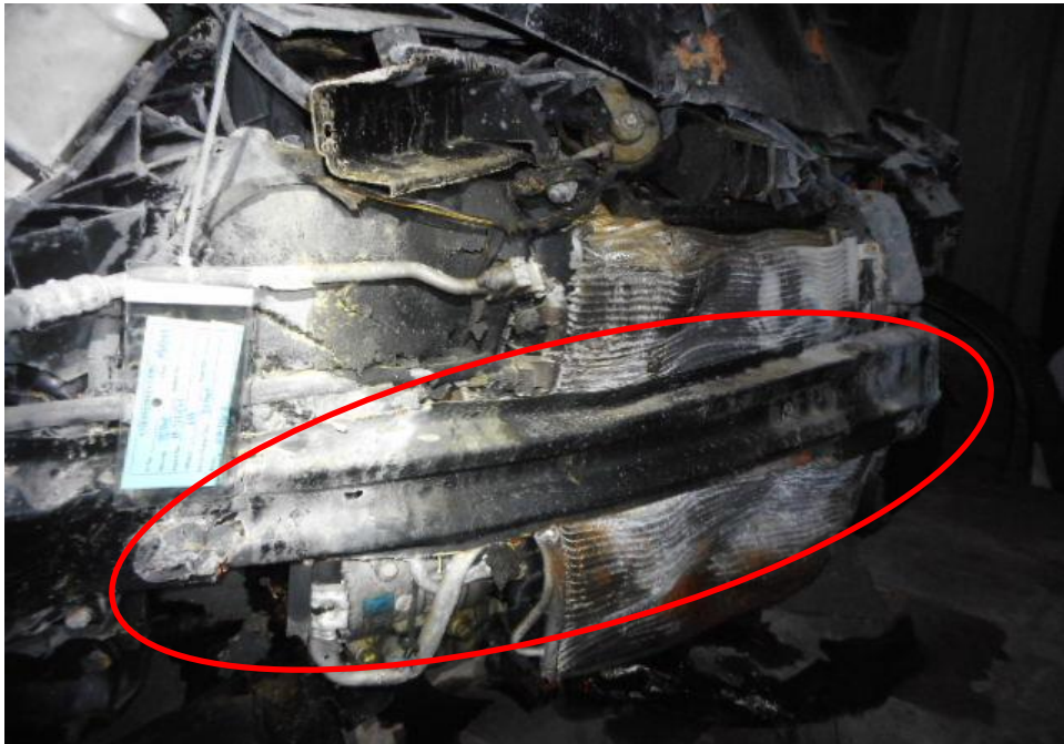
Photo 6 shows the close up view of the Motor Car's front body at the time of my inspection. The Motor Car was observed to have sustained damage at its front portion. Its front bumper reinforcement panel (circled) was damaged as a result of the accident.
