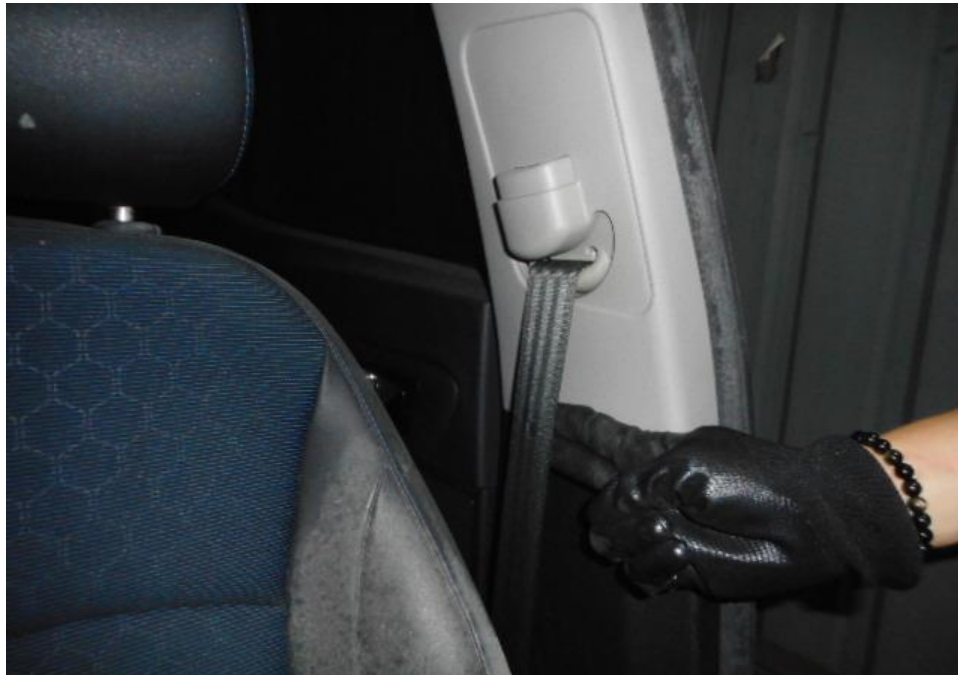
Photo 32 shows that the seat belt on the left seat was not worn at the material time of accident as the safety pre-tensioners was activated at the moment of impact and caused the seat belt to be locked into the last position.
