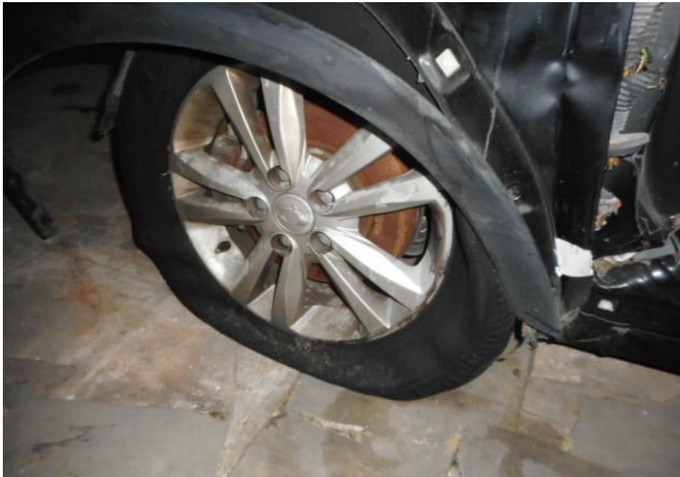
Photo 14 shows the condition of the front left tyre of the Motor Car, which was observed to be in unserviceable condition with remaining tread depth of approximately 6.1mm. The tyre, which was wrapped around alloy wheel rim, was also observed to be with burst mark and also deflated as a result of the accident.
