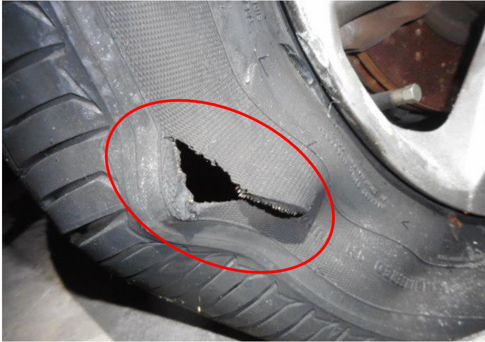
Photo 15 shows the close up view of the front right tyre of the Motor Car, which was observed to be in unserviceable condition with remaining tread depth of approximately 4mm. The tyre, which was wrapped around alloy wheel rim, was also observed to be cut and also deflated (circled) as a result of the accident.
