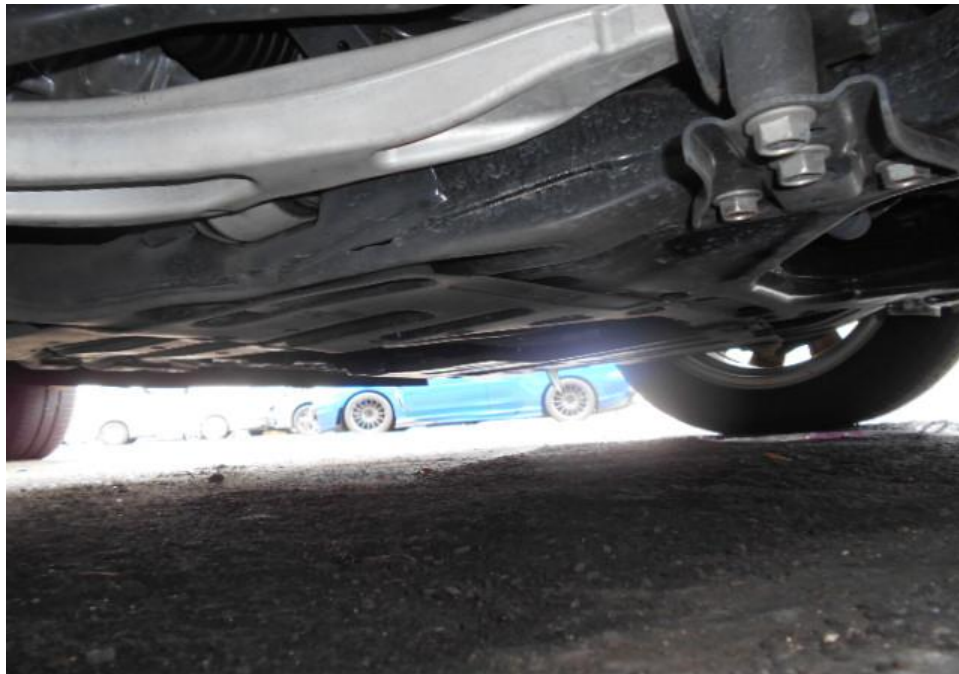
Photo 17 shows the undercarriage of the Motor Car, where the engine housing and transmission housing are located. I did not find any sign(s) or indication(s) of fluid leak and/or fluid stain(s) on the underside of the Motor Car.
