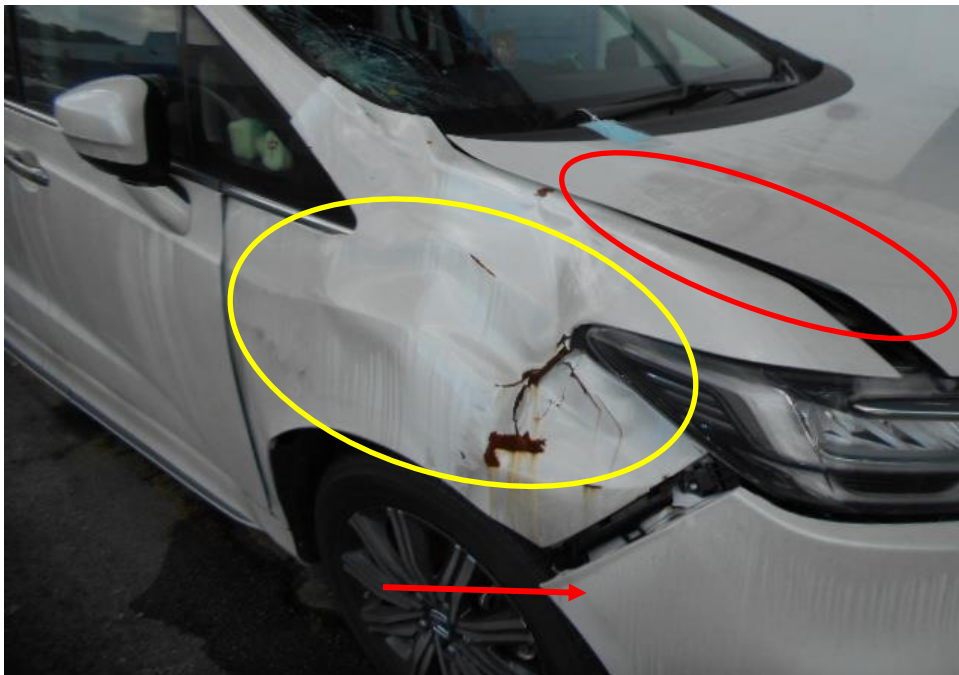
Photo 4 shows the close up view of the Motor Car's front body at the time of my inspection. The Motor car was observed to have sustained damage at its front portion. Its front right fender (yellow circle) front bonnet (red circle) and front bumper (arrowed) was damaged as a result of the accident.
