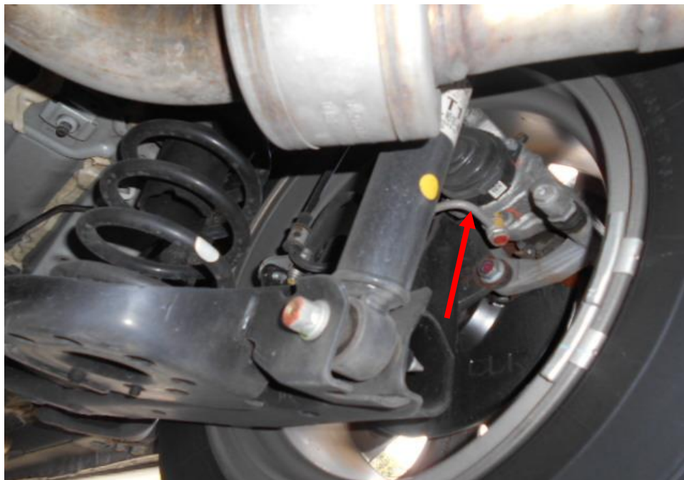
Photo 19 shows the brake hose/pipe (arrowed) at the rear right wheel of the Motor Car. No leakage of brake fluid was observed. Visual examination of the various components of the braking system like the drum brake and brake hose etc. had revealed all to be intact and without visible damage.
