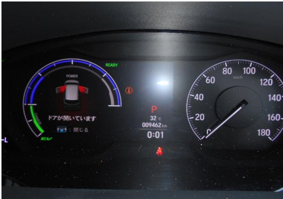
Photo 26 shows no warning lights illuminated on the instrument panel of the Motor Car after the engine was cranked. This would suggest that there was no abnormality to the electronic operating system of the Motor Car, like the ABS, EPS, TCS and SRS etc.
