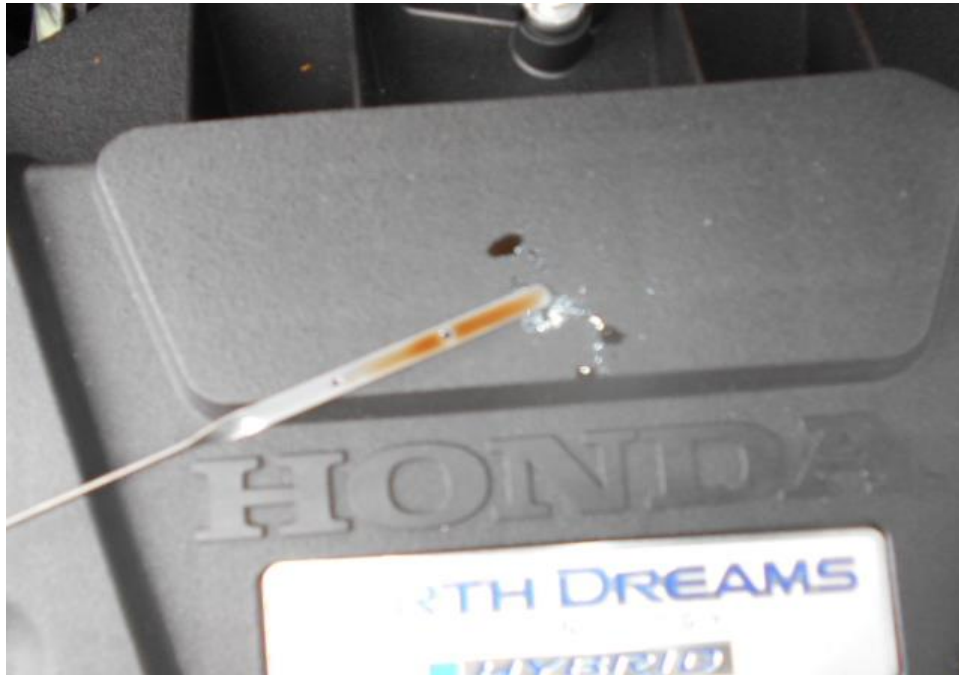
Photo 16 shows the engine oil dipstick of the Motor Car at the time of my inspection. The engine oil was observed to be of sufficient level without any visible contamination.
