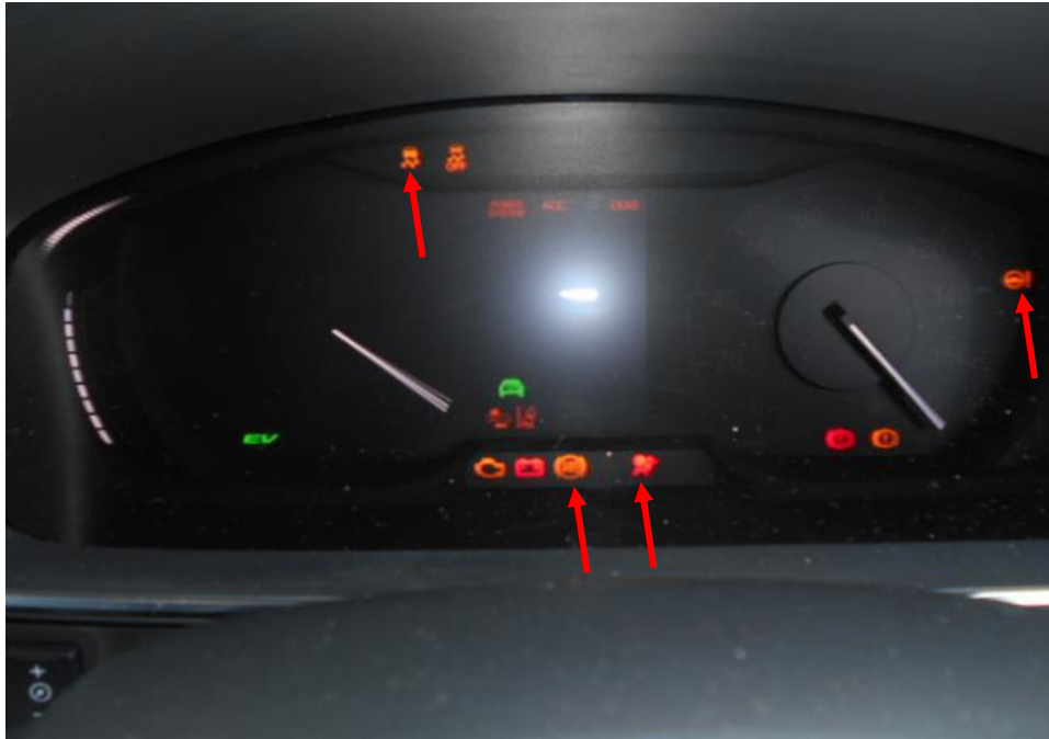
Photo 25 shows the warning light for Anti-Lock Brake System (ABS), Electric Power Steering System (EPS), Traction Control System (TCS) and Supplemental Restraint System (SRS) (arrowed) appearing on the instrument panel of the Motor Car during the self-test of its various electronic operating systems when its engine was cranked.
