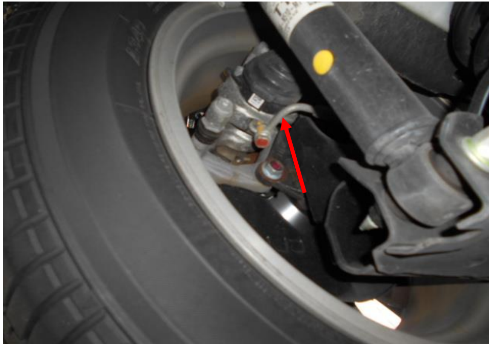
Photo 18 shows the brake hose/pipe (arrowed) at the rear left wheel of the Motor Car. No leakage of brake fluid was observed. Visual examination of the various components of the braking system like the drum brake and brake hose etc. had revealed all to be intact and without visible damage.
