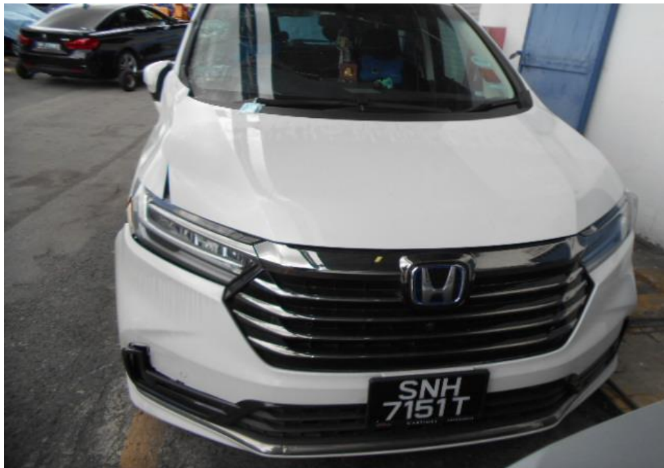
Photo 2 shows a general view of the Motor Car's front body at the time of my inspection. The Motor car was observed to have sustained damage at its front portion. Its front windscreen, front bonnet, front right fender and front bumper was amongst the body parts damaged as a result of the accident.
