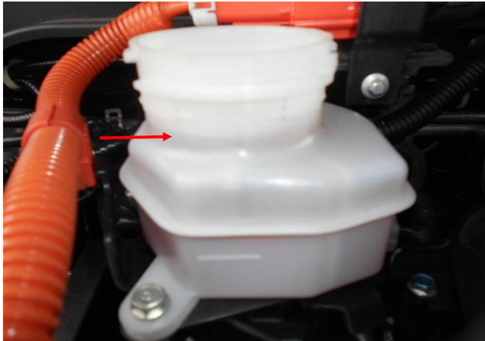
Photo 14 shows the brake fluid reservoir of the Motor Car at the time of my inspection. The brake fluid was observed to be of sufficient level (arrowed) without any visible contamination.
