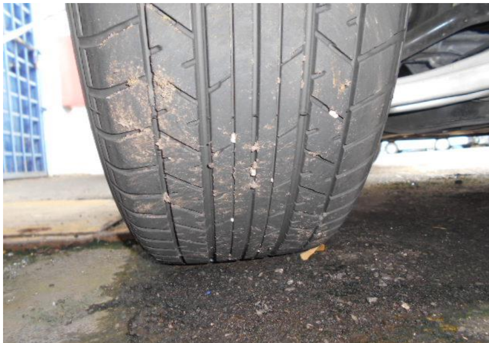
Photo 12 shows the condition of the front left tyre of the Motor Car, which was observed to be in serviceable condition with remaining tread depth of approximately 5mm. The tyre was also observed to be sufficiently inflated for vehicular operation with no tear, cut or burst mark(s).
