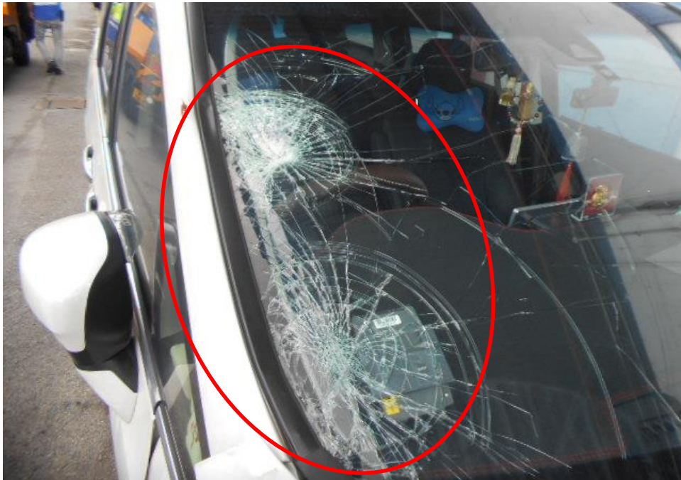
Photo 3 shows the close up view of the Motor Car's front body at the time of my inspection. The Motor Car was observed to have sustained damage at its front portion. Its front windscreen (circled) was damaged as a result of the accident
