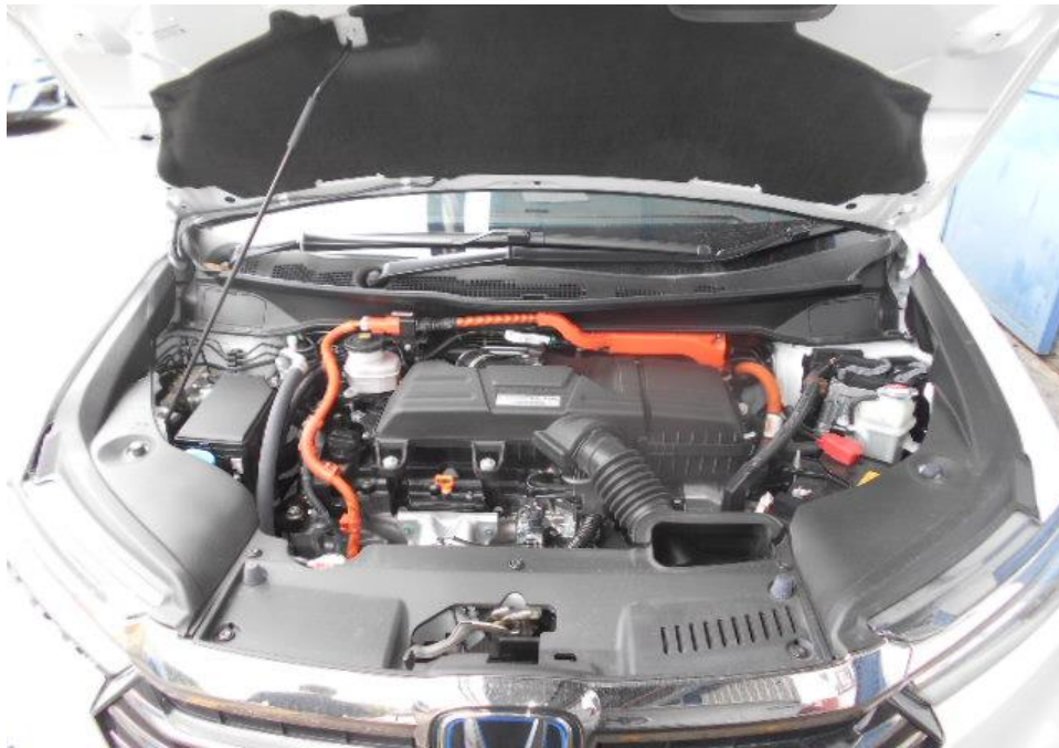
Photo 13 shows a general view of the Motor Car's engine compartment. The various parts and components inside the engine compartment were unaffected by the accident. There was also no sign(s) or indication(s) of fluid leakage and/or fluid stain within the engine bay.
