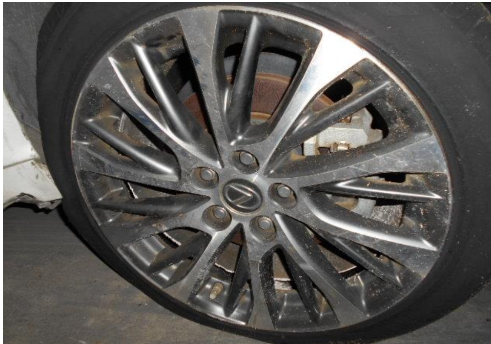
Photo 16 shows the condition of the front right tyre of the Motor Car, which was observed to be in unserviceable condition with remaining tread depth of approximately 7.2mm. The tyre was also observed to be deflated as a result of the damaged wheel rim as a result of the accident, however there was no tear, cut or burst mark(s) on the tyre.
