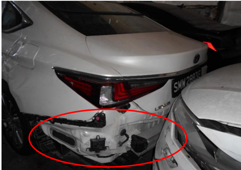
Photo 15 shows a close up view of the Motor Car's rear body at the time of my inspection. The rear portion of the Motor Car was observed to sustain damages as a result of the accident. Its rear bumper (circled) was damaged as a result of the accident.
