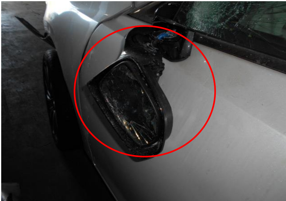
Photo 12 shows a close up view of the Motor Car's left body at the time of my inspection. The Motor car was observed to have sustained damage at its left portion. Its left rear view mirror (circled) was amongst the body parts damaged as a result of the accident.
