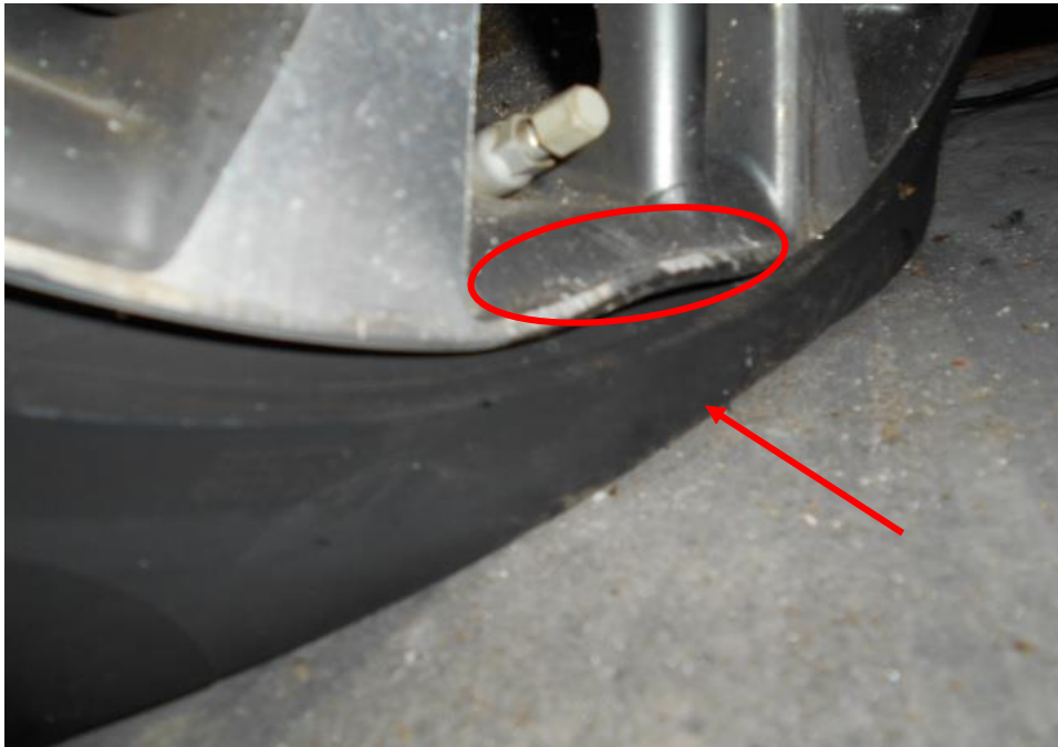
Photo 17 shows the condition of the front right tyre and wheel rim of the Motor Car, the tyre was also observed to be deflated (arrowed) as a result of the damaged wheel rim (arrowed) as a result of the accident, however there was no tear, cut or burst mark(s) observed on the tyre.
