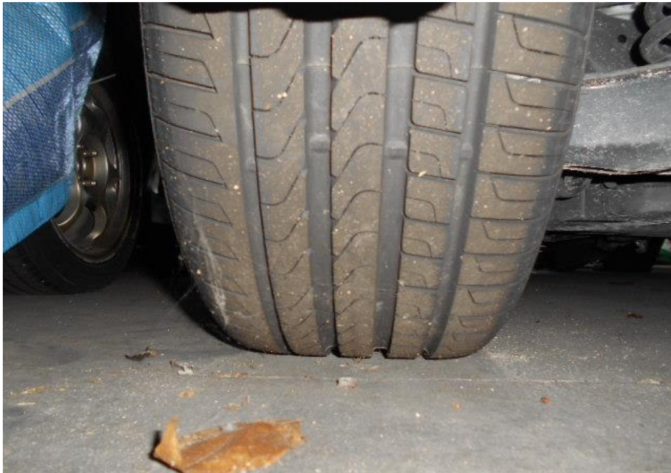
Photo 19 shows the condition of the rear left tyre of the Motor Car, which was observed to be in serviceable condition with remaining tread depth of approximately 5.0mm. The tyre was also observed to be sufficiently inflated for vehicular operation with no tear, cut or burst mark(s).
