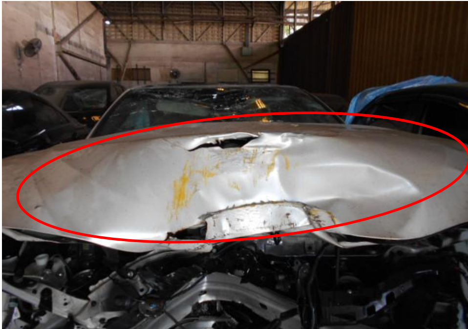
Photo 3 shows the close up view of the Motor Car's front body at the time of my inspection. The Motor car was observed to have sustained damage at its front portion. Its front bonnet (circled) was damaged as a result of the accident.
