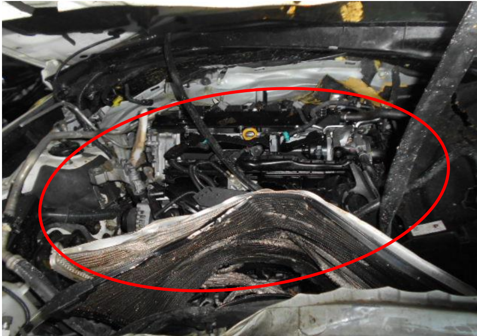
Photo 22 shows a general view of the Motor Car's engine compartment. I had observed that the Motor Car's engine (circled) was badly damaged and crushed as a result of the accident.
