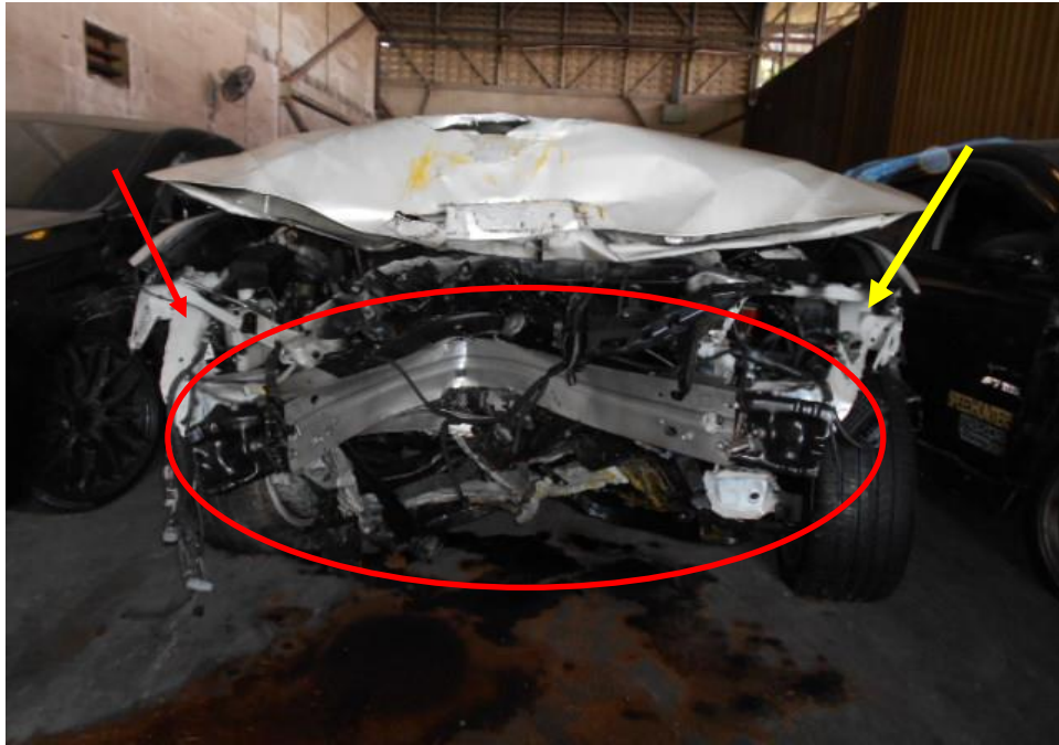
Photo 5 shows the close up view of the Motor Car's front body at the time of my inspection. The Motor car was observed to have sustained damage at its front portion. Its front bumper (circled), its front right headlamp (red arrow) and its front left headlamp (yellow arrow) was damaged as a result of the accident.
