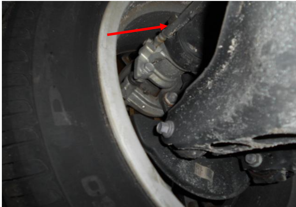
Photo 24 shows the brake hose/pipe (arrowed) at the rear left wheel of the Motor Car. No leakage of brake fluid was observed. Visual examination of the various components of the braking system like the brake caliper to be intact without visible damage.
