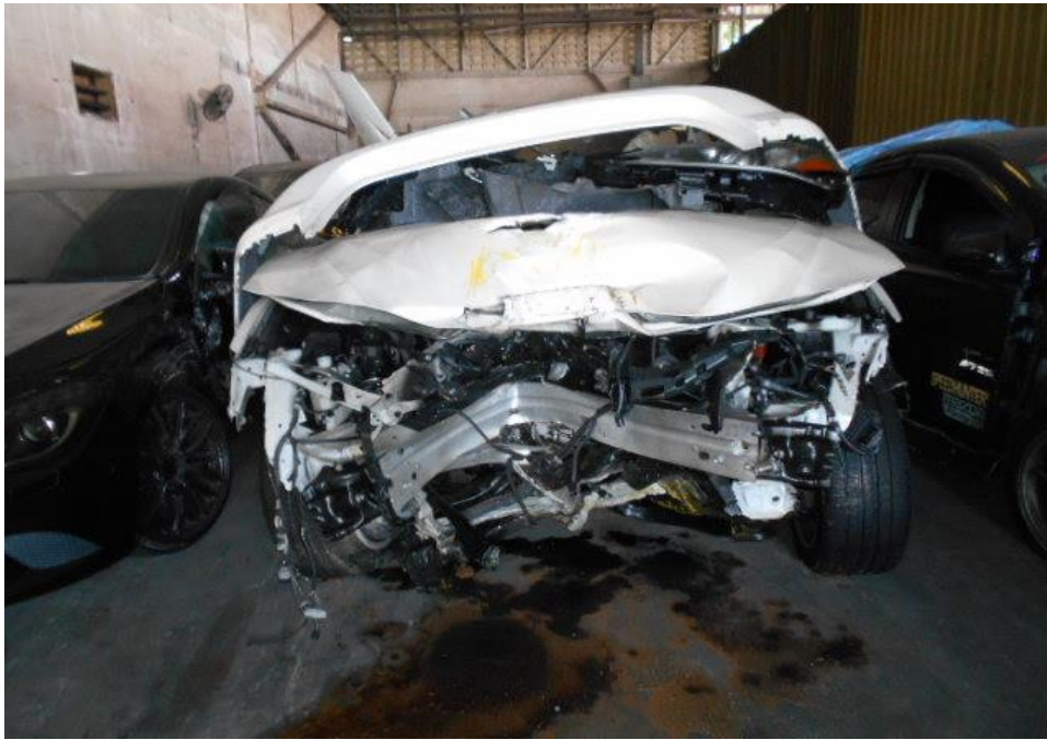
Photo 1 shows a general view of the Motor Car's front body at the time of my inspection. The front windscreen, front bonnet, front bumper, front left fender, front right and left headlamp, Its left and right door panels, roof panel, rear windscreen was amongst the body parts that were damaged as a result of the accident. The Supplemental Restraint System (SRS) was activated as a result of the accident.
