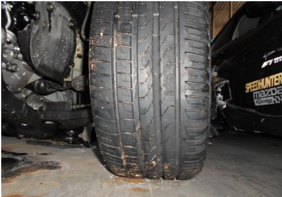
Photo 20 shows the condition of the front left tyre of the Motor Car, which was observed to be in unserviceable condition with remaining tread depth of approximately 5.9mm. The tyre was also observed to be deflated as a result of the damaged wheel rim as a result of the accident, however there was no tear, cut or burst mark(s) on the tyre.
