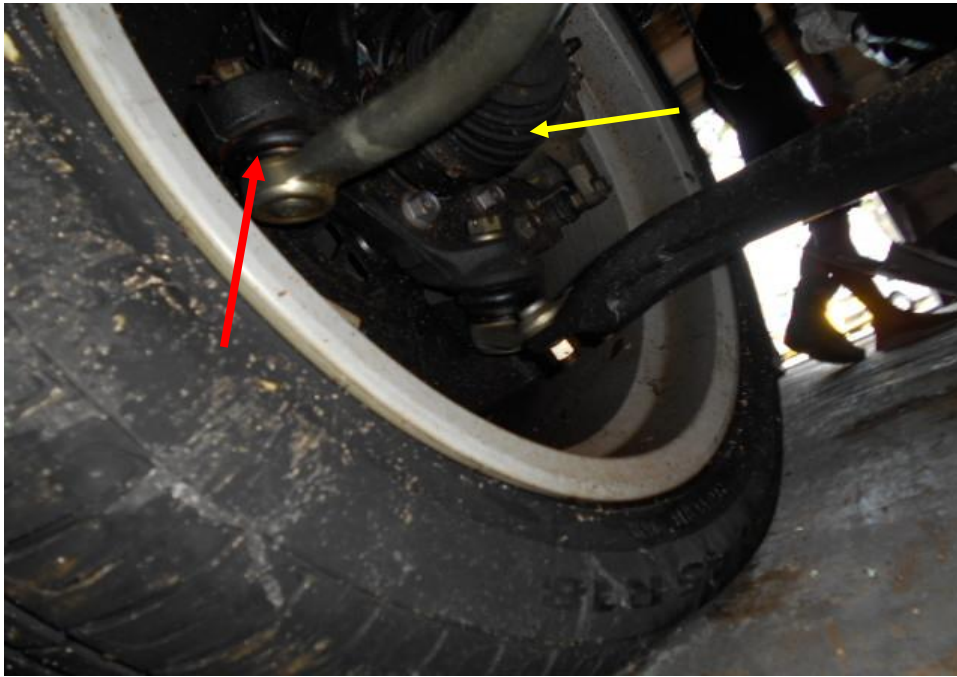
Photo 29 shows the various undercarriage components at the front right wheel of the Motor Car, in particular the steering tie rod (red arrow) and the driveshaft (yellow arrow). The various steering components were all found to be intact.
