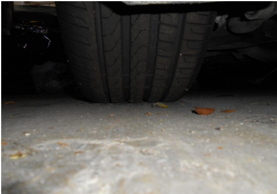
Photo 18 shows the condition of the rear right tyre of the Motor Car, which was observed to be in serviceable condition with remaining tread depth of approximately 9.7mm. The tyre was also observed to be sufficiently inflated for vehicular operation with no tear, cut or burst mark(s).
