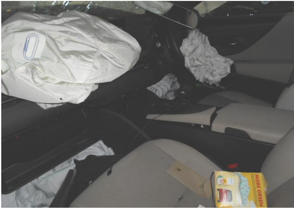
Photo 21 shows the deployment of the Supplemental Restraint System (SRS) airbag in the Motor Car as a result of the accident.
