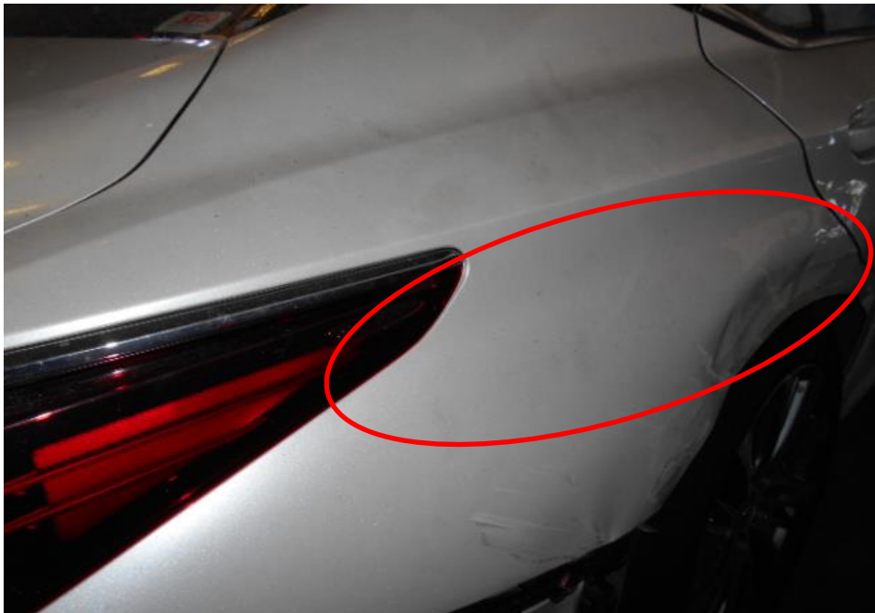
Photo 10 shows a close up view of the Motor Car's right body at the time of my inspection. The Motor car was observed to have sustained damage at its right portion. Its right rear quarter panel was amongst the body parts damaged as a result of the accident.
