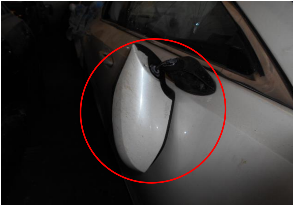
Photo 8 shows a close up view of the Motor Car's right body at the time of my inspection. The Motor car was observed to have sustained damage at its right portion. Its rear right rear view mirror (circled) was amongst the body parts damaged as a result of the accident.
