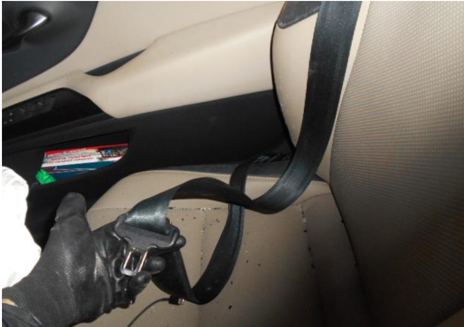
Photo 30 shows that the front right seat belt was worn at the material time of accident as the safety pre-tensioners was activated at the moment of impact and caused the seat belt to be locked into the last position.
