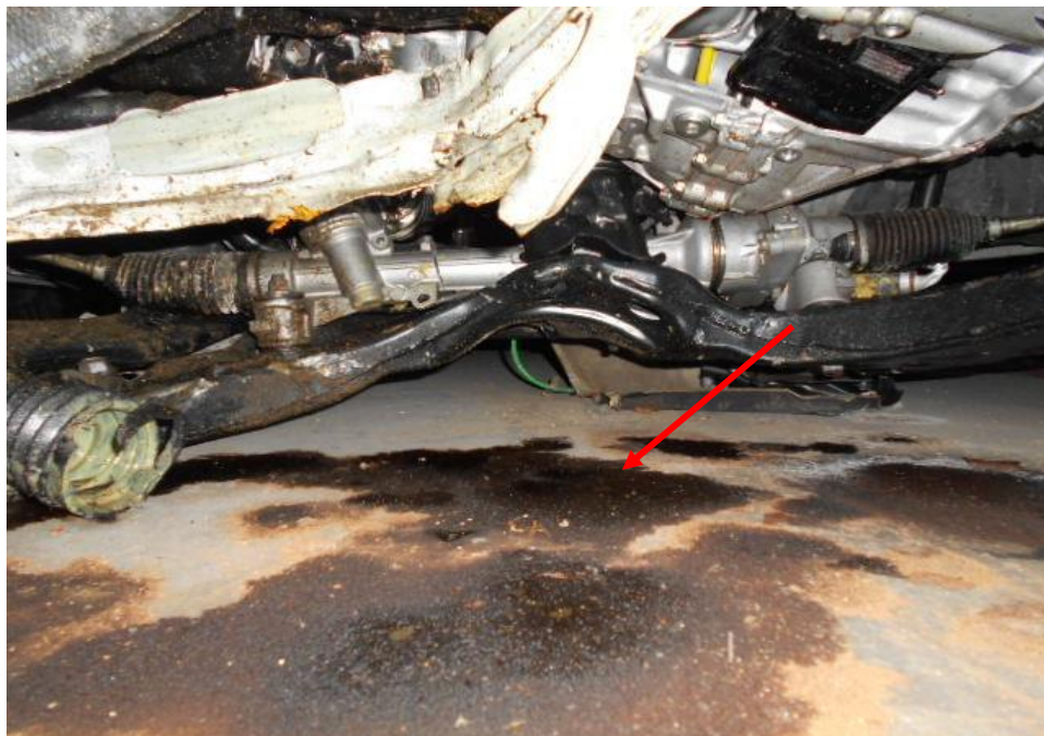
Photo 23 shows the undercarriage of the Motor Car, at the area where the engine housing and transmission housing are located. I observed signs of engine oil (arrowed) on the underside of the Motor Car.
