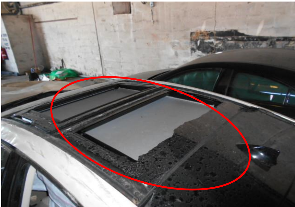
Photo 4 shows the close up view of the Motor Car's top body and roof panel at the time of my inspection. The Motor car was observed to have sustained damage at its top portion. Its roof and sunroof panel (circled) was damaged as a result of the accident.
