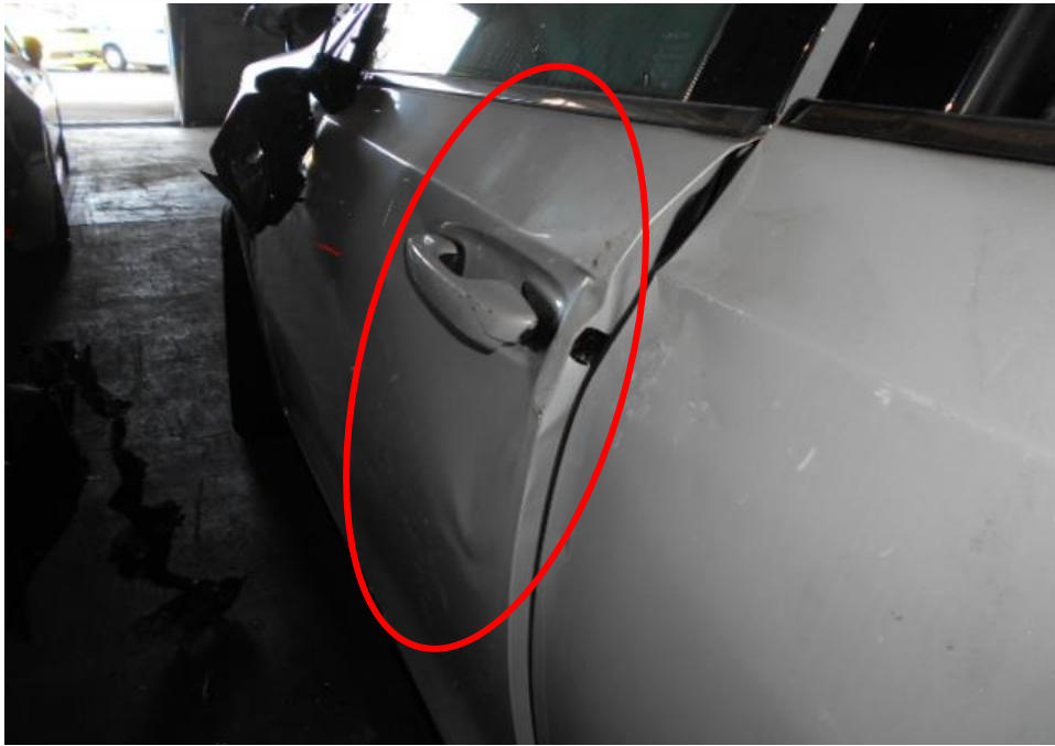
Photo 13 shows a close up view of the Motor Car's left body at the time of my inspection. The Motor car was observed to have sustained damage at its left portion. Its front left door was amongst the body parts damaged as a result of the accident.
