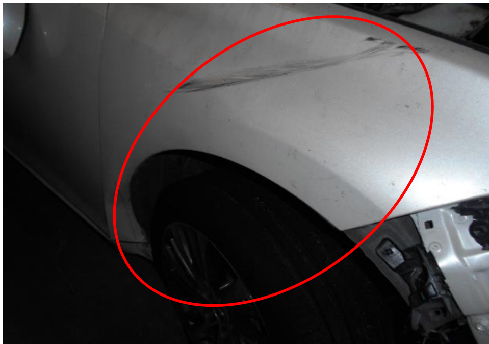
Photo 6 shows the close up view of the Motor Car's front body at the time of my inspection. The Motor car was observed to have sustained damage at its front portion. Its front right fender (circled) was amongst the body part damaged as a result of the accident.
