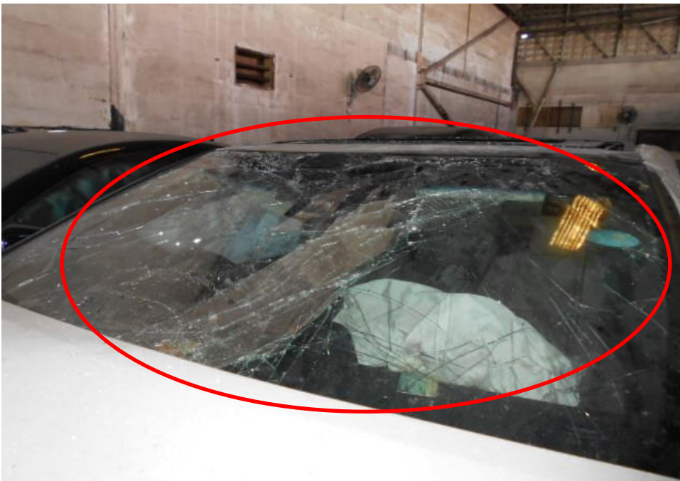
Photo 2 shows the close up view of the Motor Car's front body and roof panel at the time of my inspection. The Motor car was observed to have sustained damage at its front portion. Its front windscreen (circled) was damaged as a result of the accident.
