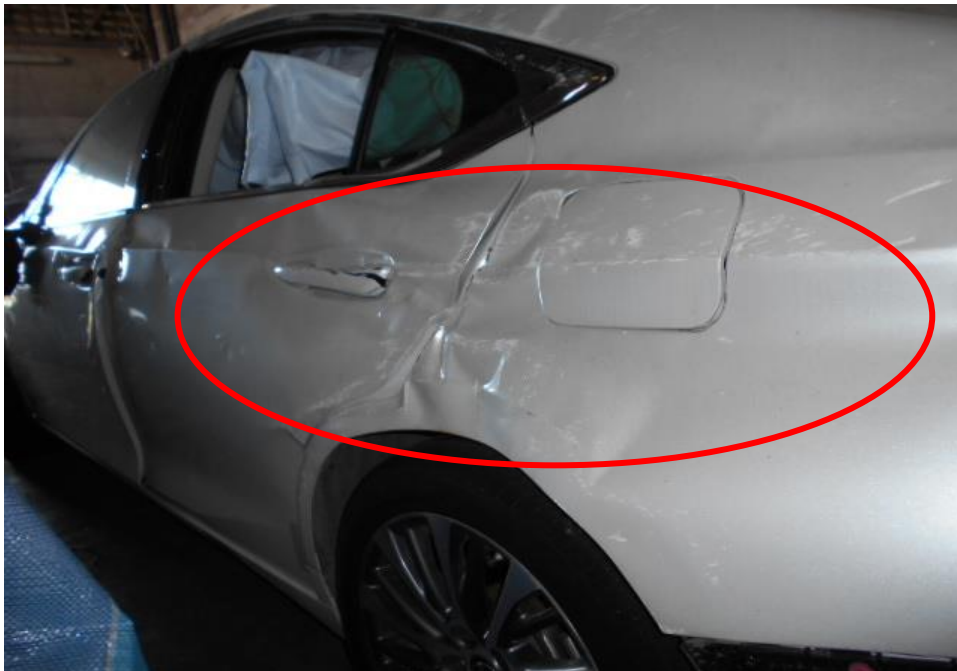
Photo 14 shows a close up view of the Motor Car's left body at the time of my inspection. The Motor car was observed to have sustained damage at its left portion. Its rear left door and rear left quarter panel (circled) was amongst the body parts damaged as a result of the accident.
