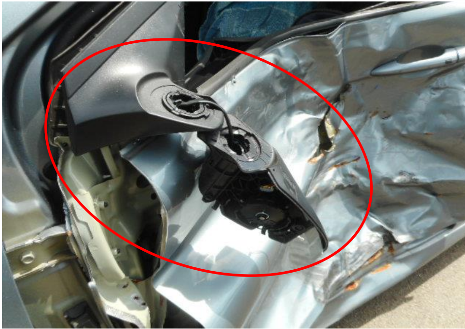
Photo 4 shows a close up view of the Motor Car's left body at the time of my inspection. The left portion of the Motor Car was observed to have sustained damage. Its left rear view mirror (circled) was the body parts that were damaged as a result of the accident.
