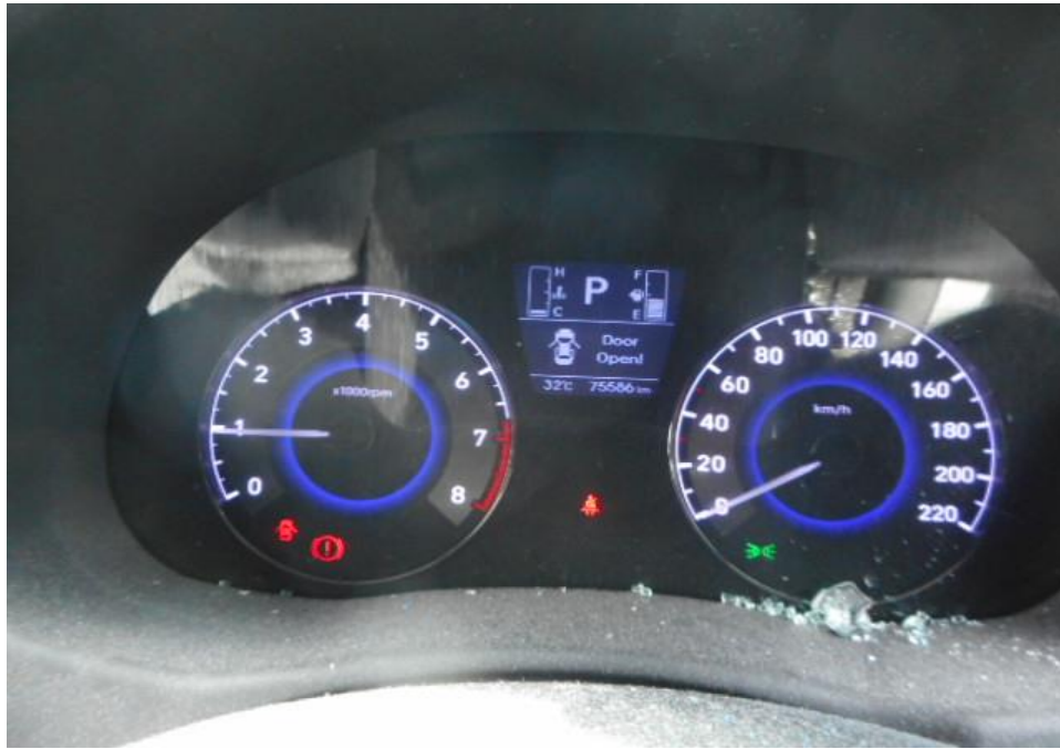
Photo 25 shows no warning lights illuminated on the instrument panel of the Motor Car after the engine was cranked. This would suggest that there was no abnormality to the electronic operating system of the Motor Car, like the ABS, TCS, EPS, SRS and etc.
