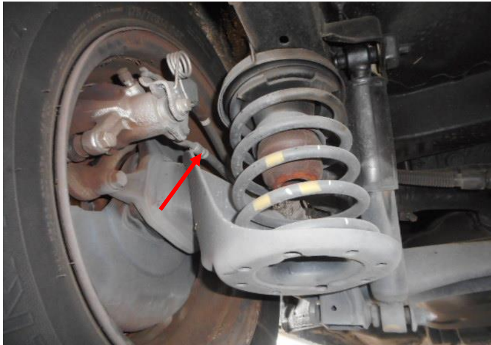
Photo 18 shows the brake hose/pipe (arrowed) at the rear left wheel of the Motor Car. I did not observe any leakage of brake fluid at the time of my inspection of the Motor Car. Static tests of the Motor Car's braking system had indicated that there was no internal leakage of pressure/vacuum. The undercarriage components of the Motor Car were also all found to be intact and without any visible damage.
