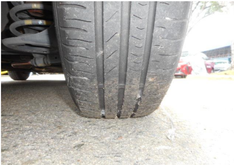
Photo 9 shows the condition of the rear right tyre of the Motor Car, which was observed to be in serviceable condition with remaining tread depth of approximately 4.5mm. The tyre was also observed to be sufficiently inflated for vehicular operation with no tear, cut or burst mark(s).
