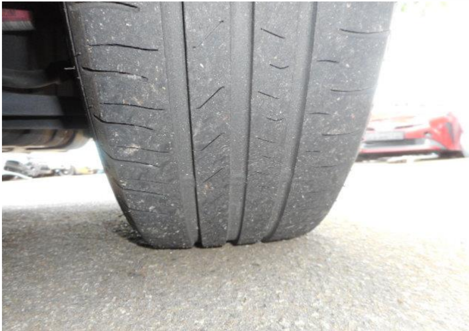
Photo 8 shows the condition of the front right tyre of the Motor Car, which was observed to be in serviceable condition with remaining tread depth of approximately 3.7mm. The tyre was sufficiently inflated for vehicular operation with no tear, cut or burst mark(s) on the outer and the inner sidewalls as well as across the tread. The 4 tyres of the Motor Car were wrapped around standard alloy wheel rims without any damage.
