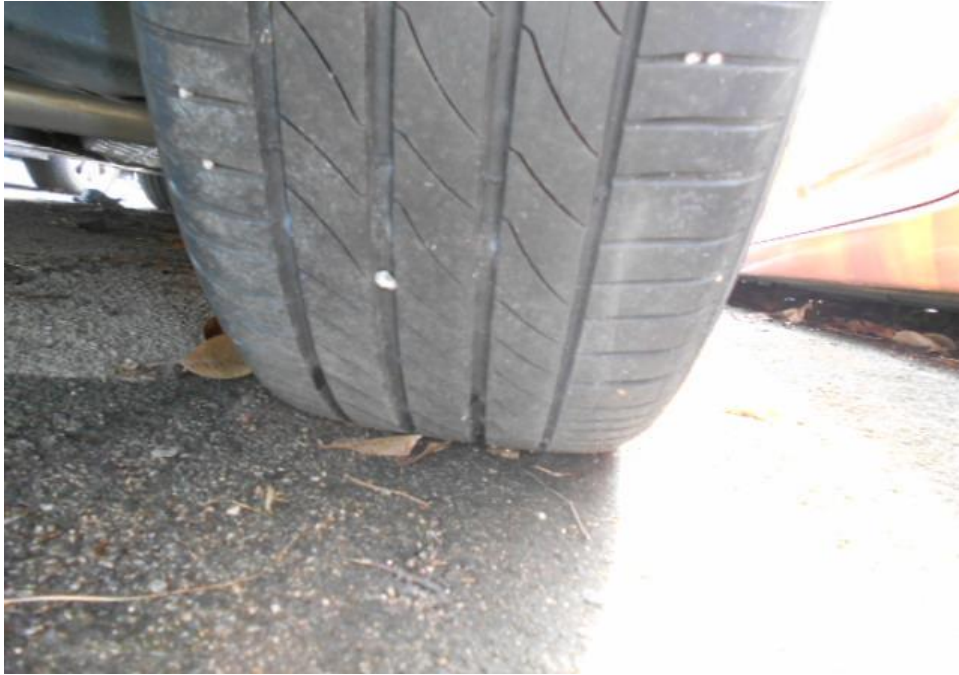
Photo 21 shows the condition of the rear left tyre of the Motor Car, which was observed to be in serviceable condition with remaining tread depth of approximately 4mm. The tyre was also observed to be sufficiently inflated for vehicular operation with no tear, cut or burst mark(s).
