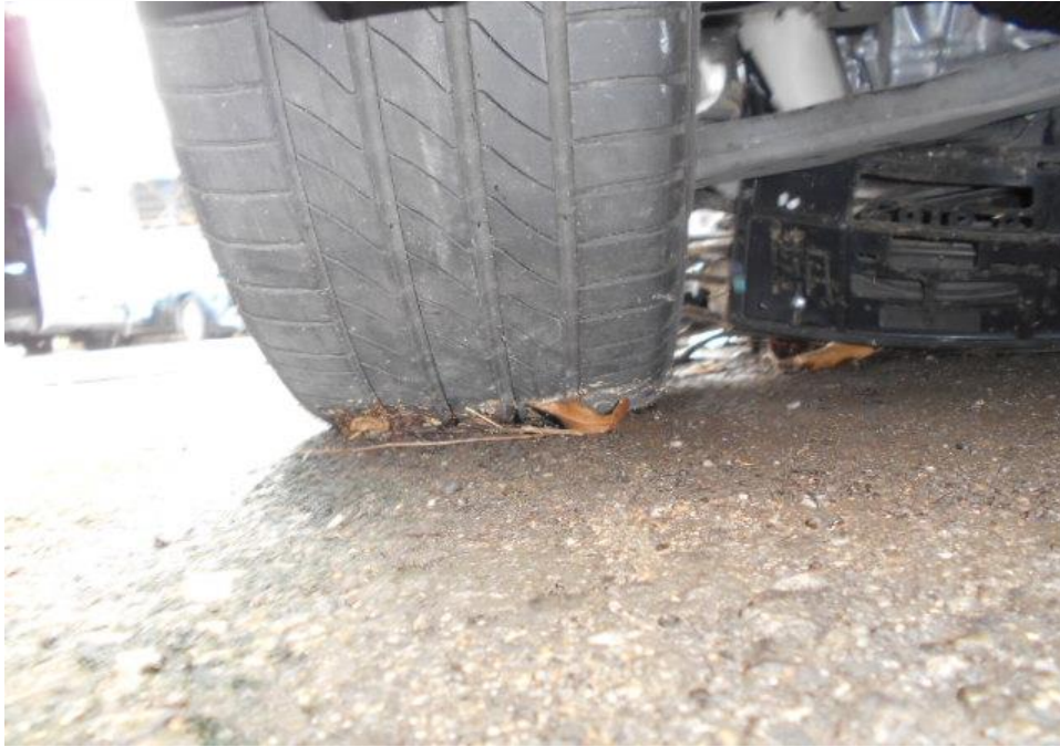
Photo 23 shows the condition of the front left tyre of the Motor Car, which was observed to be in serviceable condition with remaining tread depth of approximately 4.6mm. The tyre was also observed to be sufficiently inflated for vehicular operation with no tear, cut or burst mark(s).
