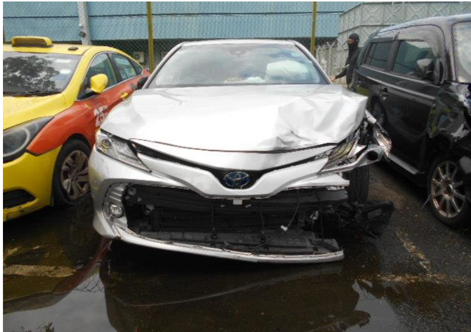
Photo 2 shows a general view of the Motor Car's front body at the time of my inspection. The front portion of the Motor Car was observed to have sustained damage. Its front windscreen, front bumper, front left and right headlamp was amongst the body parts that were damaged as a result of the accident.
