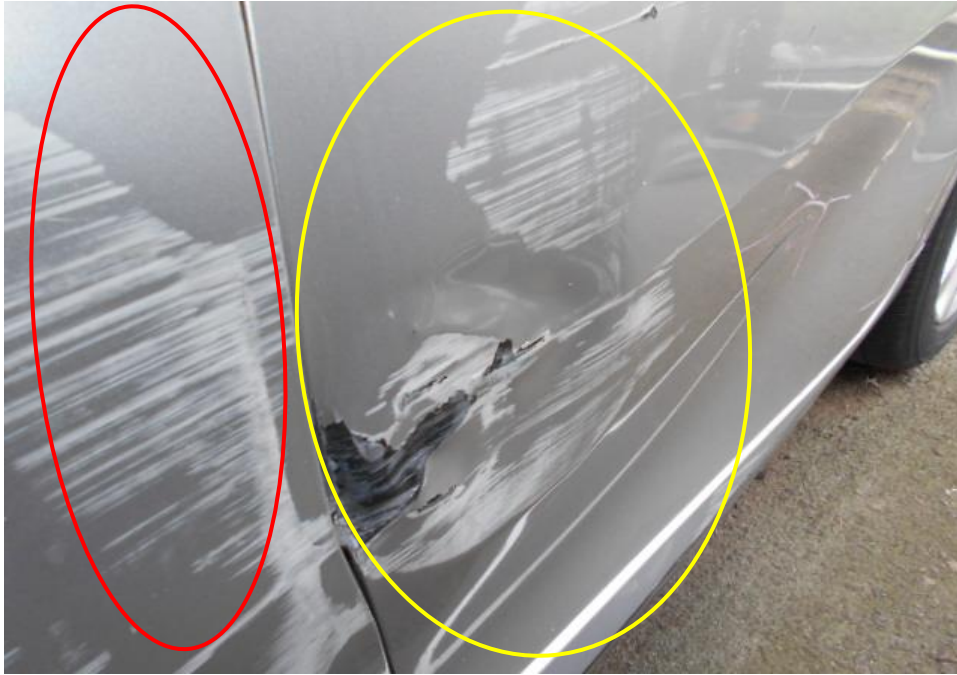
Photo 13 shows a close up view of the Motor Car's left body at the time of my inspection. The Motor Car was observed to have sustained damage at its left, portion. Its left fender (red circle) and left door (yellow circle) was amongst the body parts that were damaged as a result of the accident.
