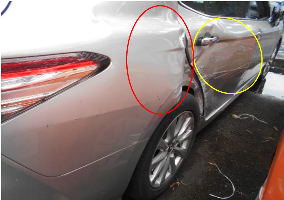
Photo 10 shows a close up view of the Motor Car's right body at the time of my inspection. The Motor Car was observed to have sustained damage at its right, portion. Its right rear quarter panel (red circle) and right door (yellow circle) was amongst the body parts that were damaged as a result of the accident.
