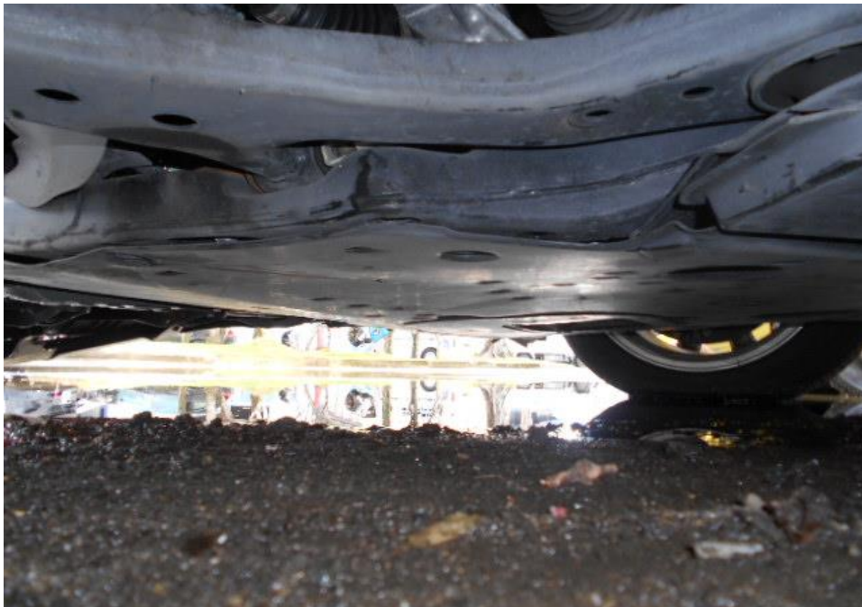
Photo 29 shows the undercarriage of the Motor Car, at the area where the engine housing and transmission housing are located. I did not find any sign(s) or indication(s) of fluid leak and/or fluid stain(s) on the underside of the Motor Car.
