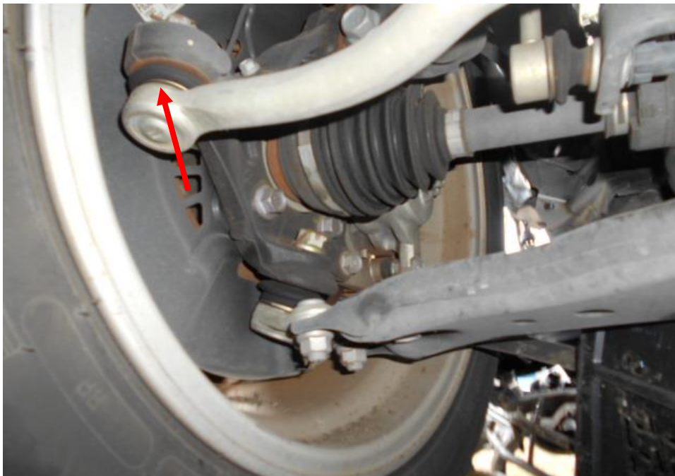
Photo 36 shows the various undercarriage components at the front left wheel of the Motor Car, in particular the steering tie rod (red arrow) was found to be intact. There was also no sign of fluid stain observed on the various undercarriage components at the front left wheel of the Motor Car.
