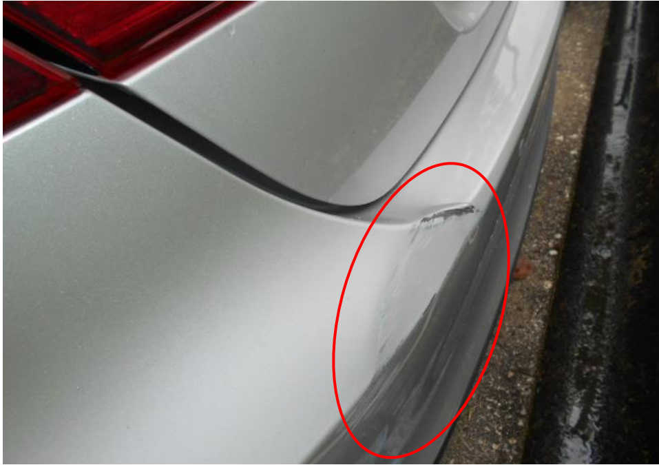
Photo 17 shows a close up view of the Motor Car's rear body at the time of my inspection. The Motor Car was observed to have sustained damage at its rear, portion. Its rear bumper (circled) was amongst the body parts that were damaged as a result of the accident.
