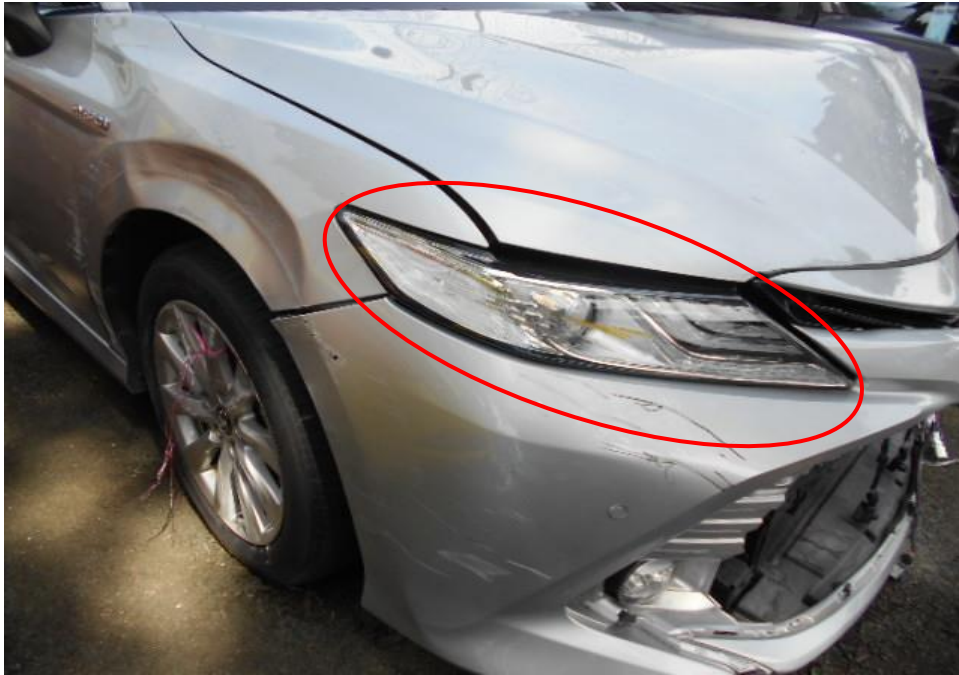
Photo 5 shows the close up view of the Motor Car's front body at the time of my inspection. The Motor Car was observed to have sustained damage at its front portion. Its front right headlamp (circled) was damaged as a result of the accident.
