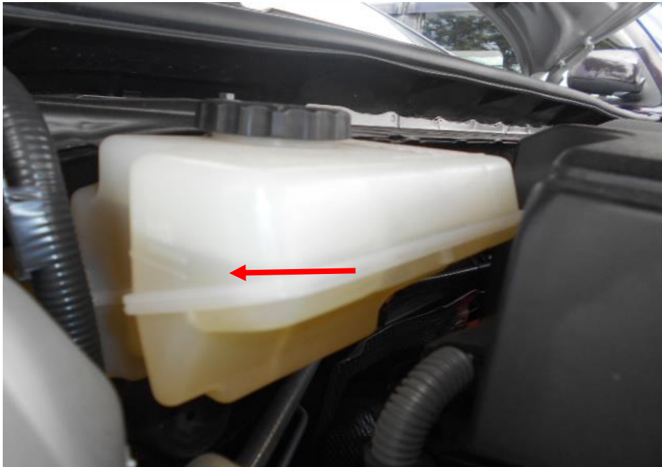
Photo 26 shows the brake fluid reservoir of the Motor Car at the time of my inspection. The brake fluid was observed to be of sufficient level (arrowed) and without any visible contamination.
