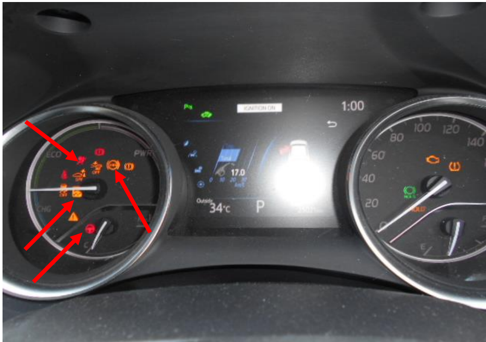
Photo 37 shows the warning light for Anti-Lock Brake System (ABS), Traction Control System (TCS), Electric Power Steering (EPS), and Supplemental Restraint System (SRS) (arrowed) appearing on the instrument panel of the Motor Car during the self-test of its various electronic operating systems when its engine was cranked.
