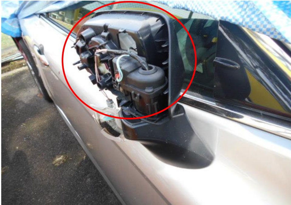
Photo 7 shows a close up view of the Motor Car's right body at the time of my inspection. The Motor Car was observed to have sustained damage at its right, portion. Its right rear view mirror (circled) was amongst the body parts that were damaged as a result of the accident.
