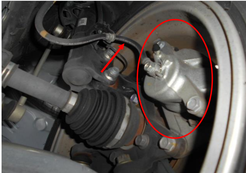
Photo 33 shows the brake hose/pipe (arrowed) at the front left wheel of the Motor Car. No leakage of brake fluid was observed. Visual examination of the various components of the braking system the brake caliper (circled) to be intact and without visible damage.
