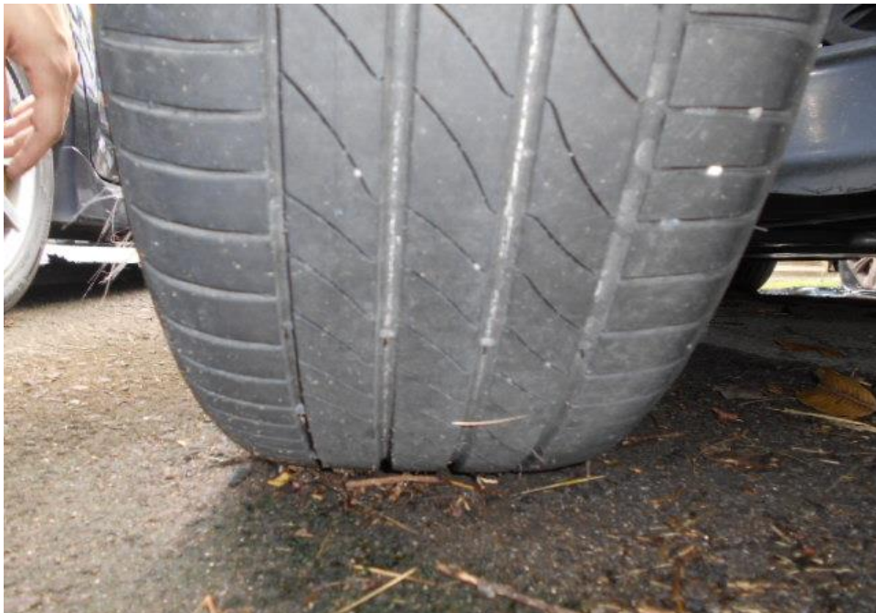
Photo 22 shows the condition of the rear left tyre of the Motor Car, which was observed to be in serviceable condition with remaining tread depth of approximately 4.4mm. The tyre was also observed to be sufficiently inflated for vehicular operation with no tear, cut or burst mark(s).
