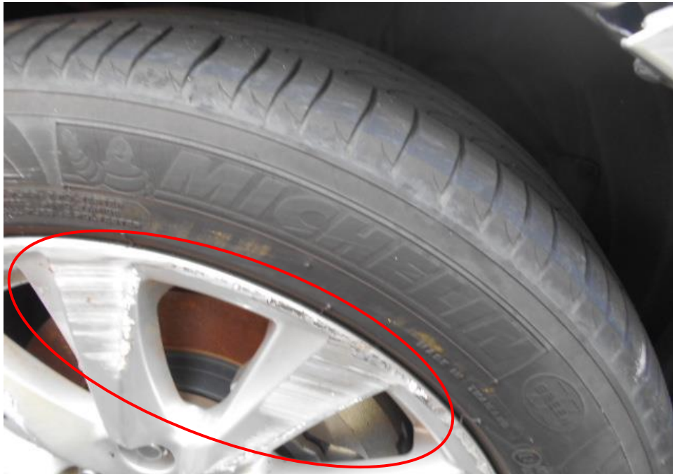
Photo 19 shows the close up condition of the front right wheel rim (circled) of the Motor Car, which was observed to be damaged as a result of the accident.
