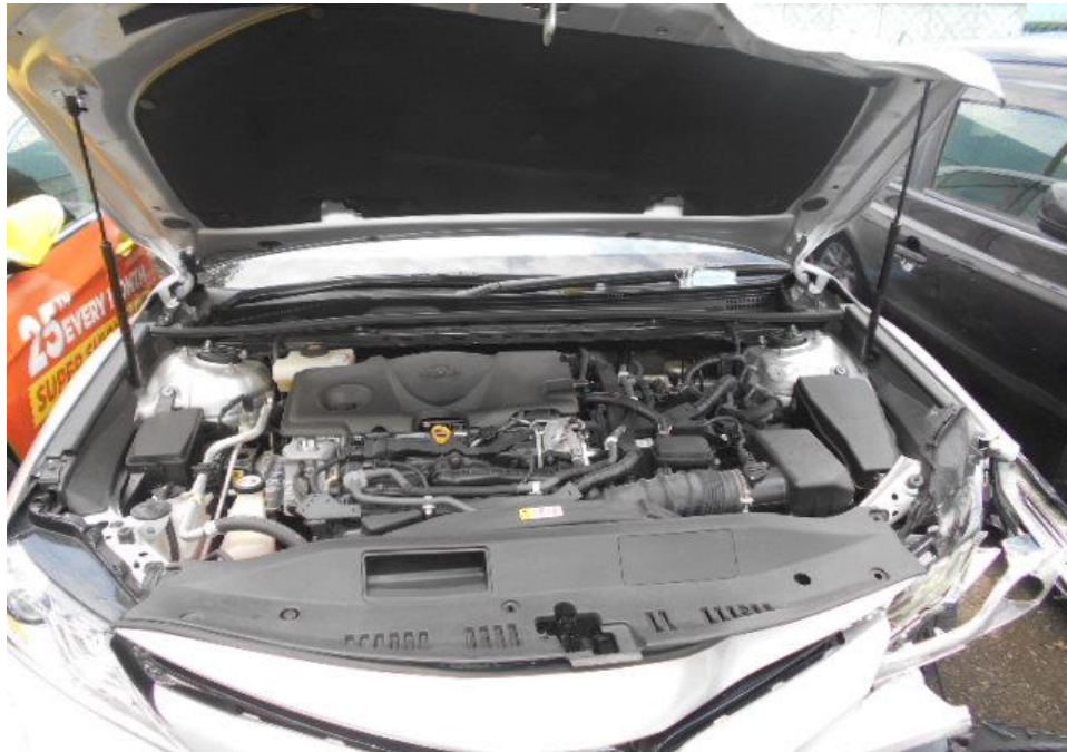
Photo 25 shows a general view of the Motor Car's engine compartment, which was accessed by lifting the front bonnet of the Motor Car. The various parts and components inside the engine compartment were unaffected by the accident. There was also no sign(s) or indication(s) of fresh fluid leakage and/or fluid stain within the engine compartment.
