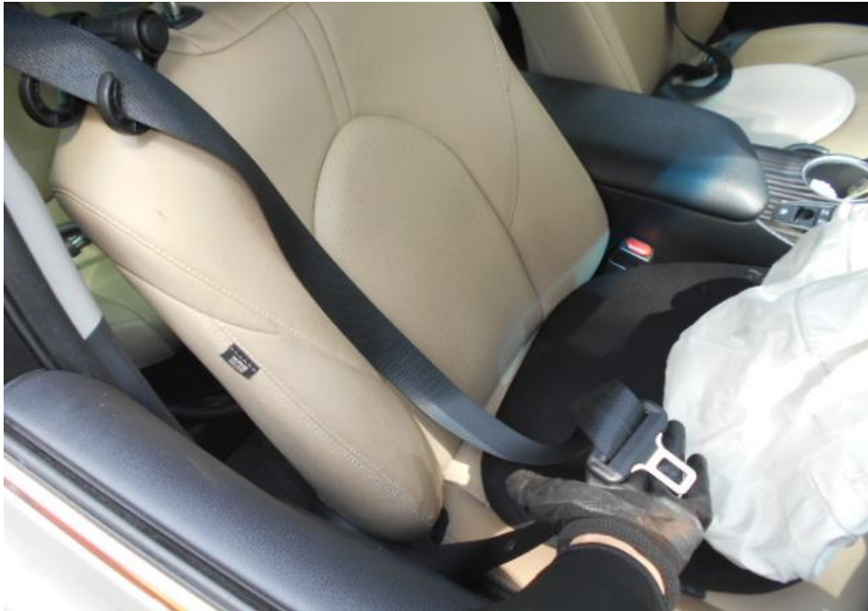
Photo 39 shows that the seat belt on the right seat was worn at the material time of accident as the safety pre-tensioners was activated at the moment of impact and caused the seat belt to be locked into the last position.
