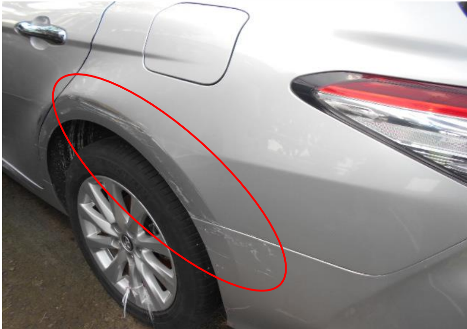
Photo 15 shows a close up view of the Motor Car's rear body at the time of my inspection. The Motor Car was observed to have sustained damage at its rear, portion. Its rear left quarter panel (circled) was amongst the body parts that were damaged as a result of the accident.
