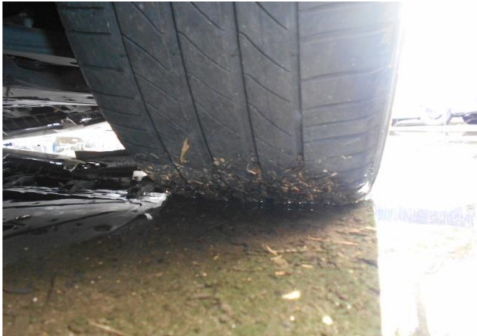
Photo 20 shows the condition of the front right tyre of the Motor Car, which was observed to be in serviceable condition with remaining tread depth of approximately 4.6mm. The tyre was also observed to be sufficiently inflated for vehicular operation with no tear, cut or burst mark(s).
