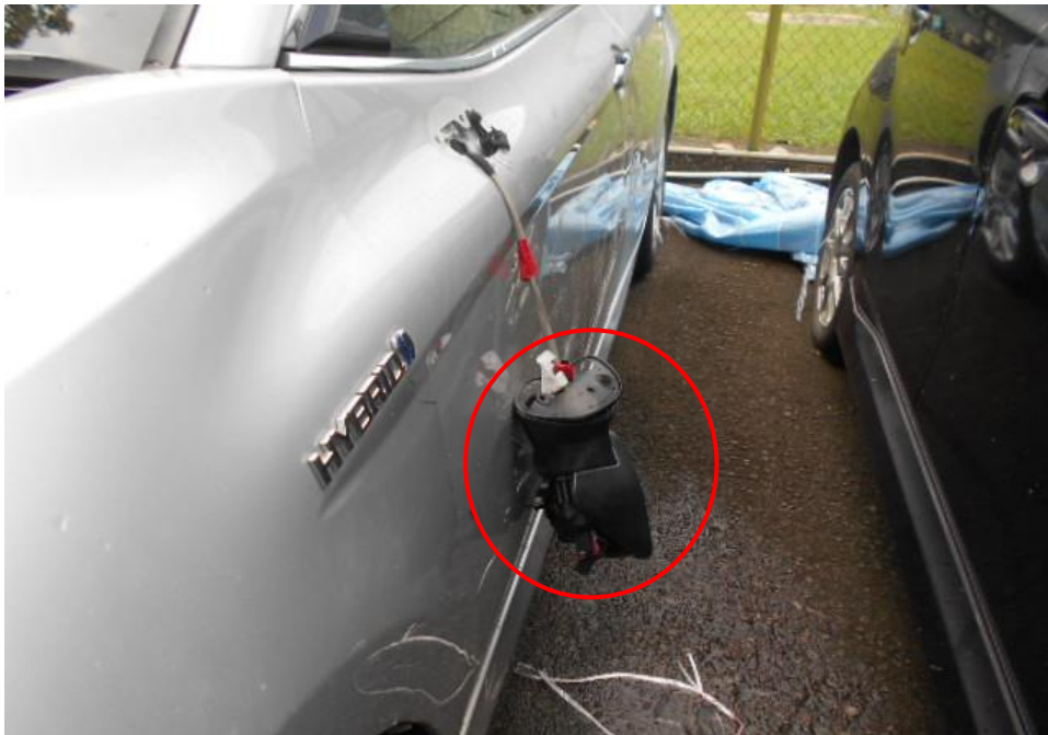
Photo 12 shows a close up view of the Motor Car's left body at the time of my inspection. The Motor Car was observed to have sustained damage at its right, portion. Its left rear view mirror (circled) was amongst the body parts that were damaged as a result of the accident.
