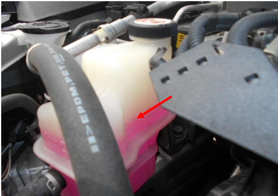
Photo 27 shows the coolant reservoir of the Motor Car at the time of my inspection. The coolant was observed to be sufficient (arrowed) and without any visible contamination.
