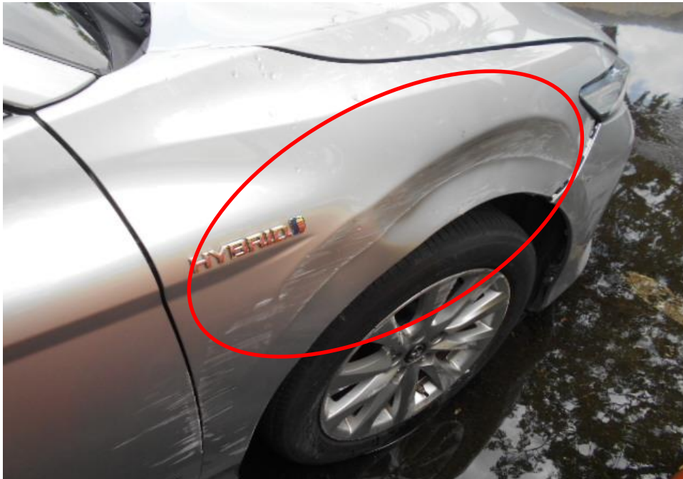
Photo 8 shows a close up view of the Motor Car's right body at the time of my inspection. The Motor Car was observed to have sustained damage at its right, portion. Its right front fender (circled) was amongst the body parts that were damaged as a result of the accident.
