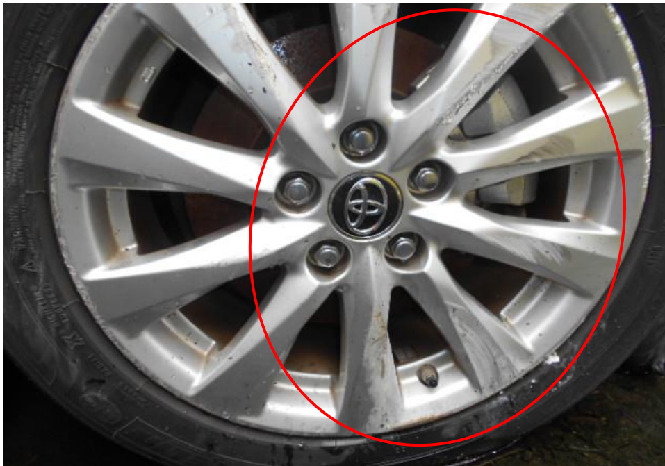
Photo 18 shows the general view of the front right wheel rim (circled) of the Motor Car, which was observed to be damaged as a result of the accident.
