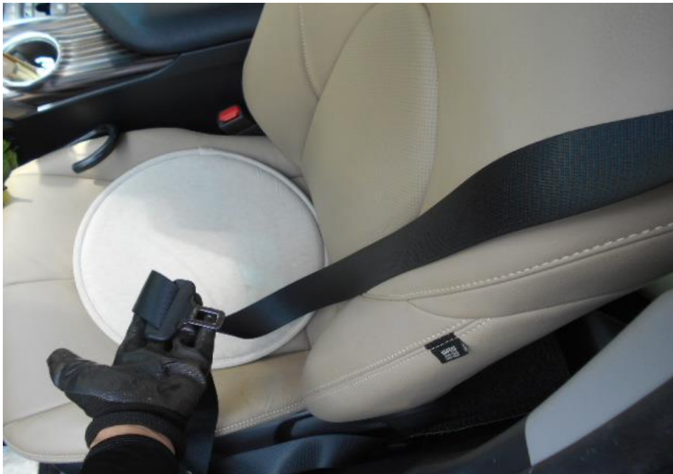
Photo 40 shows that the seat belt on the left seat was worn at the material time of accident as the safety pre-tensioners was activated at the moment of impact and caused the seat belt to be locked into the last position.
