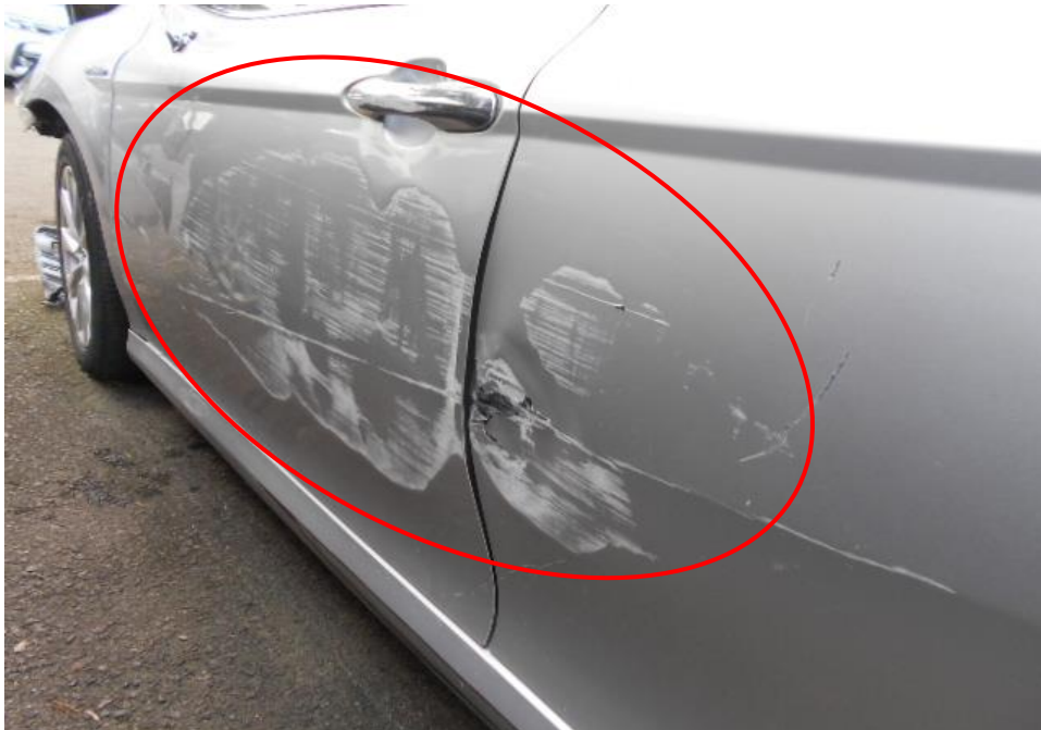
Photo 14 shows a close up view of the Motor Car's left body at the time of my inspection. The Motor Car was observed to have sustained damage at its left, portion. Its left doors (circled) was amongst the body parts that were damaged as a result of the accident.
