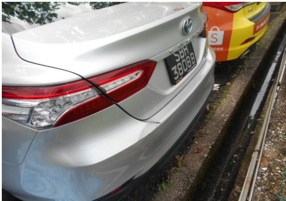
Photo 16 shows the general view of the Motor Car's rear body at the time of my inspection. The Motor Car was observed to have sustained damage at its rear, portion. Its rear bumper was amongst the body parts that were damaged as a result of the accident.
