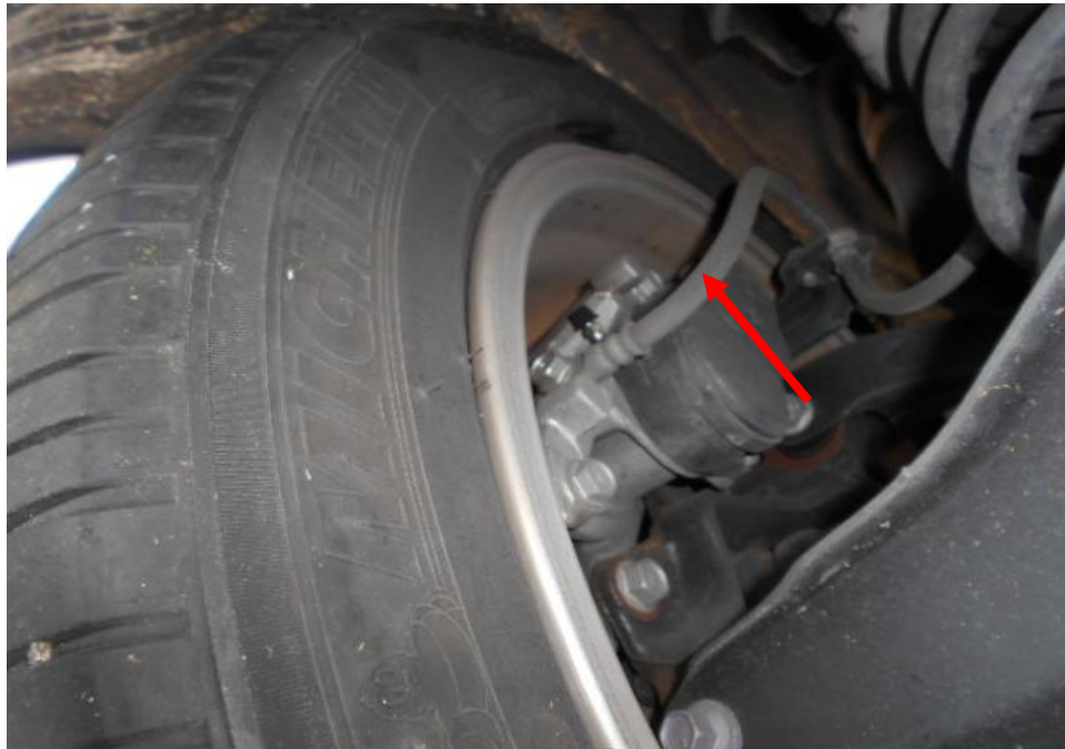
Photo 31 shows the brake hose/pipe (arrowed) at the rear left wheel of the Motor Car. No leakage of brake fluid was observed. Visual examination of the various components of the braking system like the brake caliper to be intact and without visible damage.
