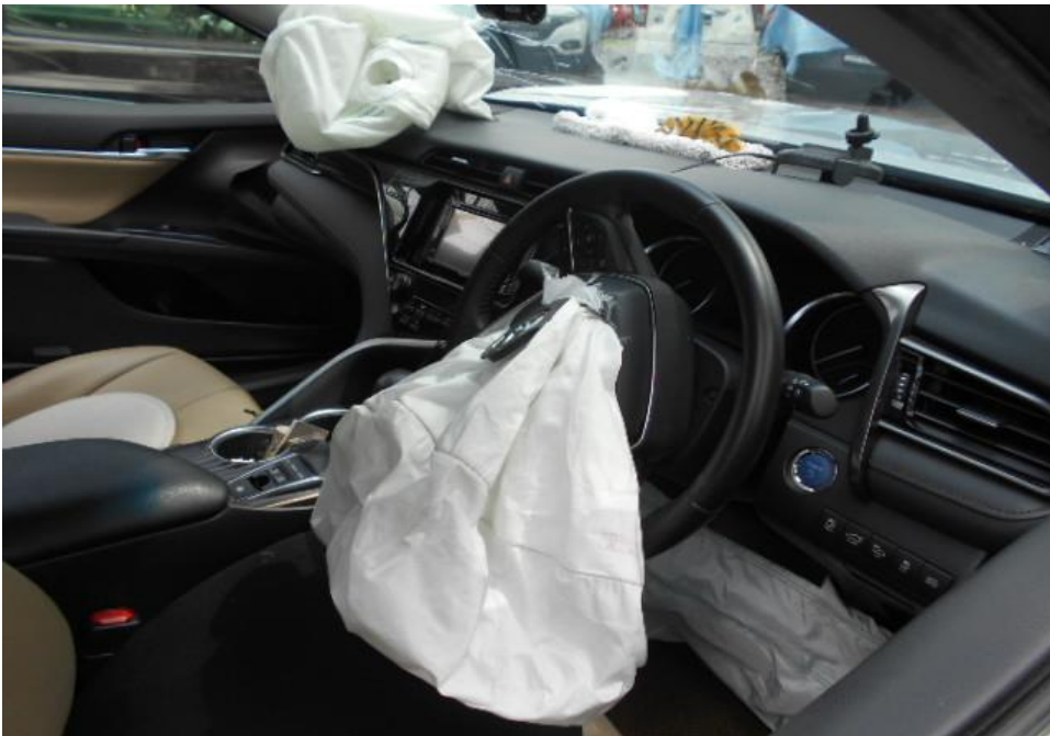
Photo 24 shows the deployment of the Supplemental Restraint System (SRS) airbag in the Motor Car as a result of the accident.
