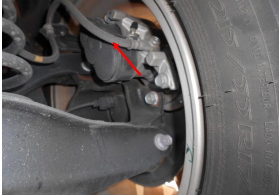
Photo 30 shows the brake hose/pipe (arrowed) at the rear right wheel of the Motor Car. No leakage of brake fluid was observed. Visual examination of the various components of the braking system like the brake caliper to be intact and without visible damage.
