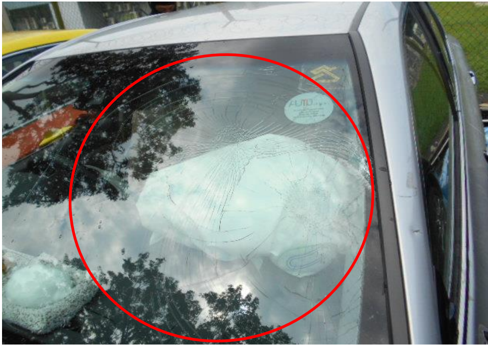
Photo 3 shows a close up view of the Motor Car's front body at the time of my inspection. The Motor Car was observed to have sustained damage at its front portion. Its front windscreen (circled) was damaged as a result of the accident.
