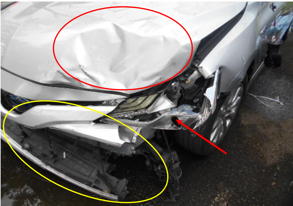
Photo 4 shows the close up view of the Motor Car's front body at the time of my inspection. The Motor Car was observed to have sustained damage at its front portion. Its front bumper (yellow circle), front bonnet (red circle) and front left headlamp (arrowed) was damaged as a result of the accident.
