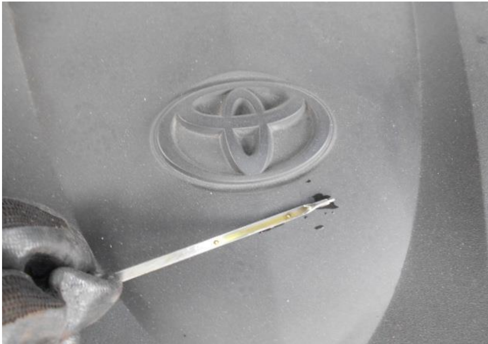
Photo 28 shows the engine oil dipstick of the Motor Car at the time of my inspection. The engine oil was observed to be sufficient (arrowed) and without any visible contamination.
