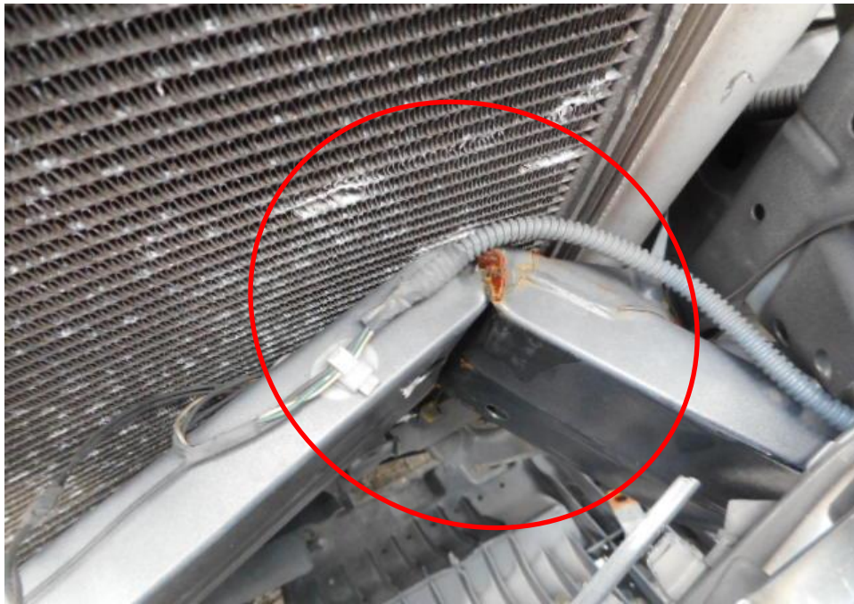
Photo 14 shows the close up view of the engine compartment of the Motor Car at the time of my inspection. The engine radiator (circled) was observed to be damaged and as a result of the accident.
