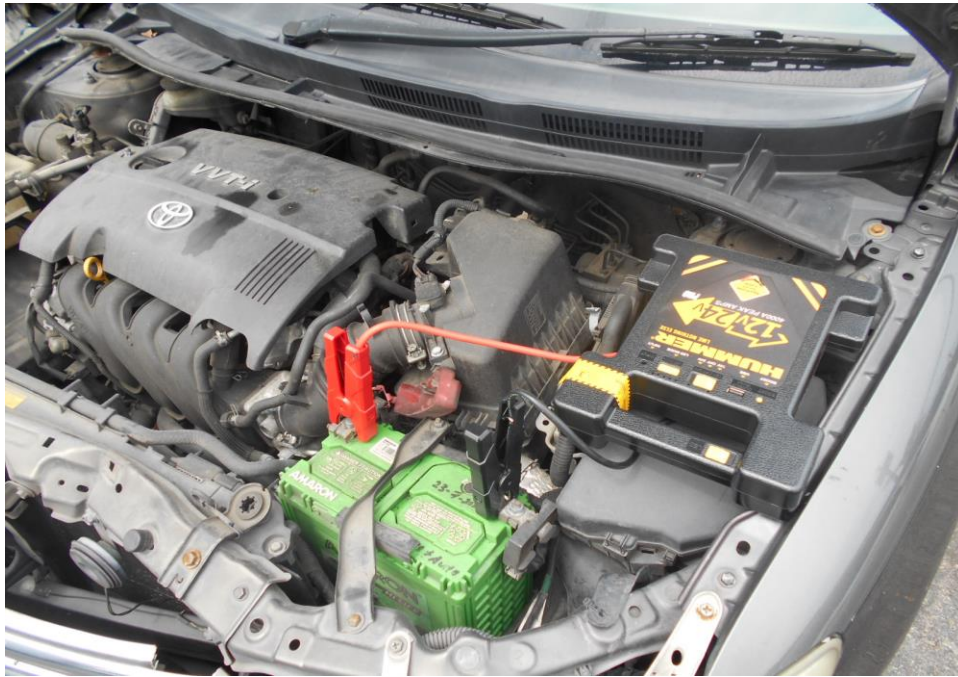
Photo 25 shows the jumpstarting of the Motor Car using a jump starter. The engine of the Motor Car was unable to be started up despite multiple attempts in jumpstarting it.
