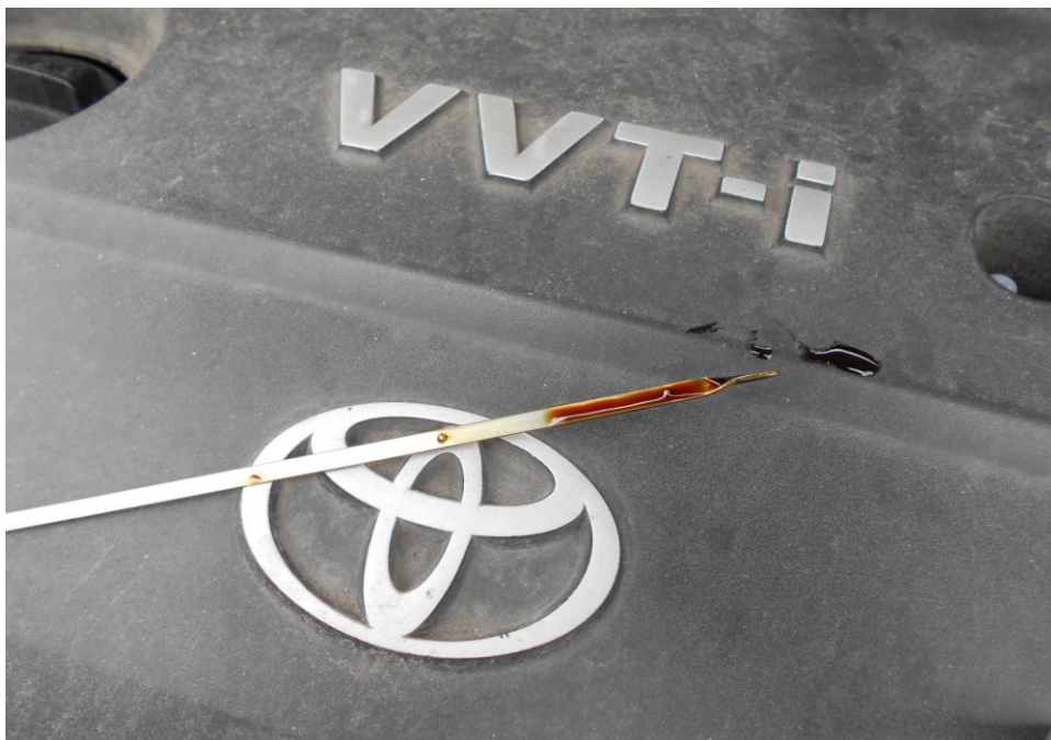
Photo 17 shows the engine oil level dipstick of the Motor Car at the time of my inspection. The engine oil was observed to be of sufficient level and without any visible contamination.
