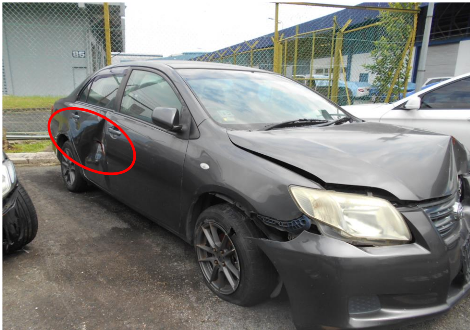
Photo 4 shows a general view of the Motor Car's right portion at the time of my inspection. The right rear door (circled) of the Motor Car was observed to have been damaged as a result of the accident.
