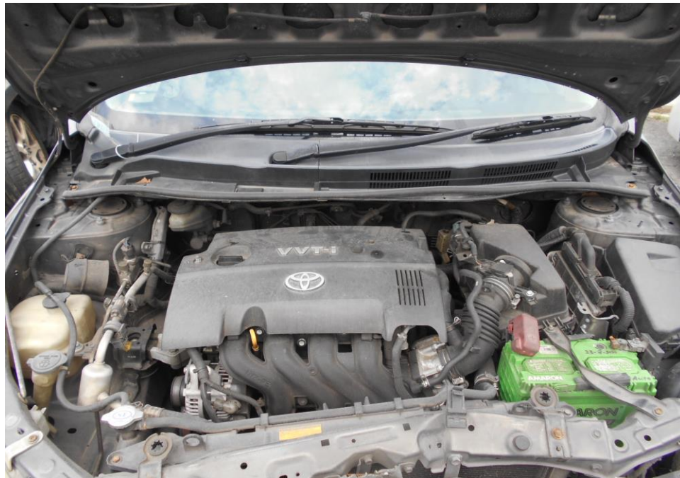
Photo 13 shows a general view of the Motor Car's engine compartment, which was accessed by lifting the front bonnet of the Motor Car. The various parts and components inside the engine compartment were unaffected by the accident. There was also no sign(s) or indication(s) of fresh fluid leakage and/or fluid stain within the engine compartment.
