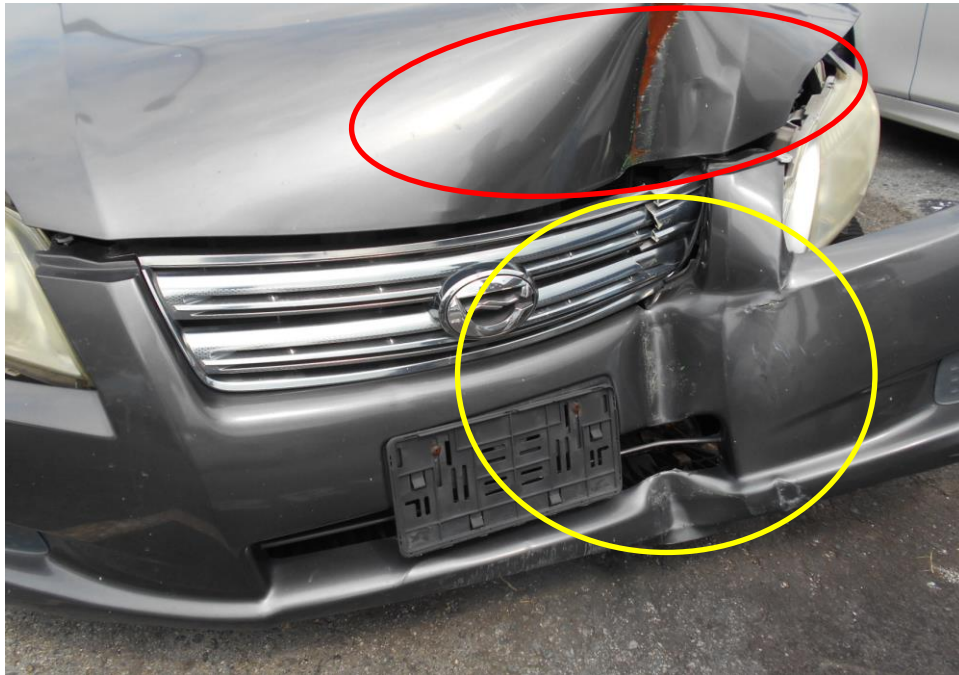
Photo 3 shows the close up view of the Motor Car's front body at the time of my inspection. The Motor car was observed to have sustained damage at its front portion. Its front bonnet (red circle), its front grille and bumper (yellow circle) was damaged as a result of the accident.
