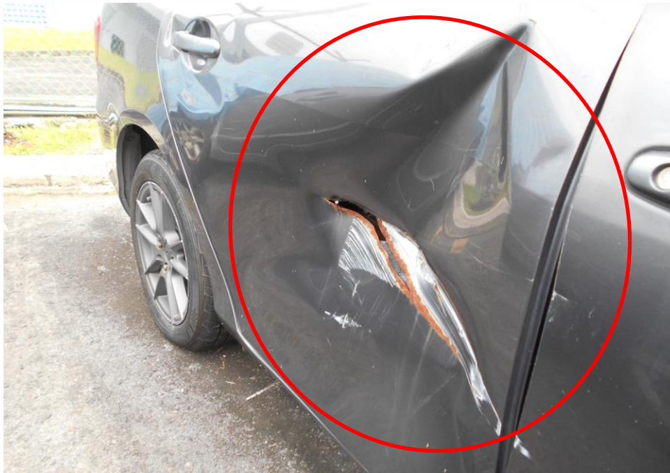
Photo 5 shows the close up view of the Motor Car's right portion at the time of my inspection. The right rear door (circled) of the Motor Car was observed to have been damaged as a result of the accident.
