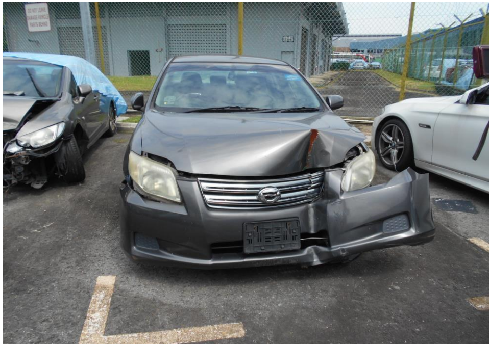
Photo 2 shows a general view of the Motor Car's front body at the time of my inspection. The Motor Car was observed to have sustained damage at its front portion. Its front bonnet, front bumper as well as its front grille were amongst the body parts that were damaged as a result of the accident.
