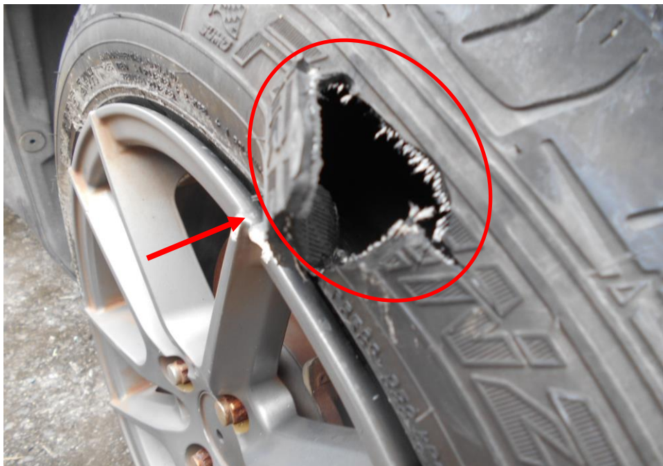
Photo 8 shows the close up condition of the front right tyre and wheel rim of the Motor Car, which was observed to be cut and deflated (circled) and the wheel rim (arrowed) was damaged as a result of the accident with remaining tread depth of approximately 5.1mm
