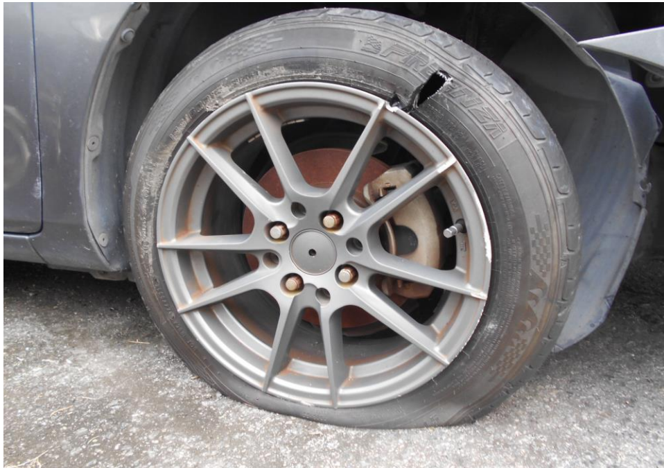
Photo 7 shows the general condition of the front right tyre and wheel rim of the Motor Car, which was observed to be cut and deflated and the wheel rim was damaged as a result of the accident with remaining tread depth of approximately 5.1mm.
