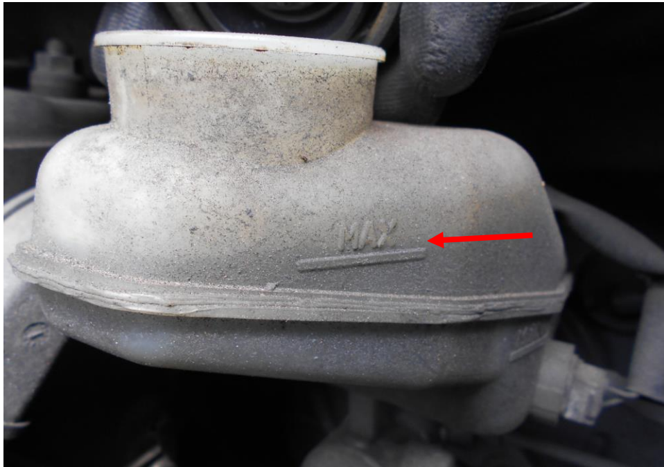
Photo 16 shows the brake fluid reservoir of the Motor Car at the time of my inspection. The coolant was observed to be of sufficient level (arrowed) without any visible contamination.
