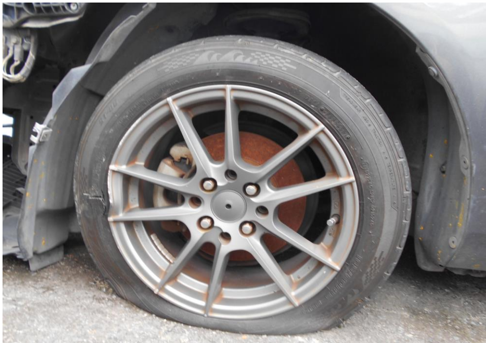
Photo 11 shows the general condition of the front left tyre and wheel rim of the Motor Car, which was observed to be cut and deflated and the wheel rim was damaged as a result of the accident with remaining tread depth of approximately 4.6mm.
