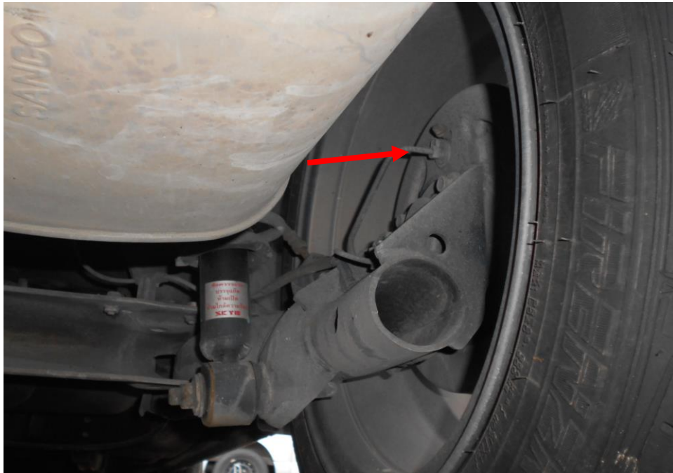
Photo 23 shows the brake hose/pipe (arrowed) at the rear right wheel of the Motor Car. No leakage of brake fluid was observed. Visual examination of the various components of the braking system like the drum brake, brake booster, brake pedal etc. had revealed all to be intact and without visible damage.
