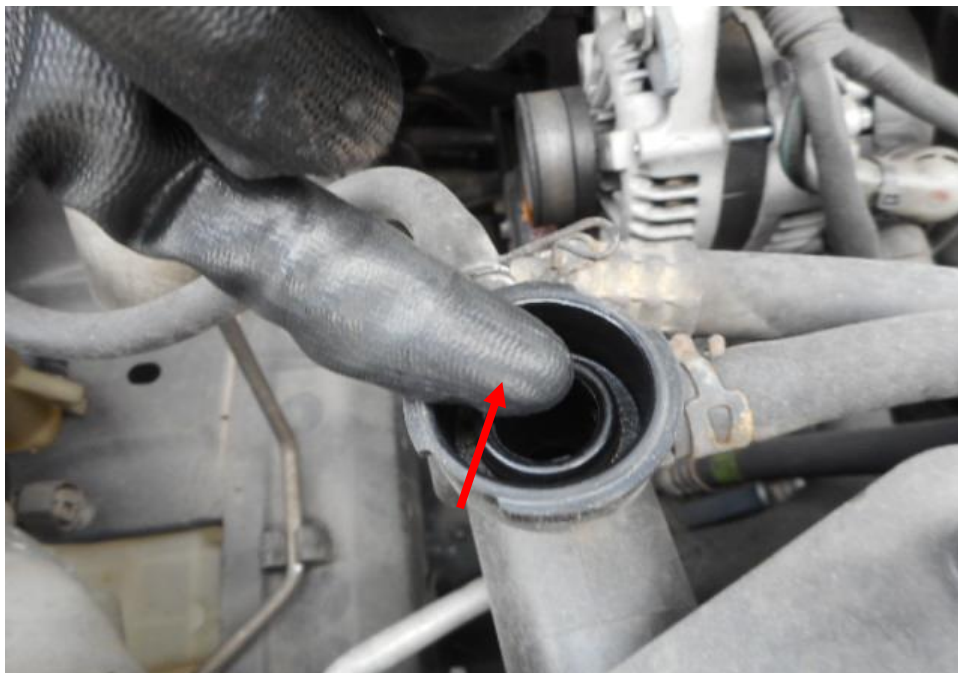
Photo 15 shows the engine coolant radiator cap of the Motor Car at the time of my inspection. The coolant was observed to be of insufficient level (arrowed) as a result of the accident.
