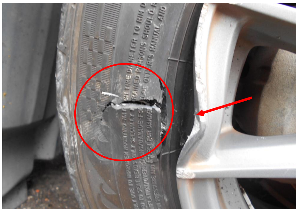
Photo 12 shows the close up condition of the front left tyre and wheel rim of the Motor Car, which was observed to be cut and deflated (circled) and the wheel rim (arrowed) was damaged as a result of the accident with remaining tread depth of approximately 4.6mm
