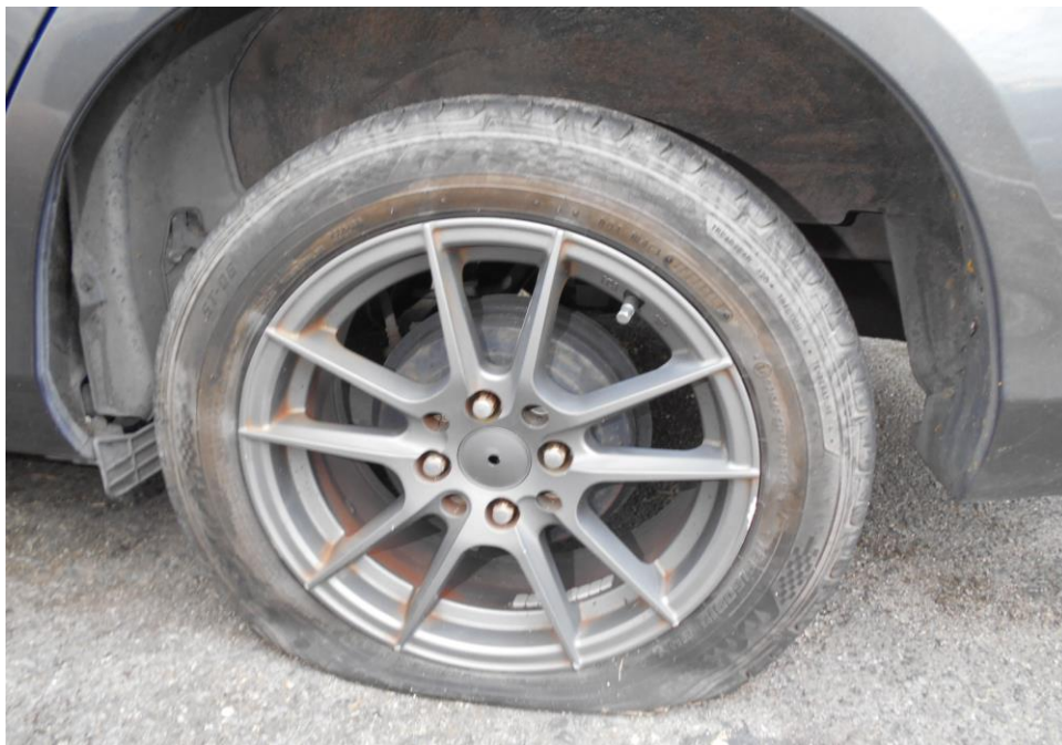
Photo 10 shows the general condition of the rear left tyre and wheel rim of the Motor Car, which was observed to be deflated as a result of the accident with remaining tread depth of approximately 5.9mm.
