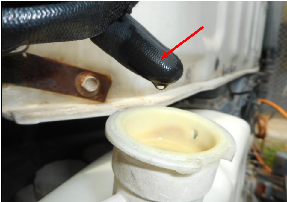
Photo 14 shows the engine coolant reservoir of the Tipper Truck at the time of my inspection. The engine coolant was observed to be of sufficient level (arrowed) and without any visible contamination.
