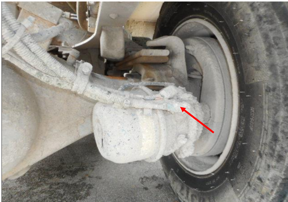
Photo 18 shows the brake pipe (arrowed) at the rear right wheel of the Tipper Truck. I did not observe any leakage of brake fluid at the time of my inspection of the Tipper Truck. My static tests of the Tipper Truck's braking system, along with my visual examination of the various mechanical components in the braking system, had indicated that there was no internal leakage of pressure/vacuum. Hence the braking system of the Tipper Truck was likely to be in serviceable condition at the material time of accident.
