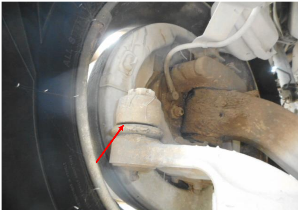
Photo 24 shows the various undercarriage components at the front left wheel of the Tipper Truck, in particular the steering tie rod end (arrowed). The various undercarriage components of the Tipper Truck were all found to be intact without any visible damage. There was also no sign of fluid stain(s) observed on the various undercarriage components.
