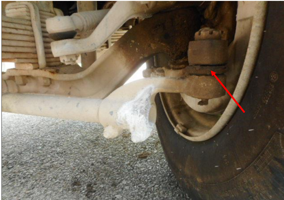
Photo 23 shows the various undercarriage components at the front right wheel of the Tipper Truck, in particular the steering tie rod end (arrowed). The various steering components were all found to be intact, suggesting that the steering system of the Tipper Truck was likely to be in serviceable condition at the material time of accident. There was also no sign of fluid stain(s) observed on the various undercarriage components.
