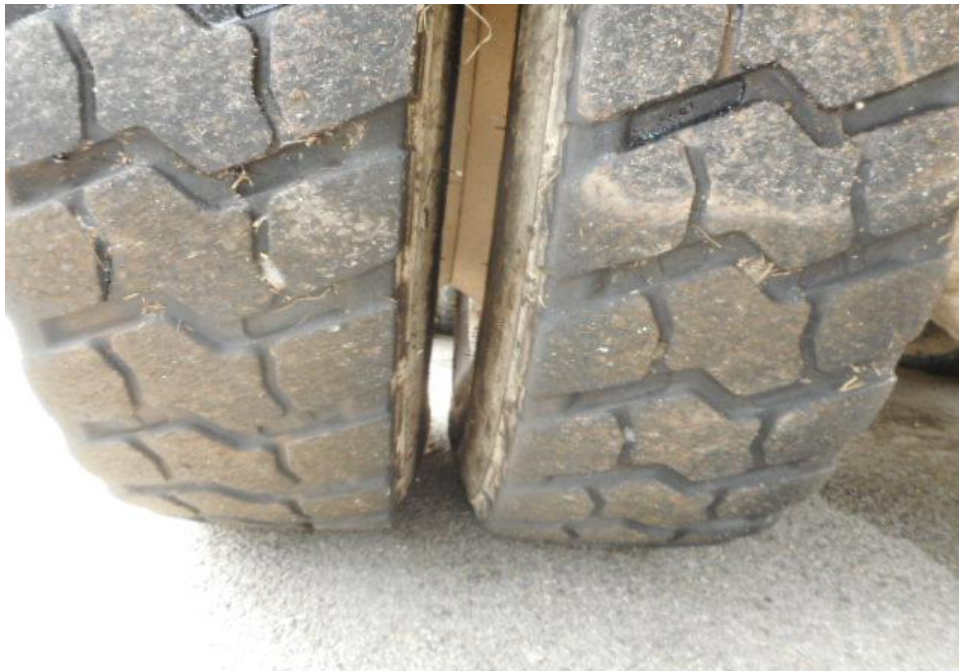
Photo 10 shows the condition of the rear left tyres of the Tipper Truck, which was observed to be in serviceable condition with remaining tread depth of approximately 7.5mm. The tyres, which were wrapped around standard steel wheel rim, were also observed to be sufficiently inflated for vehicular operation. There was also no damage found on all 12 steel wheel rims of the Tipper Truck.
