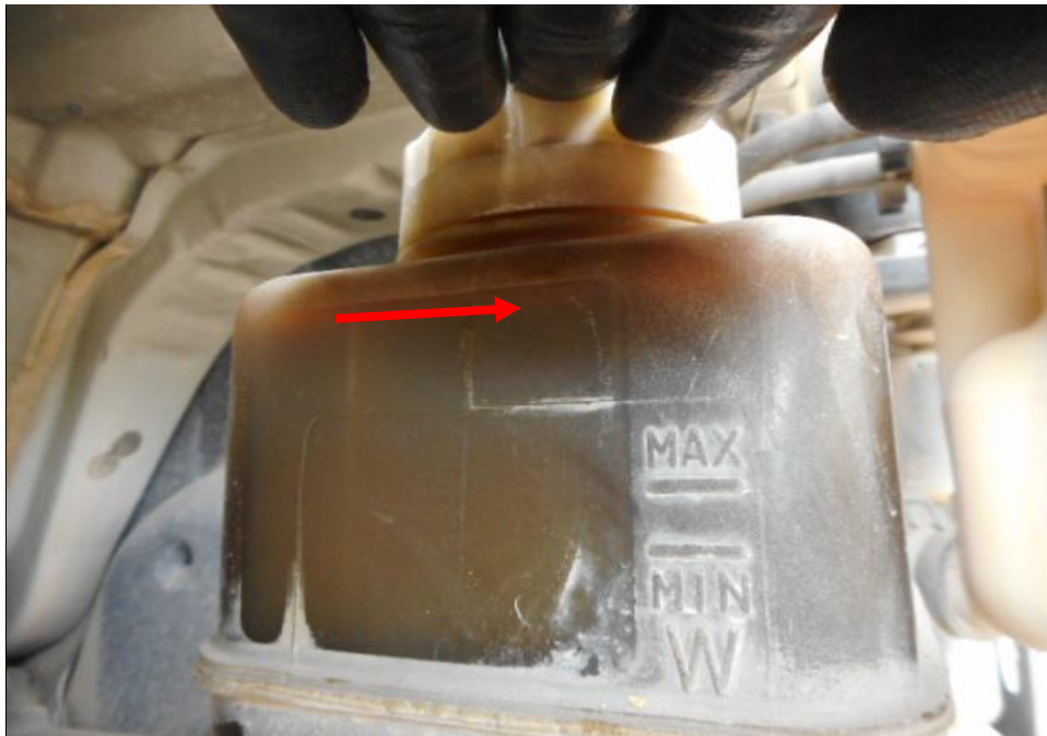
Photo 15 shows the power steering fluid reservoir of the Tipper Truck at the time of my inspection. The power steering fluid was observed to be of sufficient level (arrowed) and without any visible contamination.
