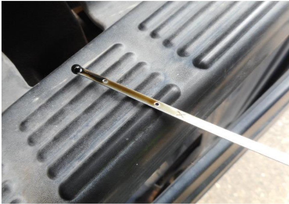
Photo 16 shows the engine oil dip stick of the Tipper Truck at the time of my inspection. The engine oil was observed to be of insufficient level at the time of our inspection.
