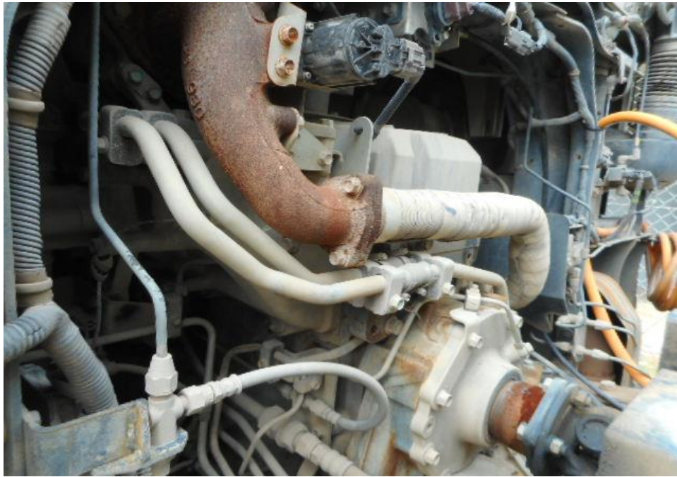
Photo 12 shows a general view of the Tipper Truck's engine compartment, which was accessed by lifting the front cabin of the Tipper Truck. The various parts and components inside the engine compartment were unaffected by the accident. There was also no sign(s) or indication(s) of fresh fluid leakage and/or fluid stain within the engine compartment
