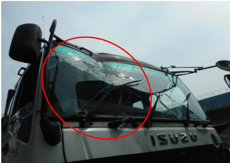
Photo 3 shows a general view of the front body of the Tipper Truck at the time of my inspection. The Tipper Truck was observed to sustain damaged on its front portion. Its front windscreen (circled) was damaged at the time of my inspection.
