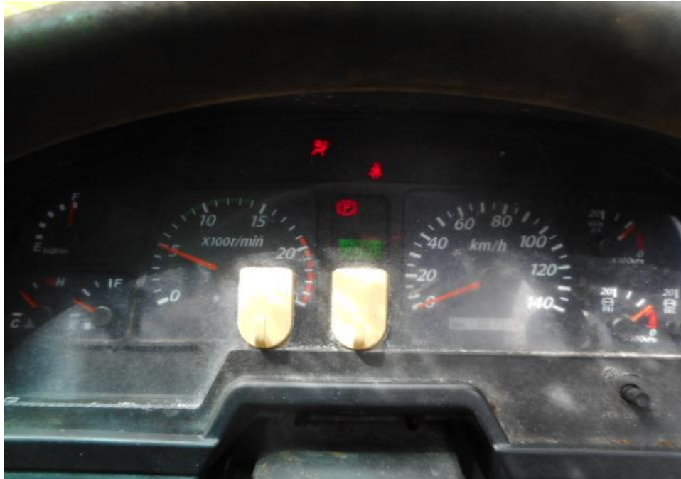
Photo 28 shows no warning lights illuminated on the instrument panel of the Motor Lorry after the engine was cranked. This would suggest that there was no abnormality to the electronic operating system of the Motor Lorry, like the ABS and etc.
