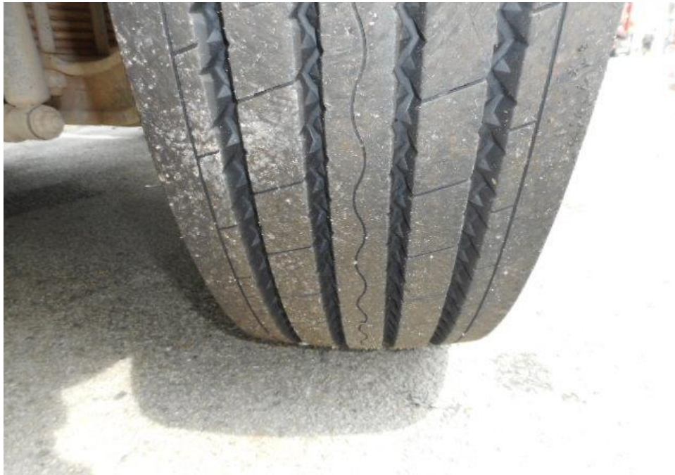
Photo 11 shows the condition of the front left tyres of the Tipper Truck, which were observed to be in serviceable condition with remaining tread depth of approximately 11.3mm. There was also no tear, cut or burst mark(s) on the outer and the inner sidewalls as well as across the tread of the 12 tyres that were fitted on the Tipper Truck.
