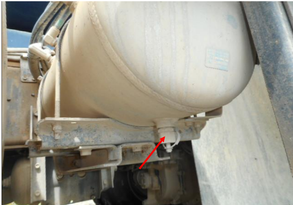
Photo 22 shows the air brake cylinders (arrowed) at the undercarriage of the Tipper Truck. I did not observe any leakage of air brake fluid at the time of my inspection of the Tipper Truck. My static tests of the Tipper Truck's braking system, along with my visual examination of the various mechanical components in the braking system had indicated that there was no internal leakage of pressure/vacuum. Hence the braking system of the Tipper Truck was likely to be in serviceable condition at the material time of accident.
