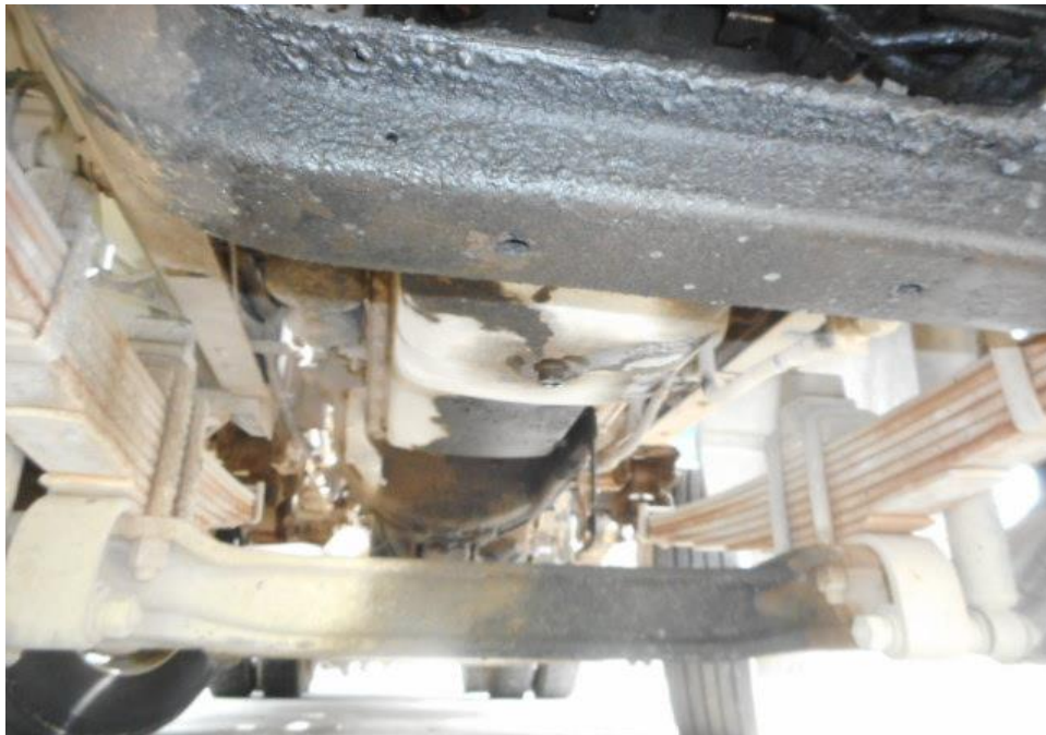
Photo 17 shows the undercarriage of the Tipper Truck, at the area where the engine housing located. I observed old fluid stains on the underside of the Tipper Truck.
