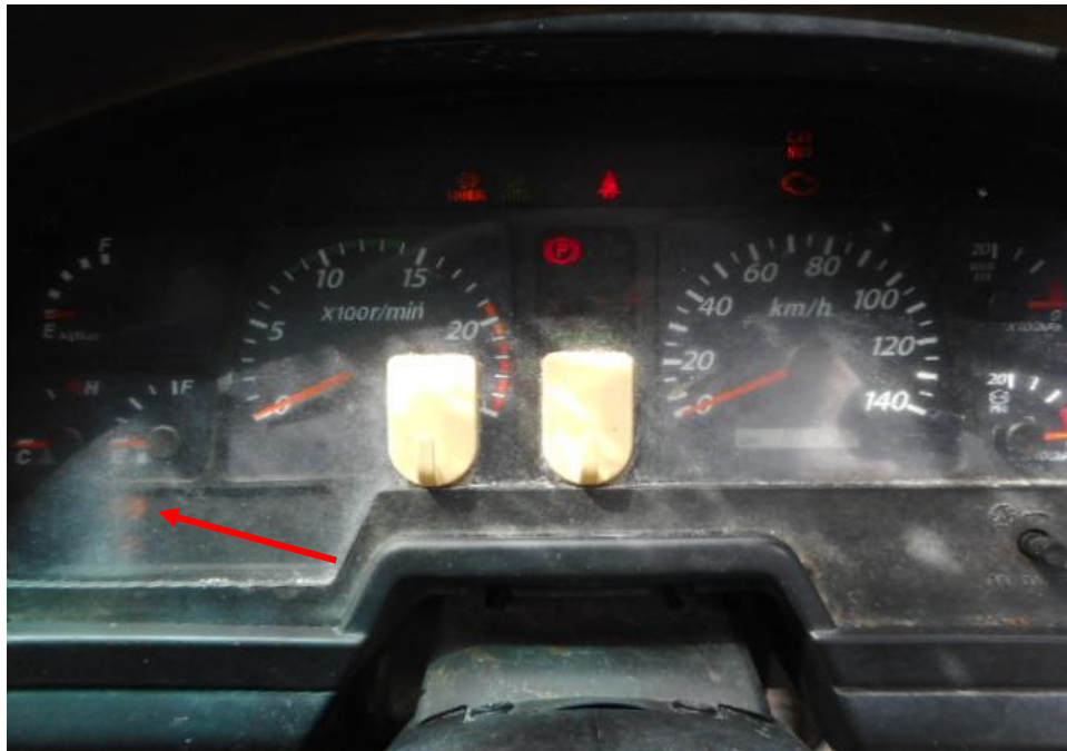
Photo 27 shows the warning light for Anti-lock brake system (ABS) (arrowed) appearing on the instrument panel of the Tipper Truck during the self-test of its various electronic operating systems when its engine was cranked.
