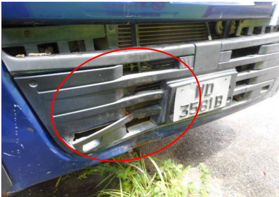
Photo 4 shows a general view of the front body of the Tipper Truck at the time of my inspection. The Tipper Truck was observed to sustain damaged on its front portion. Its front bumper (circled) was damaged at the time of my inspection.
