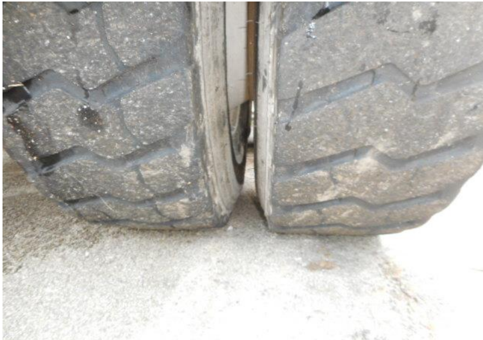
Photo 9 shows the condition of the rear right tyres of the Tipper Truck, which was observed to be in serviceable condition with remaining tread depth of approximately 6mm. The tyre, which was wrapped around standard steel wheel rim, was also observed to be sufficiently inflated for vehicular operation.
