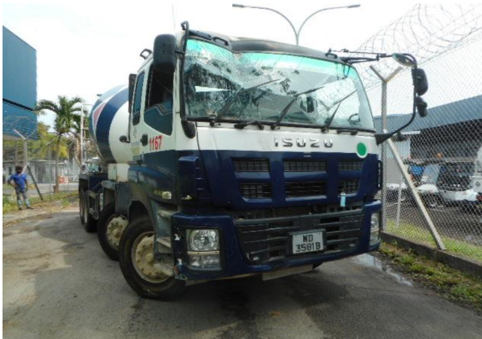
Photo 26 shows the front left wheel of the Tipper Truck turned to its full left. During my steering system test, I did not experience any abnormal free play and/or resistance when I had turned the steering wheel towards full left and full right. This would suggest that the steering system of the Tipper Truck was likely to be in serviceable condition at the material time of accident.
