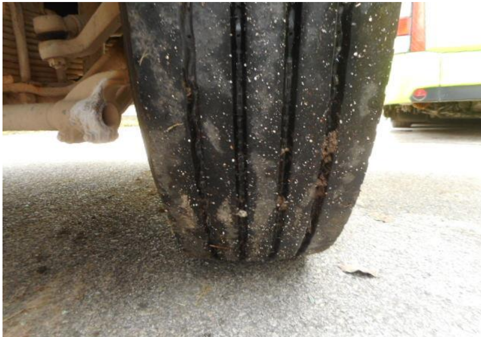
Photo 8 shows the condition of the front right tyre of the Tipper Truck, which was observed to be in serviceable condition with remaining tread depth of approximately 10.3mm. The tyre, which was wrapped around standard steel wheel rim, was also observed to be sufficiently inflated for vehicular operation. There was no tear, cut or burst mark(s) on the outer and the inner sidewalls as well as across the tread of the 12 tyres that were fitted on the Tipper Truck.
