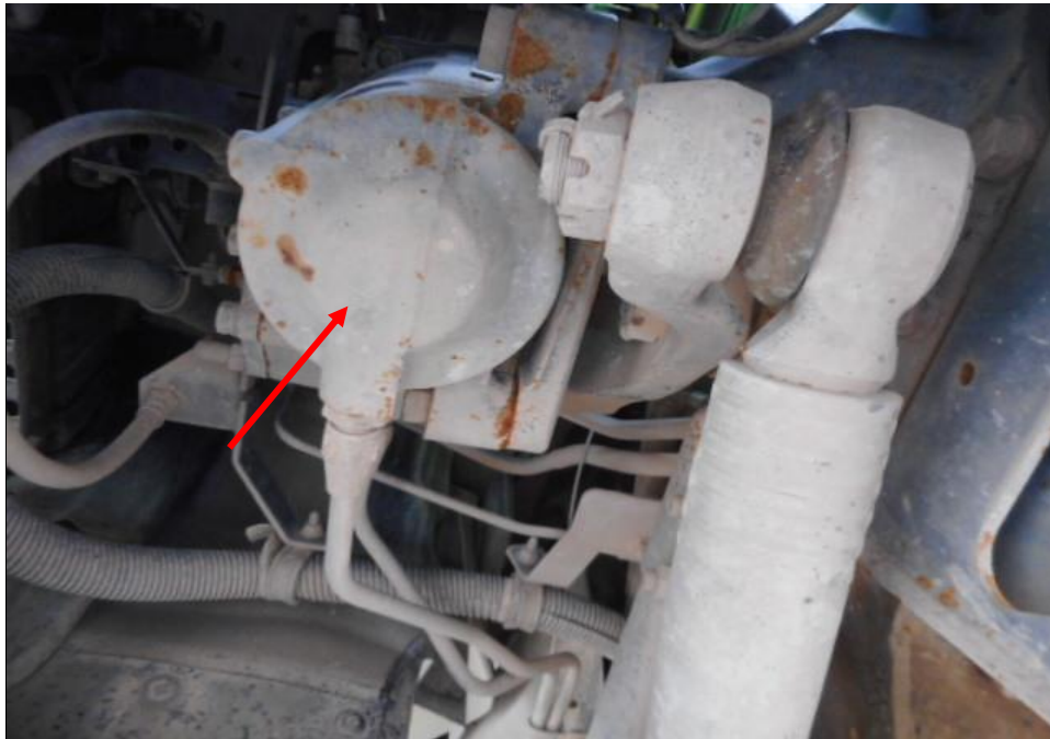
Photo 25 shows the steering box component (arrowed) at the undercarriage of the Tipper Truck was found to be intact without any visible damage. There was also no sign of fluid stain(s) observed on the various undercarriage components.
