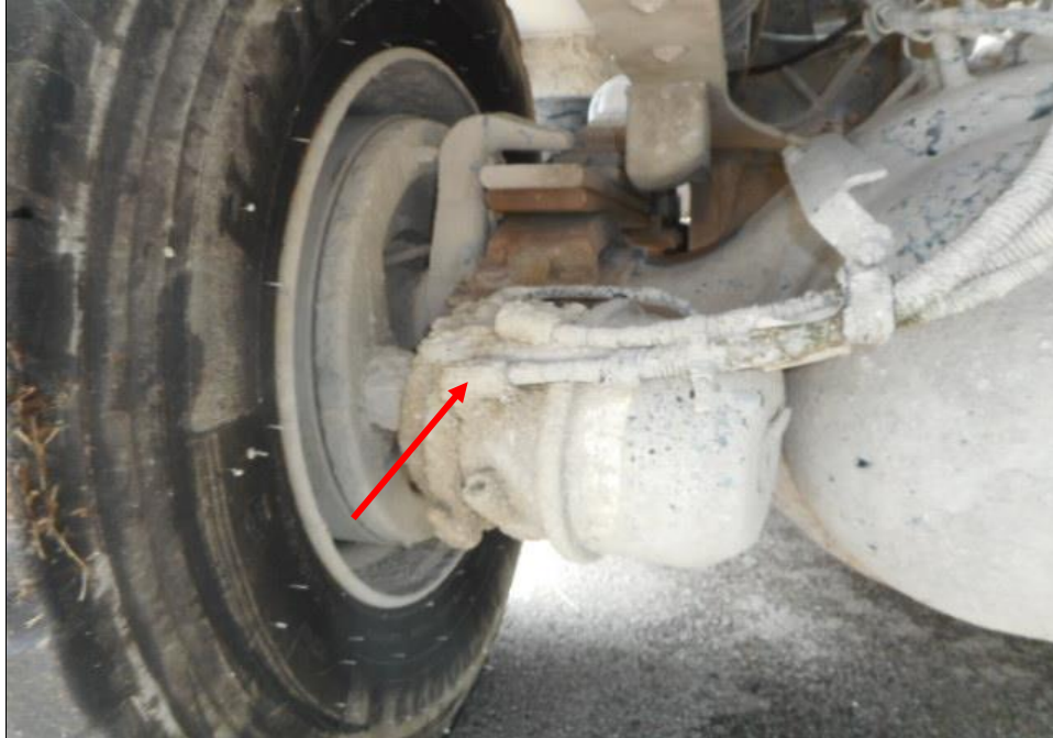
Photo 19 shows the brake pipe (arrowed) at the rear left wheel of the Tipper Truck. I did not observe any leakage of brake fluid at the time of my inspection of the Tipper Truck. My static tests of the Tipper Truck's braking system, along with my visual examination of the various mechanical components in the braking system, had indicated that there was no internal leakage of pressure/vacuum. Hence the braking system of the Tipper Truck was likely to be in serviceable condition at the material time of accident.
