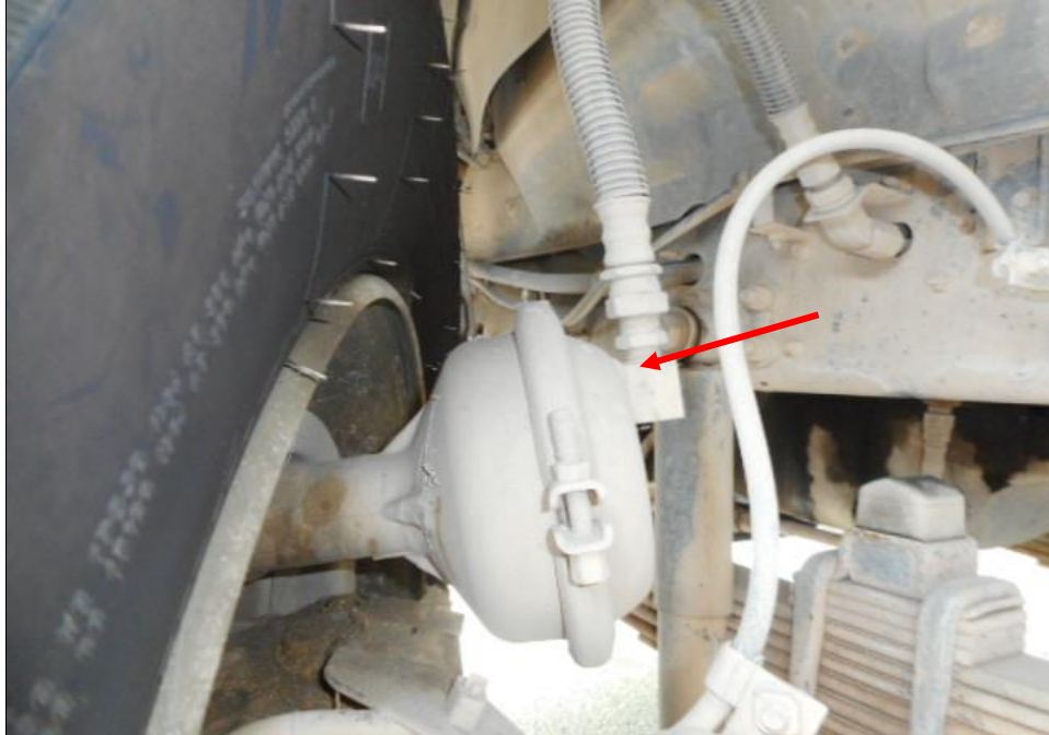
Photo 21 shows the brake pipe (arrowed) at the front left wheel of the Tipper Truck. I did not observe any leakage of brake fluid at the time of my inspection of the Tipper Truck. My static tests of the Tipper Truck's braking system, along with my visual examination of the various mechanical components in the braking system had indicated that there was no internal leakage of pressure/vacuum. Hence the braking system of the Tipper Truck was likely to be in serviceable condition at the material time of accident.
