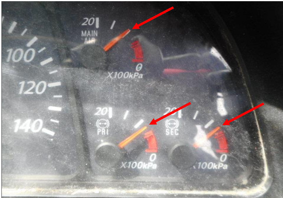
Photo 13 shows the air in the air brake cylinders of the Tipper Truck at the time of my inspection. The air in the cylinder was observed to be of sufficient level & serviceable at the time of the accident.
