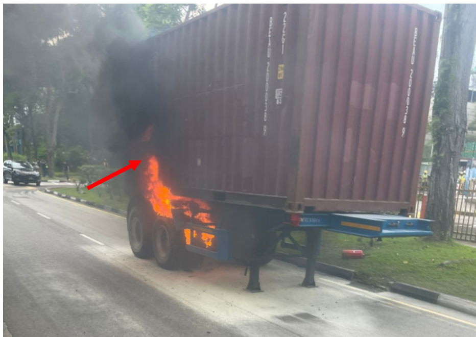
Photo 11 shows flames emitting from the right centre portion Insured Vehicle (arrowed) of the Insured Vehicle at the material time of incident. The photograph had showed similar extent of damage and burn pattern to the Insured Vehicle as per what we had observed during our physical inspection of the Insured Vehicle.
