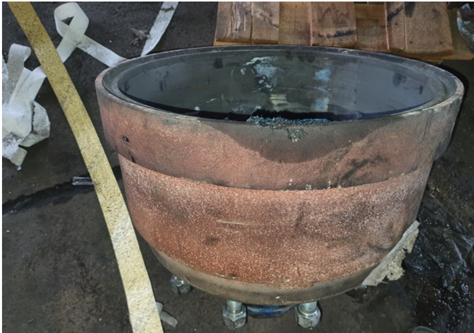
Photo 9 shows a general view of the rear left brake drum of the Insured Vehicle. Upon closer examination, we did not observe any damages to the exterior surface of the brake drum.
