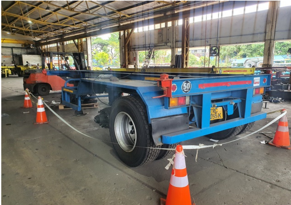
Photo 3 shows the general view of the left portion of the Insured Vehicle at the time of our inspection. The exterior body of the Insured Vehicle had sustained fire damage at the centre portion. Affected parts had included the centre wheel panels.
