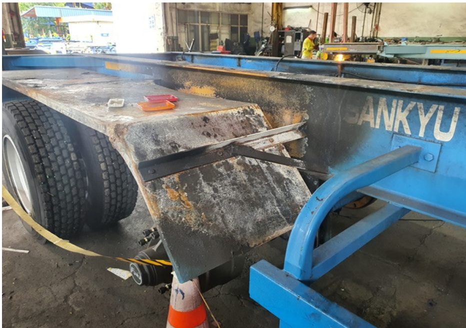
Photo 6 shows a closer view of the right centre portion of the Insured Vehicle at the time of our inspection. The fire damage was observed to be at its right centre portion. The right centre wheel panel was observed to be affected by the fire.
