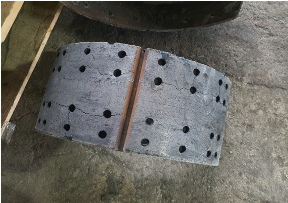
Photo 8 shows a close up view of the rear left top brake drum pad of the Insured Vehicle. Upon closer examination, we did not observed any damages to the brake drum pad.
