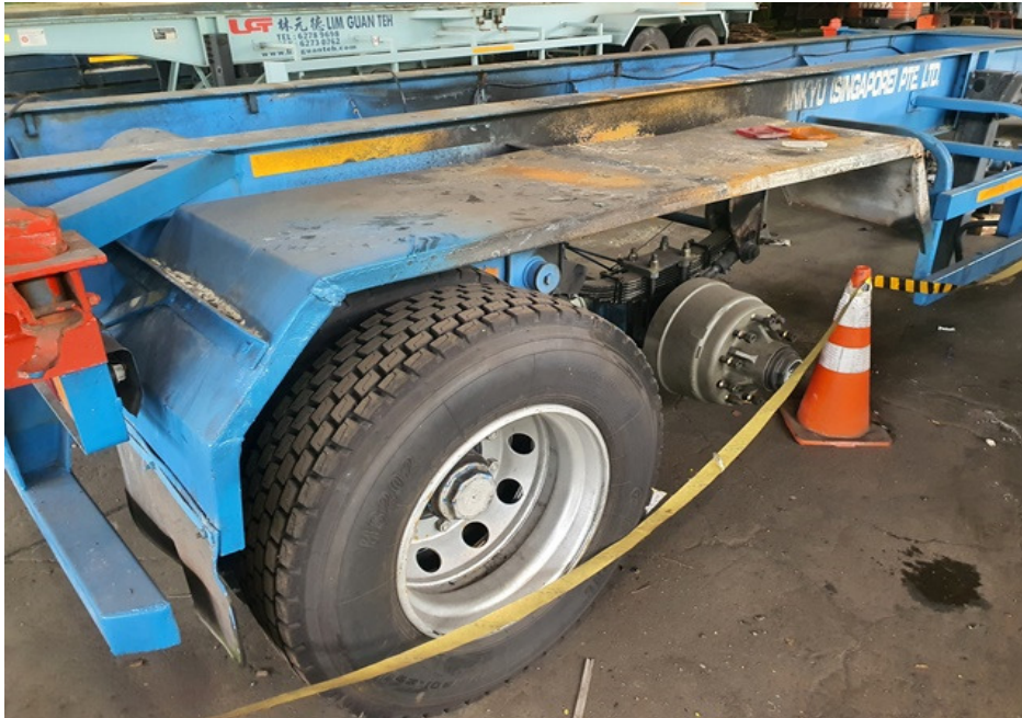
Photo 5 shows the close up view of the right centre portion of the Insured Vehicle at the time of our inspection. The right wheel panel and right centre wheel rims and the tyres of the Insured Vehicle had sustained severe fire damage.
