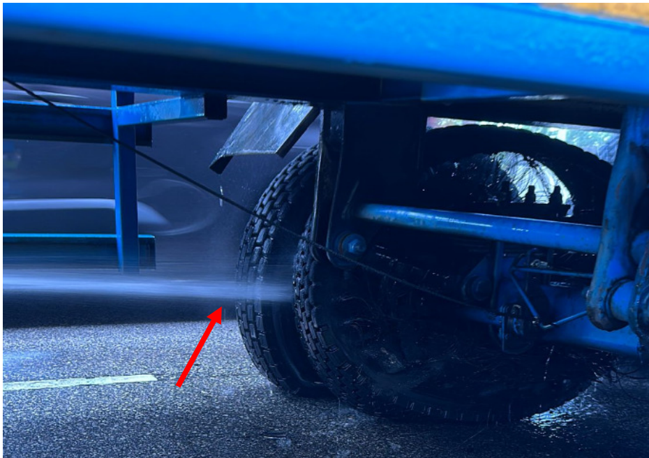
Photo 13 shows a close up view of the water being doused onto the right centre tyres of the Insured Vehicle with water post- incident (arrowed). Generally, the information that could be gathered from the incident scene photographs provided by Mr Tan had corresponded to the events that he had related to us, which is the fire had started from the right centre wheel.
