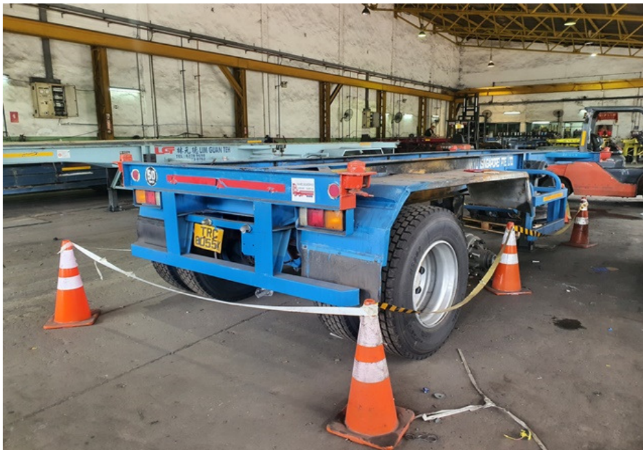
Photo 4 shows the general view of the right portion of the Insured Vehicle at the time of our inspection. The exterior body of the Insured Vehicle had sustained fire damages at the right centre wheel and rim area as well as its right centre wheel panel portion. Affected parts had included the right wheel panel and the right centre wheel and rims.
