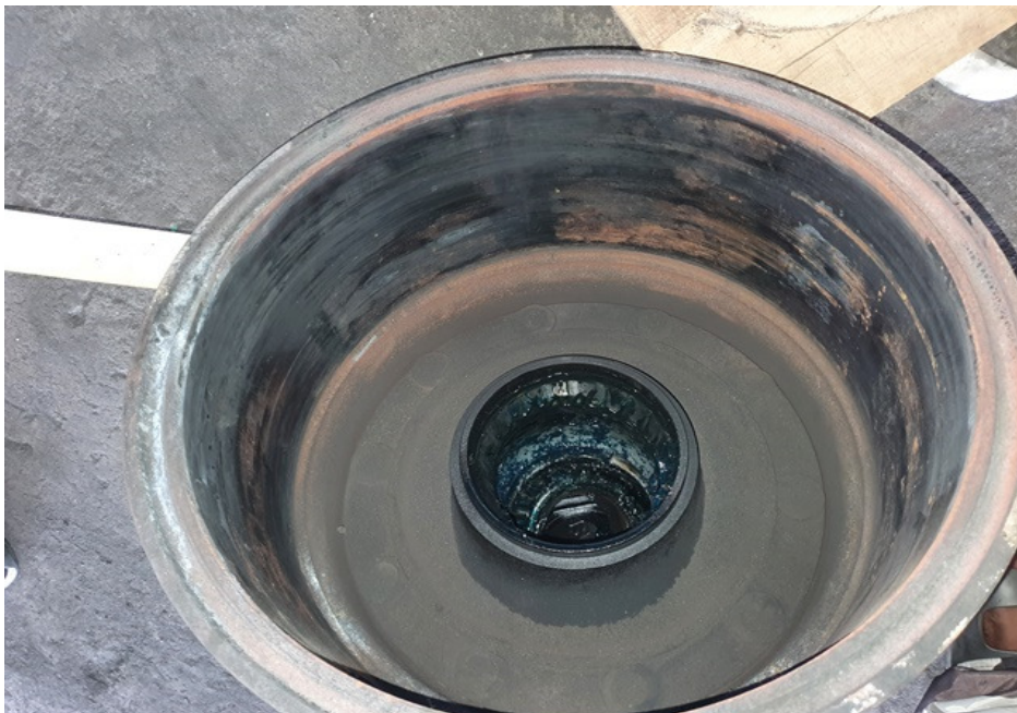
Photo 10 shows a general view of the rear left brake drum of the Insured Vehicle. Upon closer examination, we did not observe any damages to the interior surface of the brake drum.
