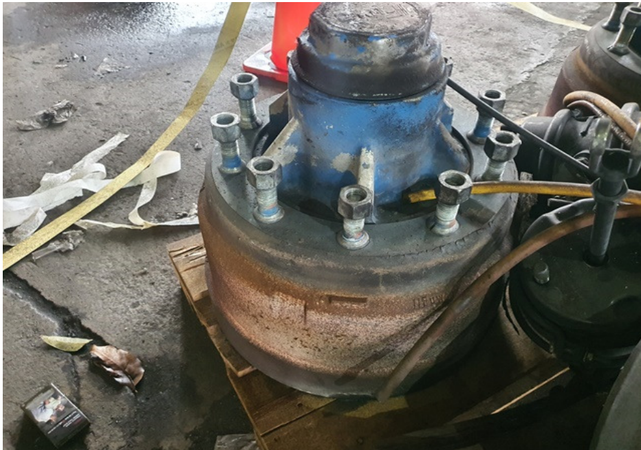
Photo 7 shows a general view of the right centre brake drum and brake pad of the Insured Vehicle after the wheel rim was removed. Upon closer examination, we did not observe any damages to the brake drum.
