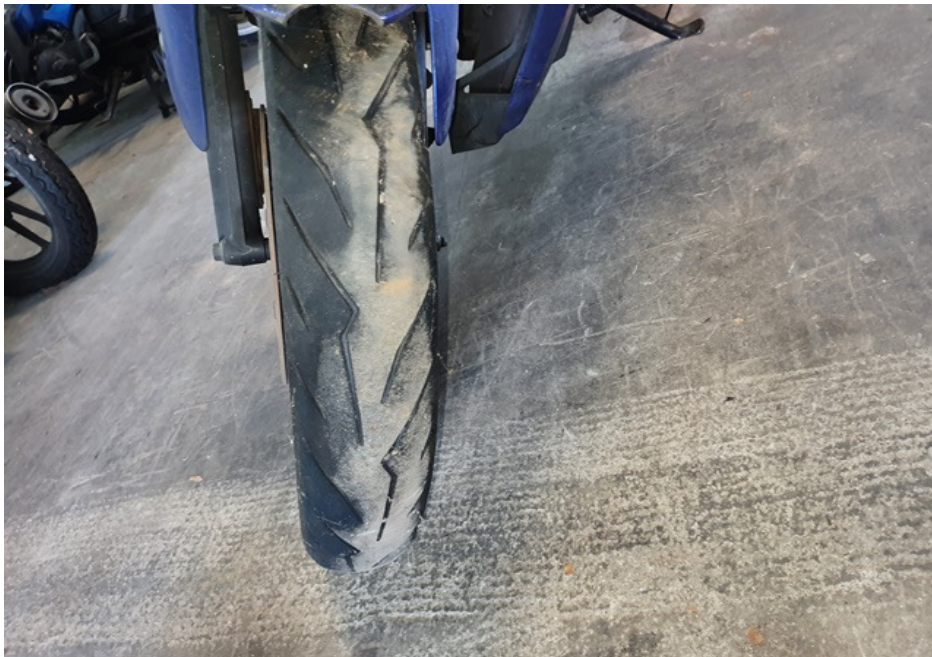
Photo 15 shows the front tyre of the Motorcycle at the time of our inspection. The front tyre was observed to be in serviceable condition with remaining tread depth of approximately 1mm. The pattern of the tread was also clearly visible. There was no tear, burst mark(s) and/or punctured hole(s) on the sidewalls as well as across the tread of the front tyre.
