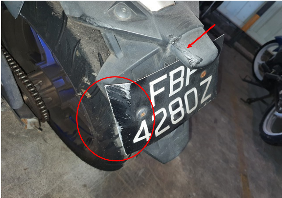
Photo 14 shows a closer view of the grazed rear mudguard (arrowed) and dented number plate (circled) of the Motorcycle at the time of our inspection.
