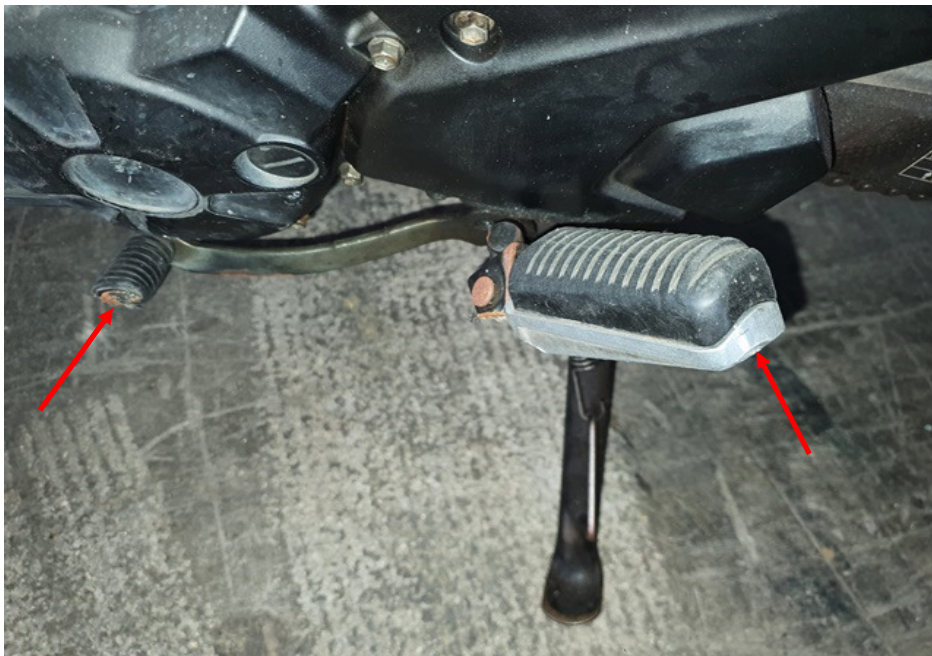
Photo 13 shows the gear shift pedal and left front footrest of the Motorcycle that had sustained damage at the time of our inspection (arrowed).
