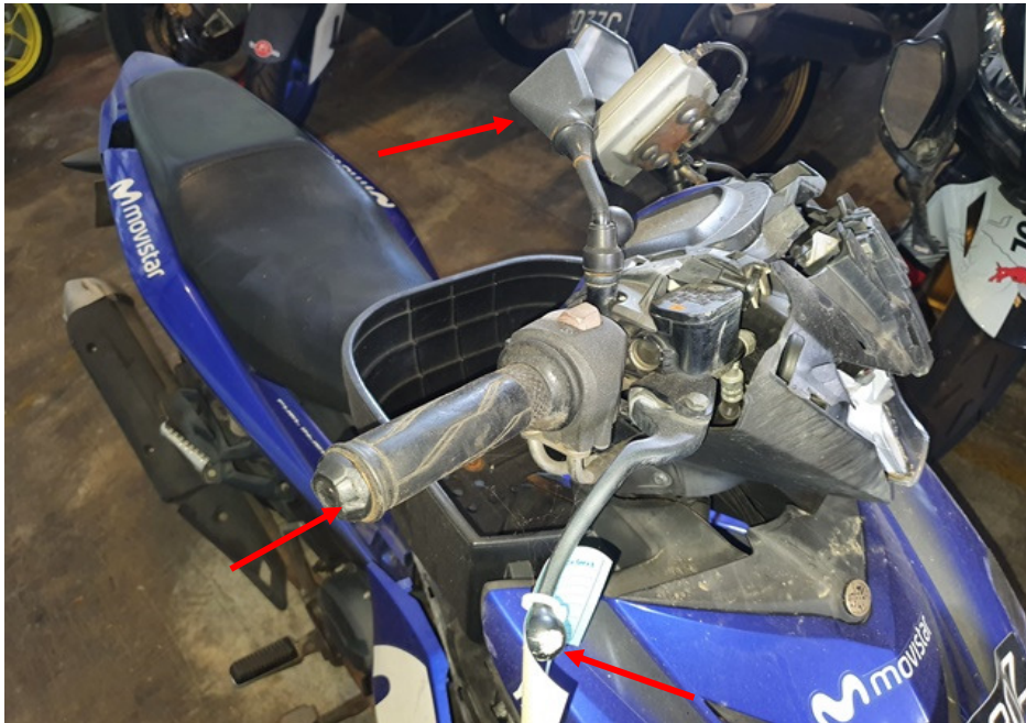
Photo 8 shows the right handlebar end, front brake lever and right side mirror (arrowed), which were amongst the body parts of the Motorcycle that had sustained damage at the time of our inspection.
