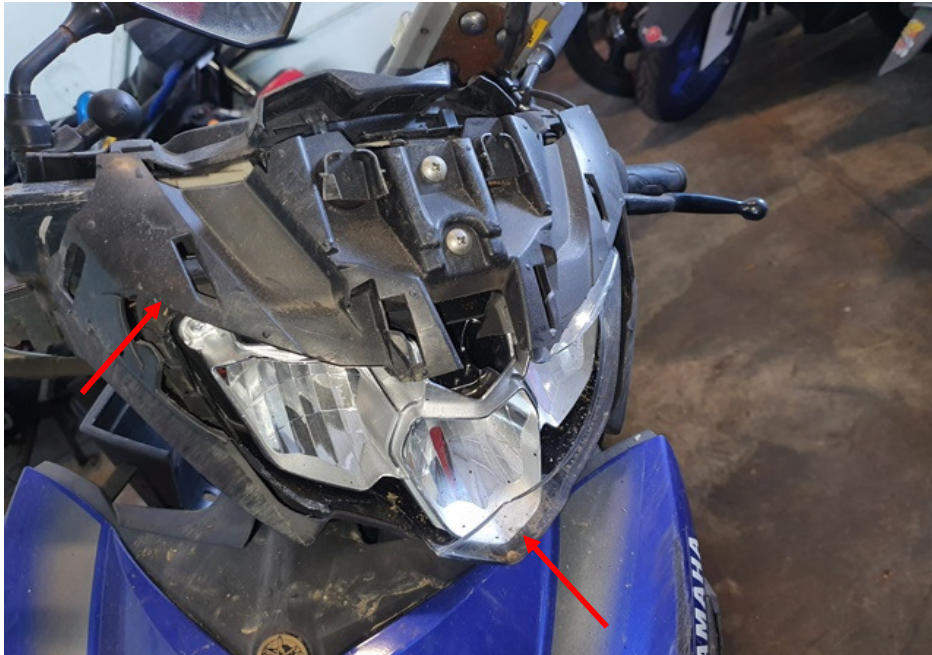
Photo 6 shows the head cowl and headlight (arrowed), which was amongst the body parts of the Motorcycle that had sustained damage at the time of our inspection.
