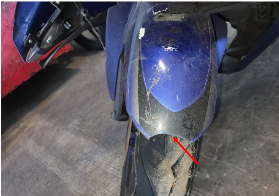
Photo 7 shows a closer view of cracked front mudguard (arrowed) of the Motorcycle at the time of our inspection.
