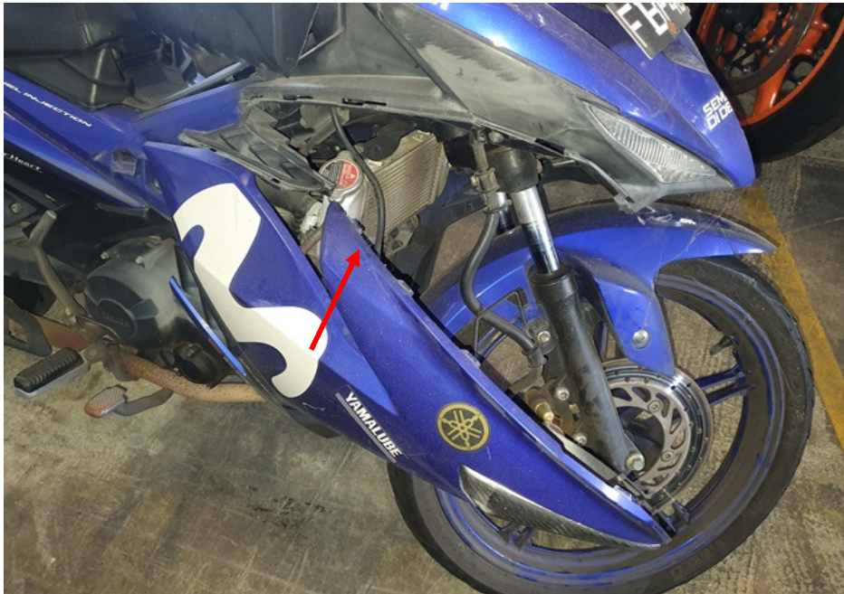
Photo 10 shows a closer view of cracked right cowling (arrowed) of the Motorcycle at the time of our inspection.
