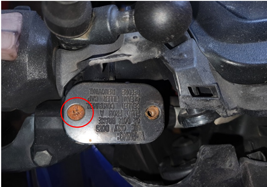
Photo 25 shows the brake fluid reservoir cover for the front brake of the Motorcycle. We were unable to examine whether the front brake fluid was without contamination due to a worn out screw (circled).
