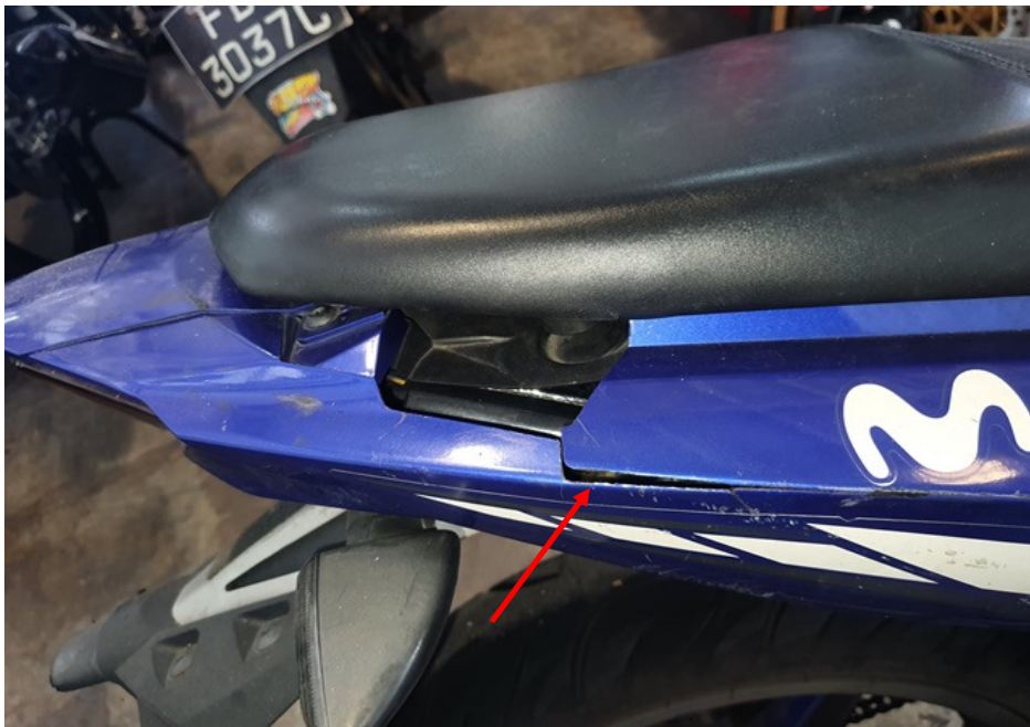
Photo 11 shows a closer view of the cracked right rear side cover of the Motorcycle at the time of our inspection (arrowed).
