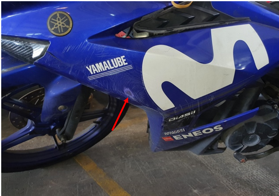
Photo 9 shows a closer view of grazed left cowling (arrowed) of the Motorcycle at the time of our inspection.
