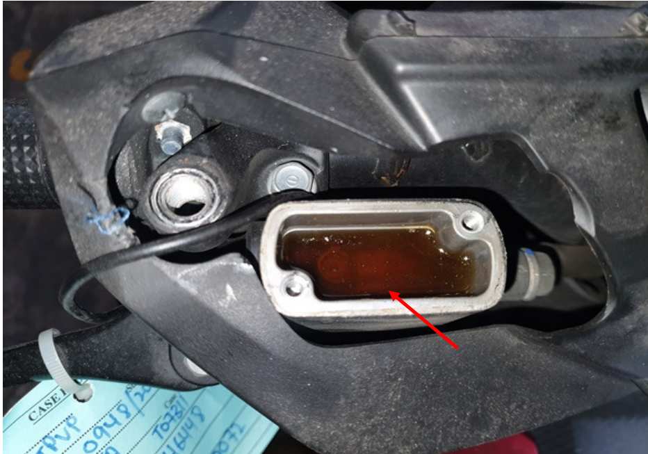
Photo 25 shows the brake fluid reservoir for the front brake of the Motorcycle. The brake fluid was observed to be of sufficient level for operational purposes. However it was found to be slightly contaminated (arrowed).
