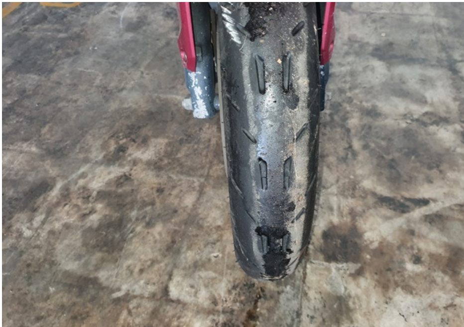
Photo 15 shows the front tyre of the Motorcycle at the time of our inspection. The front tyre was observed to be in serviceable condition with remaining tread depth of approximately 3mm. The pattern of the tread was also clearly visible. There was no tear, burst mark(s) and/or punctured hole(s) on the sidewalls as well as across the tread of the front tyre.
