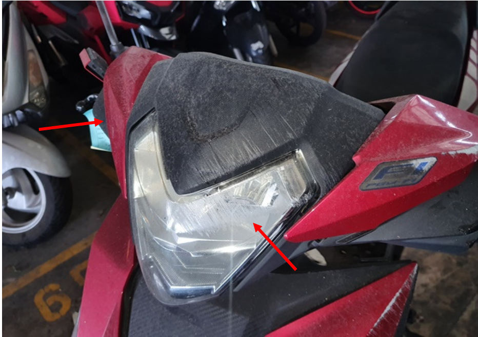
Photo 6 shows the head cowling and headlight (arrowed), which was amongst the body parts of the Motorcycle that had sustained damage at the time of our inspection.
