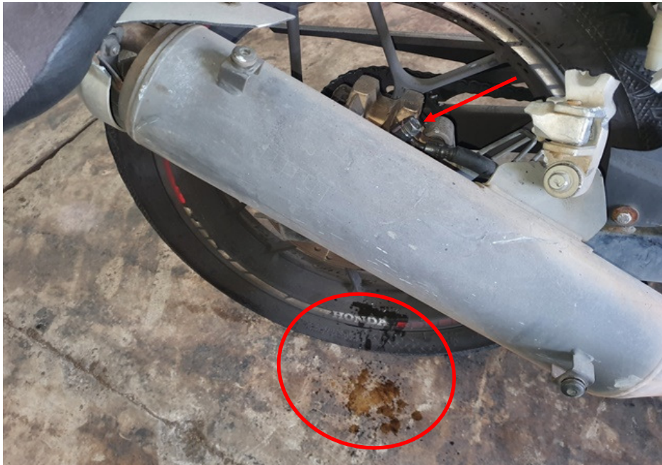
Photo 29 shows the rear wheel of the Motorcycle which was unable to stop rotating upon stepping on the brake pedal during the operational test of the rear braking system. Upon closer examination, we observed leakage of brake fluid (circled) from the rear brake caliper (arrowed) of the Motorcycle.
