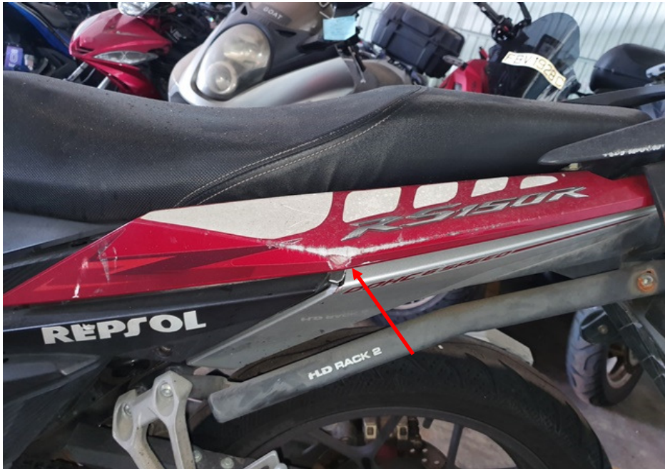
Photo 12 shows a closer view of the grazed left rear side cover of the Motorcycle at the time of our inspection (arrowed).
