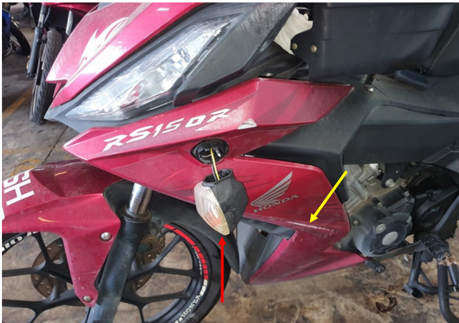
Photo 9 shows a closer view of grazed left cowling and dislodged left front signal lamp (arrowed) of the Motorcycle at the time of our inspection.
