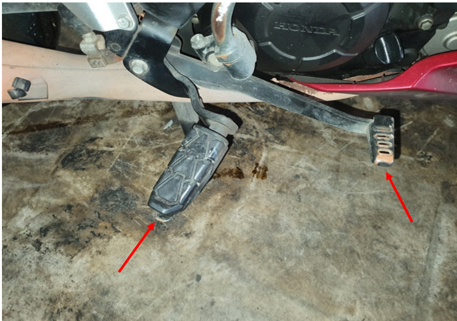
Photo 13 shows the rear brake pedal and right front footrest of the Motorcycle that had sustained damage at the time of our inspection (arrowed).
