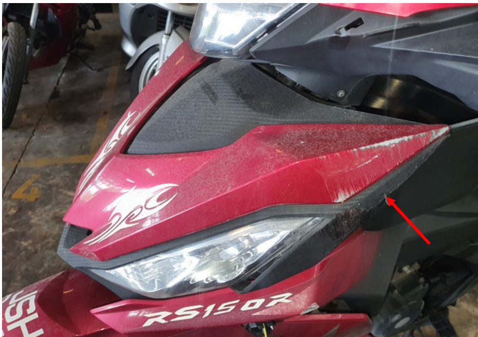
Photo 5 shows a closer view of grazed front cowlings (arrowed) of the Motorcycle at the time of our inspection.
