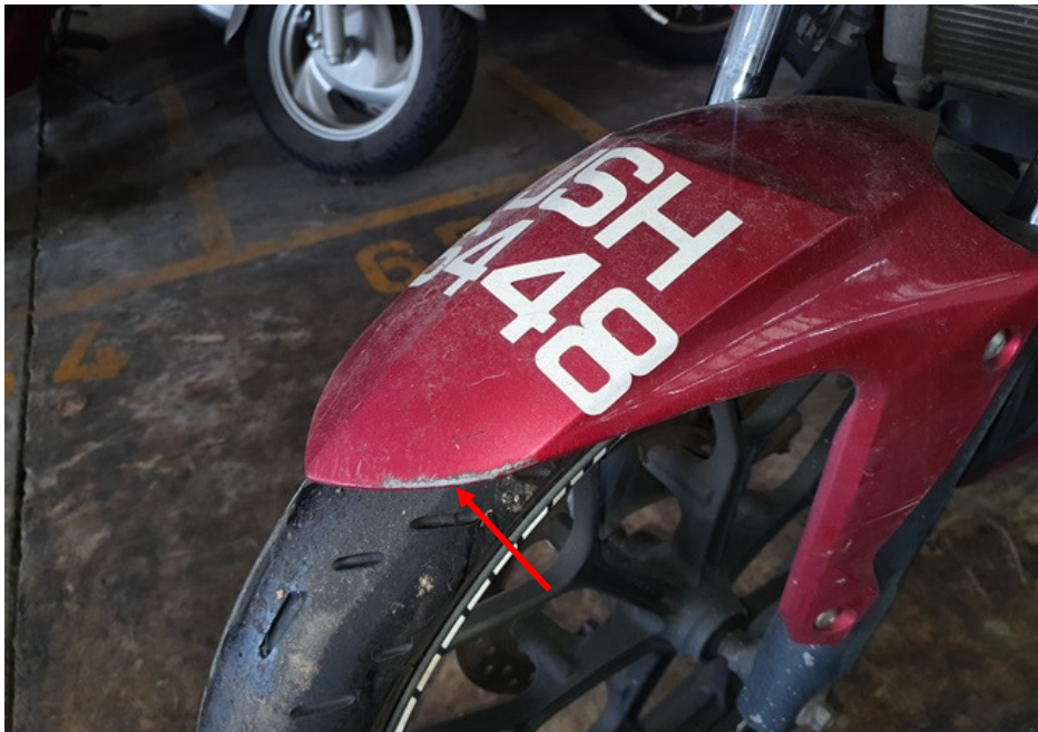
Photo 7 shows a closer view of grazed front mudguard (arrowed) of the Motorcycle at the time of our inspection.
