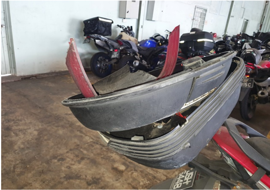
Photo 14 shows a closer view of the broken top box of the Motorcycle at the time of our inspection.
