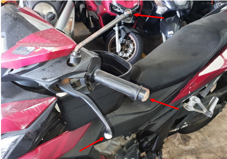
Photo 8 shows the left handlebar end, clutch lever and left side mirror (arrowed), which were amongst the body parts of the Motorcycle that had sustained damage at the time of our inspection.
