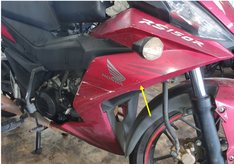
Photo 10 shows a closer view of grazed right cowling (arrowed) of the Motorcycle at the time of our inspection.
