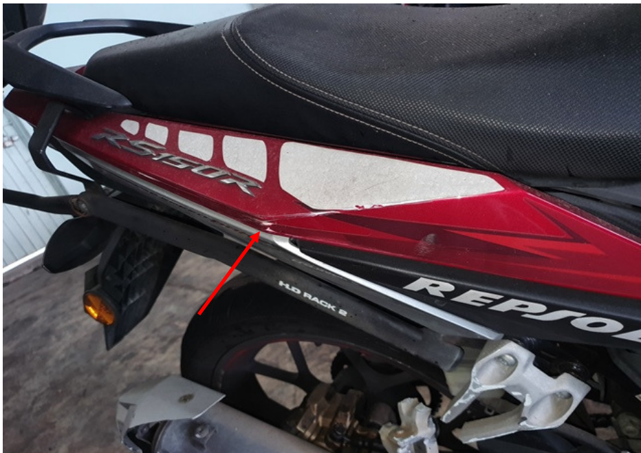
Photo 11 shows a closer view of the grazed right rear side cover of the Motorcycle at the time of our inspection (arrowed).
