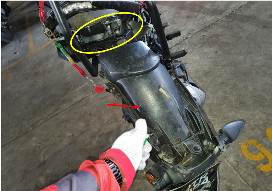
Photo 17 shows the dislodged rear mudguard (arrowed) and missing tail light (circled) of the Motorcycle at the time of our inspection.
