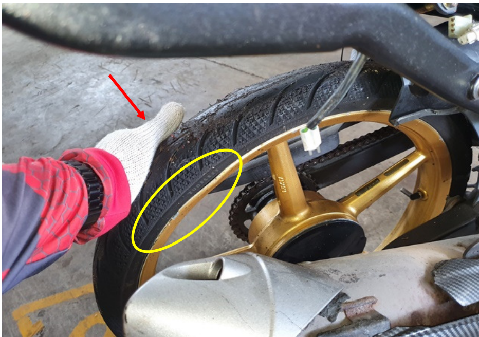
Photo 20 shows the deflated rear tyre (arrowed) and bent rear wheel rim (circled) of the Motorcycle at the time of our inspection.
