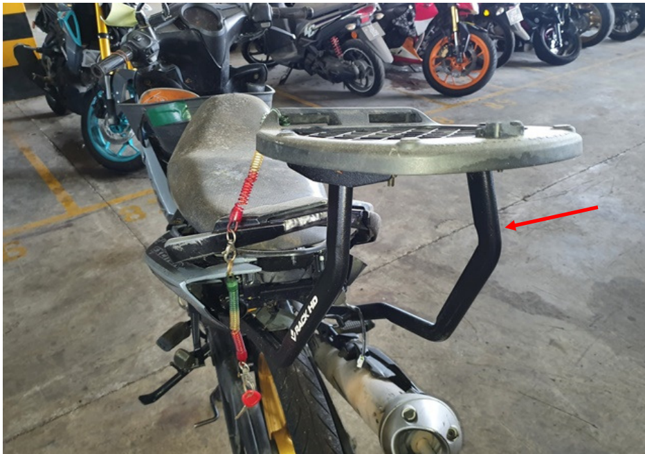
Photo 16 shows the bent top box rack (arrowed) of the Motorcycle at the time of our inspection.
