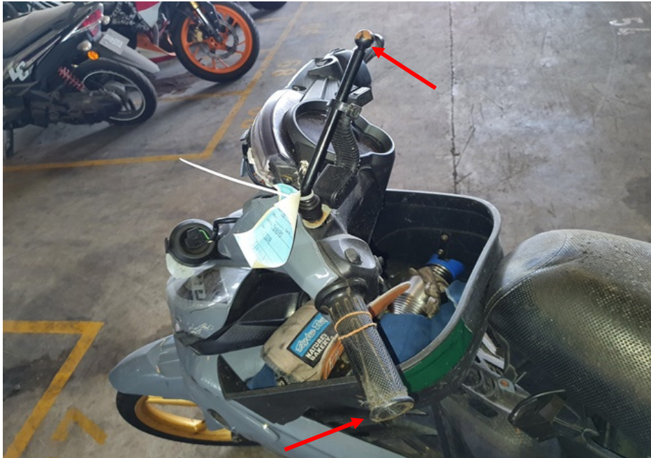
Photo 9 shows a closer view of the damaged left side mirror and left handlebar end of the Motorcycle (arrowed) at the time of our inspection.
