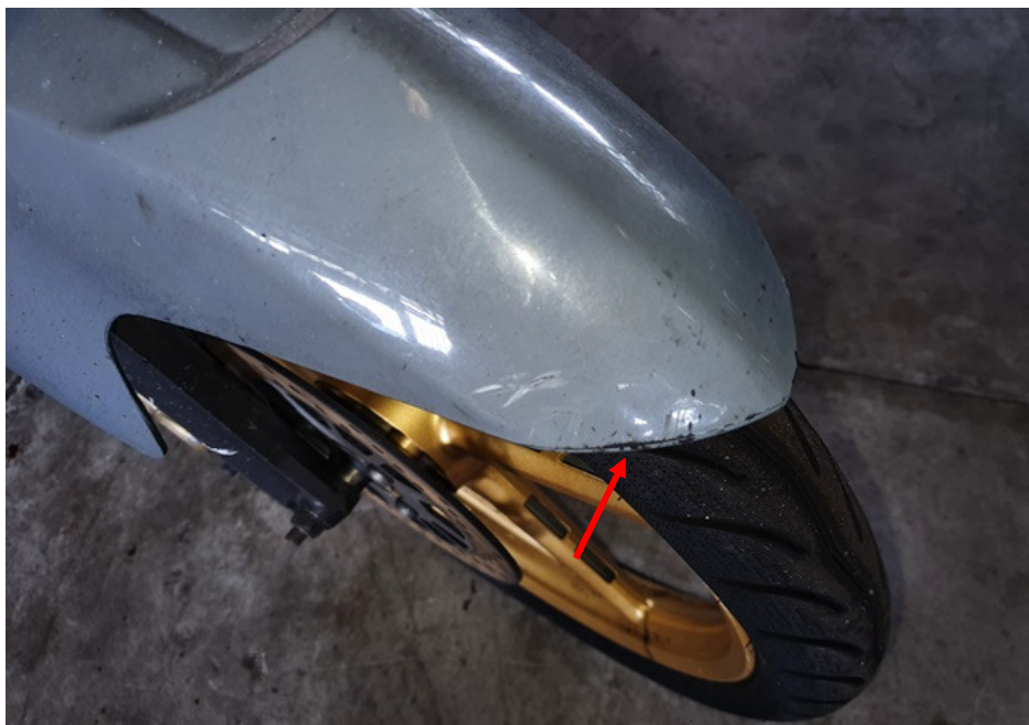
Photo 8 shows a closer view of the grazed front mudguard of the Motorcycle (arrowed) at the time of our inspection.
