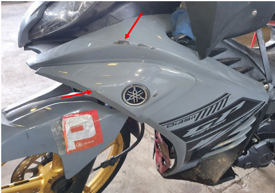
Photo 11 shows a closer view of the grazed left cowling of the Motorcycle at the time of our inspection (arrowed).
