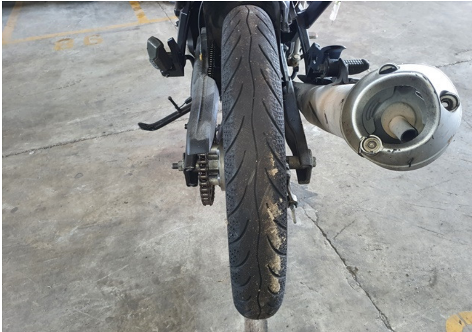
Photo 19 shows the condition of the Motorcycle's rear tyre. The rear tyre was observed to be in serviceable condition with remaining tread depth of approximately 2mm. We did not observe any tear, burst mark(s) and/or punctured hole(s) on the sidewalls as well as across the tread of the rear tyre. However the rear tyre was also observed to be deflated.
