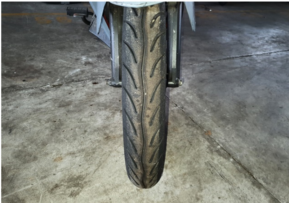
Photo 18 shows the condition of the Motorcycle's front tyre. The front tyre was observed to be in serviceable condition with remaining tread depth of approximately 4mm. There was no tear, burst mark(s) and/or punctured hole(s) on the sidewalls as well as across the tread of the front tyre.
