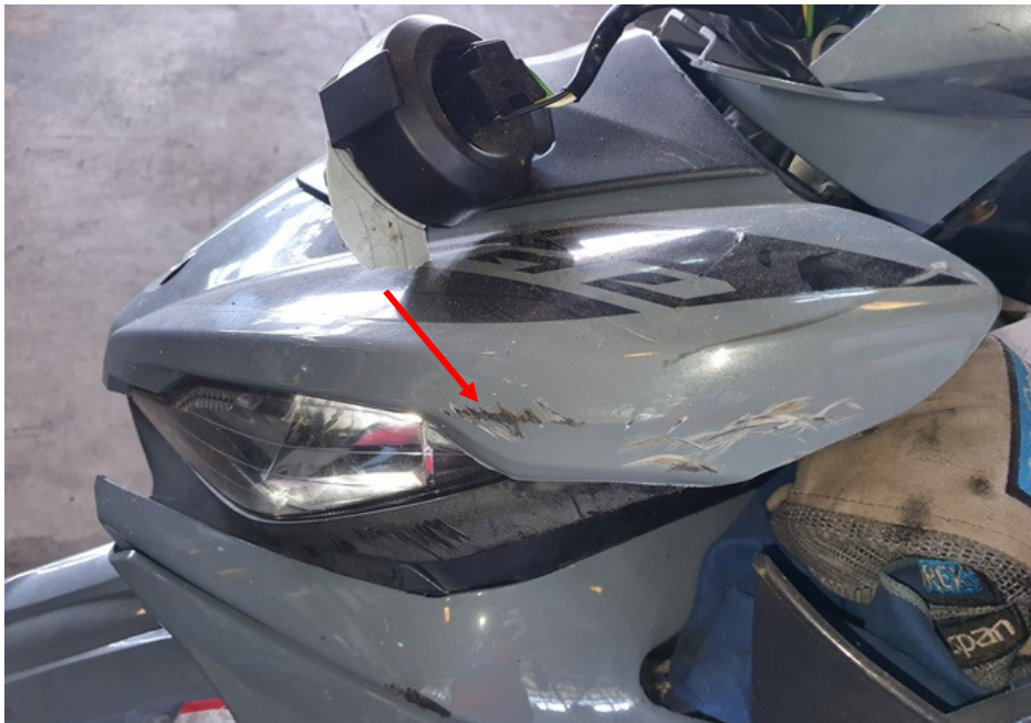
Photo 10 shows a closer view of the grazed front cowling of the Motorcycle at the time of our inspection (arrowed).
