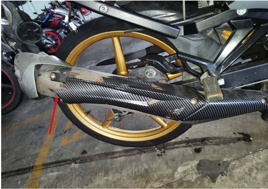
Photo 15 shows a closer view of the cracked exhaust muffler hear shield of the Motorcycle (arrowed) at the time of our inspection.
