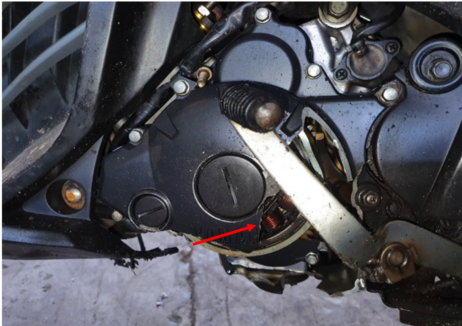
Photo 21 shows the left side of the engine of the Motorcycle at the time of our inspection. The left engine cover was found to be cracked (arrowed). However there was no fluid leak and/or fluid stain found around the left engine area of the Motorcycle.
