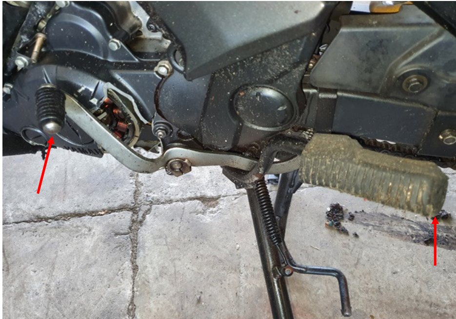
Photo 13 shows the gear shift pedal and left front footrest of the Motorcycle which had sustained damage at the time of our inspection (arrowed).
