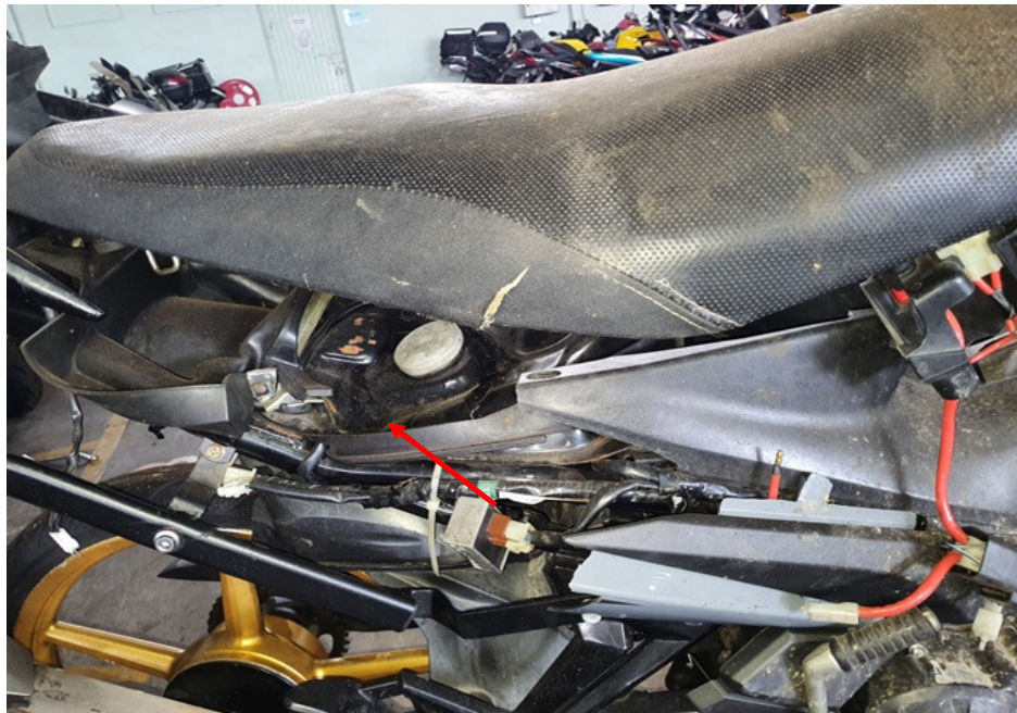
Photo 14 shows a closer view of the missing right rear side cover of the Motorcycle at the time of our inspection (arrowed).
