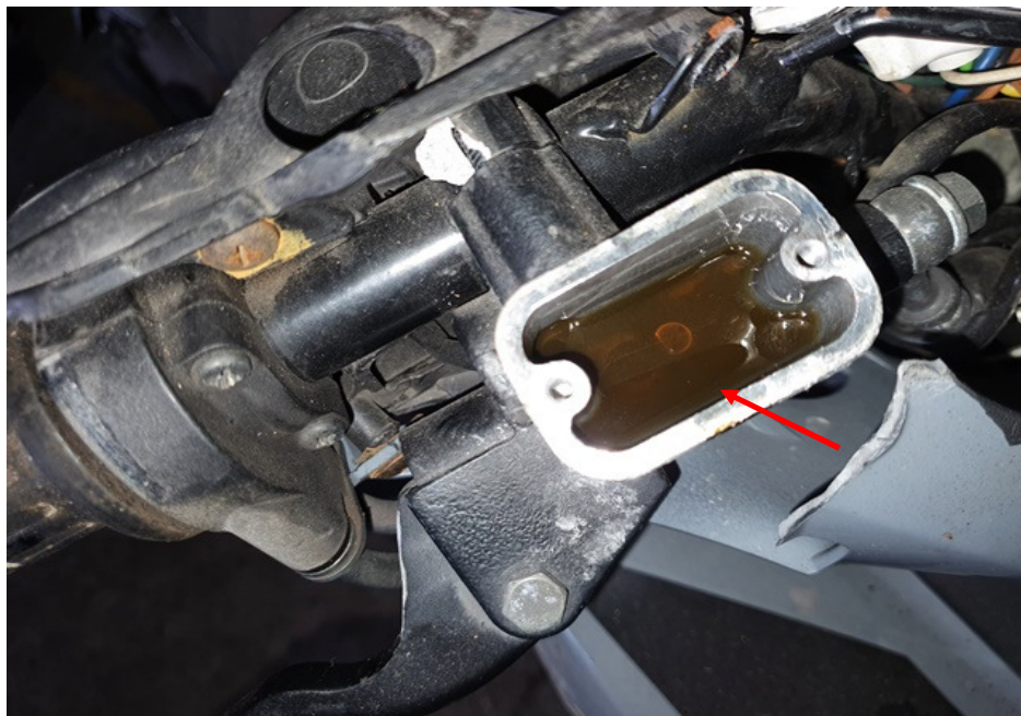
Photo 27 shows the brake fluid reservoir for the front brake of the Motorcycle. The brake fluid was found to be of sufficient level for operating purposes. However the brake fluid was found to be contaminated (arrowed).
