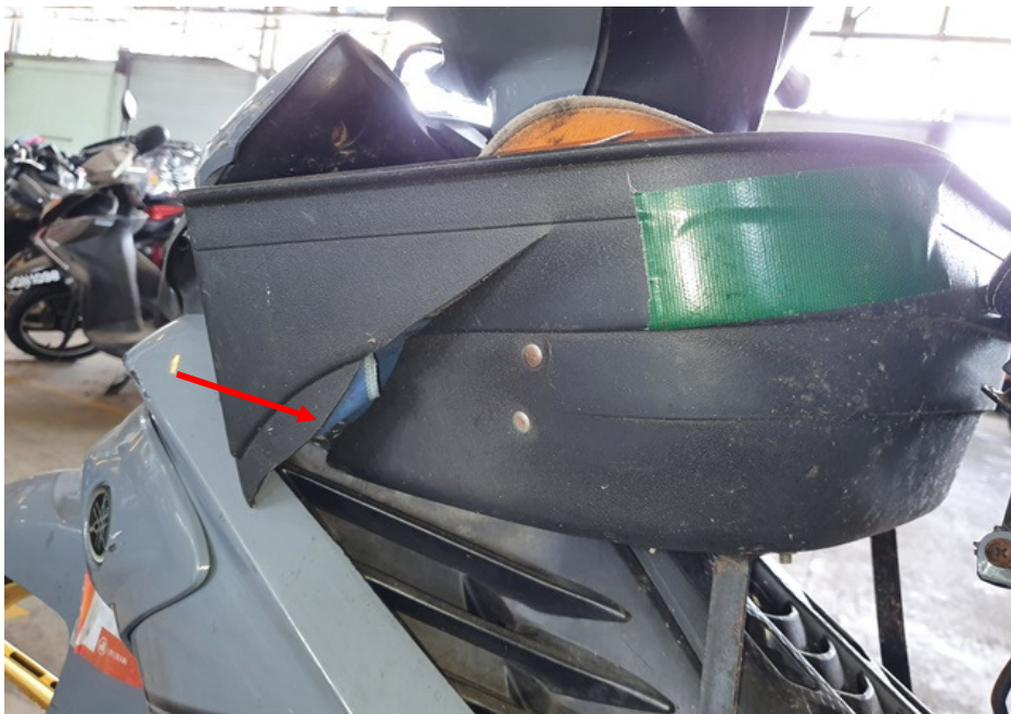
Photo 12 shows a closer view of the cracked front basket of the Motorcycle at the time of our inspection (arrowed).
