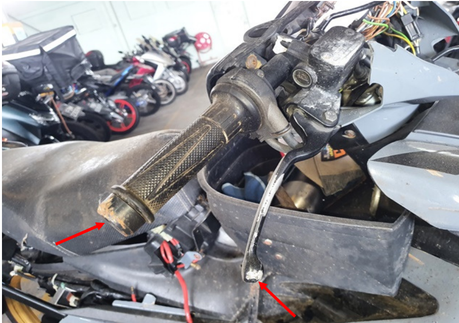
Photo 7 shows a closer view of the grazed front brake lever and right handlebar end of the Motorcycle (arrowed) at the time of our inspection.
