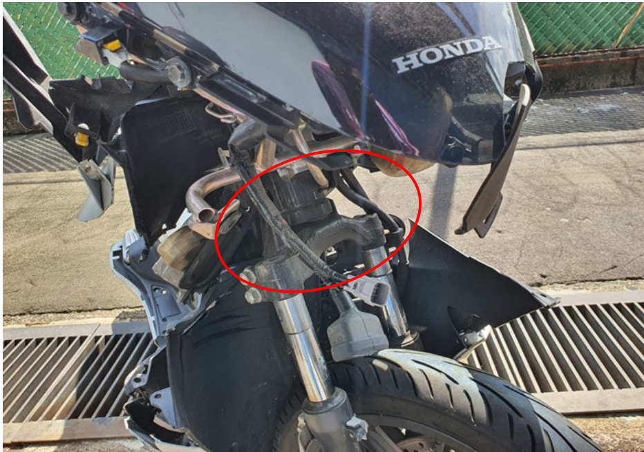
Photo 7 shows a closer view of the missing headlight assembly (arrowed) which was amongst the body parts at the front body of the Motorcycle that had sustained damage at the time of our inspection.
