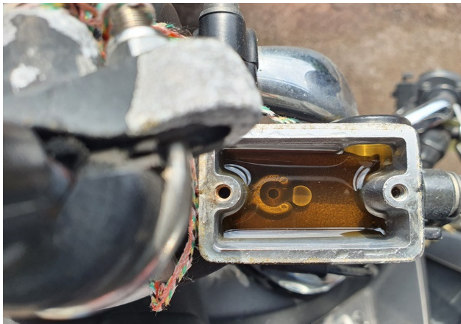
Photo 24 shows the brake fluid reservoir for the front brake of the Motorcycle. The brake fluid was observed to be of sufficient level for operational purposes and without contamination.
