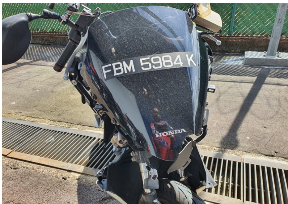
Photo 6 shows a closer view of the cracked windshield and front cowling of the Motorcycle at the time of our inspection
