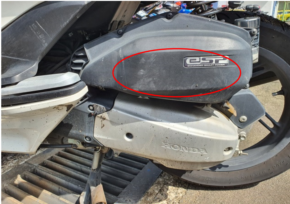
Photo 19 shows the drive train cover of the Motorcycle which had sustained damages of grazing nature at the time of our inspection (circled) however the engine components were still intact.
