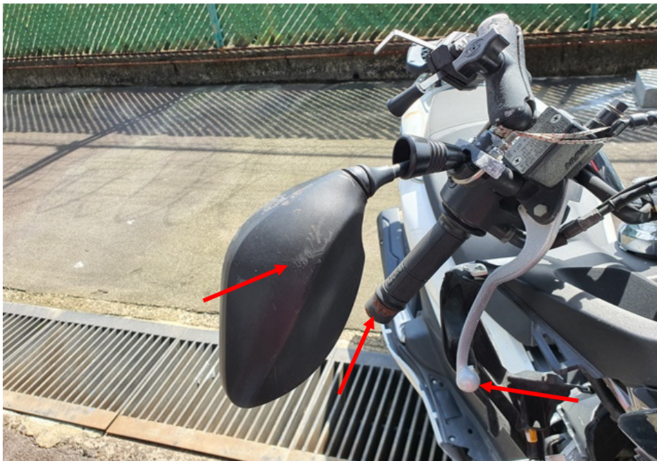
Photo 8 shows a closer view of the right side mirror, right handlebar end and front brake lever of the Motorcycle which were observed to be damaged at the time of our inspection (arrowed).
