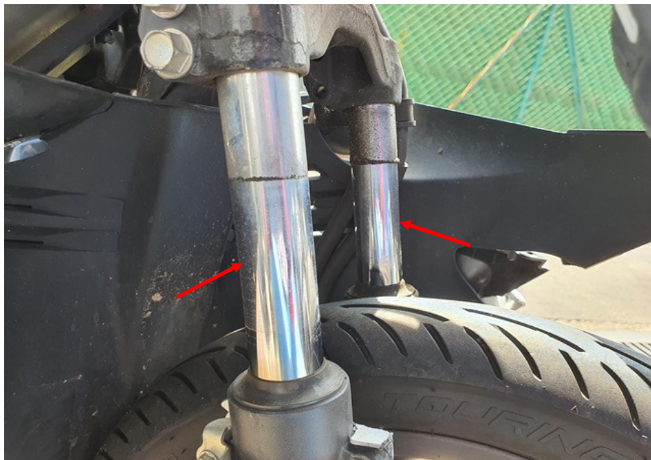
Photo 22 shows the front forks of the Motorcycle. The front forks were observed to be bent (arrowed) as a result of the accident. We were hence not able to conduct any tests on the steering system of the Motorcycle.
