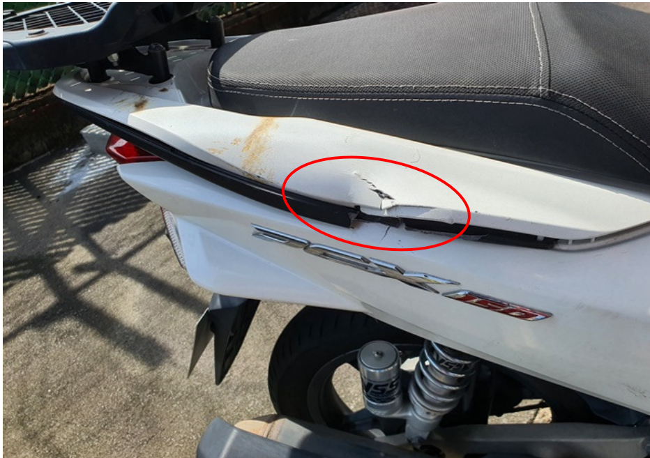
Photo 13 shows a closer view of the cracked right rear side cover of the Motorcycle at the time of our inspection (circled).
