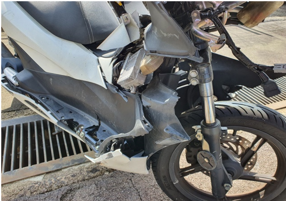
Photo 10 shows the cracked right side cowling of the Motorcycle at the time of our inspection.
