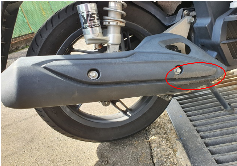
Photo 14 shows a closer view of the grazed exhaust muffler heat shield of the Motorcycle at the time of our inspection (circled).
