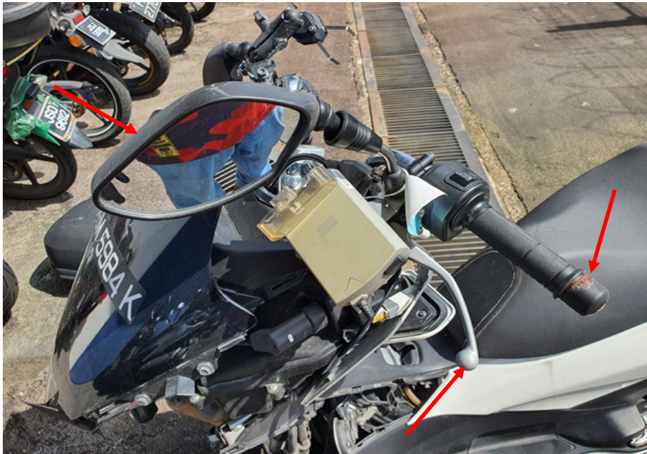
Photo 9 shows a closer view of the left side mirror, left handlebar end and rear brake lever of the Motorcycle which were observed to be damaged at the time of our inspection (arrowed).
