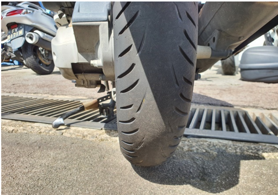
Photo 17 shows the condition of the Motorcycle's rear tyre. The rear tyre was observed to be bald. The tyre was also observed to be sufficiently inflated for vehicular operation. We did not observe any tear, burst mark(s) and/or punctured hole(s) on the sidewalls as well as across the tread of the rear tyre.
