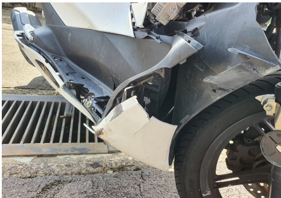
Photo 12 shows a close-up view of the cracked right bottom cowling of the Motorcycle at the time of our inspection.
