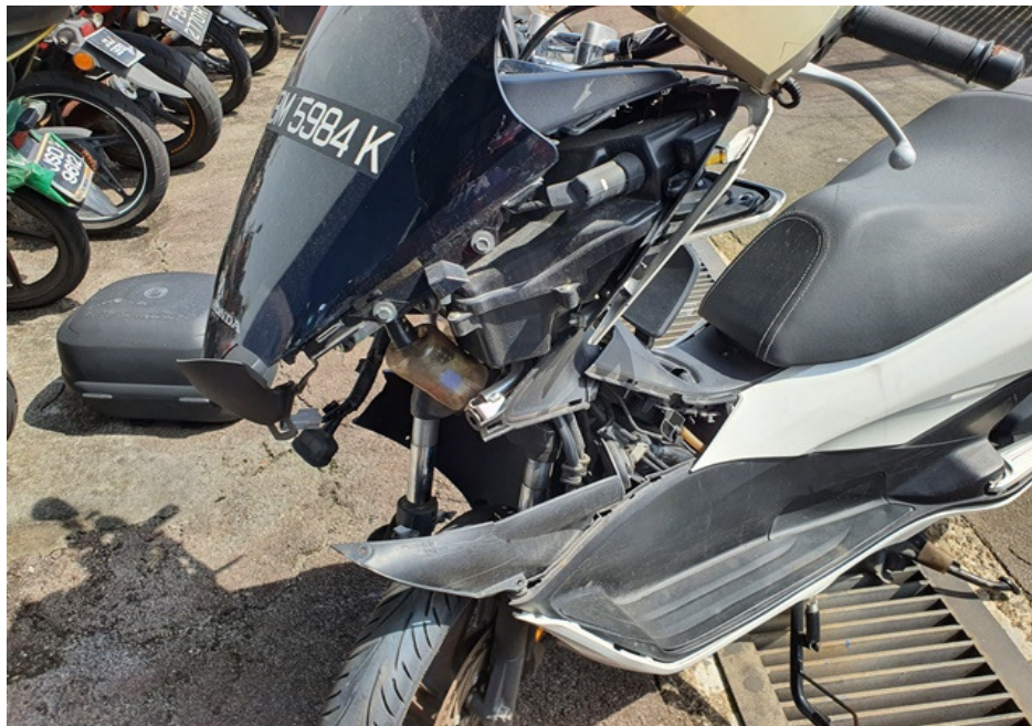
Photo 11 shows the cracked left side cowling of the Motorcycle at the time of our inspection.
