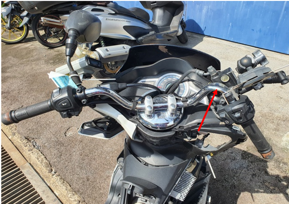
Photo 15 shows a closer view of the bent handlebar of the Motorcycle at the time of our inspection (arrowed).
