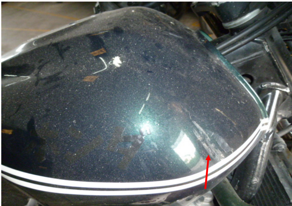
Photo 9 shows the dented petrol tank (arrowed) of the Motorcycle as a result of the accident.
