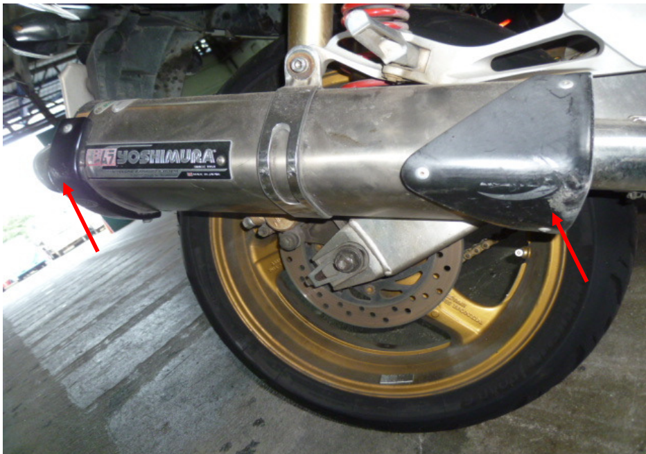
Photo 13 shows a closer view of the grazed exhaust muffler guard (arrowed) which was amongst the body parts at the rear body of the Motorcycle that had sustained damage as a result of the accident.
