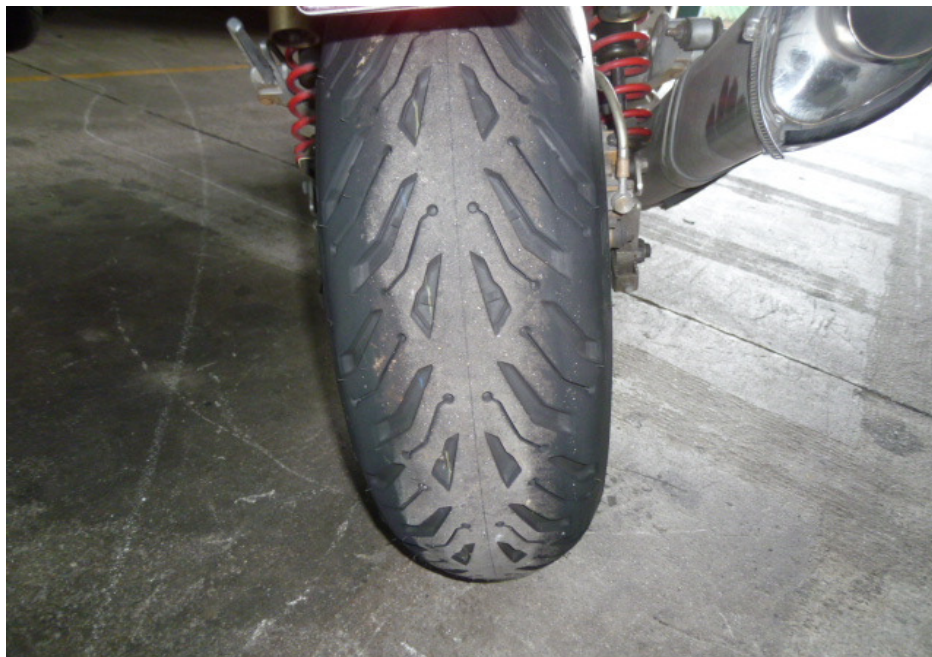
Photo 15 shows the condition of the Motorcycle's rear tyre. The rear tyre was observed to be in serviceable condition with remaining tread depth of approximately 8mm. The tyre was also observed to be sufficiently inflated for vehicular operation. We did not observe any tear, burst mark(s) and/or punctured hole(s) on the sidewalls as well as across the tread of the rear tyre.
