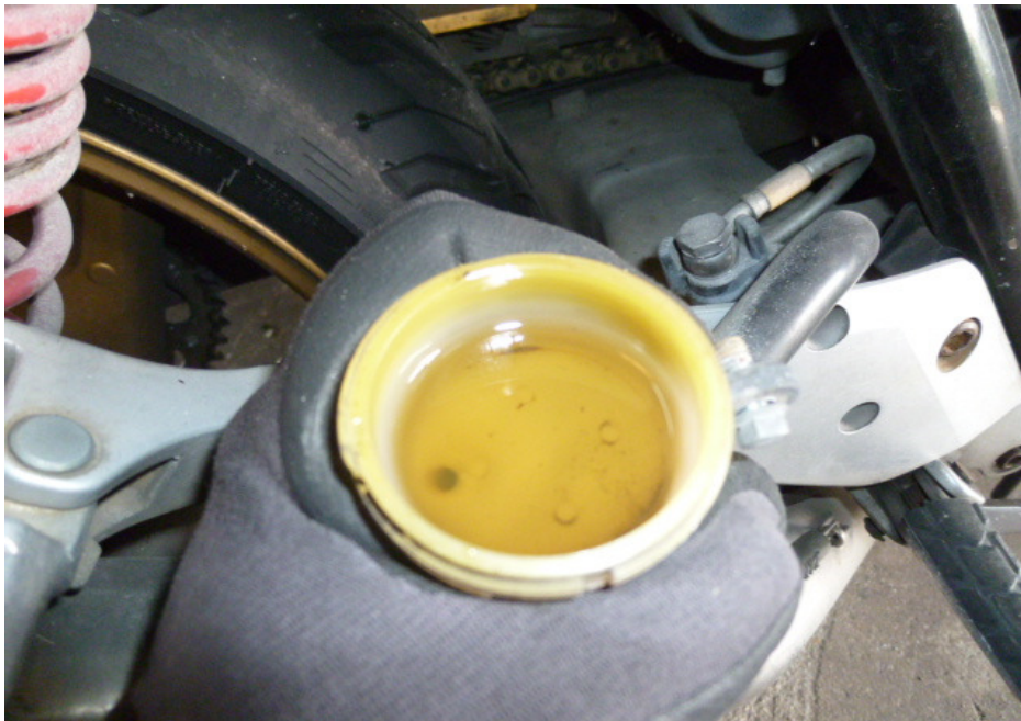
Photo 29 shows the brake fluid reservoir for the rear brake of the Motorcycle. The brake fluid was observed to be of sufficient level for operational purposes and without any contamination.
