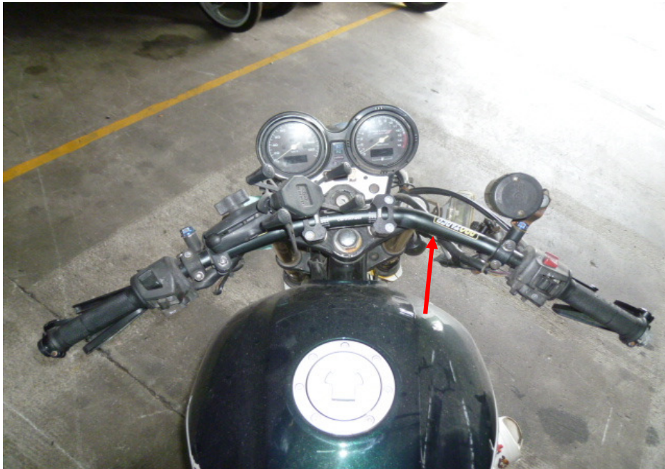
Photo 8 shows the bent handlebar of the Motorcycle (arrowed) at the time of our inspection.
