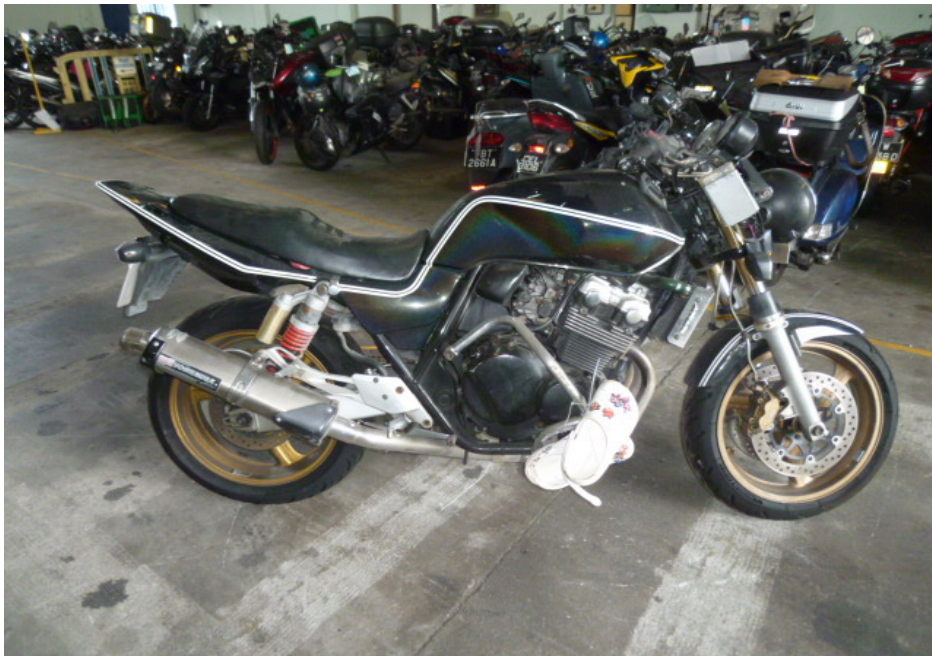
Photo 3 shows a general view of the right body of the Motorcycle at the time of our inspection. The Motorcycle was observed to have sustained damages at its frontal portion and right body. The body parts that were found to have been damaged include its headlight, front mudguard, right handlebar end, front brake lever, petrol tank, and right engine crashbar, amongst others.
