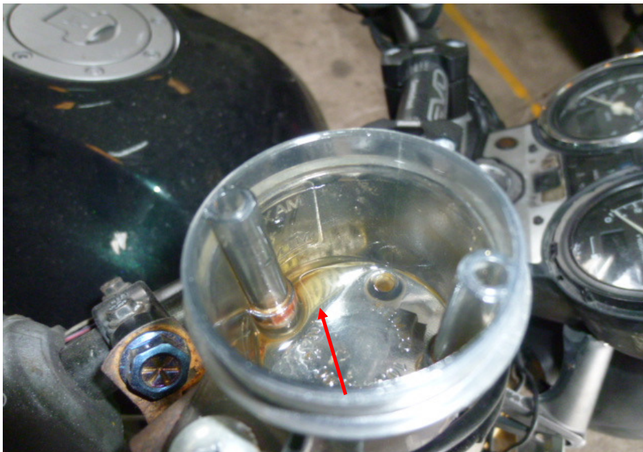
Photo 25 shows the brake fluid reservoir for the front brake of the Motorcycle. The brake fluid was observed to be of insufficient level for operational purposes (arrowed).
