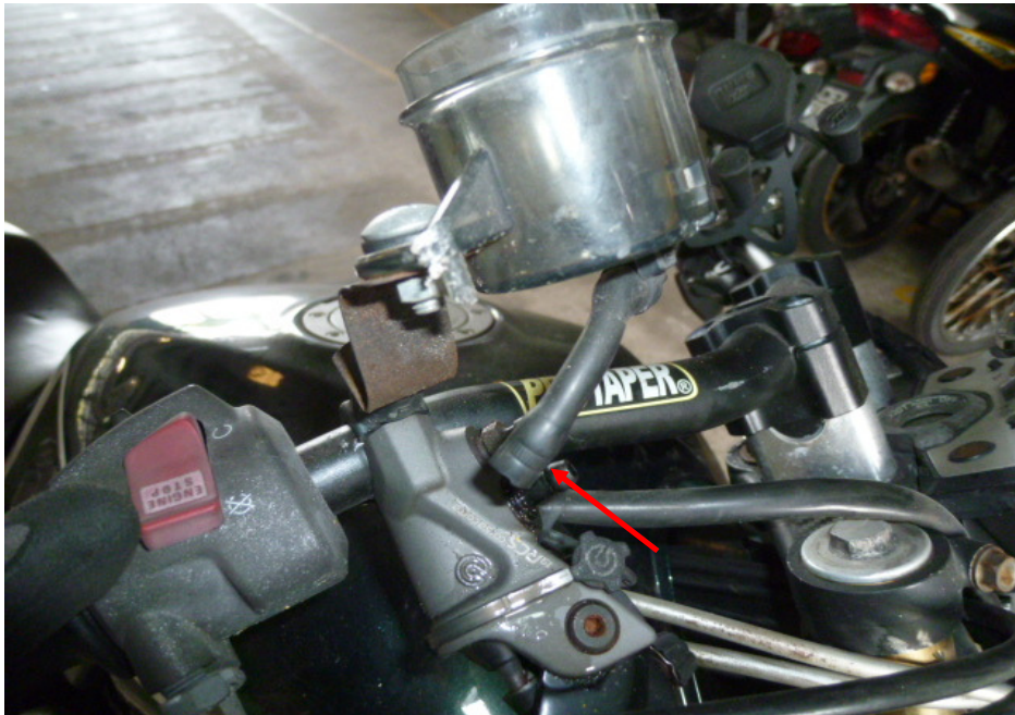
Photo 26 shows upon closer examination, we observed the reservoir hose was detached from the front brake master cylinder (arrowed) as a result of the accident.
