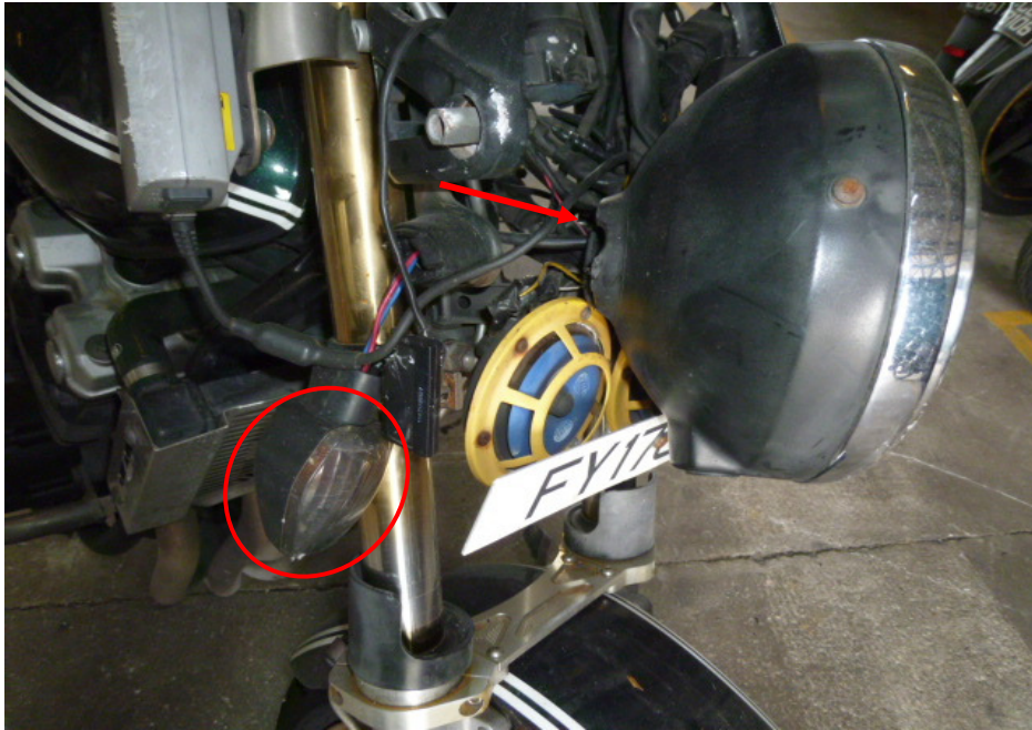
Photo 4 shows a closer view of the broken headlight (arrowed) and broken right front signal lamp (circled) of the Motorcycle as a result of the accident.
