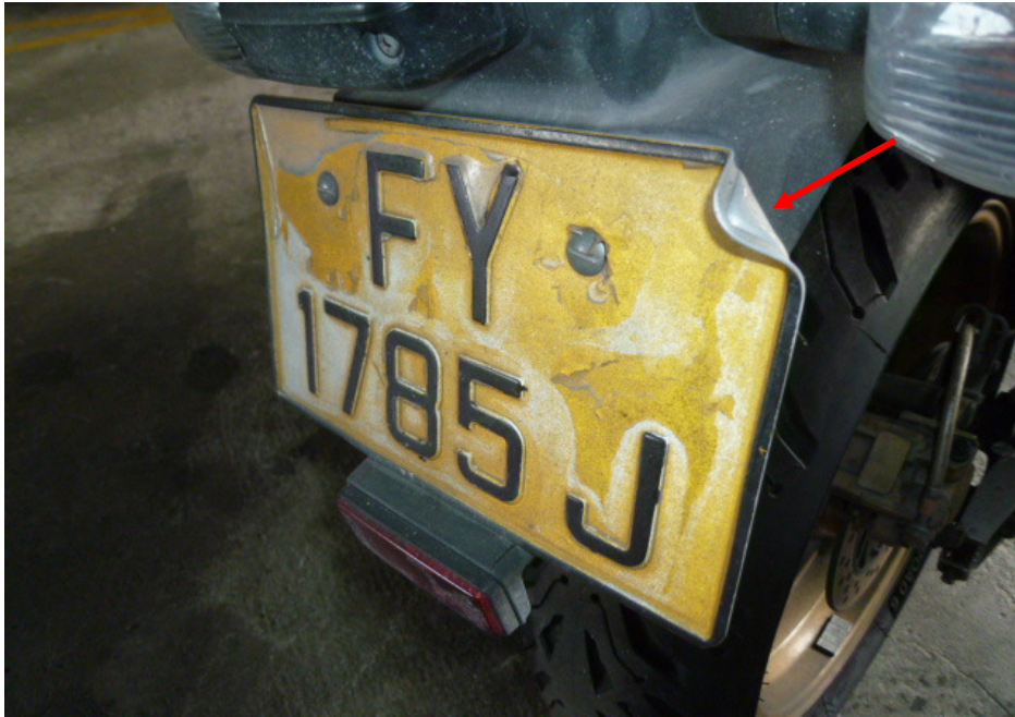
Photo 12 shows a closer view of the dented rear number plate (arrowed) of the Motorcycle as a result of the accident.
