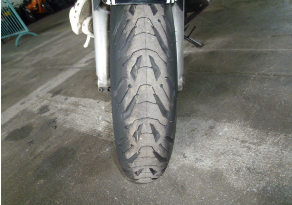
Photo 14 shows the front tyre of the Motorcycle at the time of our inspection. The front tyre was observed to be in serviceable condition with remaining tread depth of approximately 6mm. The pattern of the tread was also clearly visible. There was no tear, burst mark(s) and/or punctured hole(s) on the sidewalls as well as across the tread of the front tyre.
