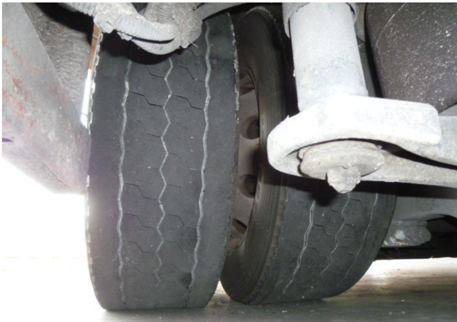
Photo 11 shows the condition of the rear right tyres of the Motor Bus, which were observed to be in serviceable condition with remaining tread depth of approximately 9mm. The tyres, which were wrapped around standard steel wheel rims, were also observed to be sufficiently inflated for vehicular operation.
