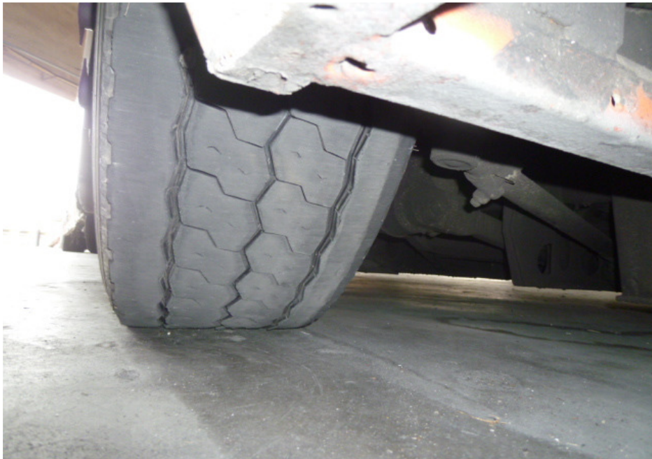
Photo 10 shows the condition of the front right tyre of the Motor Bus, which was observed to be in serviceable condition with remaining tread depth of approximately 17mm. The tyre, which was wrapped around standard steel wheel rim, was also observed to be sufficiently inflated for vehicular operation. There was no tear, cut or burst mark(s) on the outer and the inner sidewalls as well as across the tread of the 6 tyres that were fitted on the Motor Bus.
