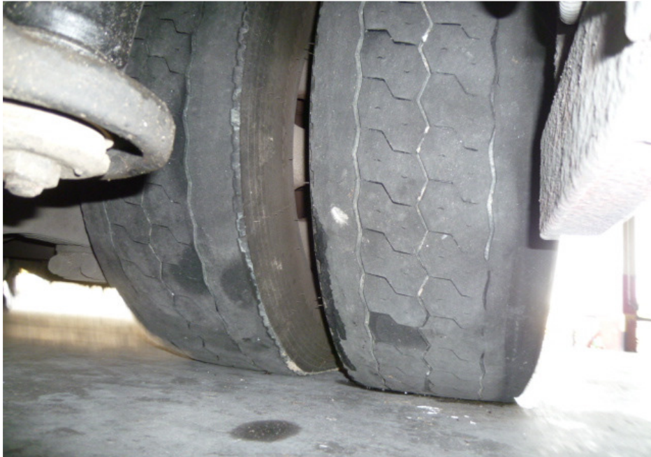
Photo 12 shows the condition of the rear left tyres of the Motor Bus, which were observed to be in serviceable condition with remaining tread depth of approximately 4mm. The tyres, which were wrapped around standard steel wheel rims, were also observed to be sufficiently inflated for vehicular operation. There was also no damage found on all 6 steel wheel rims of the Motor Bus.
