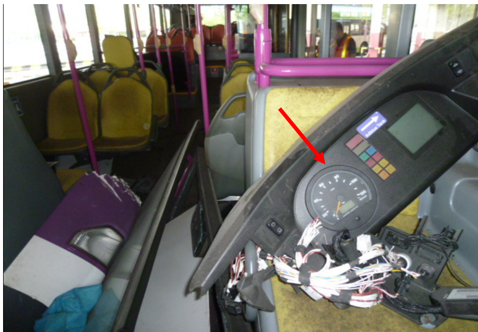
Photo 1 shows the dislodged instrument cluster (arrowed) as a result of the accident. Therefore no mileage could be recorded at the time of our inspection.
