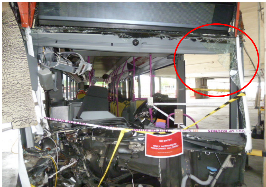
Photo 5 shows a close up view of the frontal portion of the Motor Bus at the time of our inspection. The Motor Bus was observed to sustained damages at its frontal portion. Its front windscreen was shattered as a result of the accident (circled).
