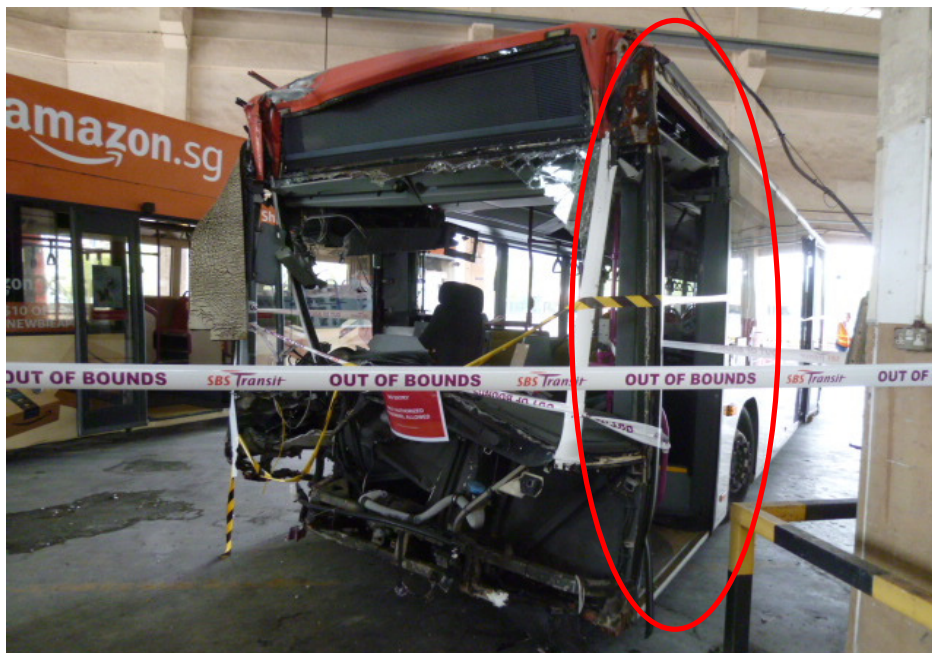
Photo 7 shows a close up of the left frontal portion of the Motor Bus at the time of our inspection. The Motor Bus was observed to sustained damage at its frontal portion. Its front door (circled) was damaged as a result of the accident.
