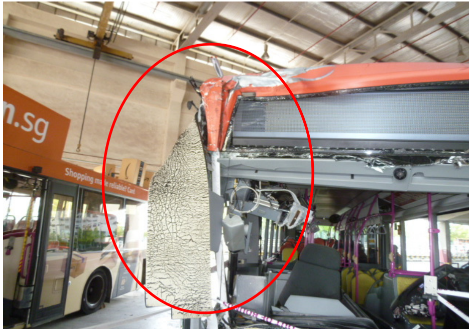
Photo 4 shows a close up view of the front body of the Motor Bus at the time of our inspection. The Motor Bus was observed to sustained damages at its frontal portion. Its front cabin structure (circled) was damaged as a result of the accident.
