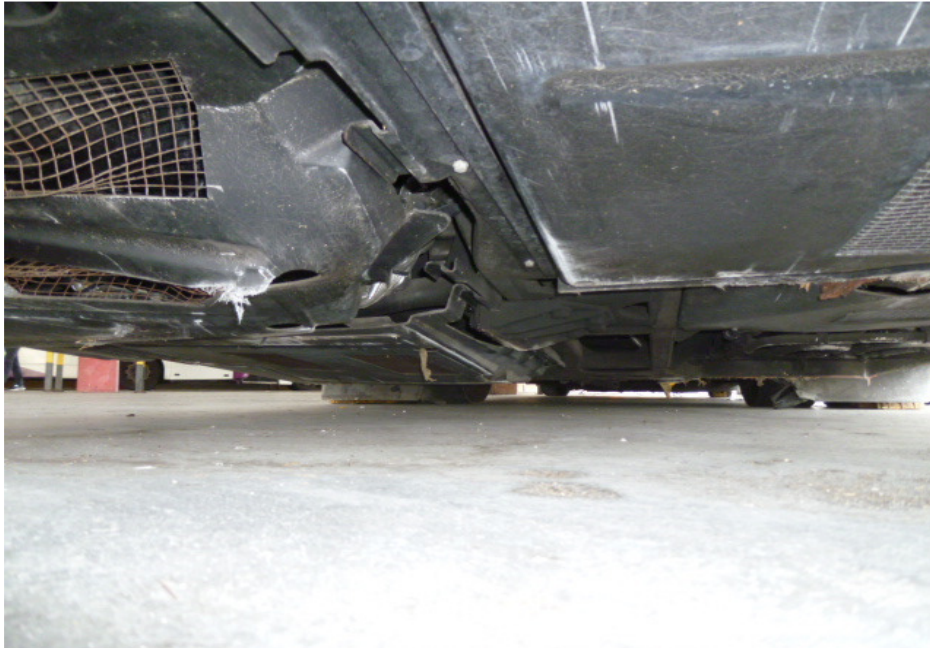
Photo 19 shows the undercarriage of the Motor Bus, at the area where the engine housing and transmission housing are located. We did not find any sign(s) or indication(s) of fluid leak and/or fluid stain(s) on the underside of the Motor Bus.
