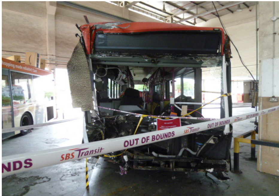
Photo 3 shows a general view of the frontal portion of the Motor Bus at the time of our inspection. The Motor Bus was observed to sustained damages at its frontal portion. Its front cabin structure, front windscreen, front bumper, front body panel and front door were damaged as a result of the accident.
