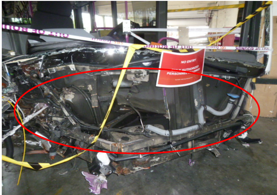
Photo 6 shows a close up view of the frontal portion of the Motor Bus at the time of our inspection. The Motor Bus was observed to sustained damage at its front portion. Its front bumper and front body panel (circled) were damaged as a result of the accident.
