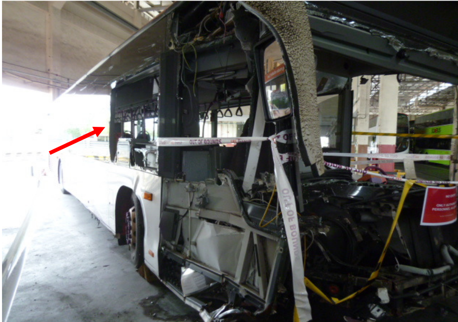
Photo 8 shows a close up view of the right body of the Motor Bus at the time of our inspection. The right portion of the Motor Bus was observed to have been unaffected by the accident. However, the windscreen was removed by the SCDF officers for rescue procedures (arrowed).
