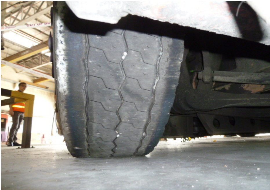
Photo 13 shows the condition of the front left tyre of the Motor Bus, which was observed to be in serviceable condition with remaining tread depth of approximately 10mm. There was also no tear, cut or burst mark(s) on the outer and the inner sidewalls as well as across the tread of the 6 tyres that were fitted on the Motor Bus.
