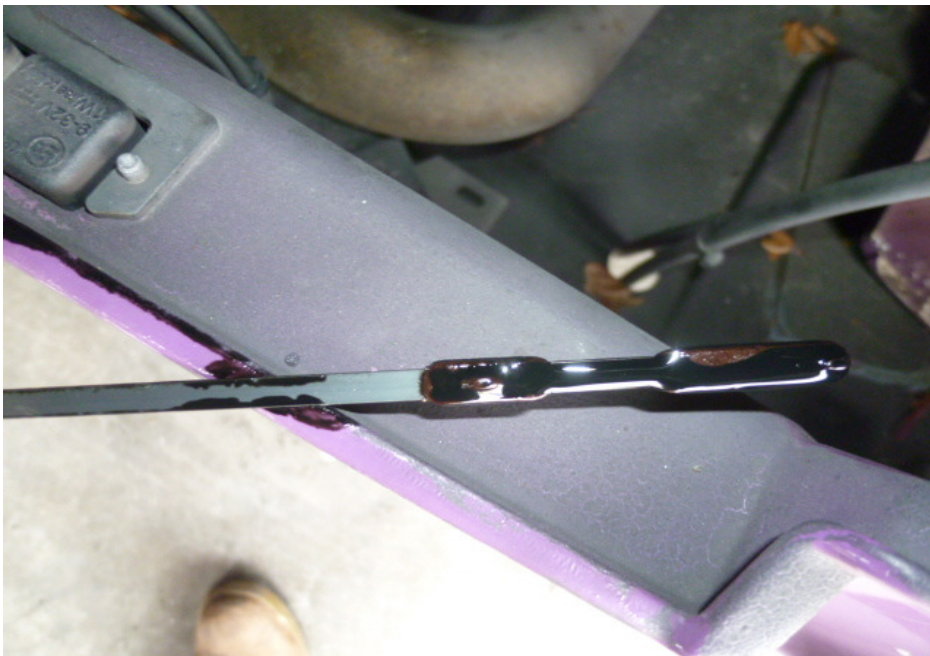
Photo 16 shows the engine oil dip stick system of the Motor Bus at the time of our inspection. The engine oil was observed to be of sufficient level for operating purposes and without any visible contamination.
