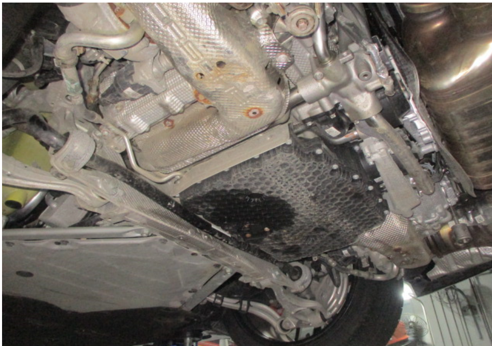
Photo 28 shows a general view of the Motor Car's engine compartment. The engine compartment was at the rear underside of the Motor Car. The various parts and components within the engine compartment were all observed to be intact and properly fitted. There was also no sign(s) or indication(s) of fluid leak and/or fluid stain found inside the engine compartment.
