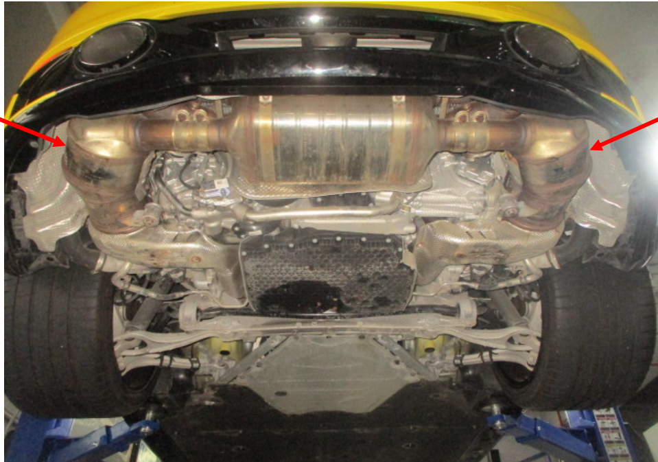
Photo 27 shows the Motor Car's exhaust system. My examination of the Motor Car's exhaust system revealed no sign(s) or indication(s) of any cut or weld marks along its exhaust pipes, on its catalytic converters (arrowed) and on its rear muffler.
