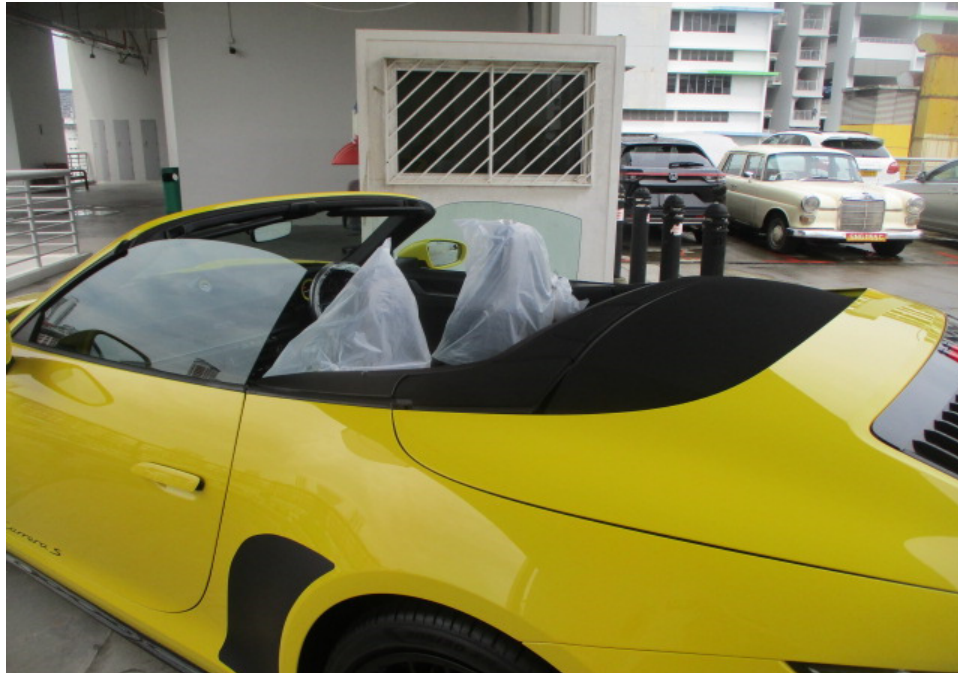
Photo 19 shows the Motor Car with its soft top roof completely folded. It was observed that as a safety feature, the soft top roof could only open and close when the Motor Car was in a stationary position or at low travelling speed. When opened, the soft top roof is completely folded into the rear compartment with no parts protruding out of the Motor Car's body. The soft top roof was also found adequately secured to the "A" pillar after closing.
