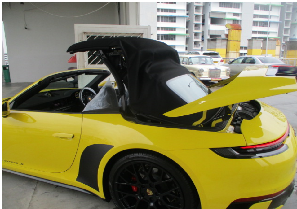
Photo 18 shows the Motor Car's soft top roof being tested. It was observed that as a safety feature, the soft top roof could only open and close when the Motor Car was in a stationary position or at low travelling speed. When opened, the soft top roof is completely folded into the rear compartment with no parts protruding out of the Motor Car's body. The soft top roof was also found adequately secured to the "A" pillar after closing.
