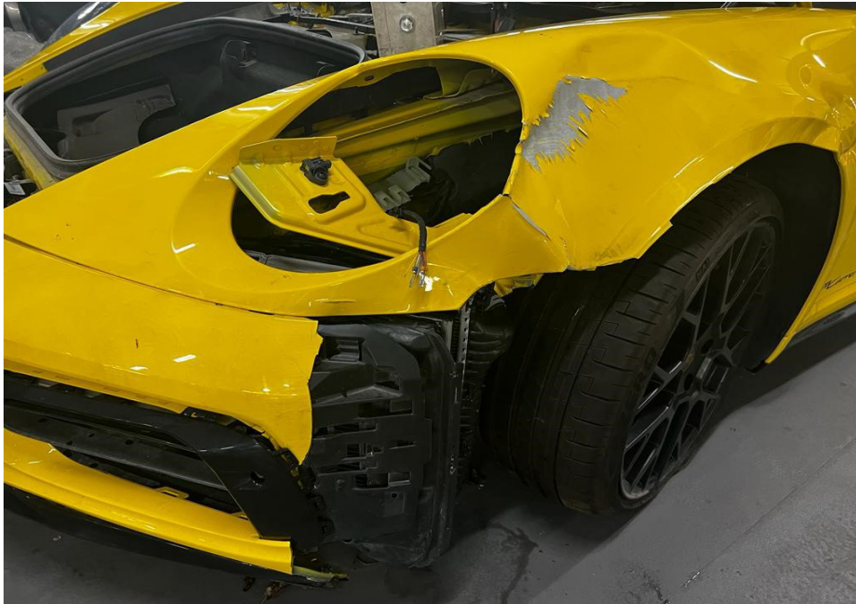
Photo 3 shows a closer view of the Motor Car's damaged front bumper, front bumper left lower grille, front bumper left bracket, front left day light, front left headlamp, front left fender and front left fender inner shield (photograph provided to me).
