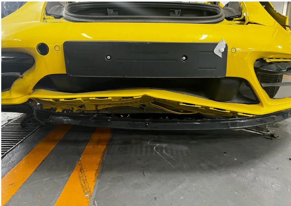
Photo 2 shows a closer view of the Motor Car's damaged front bumper, front bumper lower lip, front bumper right lower grille, front bumper left lower grille, front bumper centre air guide and front left day light (photograph provided to me).
