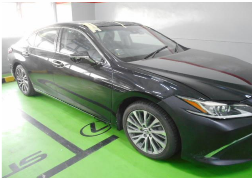
Photo 10 shows the right view of the Insured Vehicle at the time of our inspection. The exterior body of the Insured Vehicle was affected by the heat. Damages to its right side would be its rear-view mirror, all its plastic door handles and plastic door panels.
