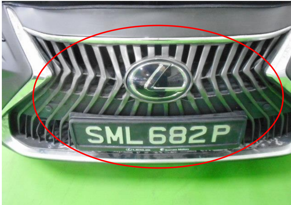
Photo 8 shows the general view of the front of the Insured Vehicle at the time of our inspection. The plastic front grille (circled) had sustained heat damage and melted as a result of the fire.
