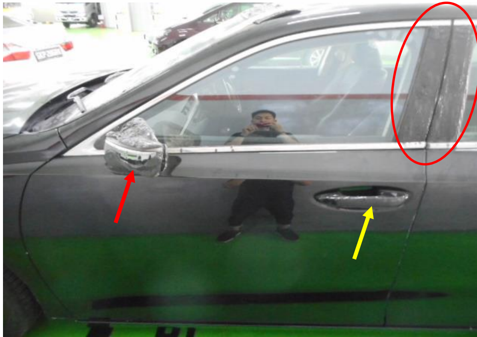
Photo 18 shows the left view of the Insured Vehicle at the time of our inspection. The exterior body of the Insured Vehicle was affected by the heat. Damages to its left side would be its rear-view mirror (red arrow), all its plastic door handles (yellow arrow) and plastic door panels (circled).
