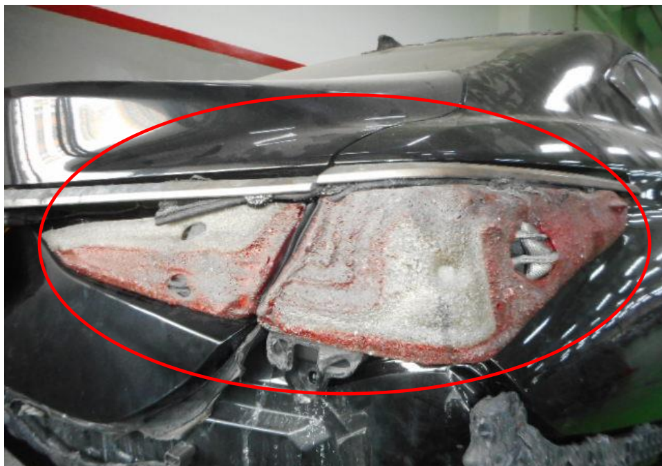
Photo 27 shows the rear view of the Insured Vehicle at the time of our inspection. The exterior body of the Insured Vehicle was affected by the heat. Damages to its rear portion would be its rear right brake lamp (circled).
