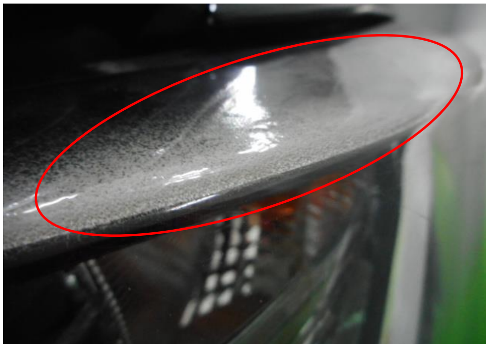
Photo 7 shows the close up view of the front of the Insured Vehicle at the time of our inspection. The front left plastic headlamp (circled) had sustained heat damage and melted as a result of the fire.
