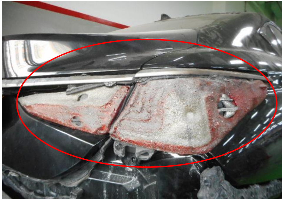
Photo 26 shows the rear view of the Insured Vehicle at the time of our inspection. The exterior body of the Insured Vehicle was affected by the heat. Damages to its rear portion would be its rear right brake lamp (circled).
