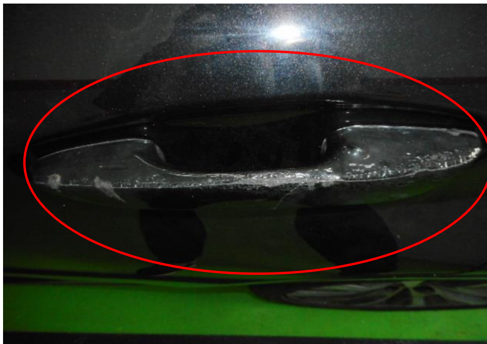
Photo 23 shows the left view of the Insured Vehicle at the time of our inspection. The exterior body of the Insured Vehicle was affected by the heat. Damages to its left side would be its plastic door handles (circled).
