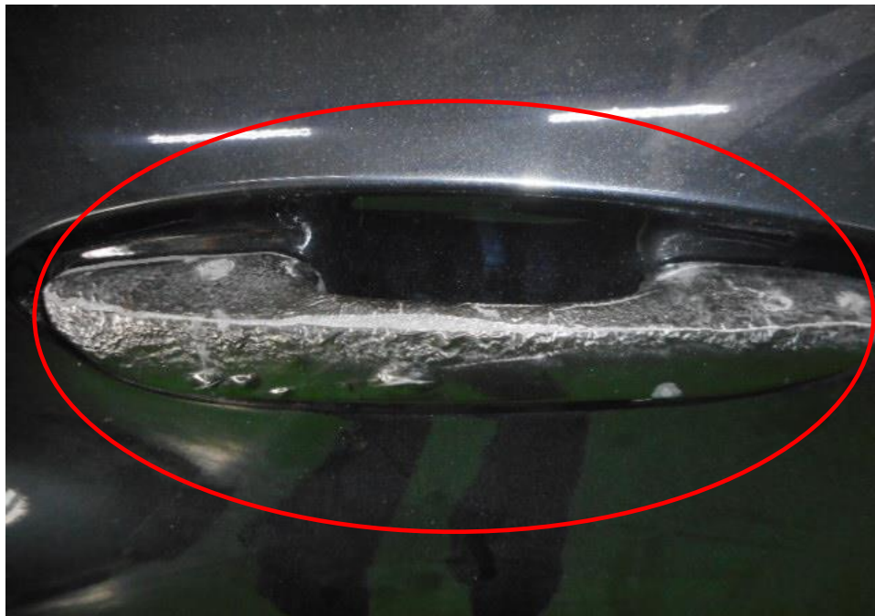
Photo 16 shows the right view of the Insured Vehicle at the time of our inspection. The exterior body of the Insured Vehicle was affected by the heat. Damages to its right side would be its plastic door handles (circled).
