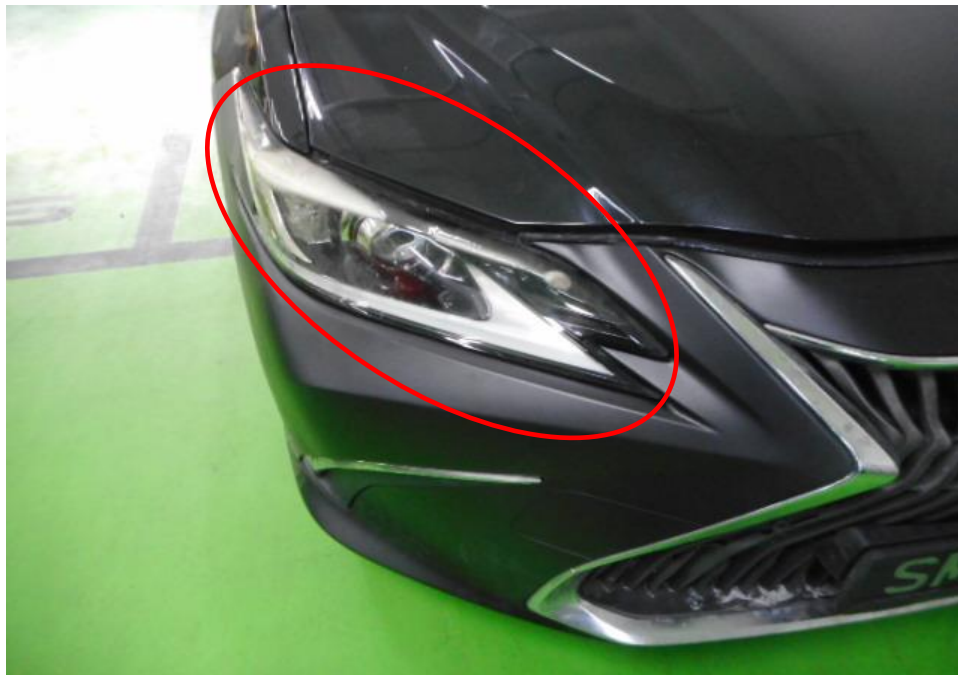
Photo 4 shows the general view of the front of the Insured Vehicle at the time of our inspection. The front right plastic headlamp (circled) had sustained heat damage and melted as a result of the fire.
