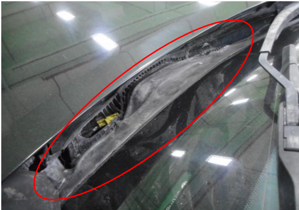
Photo 3 shows the close up view of the front of the Insured Vehicle at the time of our inspection. The front plastic water drain channel (circled) had sustained heat damage and melted as a result of the fire.
