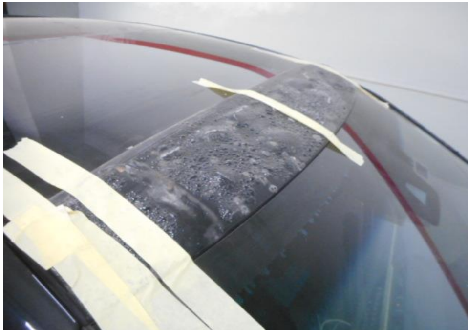
Photo 30 shows the roof view of the Insured Vehicle at the time of our inspection. The exterior body of the Insured Vehicle was affected by the heat. Damages to the roof portion would be the plastic roof panels.
