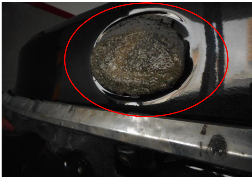
Photo 25 shows the rear view of the Insured Vehicle at the time of our inspection. The exterior body of the Insured Vehicle was affected by the heat. Damages to its rear portion would be its plastic vehicle emblem (circled).
