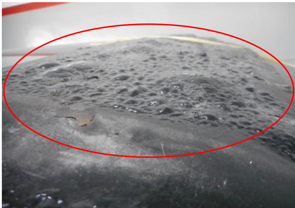
Photo 31 shows the roof view of the Insured Vehicle at the time of our inspection. The exterior body of the Insured Vehicle was affected by the heat. Damages to its roof portion would be its plastic roof panels (circled).
