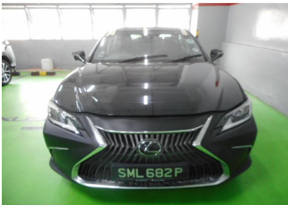
Photo 1 shows the front view of the Insured Vehicle at the time of our inspection. The exterior body of the Insured Vehicle was affected by the heat. Its front both plastic headlamps, plastic front grille, rubber weather seals and front plastic water drain channel had sustained heat damage as a result of the fire.
