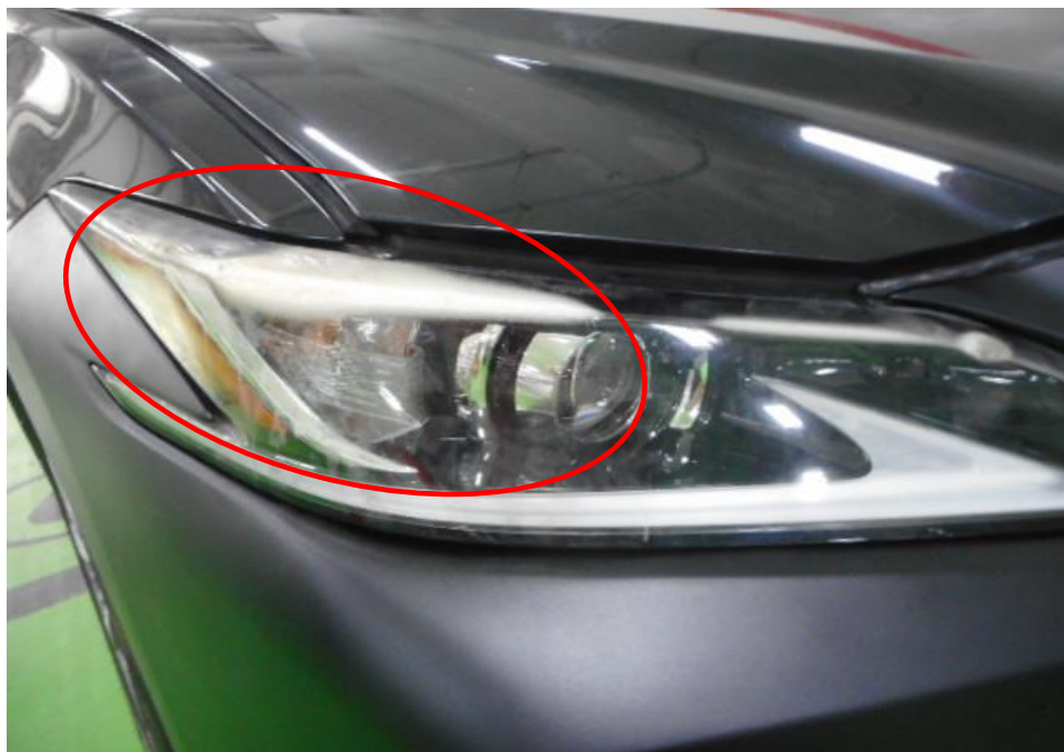
Photo 5 shows the close up view of the front of the Insured Vehicle at the time of our inspection. The front right plastic headlamp (circled) had sustained heat damage and melted as a result of the fire.
