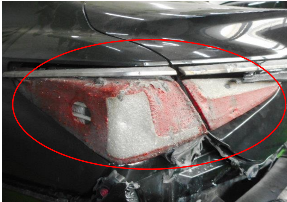
Photo 28 shows the rear view of the Insured Vehicle at the time of our inspection. The exterior body of the Insured Vehicle was affected by the heat. Damages to its rear portion would be its rear left brake lamp (circled).
