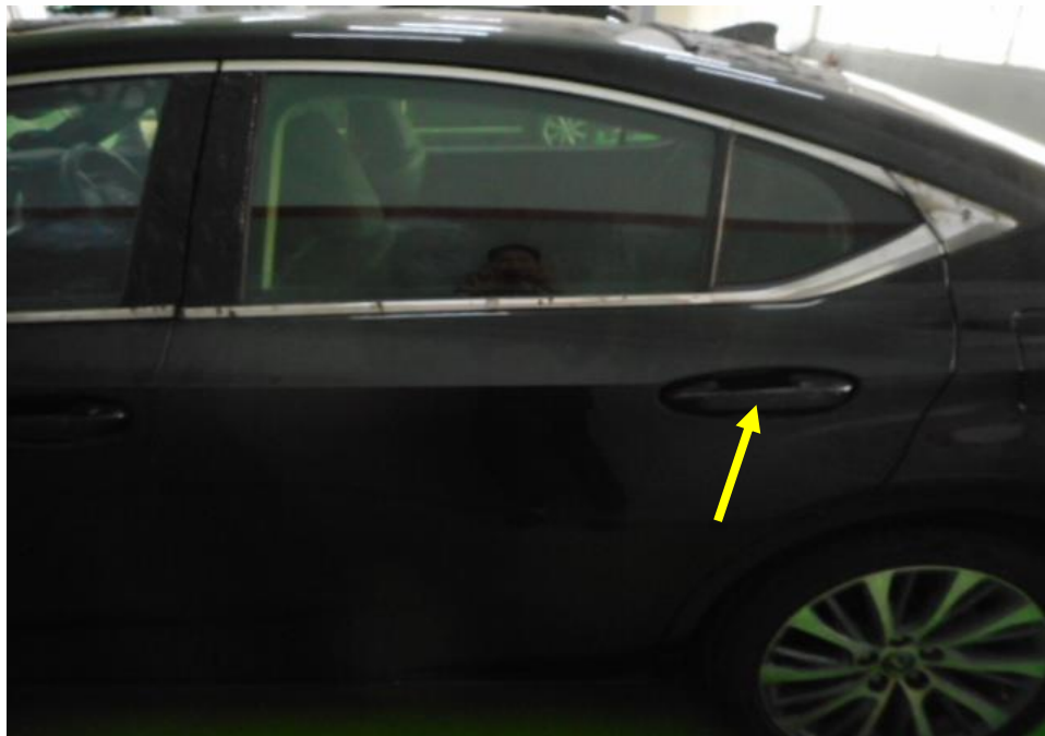
Photo 22 shows the left view of the Insured Vehicle at the time of our inspection. The exterior body of the Insured Vehicle was affected by the heat. Damages to its left side would be its door plastic handles (arrowed).
