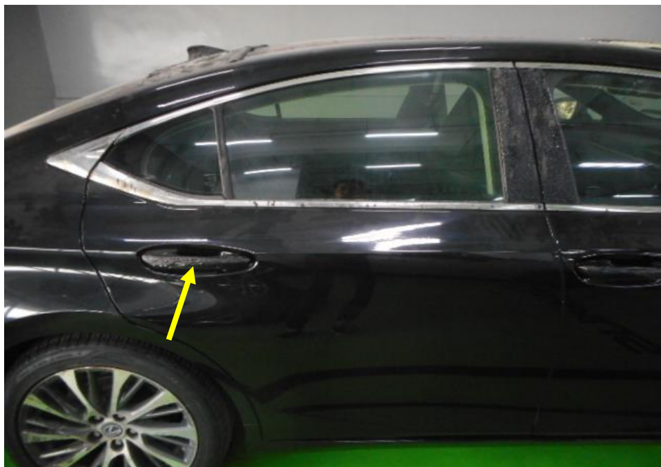
Photo 15 shows the right view of the Insured Vehicle at the time of our inspection. The exterior body of the Insured Vehicle was affected by the heat. Damages to its right side would be its plastic door handles (arrowed).
