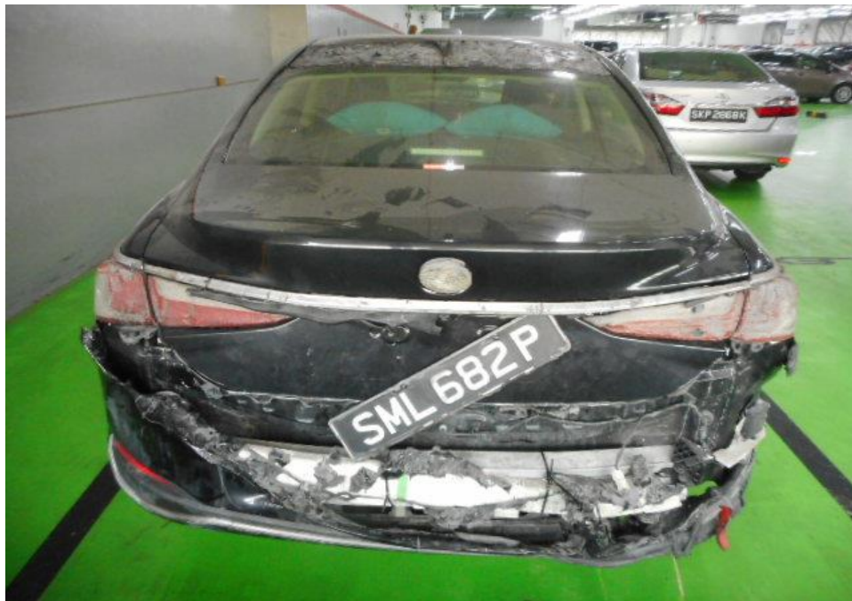
Photo 24 shows the rear view of the Insured Vehicle at the time of our inspection. The exterior body of the Insured Vehicle was affected by the heat. Damages to the rear portion would be both rear plastic brake lamps, rear plastic vehicle emblem and the rear plastic bumper.
