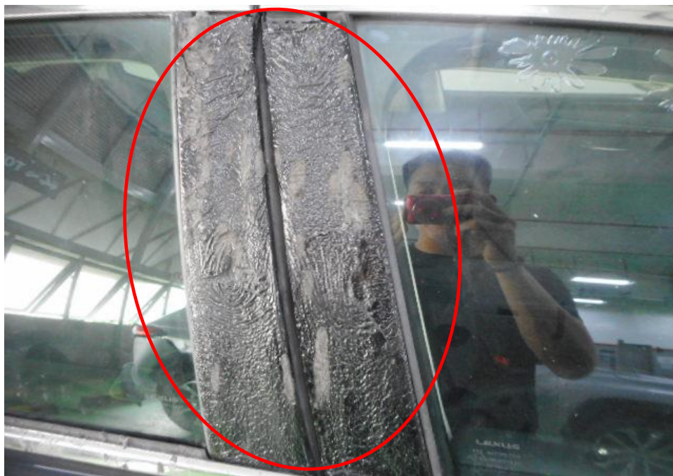
Photo 13 shows the right view of the Insured Vehicle at the time of our inspection. The exterior body of the Insured Vehicle was affected by the heat. Damages to its right side would be its plastic door panels (circled).
