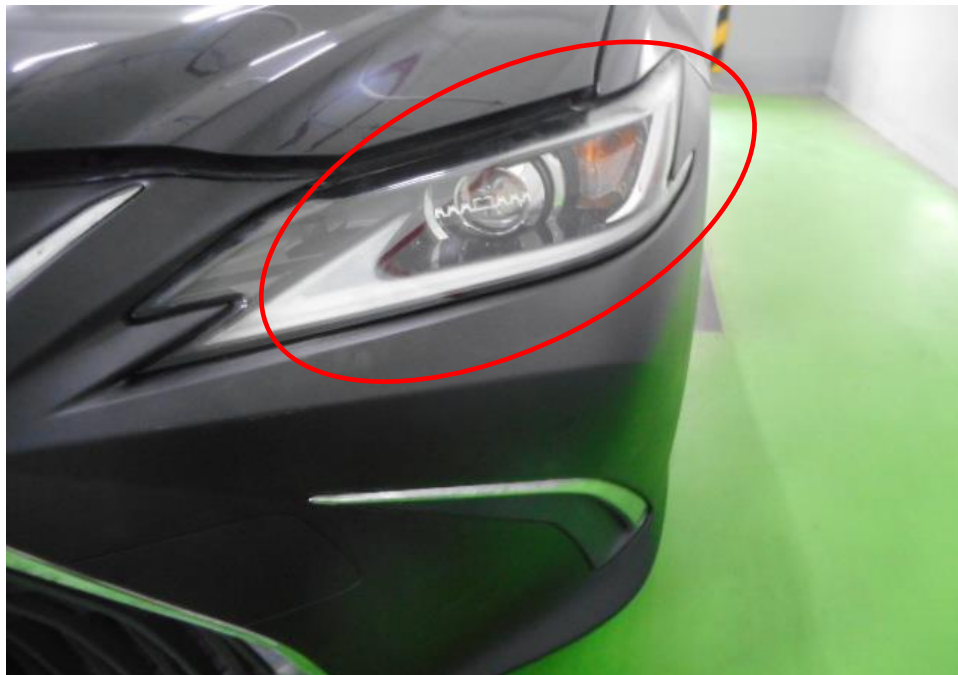
Photo 6 shows the general view of the front of the Insured Vehicle at the time of our inspection. The front left plastic headlamp (circled) had sustained heat damage and melted as a result of the fire.
