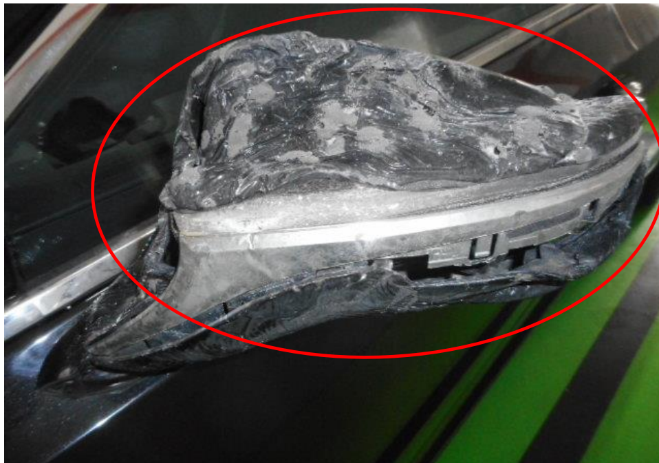
Photo 19 shows the left view of the Insured Vehicle at the time of our inspection. The exterior body of the Insured Vehicle was affected by the heat. Damages to its left side would be its rear view mirror (circled).
