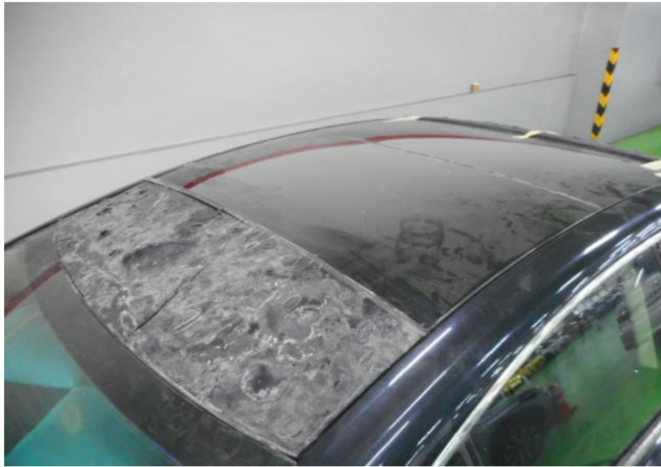
Photo 32 shows the roof view of the Insured Vehicle at the time of our inspection. The exterior body of the Insured Vehicle was affected by the heat. Damages to the roof portion would be the plastic roof panels.
