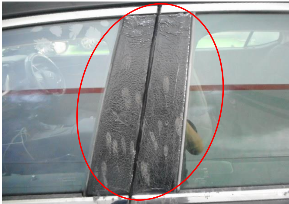
Photo 20 shows the left view of the Insured Vehicle at the time of our inspection. The exterior body of the Insured Vehicle was affected by the heat. Damages to its left side would be its plastic door panels (circled).
