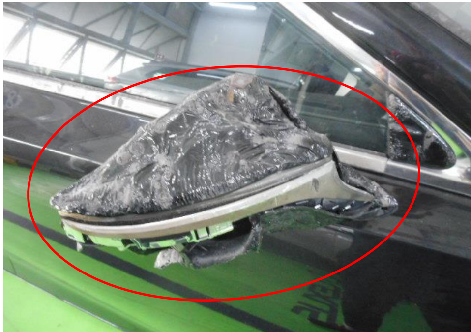
Photo 12 shows the right view of the Insured Vehicle at the time of our inspection. The exterior body of the Insured Vehicle was affected by the heat. Damages to its right side would be its rear view mirror (circled).
