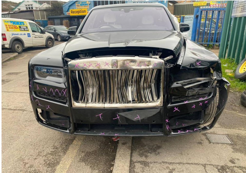
Photo 1 shows the frontal body of the Motor Car (photograph provided to me). The photographs provided to me had showed damage to the frontal portion of the Motor Car. The front bumper, front bumper centre lower garnish, front bumper centre lower grille, front bumper sensors, front bumper top cover, front radar unit, front grille and front emblem were amongst the body parts that were observed to have been damaged. The Motor Car's airbag(s) was not deployed.
