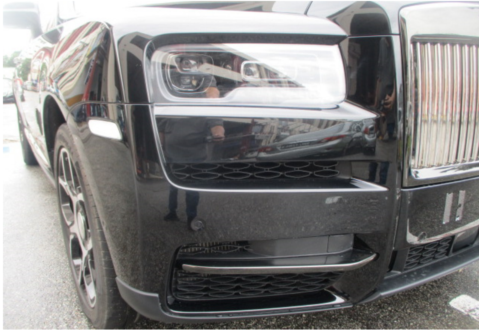
Photo 8 shows a closer view of the Motor Car's front bumper, front bumper right lower grille, front bumper right lower grille garnish, front bumper right sensors, front right signal lamp and front right headlamp. The body parts at the frontal portion of the Motor Car were visually examined and it was observed that the repair/restoration works carried out to the damaged area of the Motor Car (refer to photograph 1 - 3 above) were reasonably adequate and in order.
