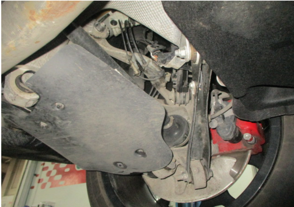
Photo 26 shows a general view of the control arms and linkages at the rear left wheel of the Motor Car. I did not observe any fluid leak and/or fluid stain on the underside of the Motor Car. All of the Motor Car's undercarriage components were observed to be intact and secured in an appropriate manner.
