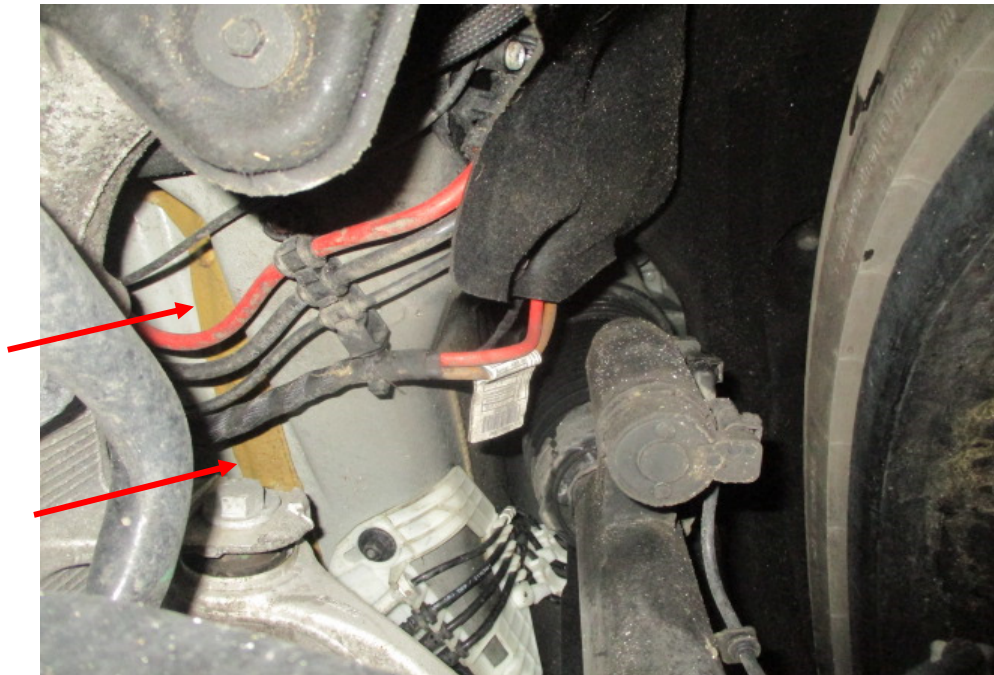
Photo 31 shows the chassis/structural body at the underside rear right of the Motor Car. I did not find any weld marks other than original spot weld marks on the chassis/structural body of the Motor Car. The original factory sealant (arrowed) at the joints along the chassis/structural body was untouched, indicating no work was done on the chassis/structural body of the Motor Car and that the chassis/structural body was originally fitted.
