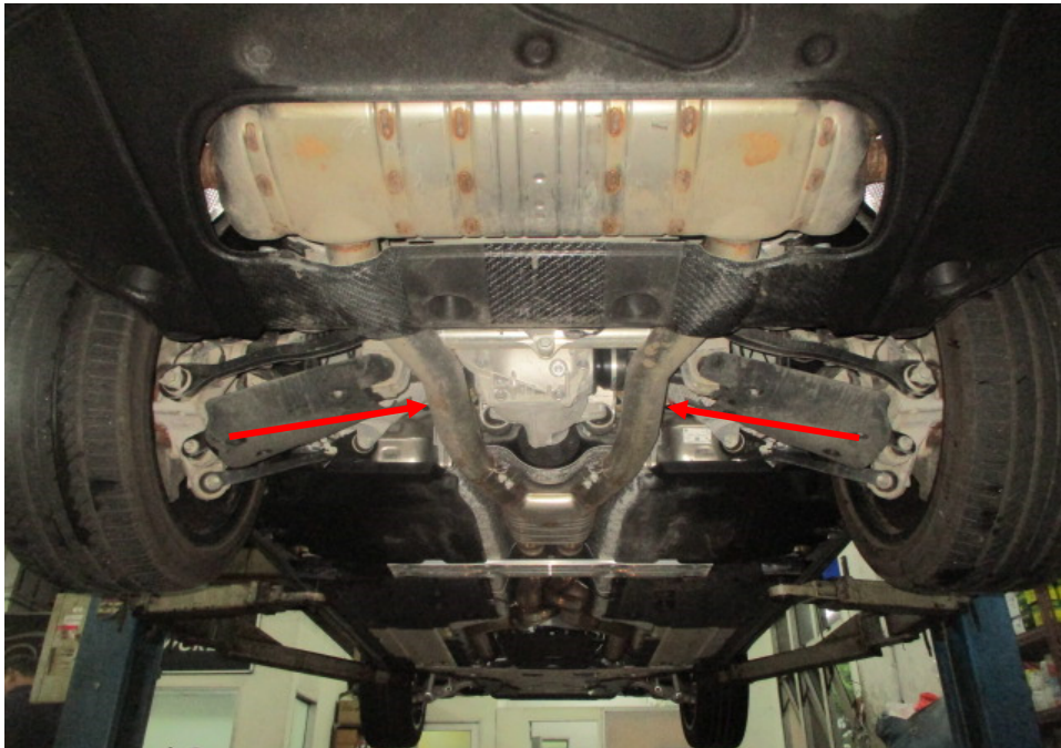
Photo 29 shows the rear section of the Motor Car's exhaust system. My examination of the Motor Car's exhaust system revealed no sign(s) or indication(s) of any cut or weld marks along its exhaust pipes (arrowed), on its rear muffler, on its centre resonator boxes and on its catalytic converters.
