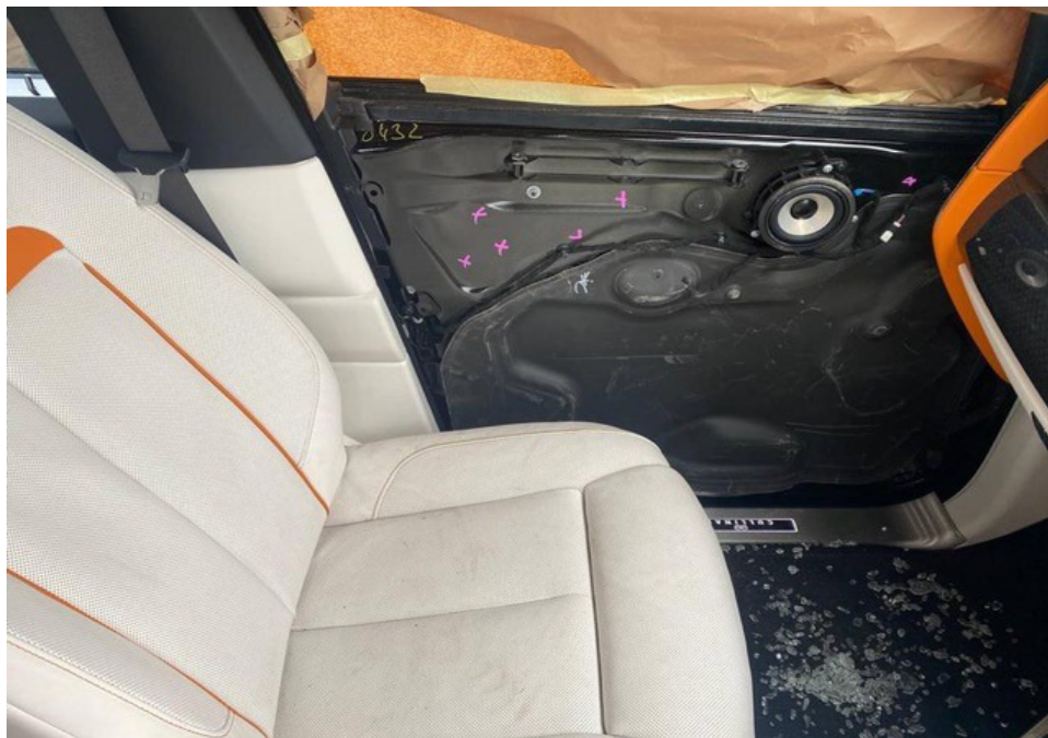
Photo 6 shows the Motor Car's front left door window shattered and its front left door inner trimboard missing/dislodged/damaged (photograph provided to me).
