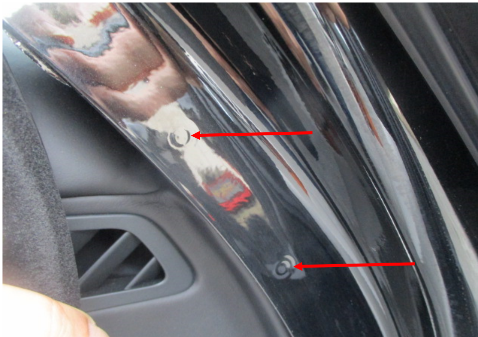
Photo 37 shows the right side "A" pillar of the Motor Car. I did not find any weld marks other than original spot weld marks (arrowed) on the right side "A" pillar of the Motor Car, which indicates that there was no re-welding works carried out. In general, I had found all the non-detachable body panels of the Motor Car to be originally fitted at the time of my inspection.
