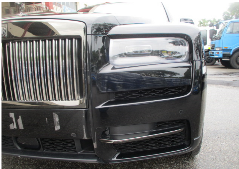
Photo 11 shows a closer view of the Motor Car's front bumper, front bumper right lower grille, front bumper right lower grille garnish and front right headlamp. The body parts at the frontal portion of the Motor Car were visually examined and it was observed that the repair/restoration works carried out to the damaged area of the Motor Car (refer to photograph 1 - 3 above) were reasonably adequate and in order.
