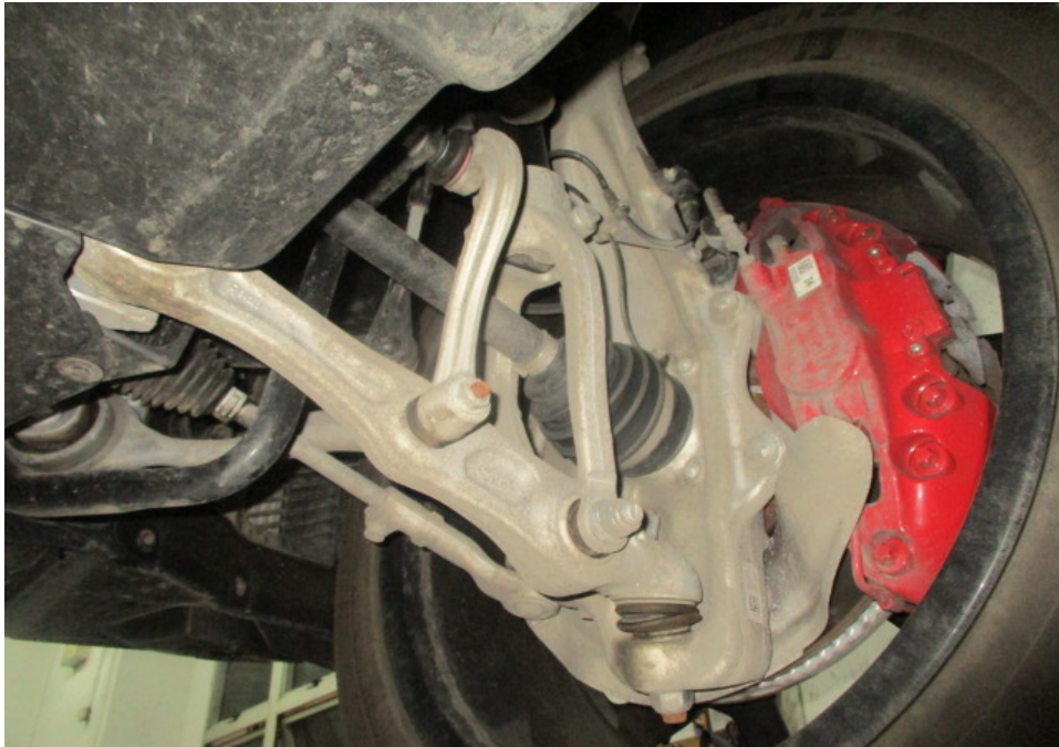
Photo 28 shows the various undercarriage components at the front right wheel of the Motor Car. The mechanical components, control arms and linkages were all found to be intact and secured in an appropriate manner. I also did not observe any fluid leak and/or fluid stain on the underside of the Motor Car.
