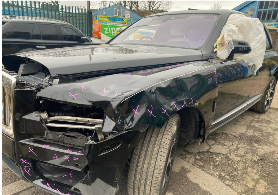
Photo 3 shows the front left body of the Motor Car (photograph provided to me). The photographs provided to me had showed damage to the frontal portion of the Motor Car. The front bumper, front bumper left lower grille, front bumper left lower grille garnish, front bumper left signal lamp, front bumper sensors, front left headlamp and front left fender were amongst the body parts that were observed to have been damaged. The Motor Car's airbag(s) was not deployed.
