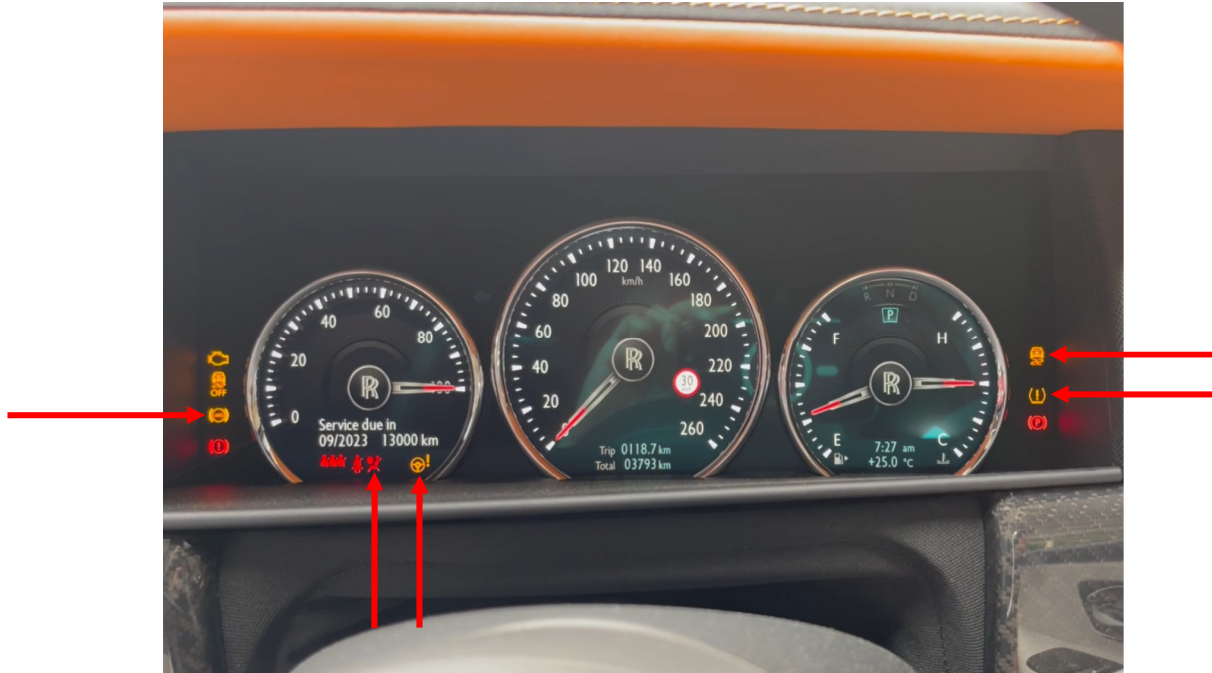
Photo 22 shows the warning lights for the various electronic safety features appearing on the instrument panel of the Motor Car during its self-test when the engine is cranked, in particular the ABS, SRS, EPS, TPM and TCS lights (arrowed).
