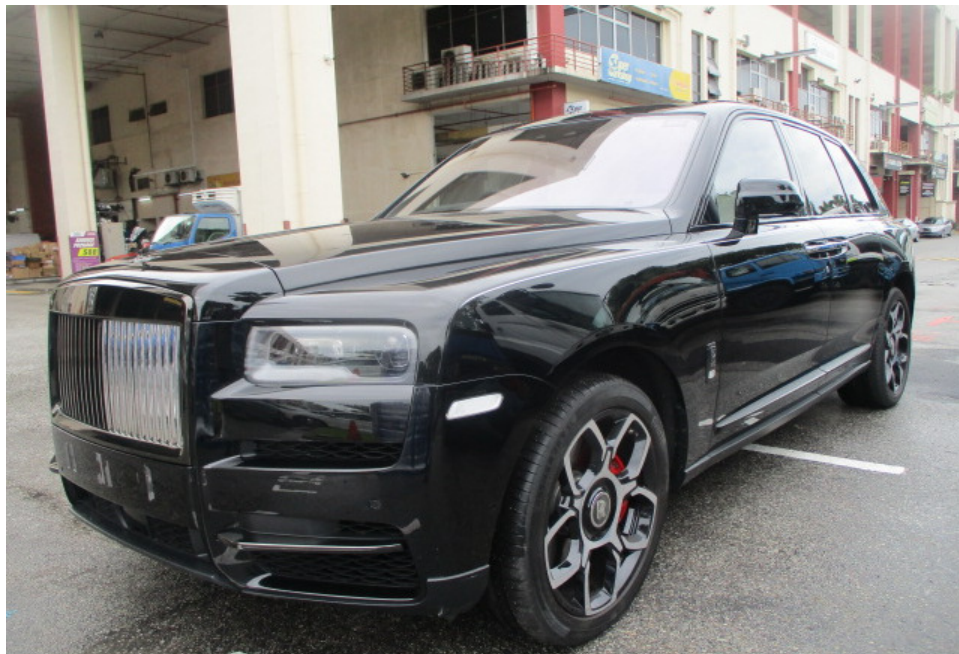
Photo 9 shows a general view of the front left body of the Motor Car at the time of my inspection. The Motor Car was observed to be in a relatively good general condition with no loose exterior fittings observed. The body parts at the frontal portion of the Motor Car were visually examined and it was observed that the repair/restoration works carried out to the damaged area of the Motor Car (refer to photograph 1 - 3 above) were reasonably adequate and in order.
