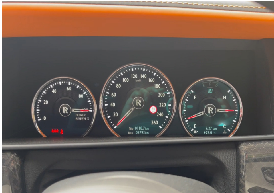
Photo 23 shows the respective warning lights no longer illuminated, indicating that there is no fault detected to the ABS, SRS, EPS, TPM and TCS systems of the Motor Car during the self-test. These electronic systems were hence in working condition at the time of my inspection.
