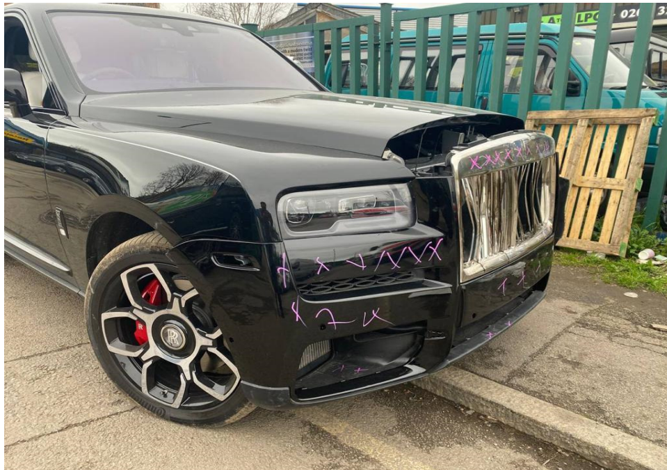
Photo 2 shows the front right portion of the Motor Car (photograph provided to me). The front bumper, front bumper right lower grille, front bumper right signal lamp, front bumper sensors, front bumper top cover, front grille and front emblem were amongst the body parts that were observed to have been damaged.
