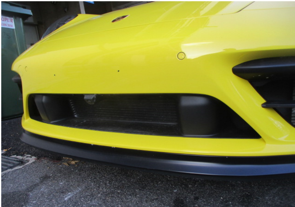
Photo 9 shows a closer view of the Motor Car's front bumper, front bumper lower lip, front bumper centre air guide and front bumper sensors. The body parts at the frontal portion of the Motor Car were visually examined and it was observed that the repair/restoration works carried out to the damaged area of the Motor Car (refer to photograph 1 & 2 above) were reasonably adequate and in order.
