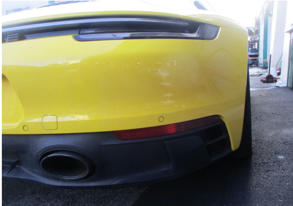
Photo 18 shows a closer view of the Motor Car's rear bumper, rear bumper lower cover, rear bumper right reflector, rear bumper sensors, rear bumper tow cover, rear right taillamp and rear right exhaust garnish. The body parts at the rear portion of the Motor Car were visually examined and it was observed that the repair/restoration works carried out to the damaged area of the Motor Car (refer to photograph 3 & 4 above) were reasonably adequate and in order.
