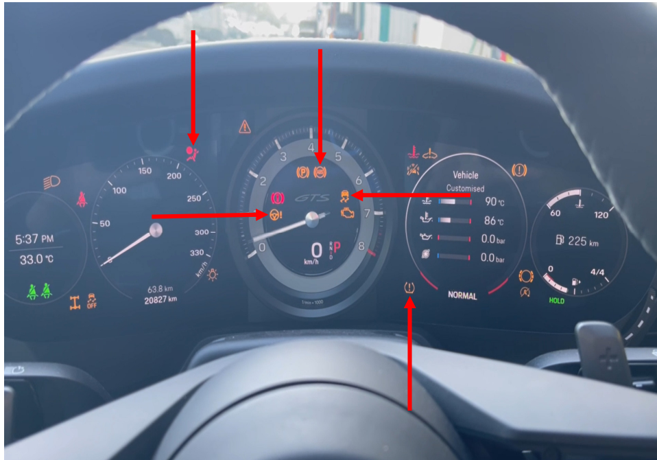
Photo 23 shows the warning lights for the various electronic safety features appearing on the instrument panel of the Motor Car during its self-test when the engine is cranked, in particular the ABS, SRS, EPS, TPM and TCS lights (arrowed).
