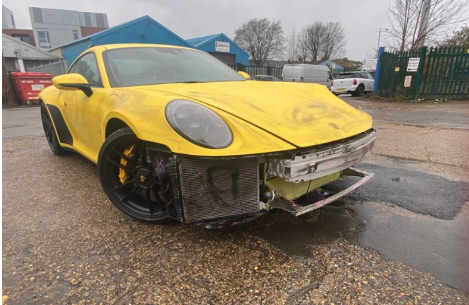
Photo 1 shows a general view of the front right body of the Motor Car (photograph provided to me). The Motor Car's front bumper and all its related parts and attachments like the front bumper lower lip, front bumper left lower grille, front bumper right lower grille, front bumper centre air guide, front bumper sensors, front left day light, front right day light, front left signal lamp and front right signal lamp amongst others, were also missing/dislodged/damaged.
