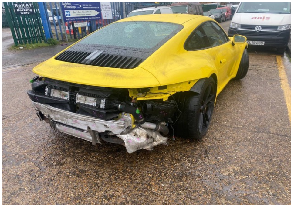
Photo 4 shows the rear right body of the Motor Car (photograph provided to me). The Motor Car's rear right taillamp, rear centre lamp, rear bumper and all its related parts and attachments like the rear bumper lower cover, rear bumper right reflector, rear bumper sensors, rear bumper tow cover and rear right exhaust garnish amongst others, were missing/dislodged/damaged.
