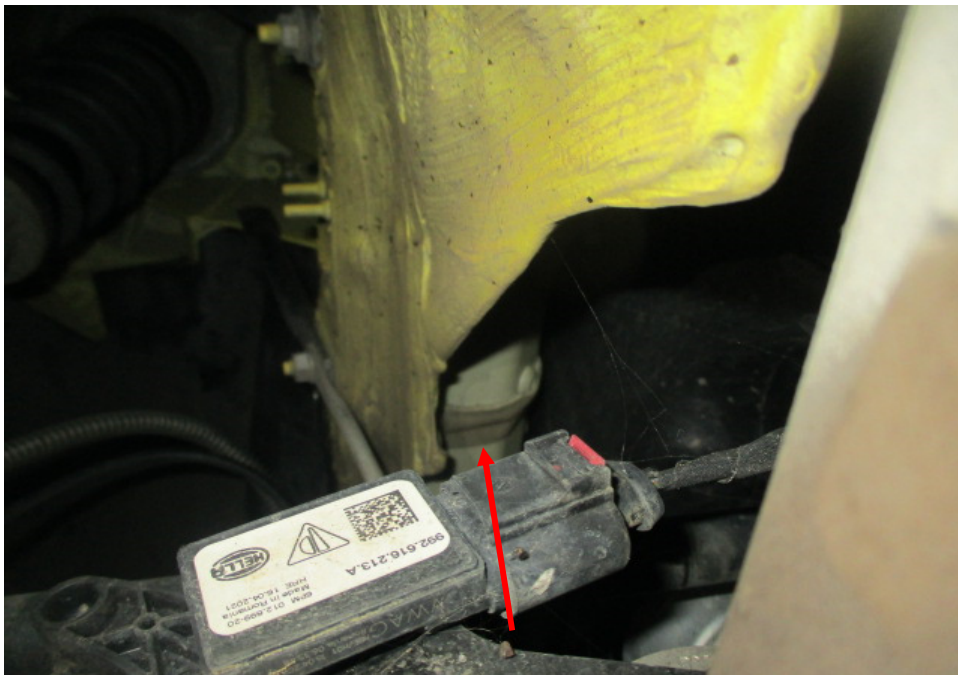
Photo 35 shows the chassis/structural body at the underside front left of the Motor Car. I did not find any weld marks other than original spot weld marks on the chassis/structural body of the Motor Car. The original factory sealant (arrowed) at the joints along the chassis/structural body was untouched, indicating no work was done on the chassis/structural body of the Motor Car and that the chassis/structural body was originally fitted.
