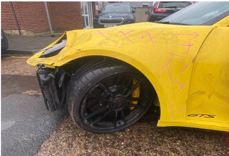
Photo 2 shows a closer view of the left front body of the Motor Car (photograph provided to me). The Motor Car's front left fender, front left fender inner shield and front left headlamp were damaged.
