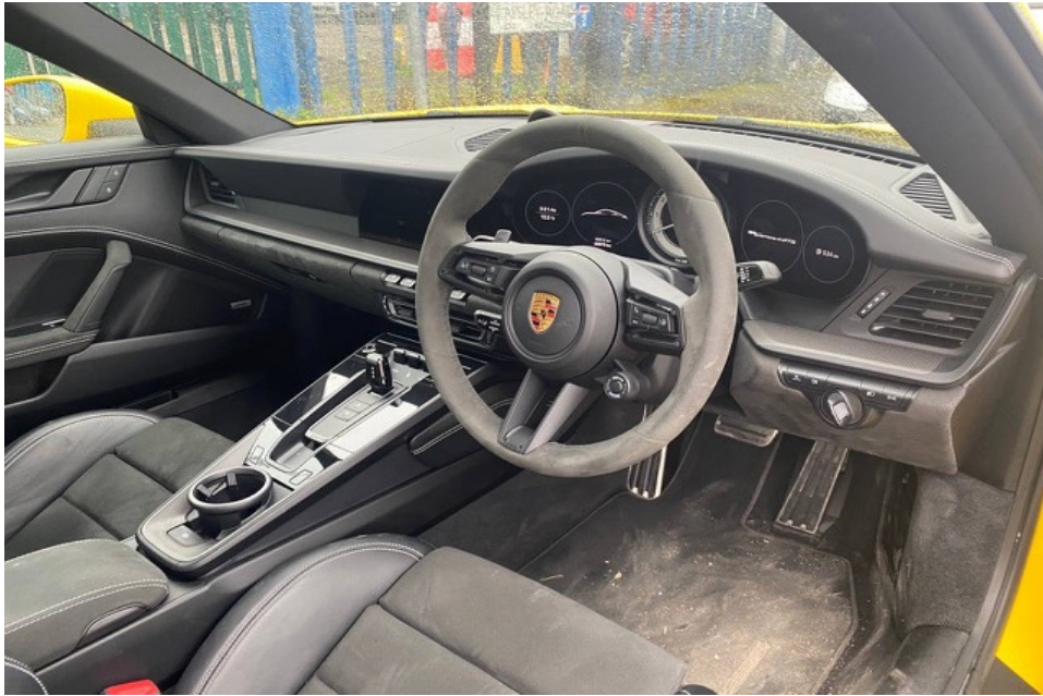
Photo 5 shows the interior compartment of the Motor Car (photograph provided to me). The various parts and components within the interior compartment were all intact and unaffected. The Motor Car's airbag(s) was not deployed as seen from the photographs that were provided to me.
