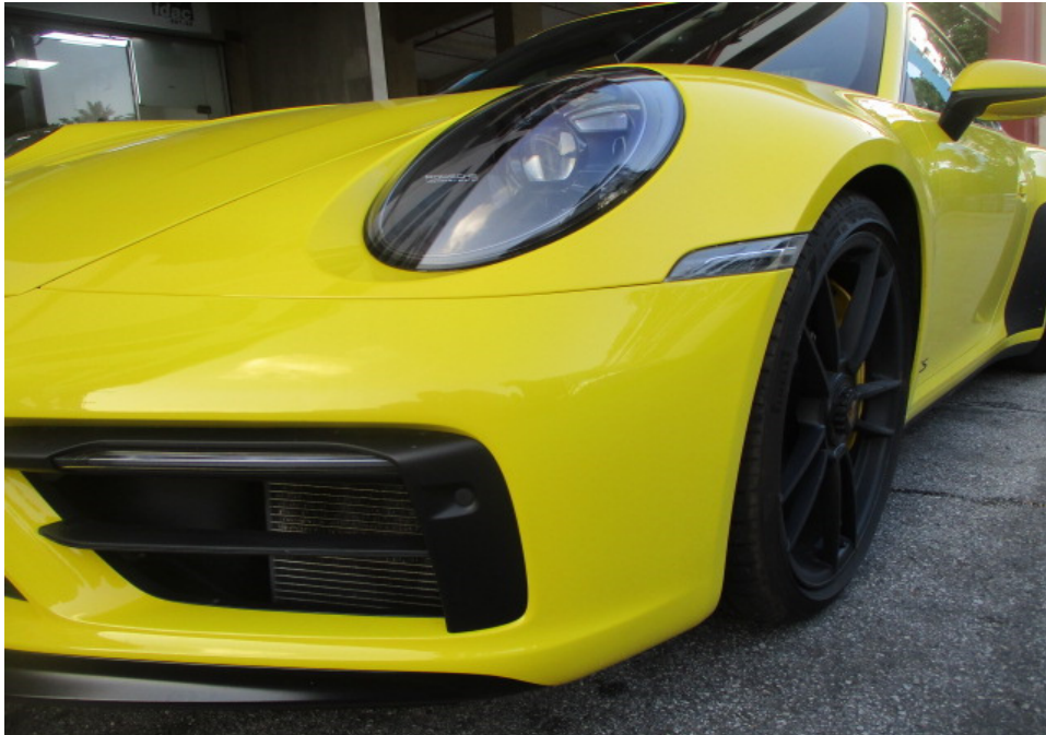
Photo 8 shows a closer view of the Motor Car's front bumper, front bumper left lower grille, front left day light, front left signal lamp and front left headlamp. The body parts at the frontal portion of the Motor Car were visually examined and it was observed that the repair/restoration works carried out to the damaged area of the Motor Car (refer to photograph 1 & 2 above) were reasonably adequate and in order.
