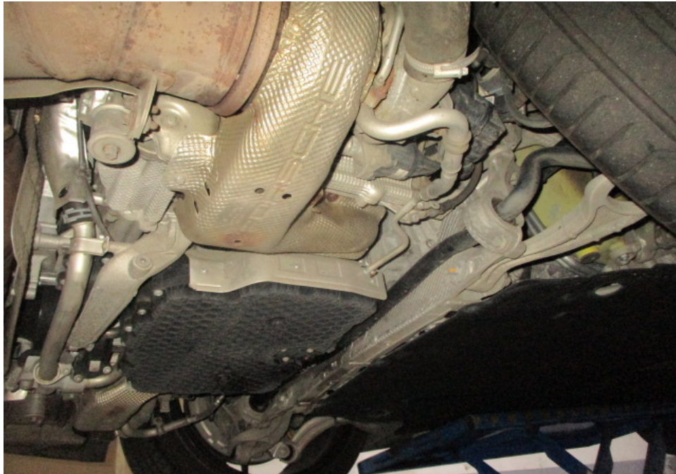
Photo 32 shows another view of the Motor Car's engine compartment. The engine compartment was at the rear underside of the Motor Car. The various parts and components within the engine compartment were all observed to be intact and properly fitted. There was also no sign(s) or indication(s) of fluid leak and/or fluid stain found inside the engine compartment.
