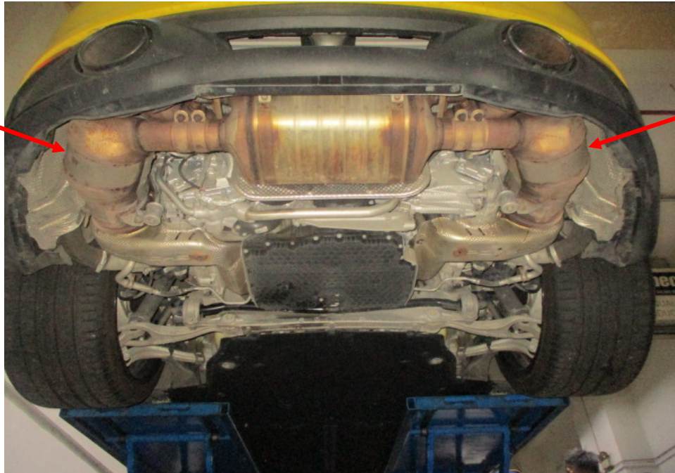
Photo 30 shows the Motor Car's exhaust system. My examination of the Motor Car's exhaust system revealed no sign(s) or indication(s) of any cut or weld marks along its exhaust pipes, on its catalytic converters (arrowed) and on its rear muffler.
