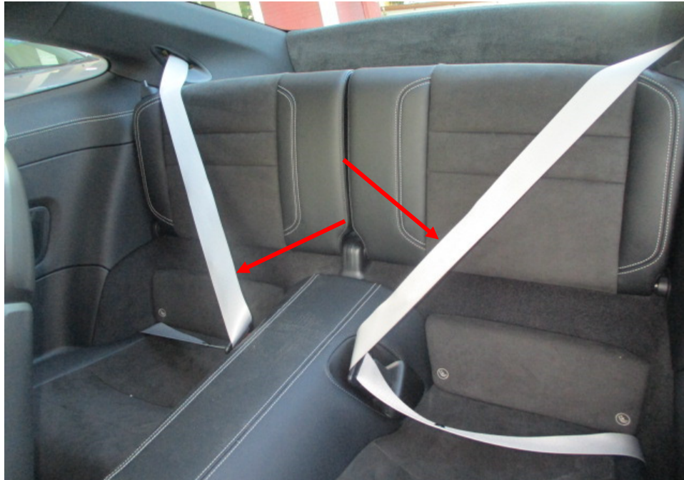
Photo 22 shows the rear seats of the Motor Car. All the seats of the Motor Car were secured via seat rails to the floorboard. They were also fitted with a retractable seat belt reel and a pre-tensioner. The seat belts (arrowed) were tested and were able to be fastened into the respective pre-tensions that were fitted on the side of each individual seat.
