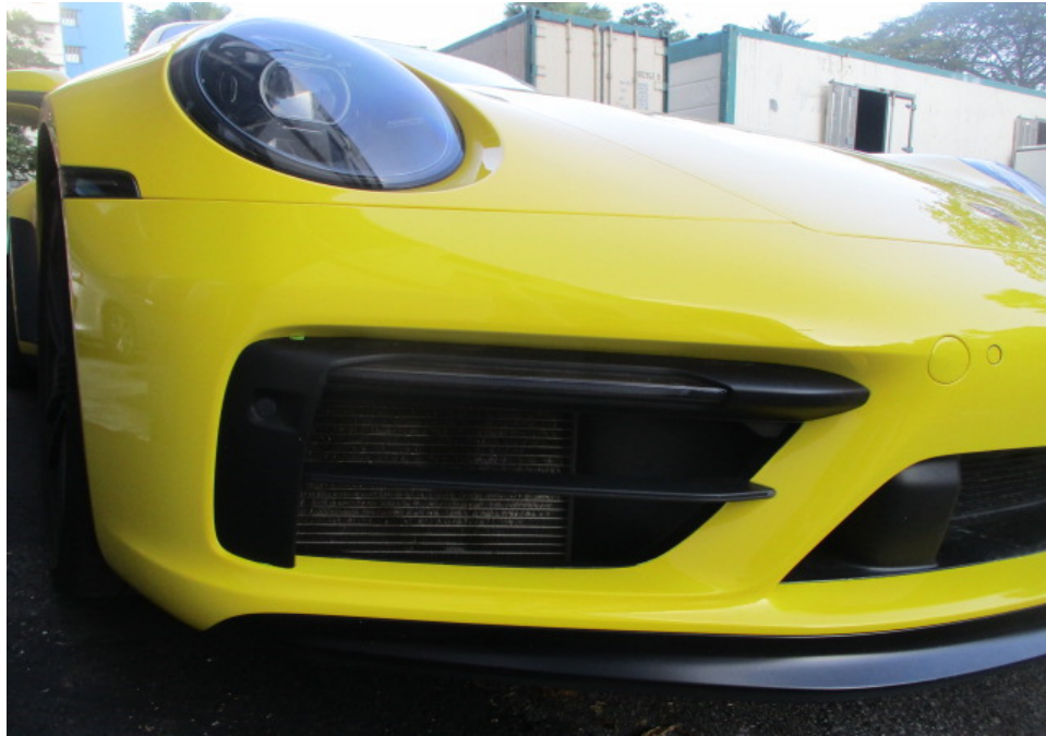
Photo 12 shows a closer view of the Motor Car's front bumper, front bumper lower lip, front bumper right lower grille, front right day light, front right signal lamp and front right headlamp. The body parts at the frontal portion of the Motor Car were visually examined and it was observed that the repair/restoration works carried out to the damaged area of the Motor Car (refer to photograph 1 & 2 above) were reasonably adequate and in order.
