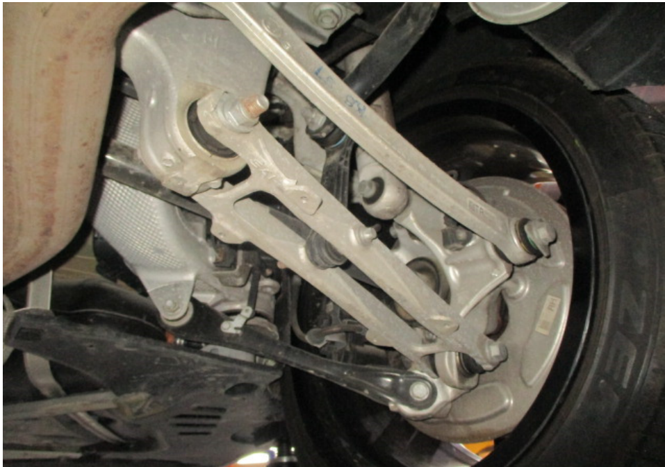
Photo 22 shows a general view of the control arms and linkages at the rear right wheel of the Motor Car. I did not observe any fluid leak and/or fluid stain on the underside of the Motor Car. All of the Motor Car's undercarriage components were observed to be intact and secured in an appropriate manner.
