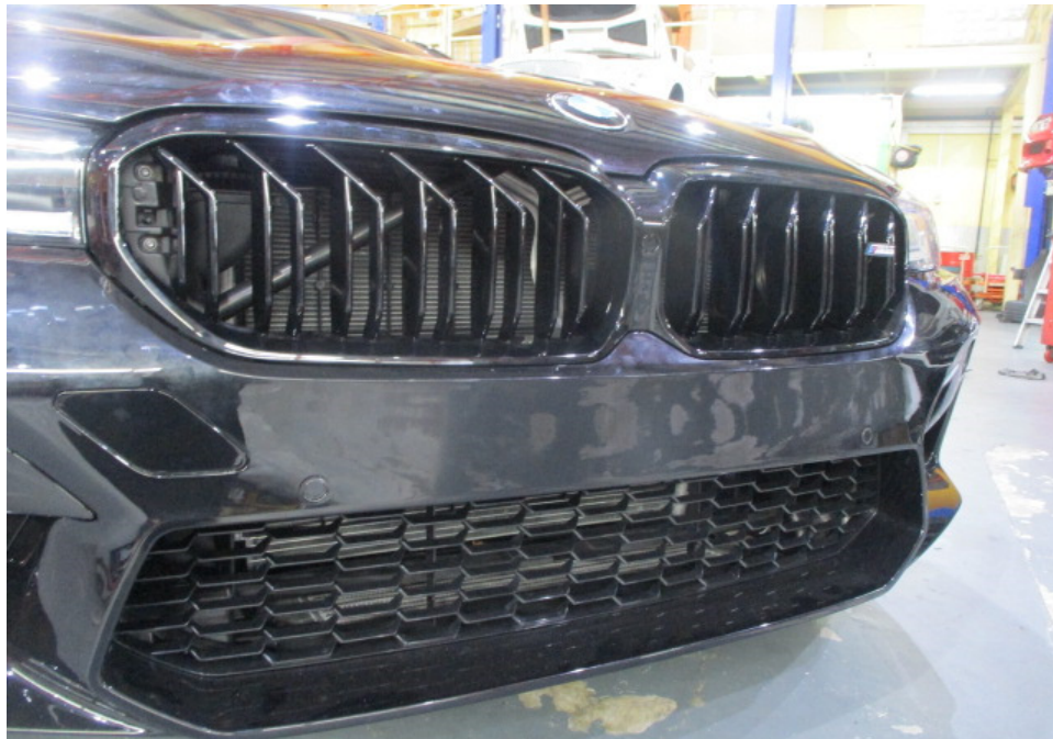
Photo 8 shows a closer view of the Motor Car's front bumper centre lower grille, front grilles, oil cooler and aircon condenser. The body parts at the frontal portion of the Motor Car were visually examined and it was observed that the repair/restoration works carried out to the damaged area of the Motor Car (refer to photograph 1 & 2 above) were reasonably adequate and in order.
