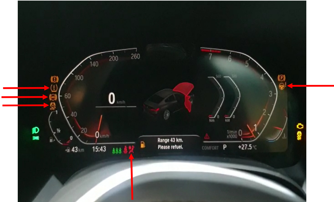
Photo 19 shows the warning lights for the various electronic safety features appearing on the instrument panel of the Motor Car during its self-test when the engine is cranked, in particular the ABS, SRS, IAS, TPM and DSC lights (arrowed).
