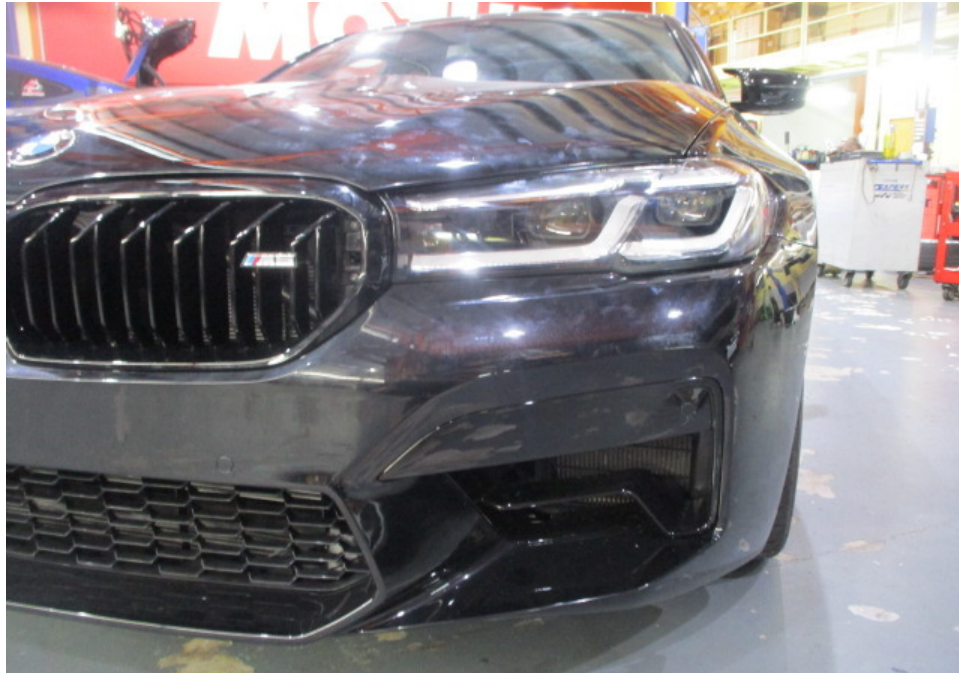
Photo 11 shows a closer view of the Motor Car's front bumper, front bumper left lower moulding, front bumper centre lower grille, front bumper left sensors, front left headlamp and front bonnet. The body parts at the frontal portion of the Motor Car were visually examined and it was observed that the repair/restoration works carried out to the damaged area of the Motor Car (refer to photograph 1 & 2 above) were reasonably adequate and in order.
