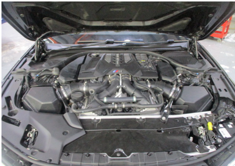
Photo 16 shows a general view of the engine compartment of the Motor Car at the time of my inspection. The various parts and components inside the engine compartment were all observed to be intact and properly fitted. There was also no sign(s) or indication(s) of fluid leak and/or fluid stain found inside the engine compartment. The repair/restoration works carried out to the various parts within the engine compartment like the front headlamp top panels, front centre top panel, front centre top panel garnish, front air guide, aircon condenser, radiator and cooling fan amongst others, were reasonably adequate and in order.
