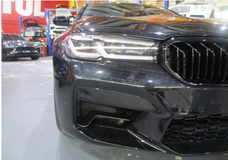
Photo 7 shows a closer view of the Motor Car's front bumper, front bumper right lower moulding, front bumper right sensors, front bumper tow cover, front right headlamp and front bonnet. The body parts at the frontal portion of the Motor Car were visually examined and it was observed that the repair/restoration works carried out to the damaged area of the Motor Car (refer to photograph 1 & 2 above) were reasonably adequate and in order.
