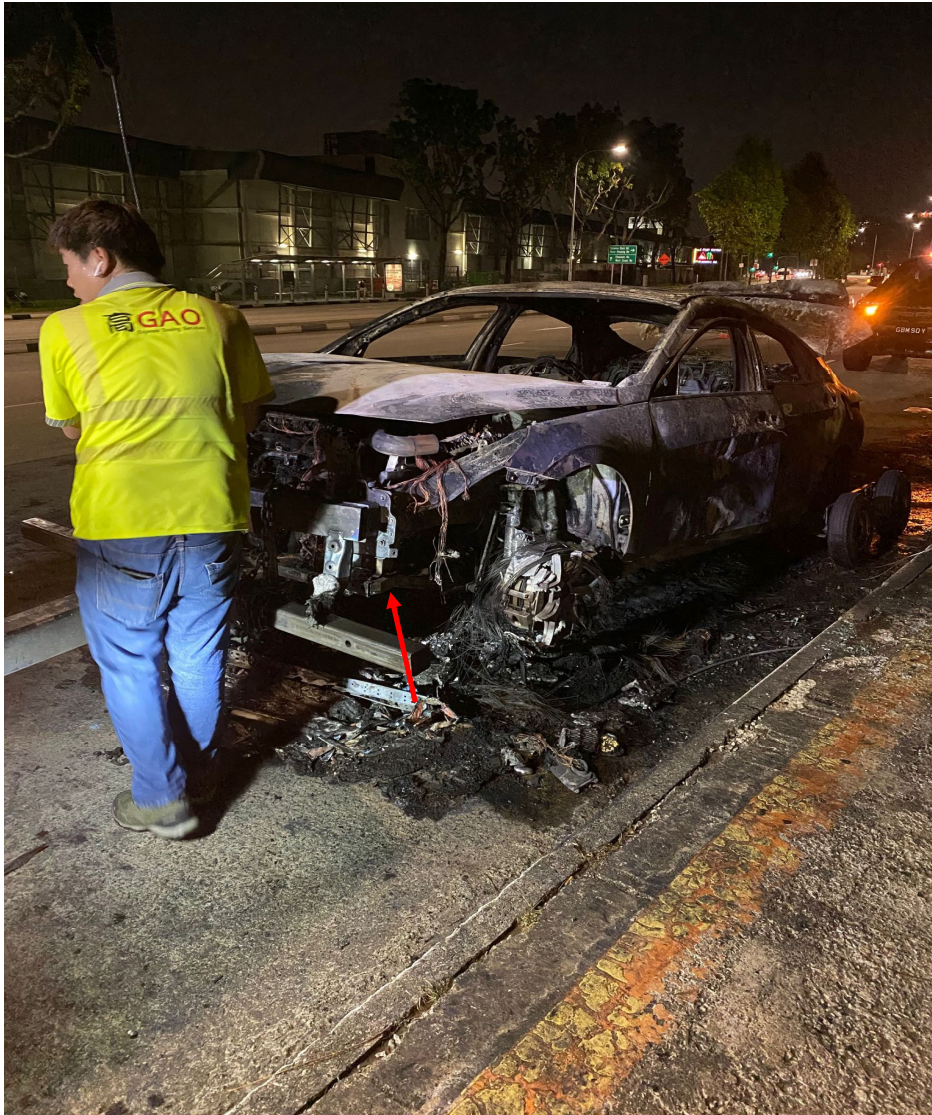
Photo 9 shows the Insured Vehicle being prepped to be towed to Cartimes post-incident. The severity of damage of the frontal portion had corresponded to the events that were related to us by Mr Tan, which is the fire had started from the engine compartment of the Insured Vehicle (arrowed).
