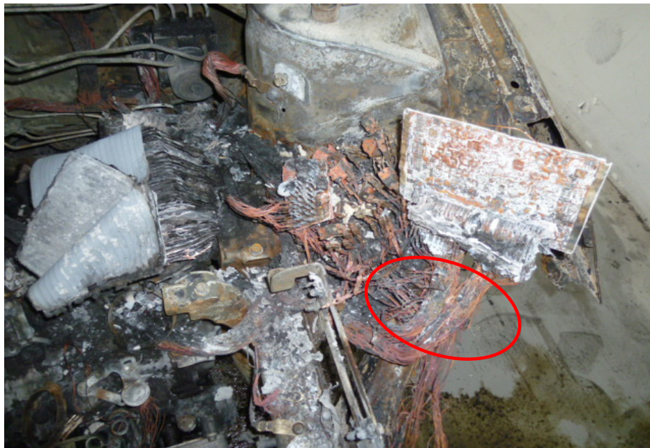
Photo 5 shows the factory fitted wirings around the left portion of the engine compartment which is near to the vicinity where the fire to the Insured Vehicle had likely started. We observed faint traces of greenish residue on some of these wirings (circled).
