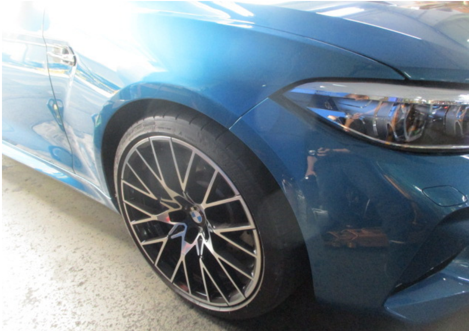
Photo 6 shows a closer view of the Motor Car's front bumper, front right headlamp, front right fender, front right wheel rim and front right tyre at the time of my inspection. The body parts at the front right portion of the Motor Car were visually examined and it was observed that the repair/restoration works carried out to the damaged area of the Motor Car (refer to photograph 1 above) were reasonably adequate and in order.
