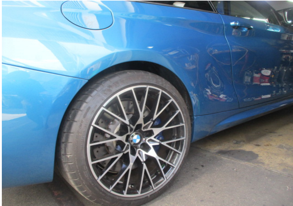
Photo 12 shows a closer view of the Motor Car's rear bumper, rear right fender, rear right wheel rim and right side rocker panel garnish. The body parts at the right rear portion of the Motor Car were visually examined and it was observed that the repair/restoration works carried out to the damaged area of the Motor Car (refer to photograph 2 above) were reasonably adequate and in order.
