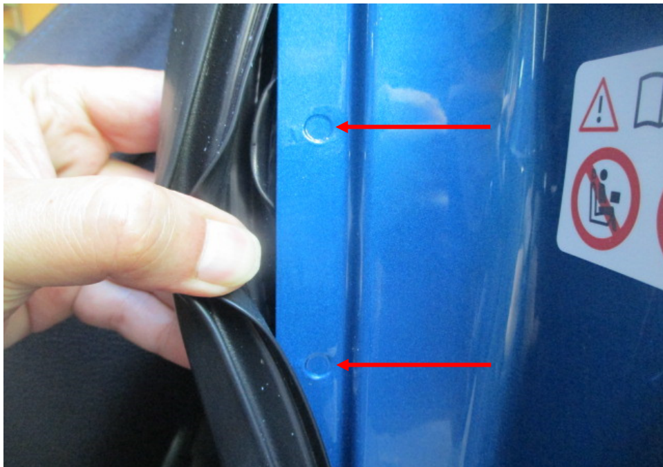
Photo 31 shows the left side rear body panel of the Motor Car. I did not find any weld marks other than original spot weld marks (arrowed) on the left side rear body panel of the Motor Car, which indicates that there was no re-welding works carried out. In general, I had found all the non-detachable body panels of the Motor Car to be originally fitted at the time of my inspection.
