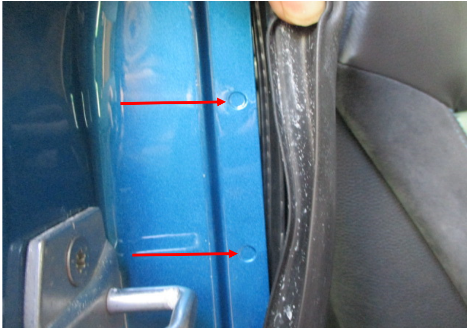
Photo 34 shows the right side rear body panel of the Motor Car. I did not find any weld marks other than original spot weld marks (arrowed) on the right side rear body panel of the Motor Car, which indicates that there was no re-welding works carried out. In general, I had found all the non-detachable body panels of the Motor Car to be originally fitted at the time of my inspection.
