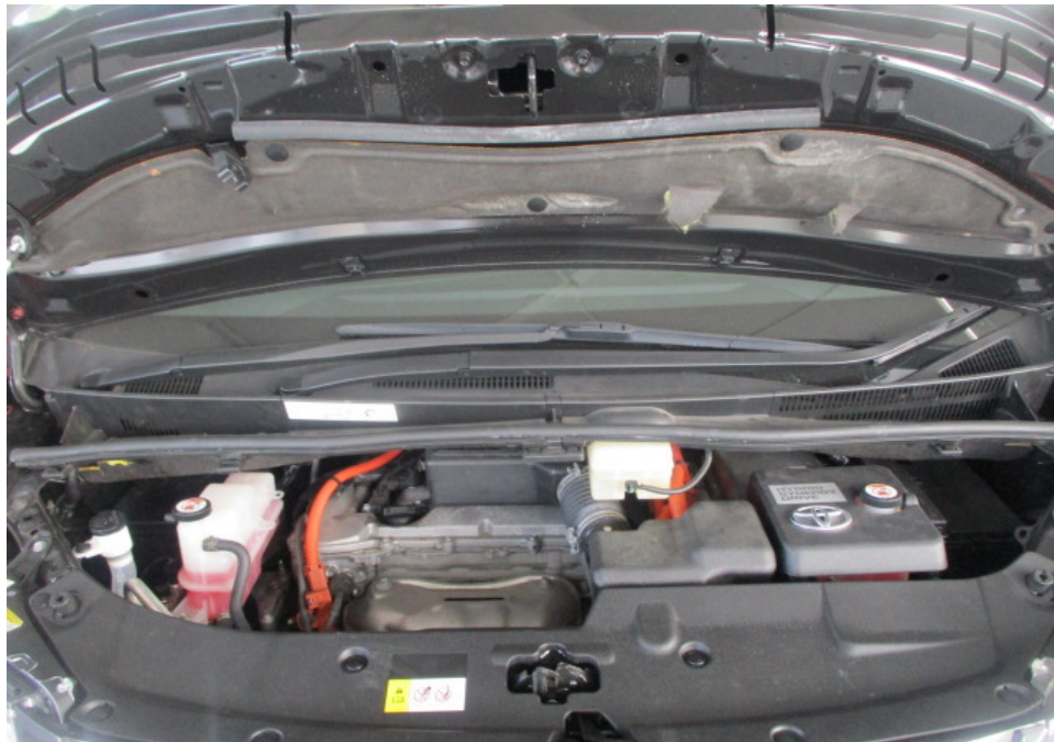
Photo 13 shows a general view of the engine compartment of the Motor Car at the time of my inspection. The various parts and components inside the engine compartment were all observed to be intact and properly fitted. There was also no sign(s) or indication(s) of fluid leak and/or fluid stain found inside the engine compartment.
