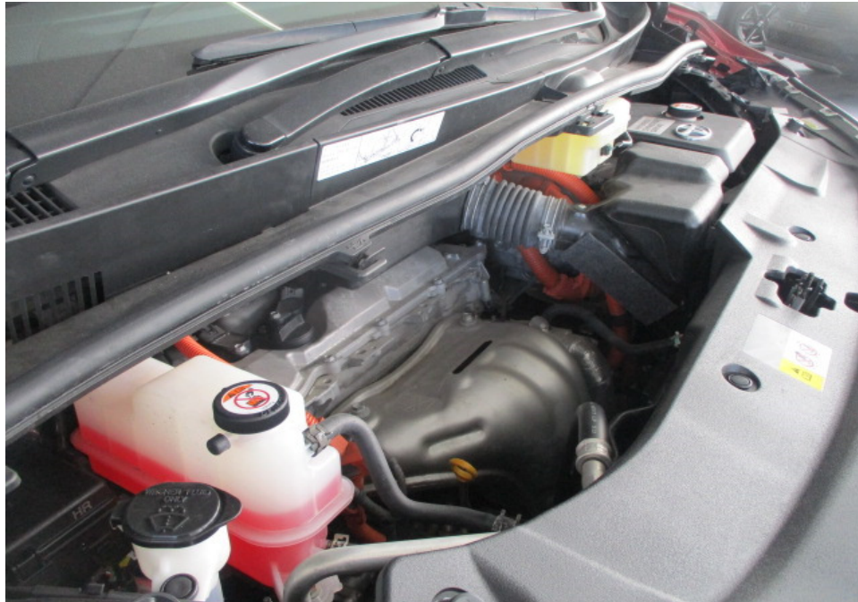
Photo 14 shows another view of the engine compartment of the Motor Car at the time of my inspection. The various parts and components inside the engine compartment were all observed to be intact and properly fitted. There was also no sign(s) or indication(s) of fluid leak and/or fluid stain found inside the engine compartment.
