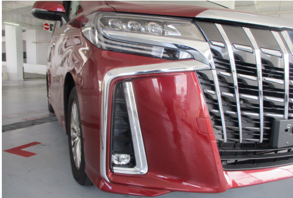
Photo 6 shows a closer view of the Motor Car's front bumper, front bumper right chrome moulding, front grille, front right fog lamp, front right headlamp and front right headlamp chrome moulding. The body parts at the front right portion of the Motor Car were visually examined and it was observed that the repair/restoration works carried out to the damaged area of the Motor Car (refer to photograph 1 above) were reasonably adequate and in order.
