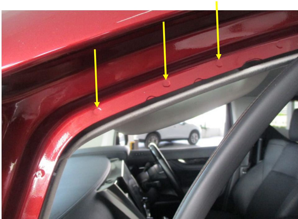
Photo 33 shows the left side "A" pillar of the Motor Car. I did not find any weld marks other than original spot weld marks (arrowed) on the left side "A" pillar of the Motor Car, which indicates that there was no re-welding works carried out. In general, I had found all the non-detachable body panels of the Motor Car to be originally fitted at the time of my inspection.
