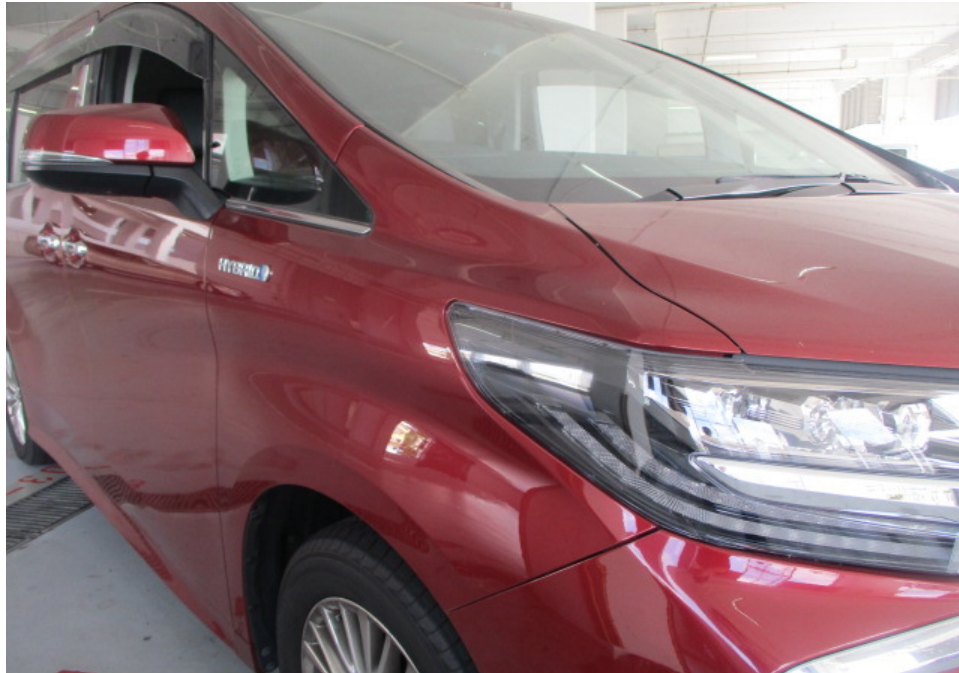
Photo 8 shows a closer view of the Motor Car's front bonnet, front right headlamp and front right fender. The body parts at the front right portion of the Motor Car were visually examined and it was observed that the repair/restoration works carried out to the damaged area of the Motor Car (refer to photograph 1 above) were reasonably adequate and in order.
