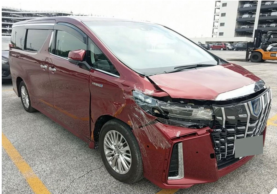
Photo 1 shows the front right body of the Motor Car (photograph provided to me). The Motor Car was observed to have sustained damage at its front right portion. The front bumper, front bumper right chrome moulding, front bumper right sensors, front right fog lamp, front right headlamp, front right headlamp chrome moulding, front right fender, front grille, front bonnet and front bonnet right hinge were amongst the body parts that were observed to have been damaged.
