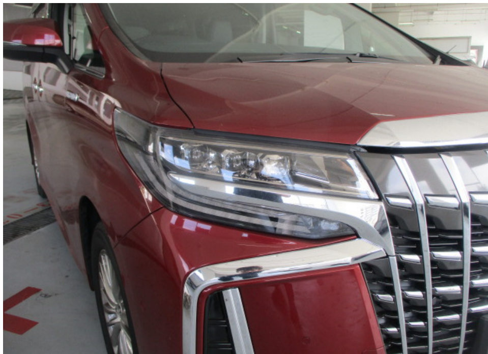
Photo 7 shows a closer view of the Motor Car's front bonnet, front right headlamp and front right headlamp chrome moulding. The body parts at the front right portion of the Motor Car were visually examined and it was observed that the repair/restoration works carried out to the damaged area of the Motor Car (refer to photograph 1 above) were reasonably adequate and in order.
