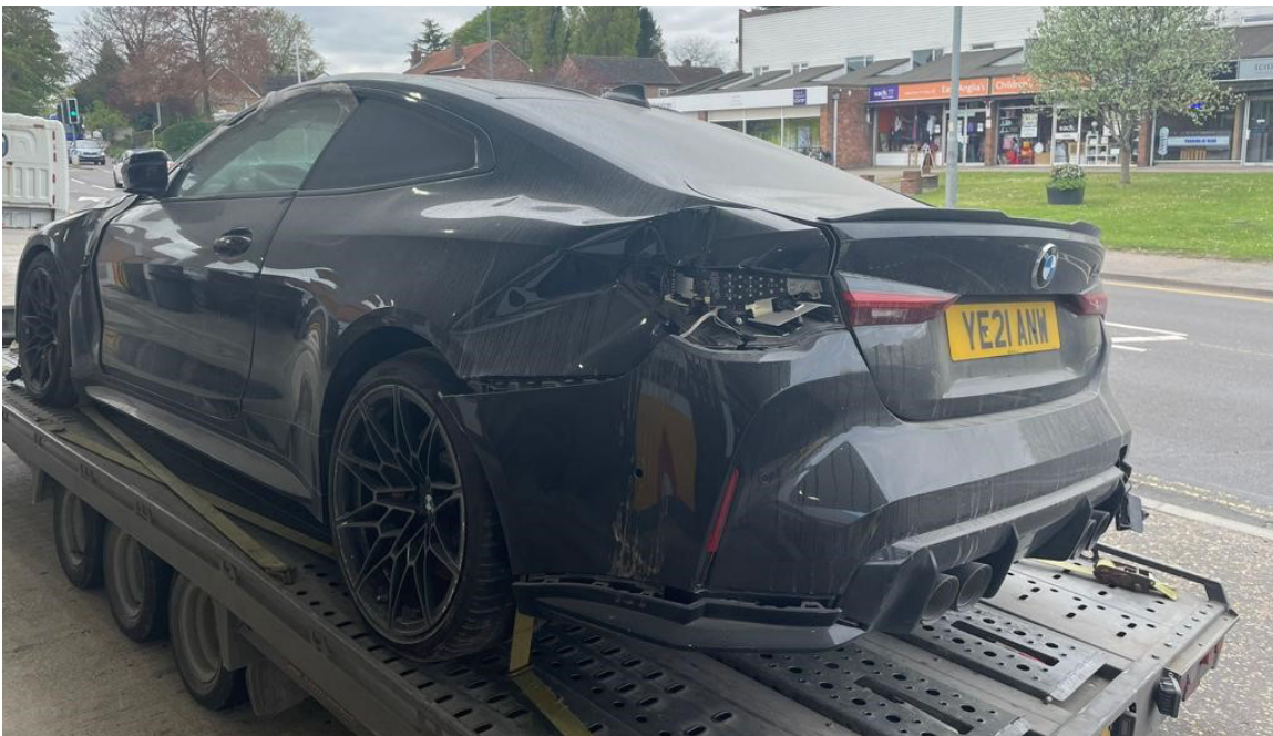
Photo 3 shows the rear left body of the Motor Car (photograph provided to me). The Motor Car's left rear portion was also observed to be damaged. The rear left fender, rear left taillamp and rear bumper were amongst the body parts that were damaged.
