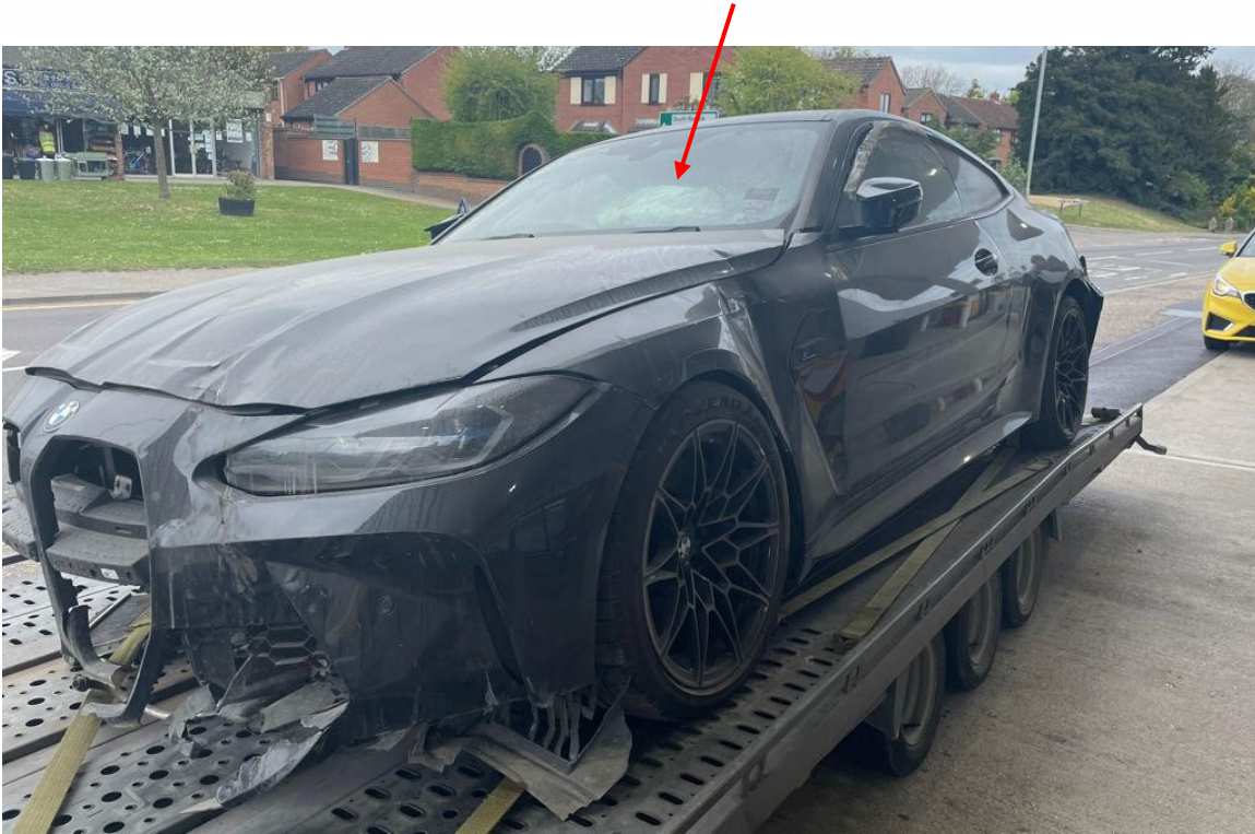
Photo 2 shows the front left body of the Motor Car (photograph provided to me). The Motor Car was observed to have sustained damage at its frontal portion. The front bumper, front bumper left lower grille, front bumper sensors, front bumper under cover, front grilles, front bonnet, front left headlamp and front left fender were amongst the body parts that were observed to have been damaged. The front left passenger airbag (arrowed) of the Motor Car was deployed.
