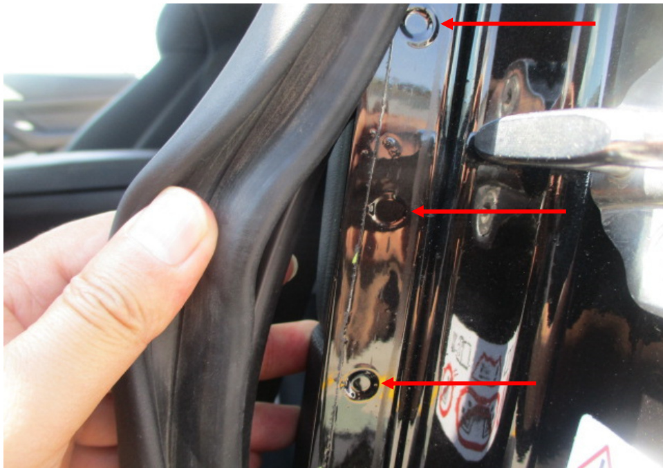
Photo 33 shows the left side rear body panel of the Motor Car. I did not find any weld marks other than original spot weld marks (arrowed) on the left side rear body panel of the Motor Car, which indicates that there was no re-welding works carried out. In general, I had found all the non-detachable body panels of the Motor Car to be originally fitted at the time of my inspection.
