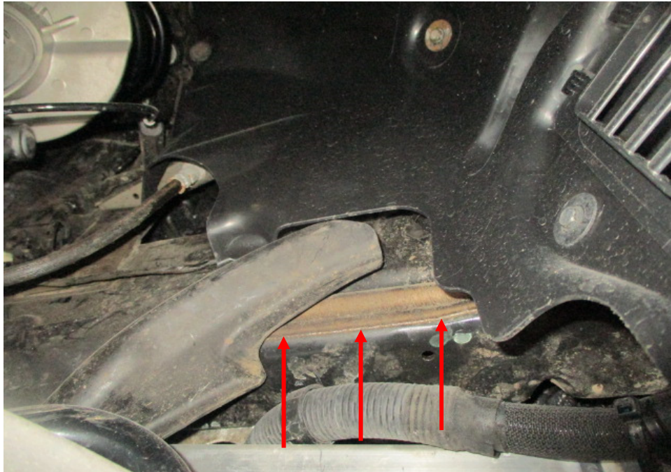
Photo 32 shows the chassis/structural body at the underside front right of the Motor Car. The original factory sealant (arrowed) at the joints along the chassis/structural body was observed to be untouched. In general, I had found no work was carried out on the chassis/structural body of the Motor Car. The chassis/structural body of the Motor Car was originally fitted.
