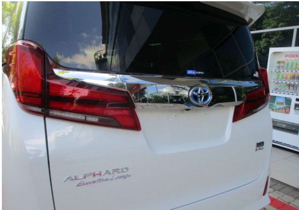
Photo 7 shows a closer view of the Motor Car's rear tailgate, rear tailgate upper chrome moulding, rear left tailgate lamp and rear left taillamp. The body parts at the rear portion of the Motor Car were visually examined and it was observed that the repair/restoration works carried out to the damaged area of the Motor Car (refer to photograph 1 & 2 above) were reasonably adequate and in order.
