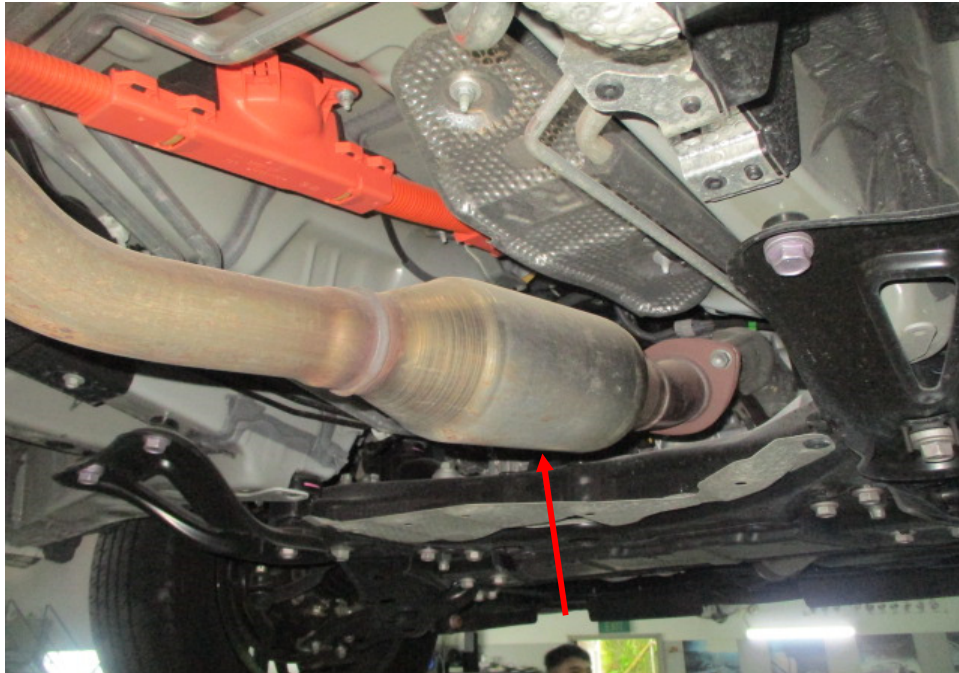
Photo 28 shows a general view of the front section of the Motor Car's exhaust system. My examination of the Motor Car's exhaust system revealed no sign(s) or indication(s) of any cut or weld marks along its exhaust pipe, on its catalytic converter (arrowed), on its centre resonator box and on its rear muffler.
