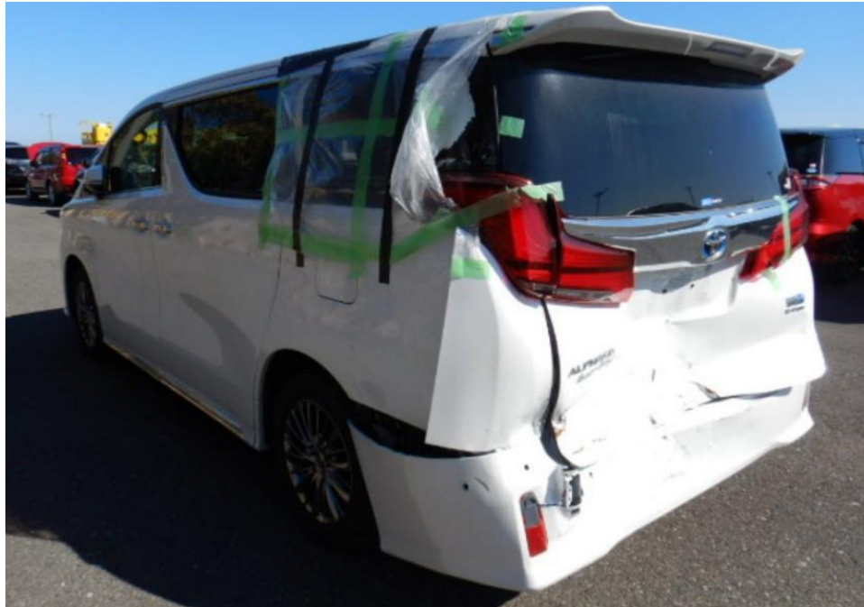
Photo 1 shows the rear left body of the Motor Car (photograph provided to me). The Motor Car was observed to have sustained damage at its rear portion (circled). The rear bumper, rear bumper left reflector, rear bumper sensors, rear left taillamp lower garnish, rear tailgate, rear tailgate lock, rear tailgate upper chrome moulding, rear left tailgate lamp and rear end panel were amongst the body parts that were observed to have been damaged.
