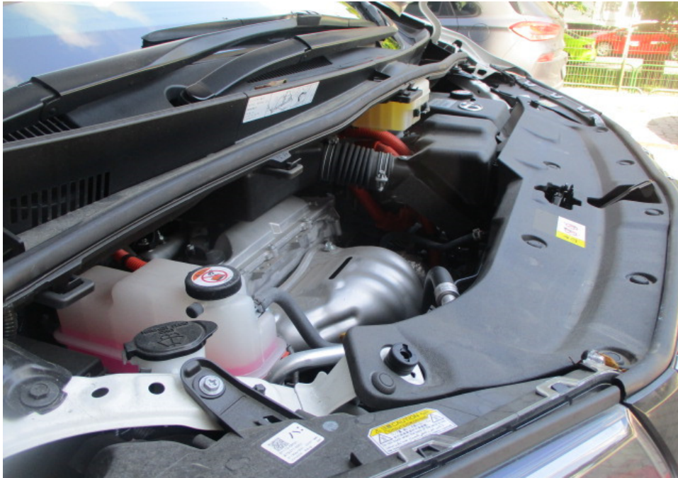
Photo 16 shows another view of the engine compartment of the Motor Car at the time of my inspection. The various parts and components inside the engine compartment were all observed to be intact and properly fitted. There was no sign(s) or indication(s) of fluid leak and/or fluid stain found inside the engine compartment.
