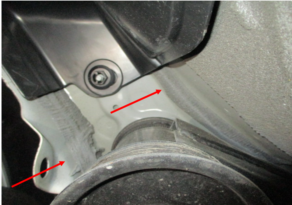
Photo 30 shows the chassis/structural body at the underside rear left of the Motor Car. The original factory sealant (arrowed) at the joints along the chassis/structural body was observed to be untouched. In general, I had found no work was carried out on the chassis/structural body of the Motor Car. The chassis/structural body of the Motor Car was originally fitted.
