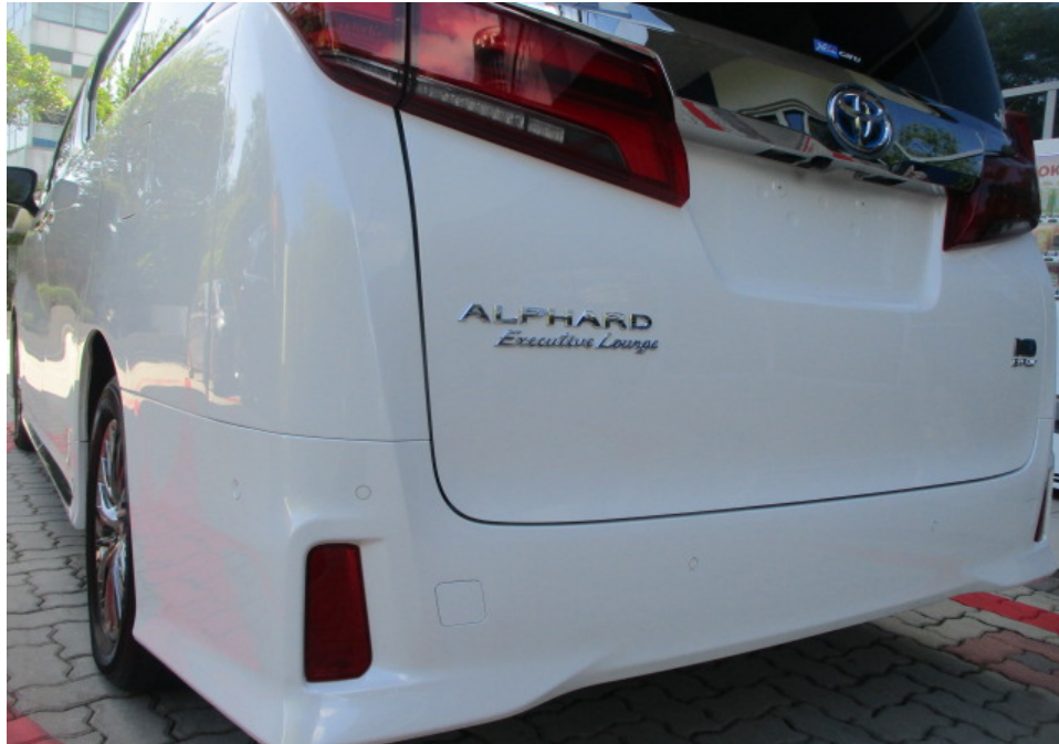
Photo 6 shows a closer view of the Motor Car's rear bumper, rear bumper left reflector, rear bumper sensors, rear bumper left tow cover and rear left taillamp lower garnish. The body parts at the rear portion of the Motor Car were visually examined and it was observed that the repair/restoration works carried out to the damaged area of the Motor Car (refer to photograph 1 & 2 above) were reasonably adequate and in order.
