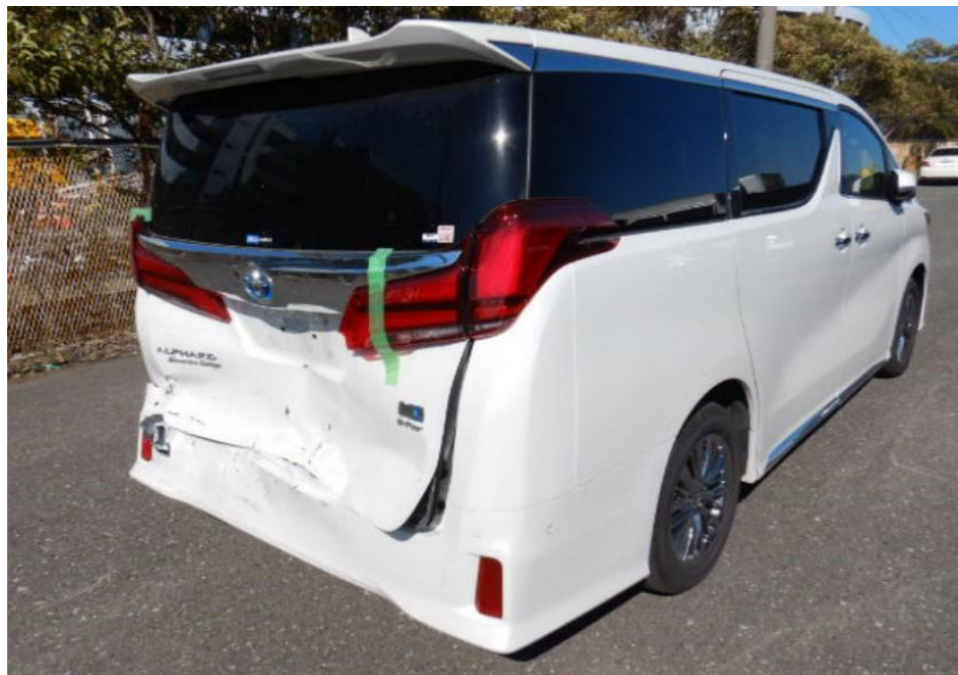
Photo 2 shows the rear right body of the Motor Car (photograph provided to me). The Motor Car was observed to have sustained damage at its rear portion (circled). The rear bumper, rear tailgate, rear tailgate lock, rear tailgate upper chrome moulding, rear right tailgate lamp and rear end panel were amongst the body parts that were observed to have been damaged.
