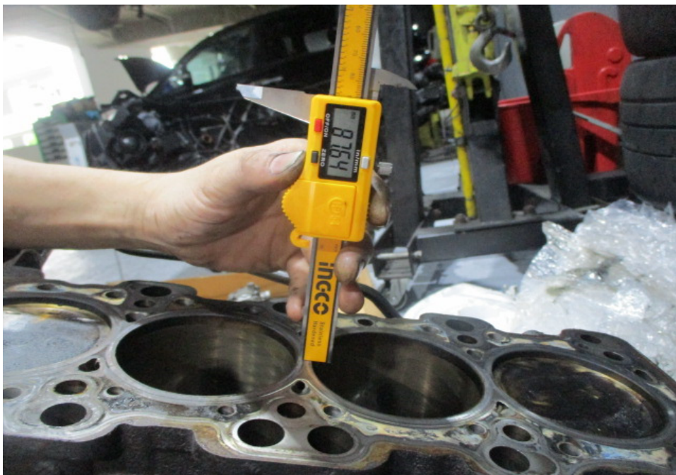
Photo 18 shows the stroke measurement of cylinder 3, which was recorded to be 87.64mm.
