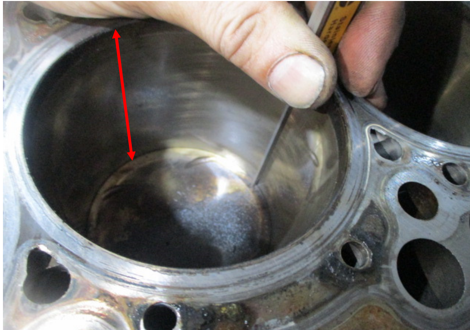
Photo 13 shows measurement being carried out to the stroke (arrowed) of cylinder 2 of the Mitsubishi engine. The bore and stroke measurements of the Mitsubishi engine were carried out using a digital Vernier Caliper that was calibrated before the start of the measurements.
