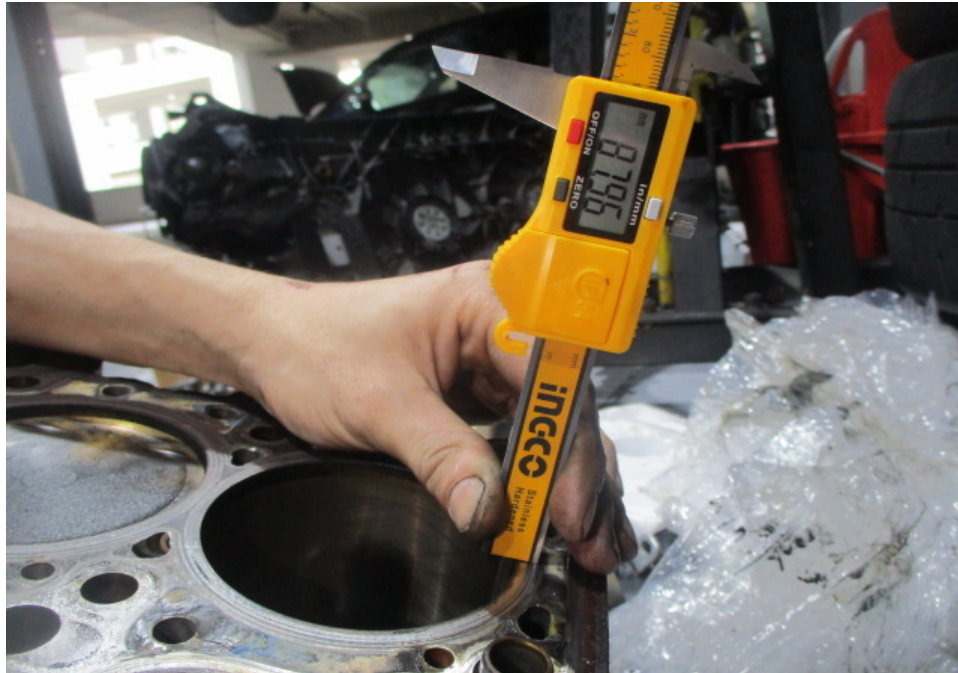
Photo 23 shows the stroke measurement of cylinder 4, which was recorded to be 87.96mm.
