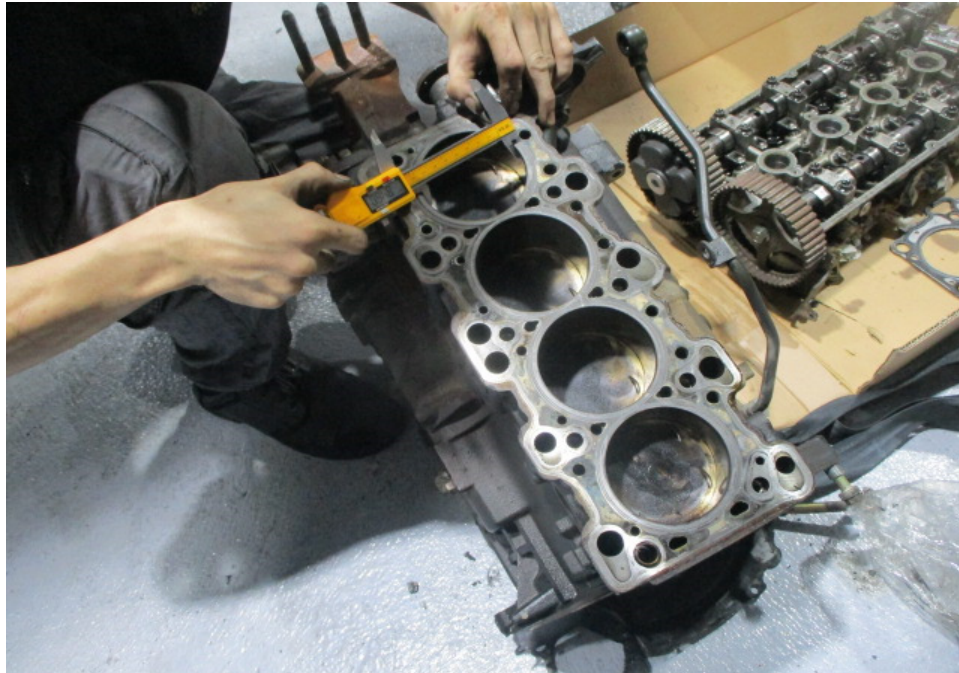
Photo 7 shows measurement being carried out to the bore of cylinder 1 of the Mitsubishi engine. The bore and stroke measurements of the Mitsubishi engine were carried out using a digital Vernier Caliper that was calibrated before the start of the measurements.
