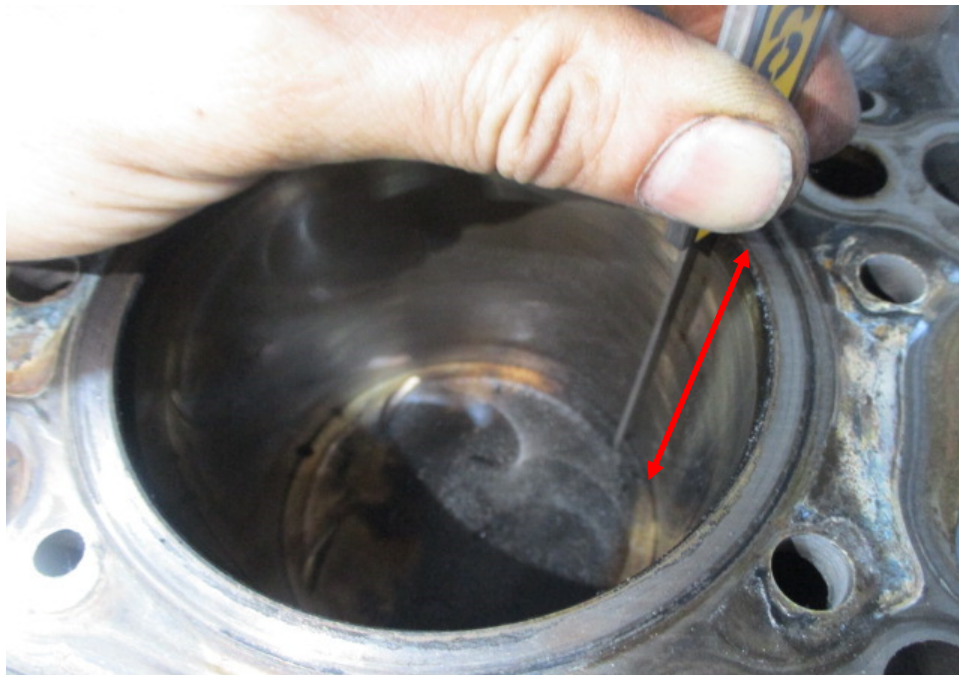
Photo 10 shows measurement being carried out to the stroke (arrowed) of cylinder 1 of the Mitsubishi engine. The bore and stroke measurements of the Mitsubishi engine were carried out using a digital Vernier Caliper that was calibrated before the start of the measurements.
