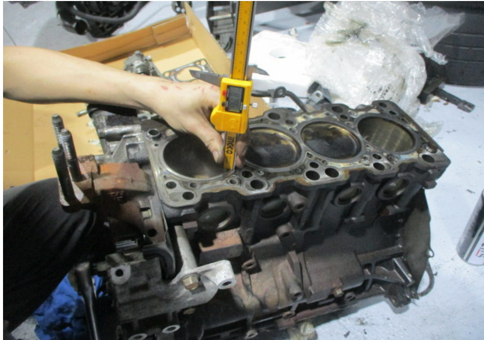
Photo 9 shows measurement being carried out to the stroke of cylinder 1 of the Mitsubishi engine. The bore and stroke measurements of the Mitsubishi engine were carried out using a digital Vernier Caliper that was calibrated before the start of the measurements.
