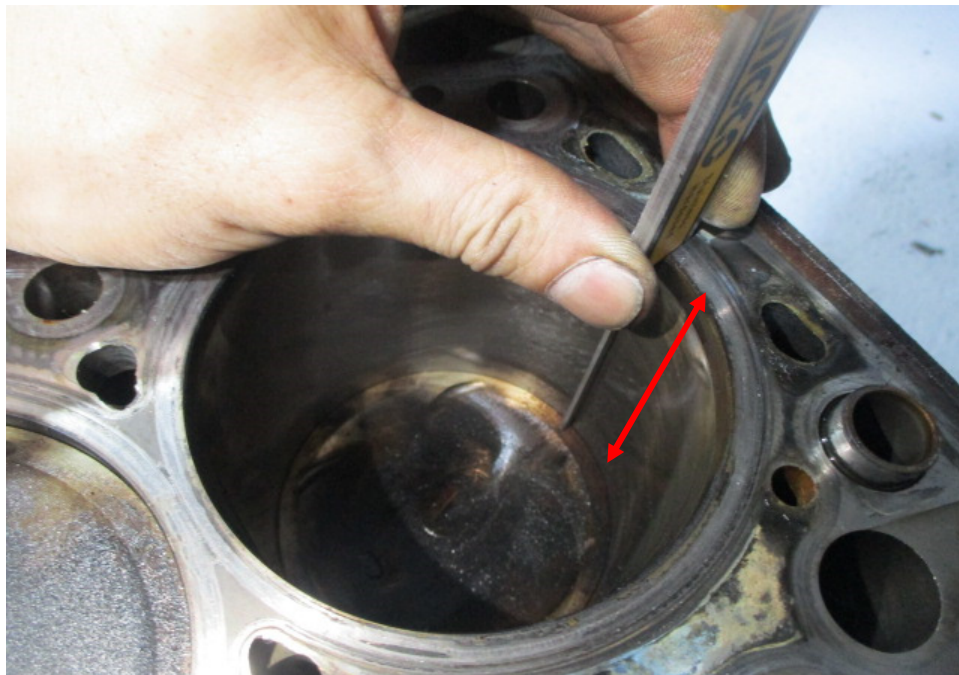
Photo 22 shows measurement being carried out to the stroke (arrowed) of cylinder 4 of the Mitsubishi engine. The bore and stroke measurements of the Mitsubishi engine were carried out using a digital Vernier Caliper that was calibrated prior to the start of measurements.
