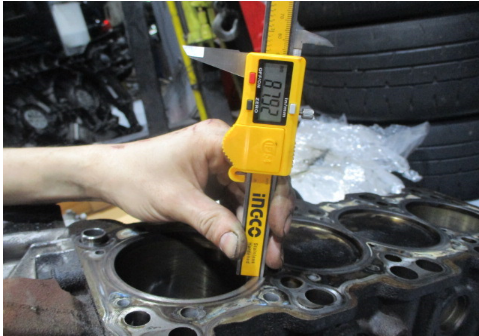
Photo 11 shows the stroke measurement of cylinder 1, which was recorded to be 87.92mm.
