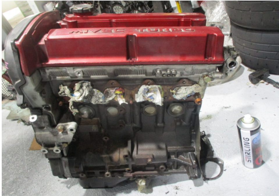
Photo 3 shows a general view of the Mitsubishi engine that I had inspected. My visual examination of the engine housing revealed the housing to be of serviceable/satisfactory condition. There was no crack and/or hole observed on the engine housing.
