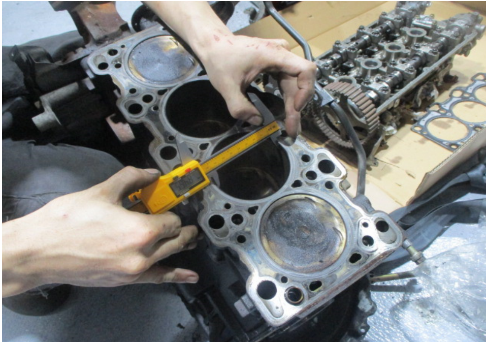
Photo 15 shows measurement being carried out to the bore of cylinder 3 of the Mitsubishi engine. The bore and stroke measurements of the Mitsubishi engine were carried out using a digital Vernier Caliper that was calibrated before the start of the measurements.
