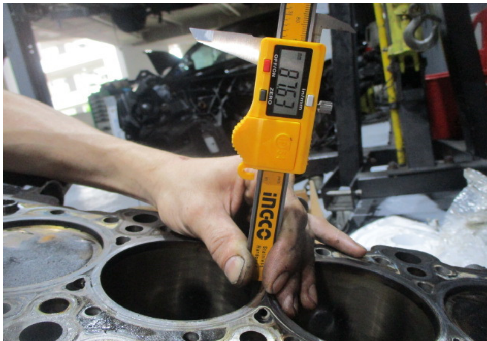
Photo 14 shows the stroke measurement of cylinder 2, which was recorded to be 87.63mm.
