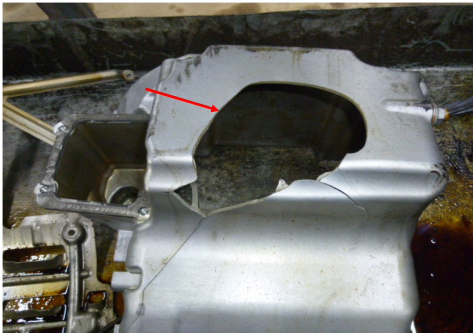
Photo 6 shows a closer view of the crack (arrowed) on the underside of the engine oil sump of the Insured Vehicle. The damage profile of the engine oil sump corresponds to the possibility of the Insured Vehicle going over an object.
