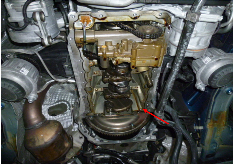
Photo 7 shows the undercarriage parts and components that were immediately after the punctured engine oil sump, covered with engine oil stains (arrowed).
