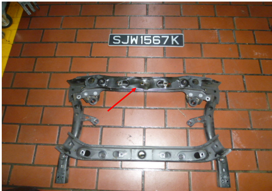
Photo 2 shows the dented dismantled engine mounting (red arrow) of the Insured Vehicle at the time of our inspection.
