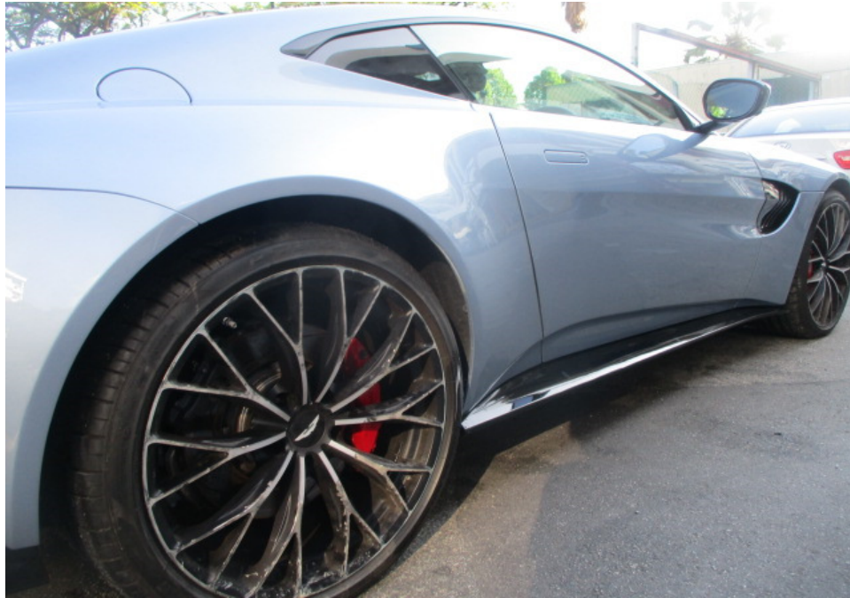
Photo 12 shows a closer view of the Motor Car's rear right wheel rim, rear right body panel and front right door. The body parts at the right side centre portion of the Motor Car were visually examined and it was observed that the repair/restoration works carried out to the damaged area of the Motor Car (refer to photograph 3 & 4 above) were reasonably adequate and in order.
