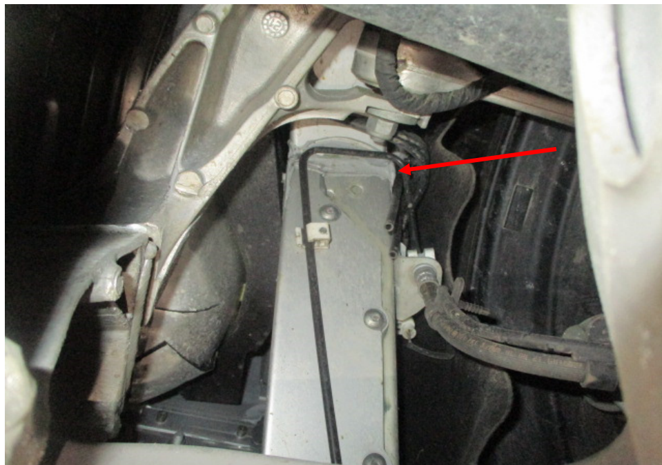
Photo 29 shows the aluminium chassis/structural body at the underside rear right of the Motor Car. The original factory sealant (arrowed) at the joints along the aluminium chassis/structural body of the Motor Car was observed to be untouched. In general, I had found no work was carried out on the aluminium chassis/structural body of the Motor Car. The aluminium chassis/structural body of the Motor Car was originally fitted.
