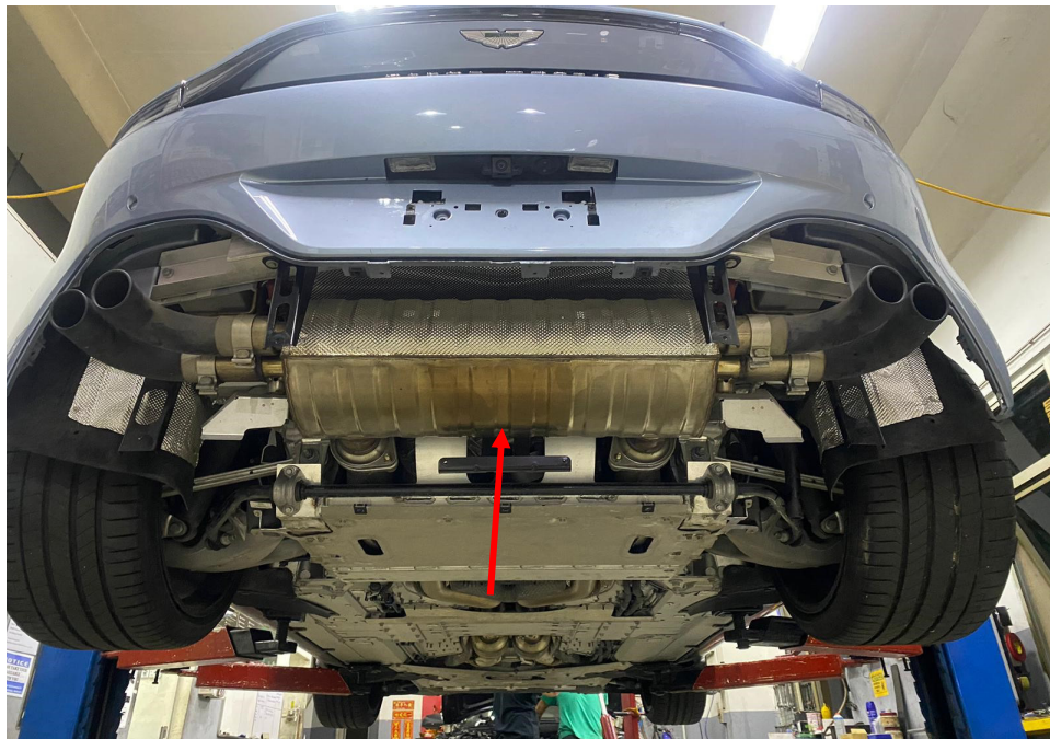
Photo 27 shows the Motor Car with its rear bumper lower diffuser removed to facilitate my examination of its exhaust system. My examination of the Motor Car's exhaust system revealed no sign(s) or indication(s) of any cut or weld marks along its exhaust pipes, on its rear muffler (arrowed), on its centre resonator boxes and on its catalytic converters.
