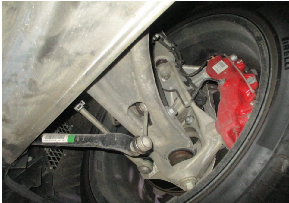
Photo 26 shows the various undercarriage components at the front right wheel of the Motor Car. The mechanical components, control arms and linkages were all found to be intact and secured in an appropriate manner. I also did not observe any fluid leak and/or fluid stain on the underside of the Motor Car.
