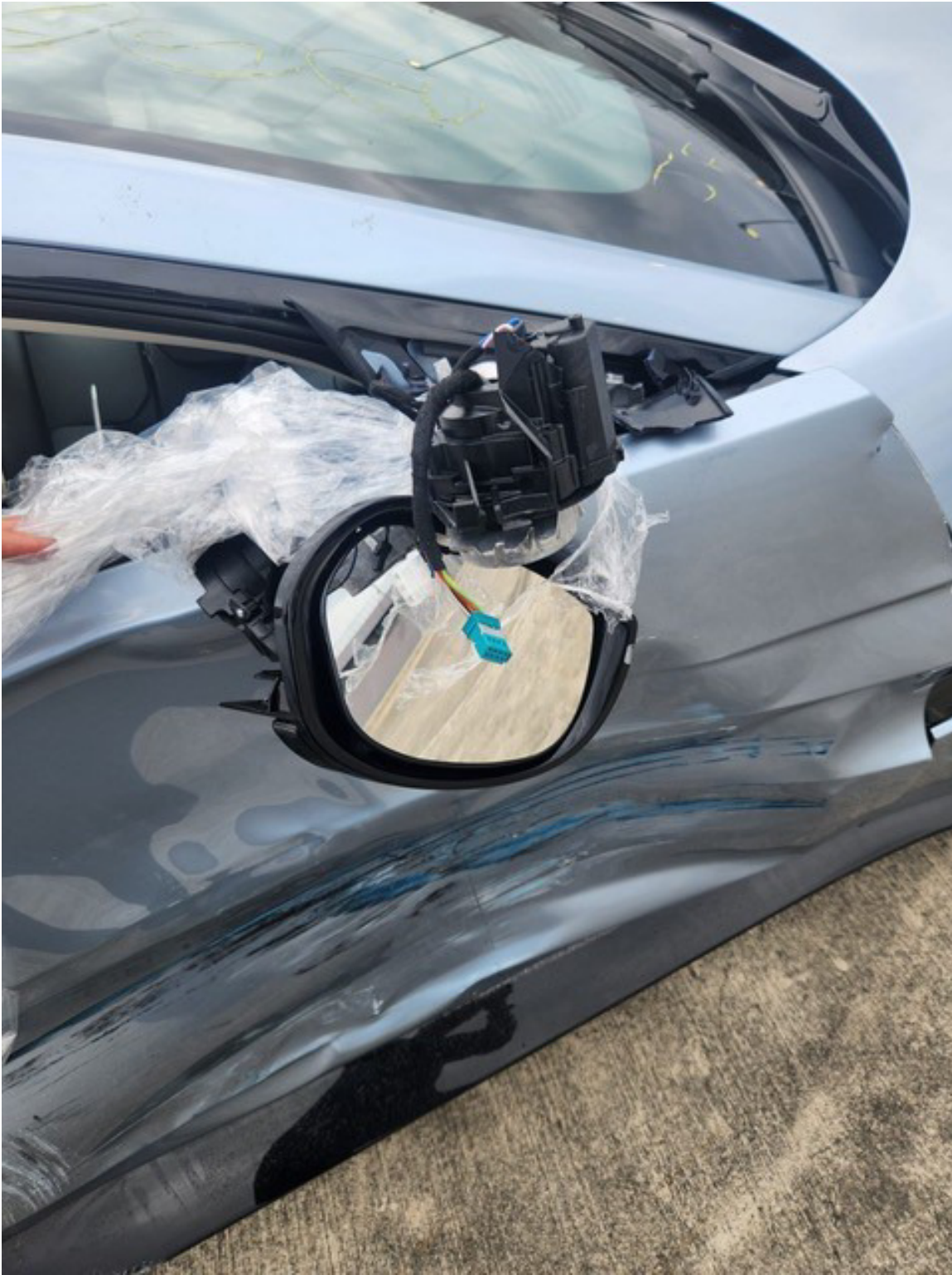
Photo 2 shows a closer view of the damage to the front right door and right side wing mirror of the Motor Car (photograph provided to me).
