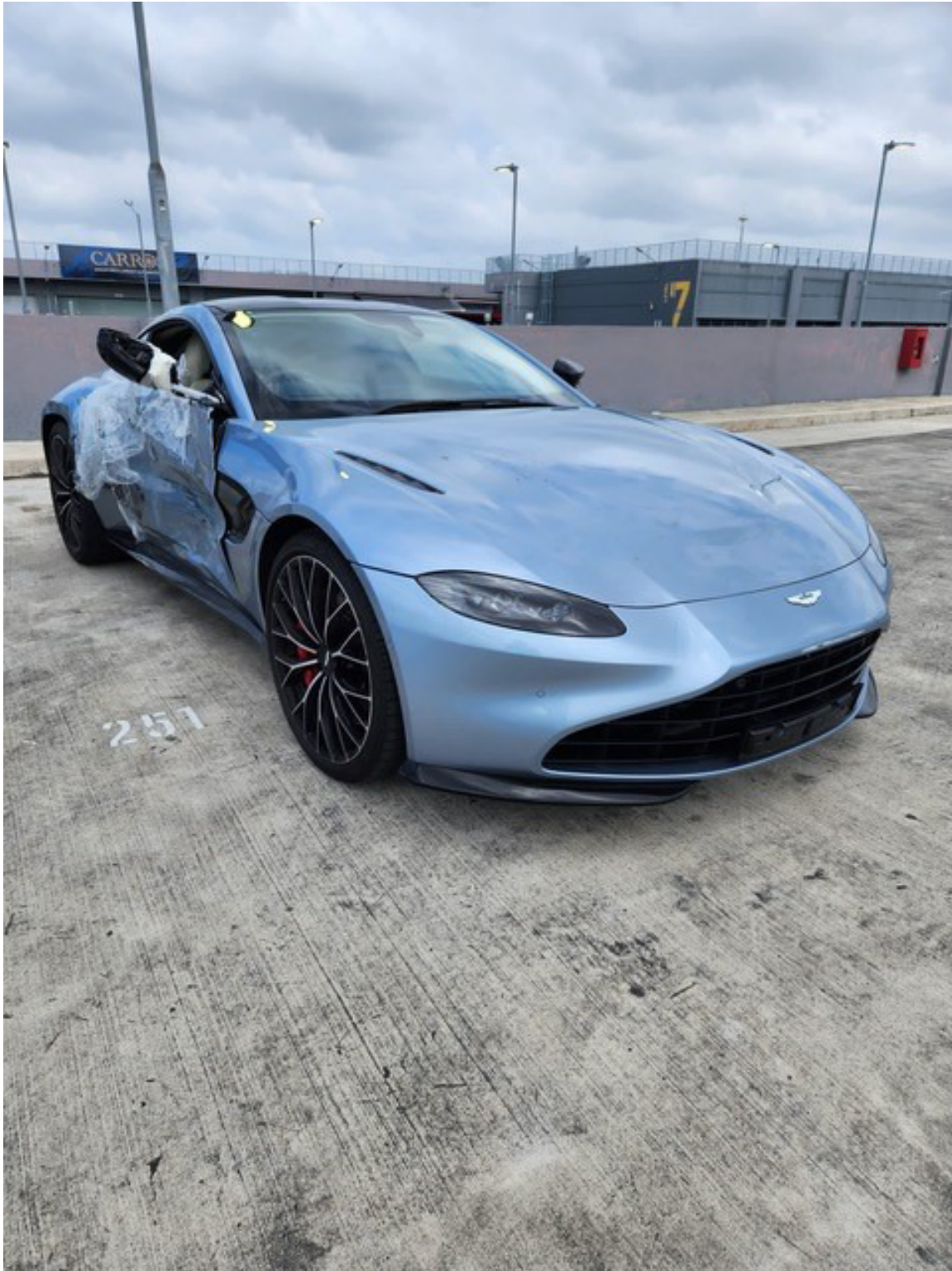
Photo 1 shows the front right body of the Motor Car (photograph provided to me). The Motor Car was observed to have sustained damage at its right side centre portion. The front right door, rear right body panel, rear right wheel rim and right side wing mirror were amongst the body parts that were observed to have been damaged.
