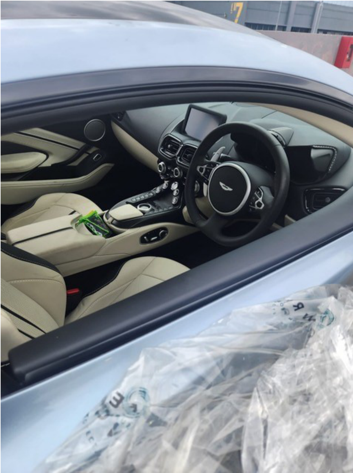
Photo 7 shows the interior compartment of the Motor Car (photograph provided to me). The various parts and components within the interior compartment were all intact and unaffected. The Motor Car's airbag(s) was not deployed as seen from the photographs that were provided to me.
