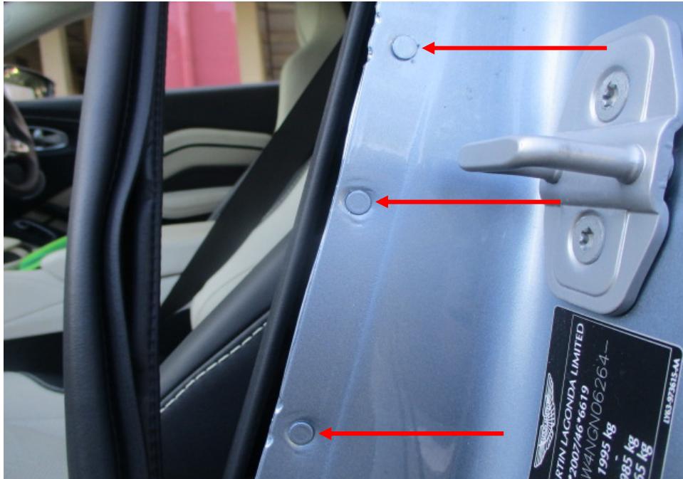
Photo 36 shows the left side rear body panel of the Motor Car. I did not find any weld marks other than original spot weld marks (arrowed) on the left side rear body panel of the Motor Car, which indicates that there was no re-welding works carried out. In general, I had found all the non-detachable body panels of the Motor Car to be originally fitted at the time of my inspection.
