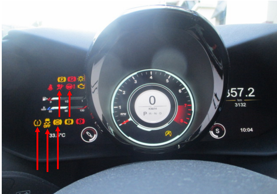
Photo 20 shows the warning lights for the various electronic safety features appearing on the instrument panel of the Motor Car during its self-test when the engine is cranked, in particular the ABS, SRS, PSS, TPM and TCS (arrowed).
