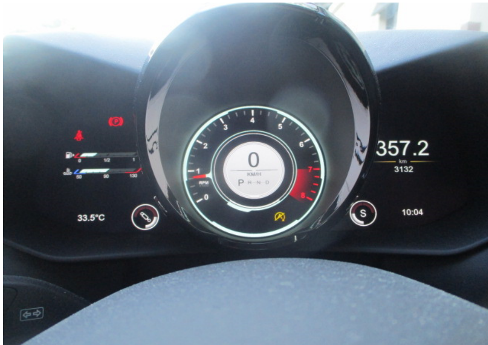
Photo 21 shows the respective warning lights no longer illuminated, indicating that there is no fault detected to the ABS, SRS, PSS, TPM and TCS systems of the Motor Car during the self-test. These electronic systems were hence in working condition at the time of my inspection.
