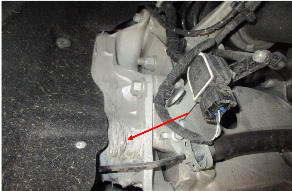
Photo 32 shows the aluminium chassis/structural body at the underside front right of the Motor Car. I did not find any weld marks other than original spot weld marks on the aluminium chassis/structural body of the Motor Car. The original factory sealant (arrowed) at the joints along the aluminium chassis/structural body was untouched, indicating no work was done on the aluminium chassis/structural body of the Motor Car and that the aluminium chassis/structural body was originally fitted.
