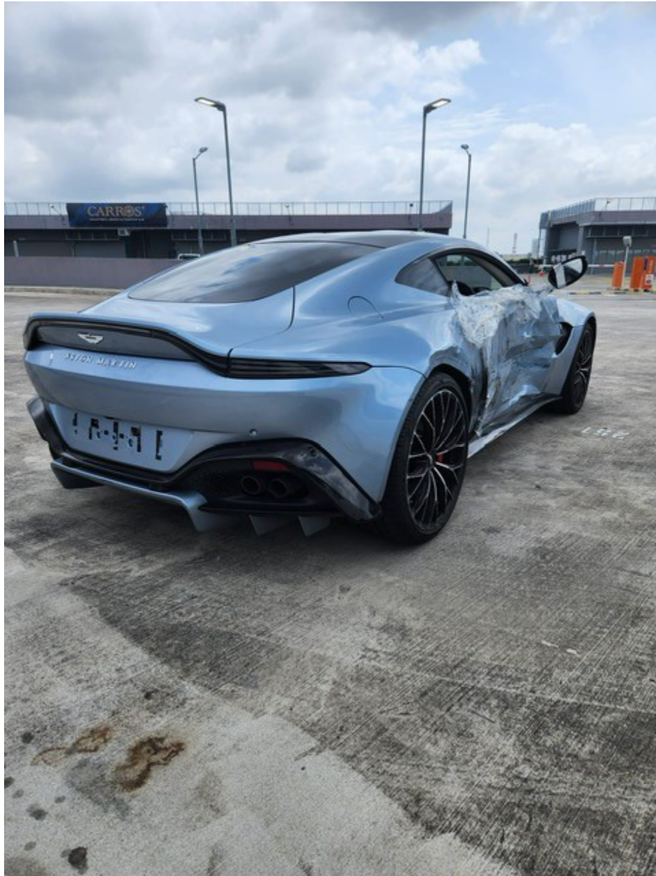
Photo 3 shows the rear right body of the Motor Car (photograph provided to me). The Motor Car was observed to have sustained damage at its right side centre portion. The front right door, rear right body panel, rear right wheel rim and right side wing mirror were amongst the body parts that were observed to have been damaged.
