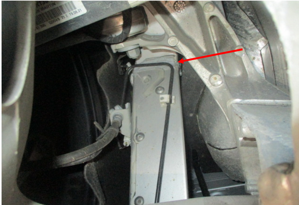
Photo 30 shows the aluminium chassis/structural body at the underside rear left of the Motor Car. I did not find any weld marks other than original spot weld marks on the aluminium chassis/structural body of the Motor Car. The original factory sealant (arrowed) at the joints along the aluminium chassis/structural body was untouched, indicating no work was done on the aluminium chassis/structural body of the Motor Car and that the aluminium chassis/structural body was originally fitted.
