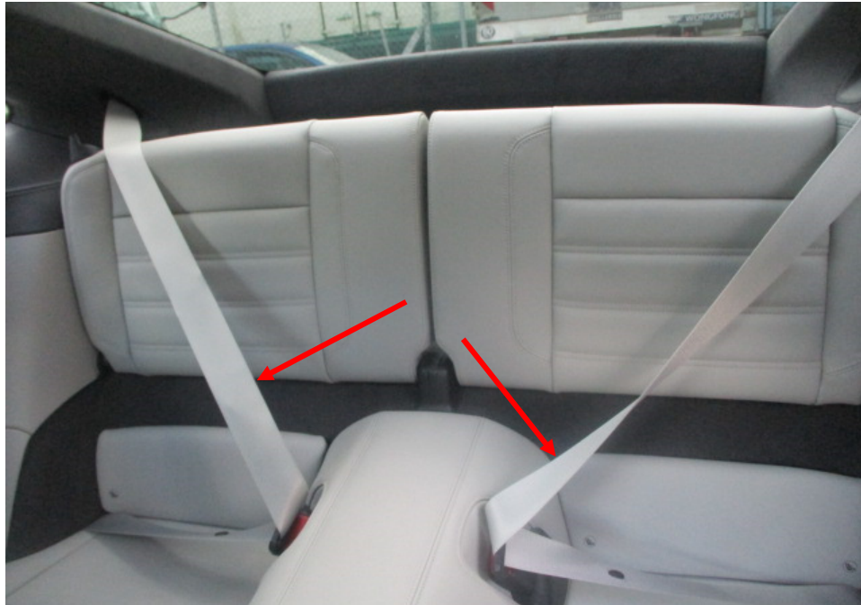
Photo 23 shows the rear seats of the Motor Car. All the seats of the Motor Car were secured via seat rails to the floorboard. They were also fitted with a retractable seat belt reel and a pre-tensioner. The seat belts (arrowed) were tested and were able to be fastened into the respective pre-tensions that were fitted on the side of each individual seat.
