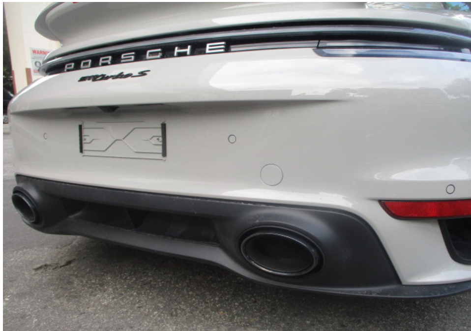
Photo 16 shows a closer view of the Motor Car's rear bumper, rear bumper lower cover, rear bumper sensors and rear centre top reflector. The body parts at the rear portion of the Motor Car were visually examined and it was observed that the repair/restoration works carried out to the damaged area of the Motor Car (refer to photograph 4 & 5 above) were reasonably adequate and in order.
