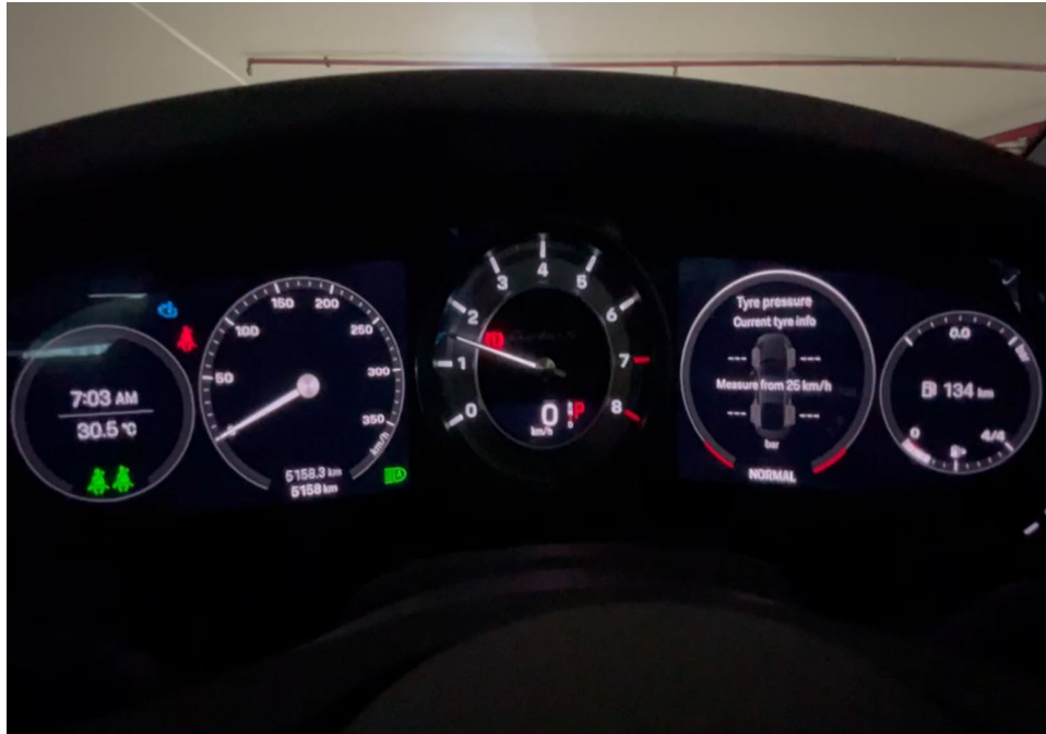
Photo 25 shows the respective warning lights no longer illuminated, indicating that there is no fault detected to the ABS, SRS, EPS, TPM and TCS systems of the Motor Car during the self-test. These electronic systems were hence in working condition at the time of my inspection.
