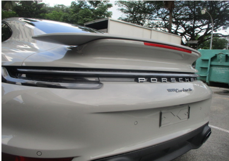
Photo 19 shows a closer view of the Motor Car's rear bumper, rear left taillamp, rear centre top reflector, rear centre top panel, rear top spoiler and third brake light. The body parts at the rear portion of the Motor Car were visually examined and it was observed that the repair/restoration works carried out to the damaged area of the Motor Car (refer to photograph 4 above) were reasonably adequate and in order.
