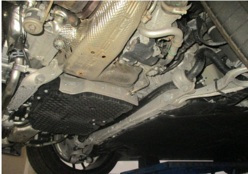
Photo 33 shows another view of the Motor Car's engine compartment. The engine compartment was at the rear underside of the Motor Car. The various parts and components inside the engine compartment were all observed to be intact and properly fitted. There was also no sign(s) or indication(s) of fluid leak and/or fluid stain found inside the engine compartment.
