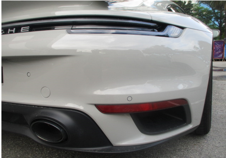
Photo 15 shows a closer view of the Motor Car's rear bumper, rear bumper lower cover, rear bumper tow cover, rear bumper right reflector, rear bumper right air duct, rear right exhaust garnish and rear right taillamp. The body parts at the rear portion of the Motor Car were visually examined and it was observed that the repair/restoration works carried out to the damaged area of the Motor Car (refer to photograph 4 & 5 above) were reasonably adequate and in order.
