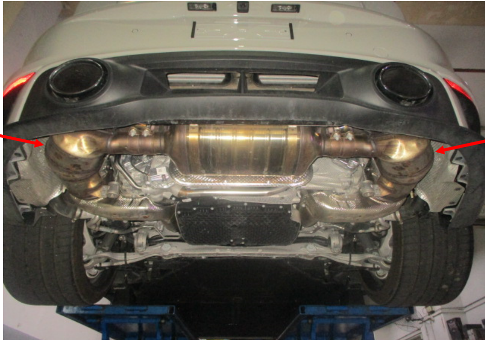
Photo 31 shows the Motor Car's exhaust system. My examination of the Motor Car's exhaust system revealed no sign(s) or indication(s) of any cut or weld marks along its exhaust pipes, on its catalytic converters (arrowed) and on its rear muffler.
