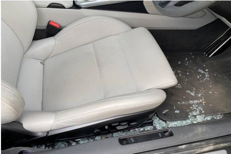
Photo 6 shows the interior compartment of the Motor Car (photograph provided to me). The various parts and components within the interior compartment were all intact and unaffected except for the front right door window glass, which was observed to be shattered.
