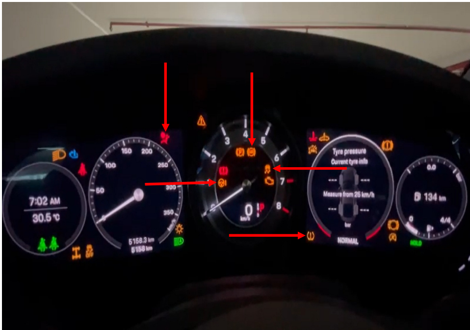
Photo 24 shows the warning lights for the various electronic safety features appearing on the instrument panel of the Motor Car during its self-test when the engine is cranked, in particular the ABS, SRS, EPS, TPM and TCS lights (arrowed).
