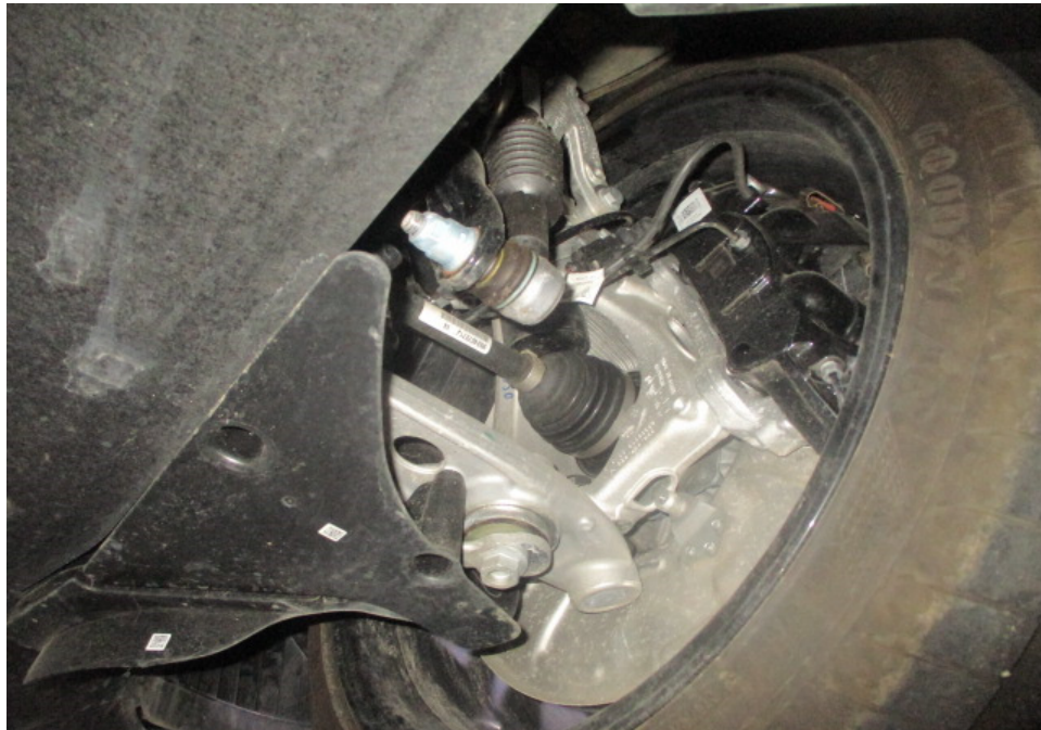
Photo 30 shows the various undercarriage components at the front right wheel of the Motor Car. The mechanical components, control arms and linkages were all found to be intact and secured in an appropriate manner. I also did not observe any fluid leak and/or fluid stain on the underside of the Motor Car.
