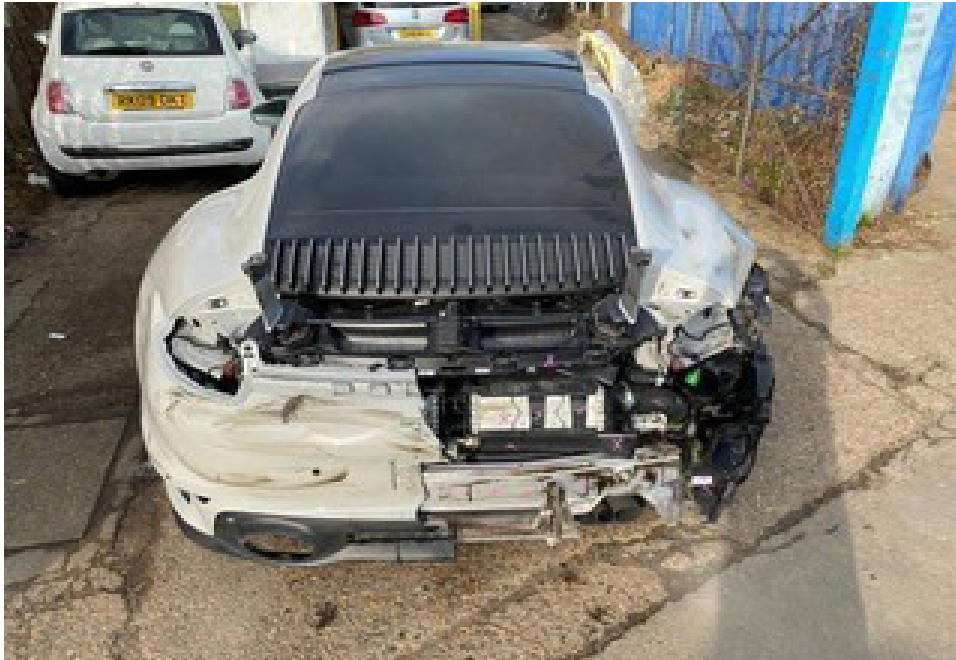
Photo 4 shows the rear body of the Motor Car (photograph provided to me). The photographs provided to me had showed damage to the rear portion of the Motor Car. Body parts that were either damaged, missing or dislodged include the rear bumper, rear bumper lower cover, rear bumper sensors, rear bumper left reflector, rear bumper right reflector, rear bumper right air duct, rear left exhaust garnish, rear right exhaust garnish, rear left taillamp, rear right taillamp, rear centre top reflector, rear centre top panel, rear top spoiler and third brake light amongst others.
