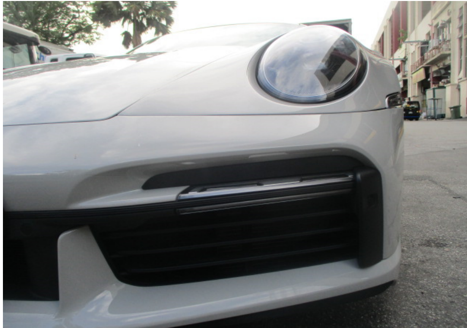
Photo 9 shows a closer view of the Motor Car's front bumper, front bumper left lower grille, front left day light and front left headlamp. The body parts at the frontal portion of the Motor Car were visually examined and it was observed that the repair/restoration works carried out to the damaged area of the Motor Car (refer to photograph 1 & 2 above) were reasonably adequate and in order.
