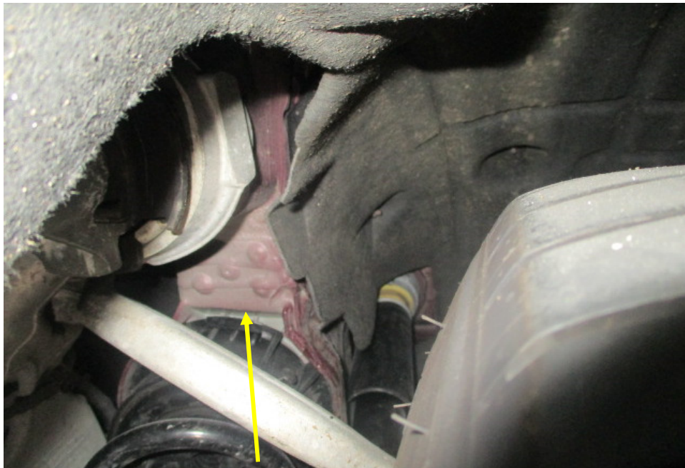
Photo 33 shows the chassis/structural body at the underside rear right of the Motor Car. I did not find any weld marks other than original spot weld marks on the chassis/structural body of the Motor Car. The original factory sealant (arrowed) at the joints along the chassis/structural body was untouched, indicating no work was done on the chassis/structural body of the Motor Car and that the chassis/structural body was originally fitted.
