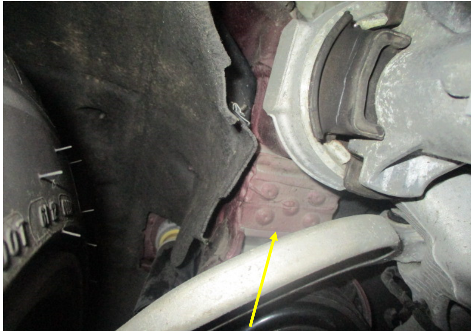
Photo 34 shows the chassis/structural body at the underside rear left of the Motor Car. The original factory sealant (arrowed) at the joints along the chassis/structural body was observed to be untouched. In general, I had found no work was carried out on the chassis/structural body of the Motor Car. The chassis/structural body of the Motor Car was originally fitted.
