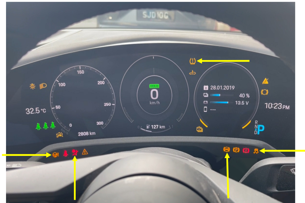
Photo 23 shows the warning lights for the various electronic safety features appearing on the instrument panel of the Motor Car during its self-test when the engine is cranked, in particular the ABS, SRS, EPS, TPM and SCS lights (arrowed).
