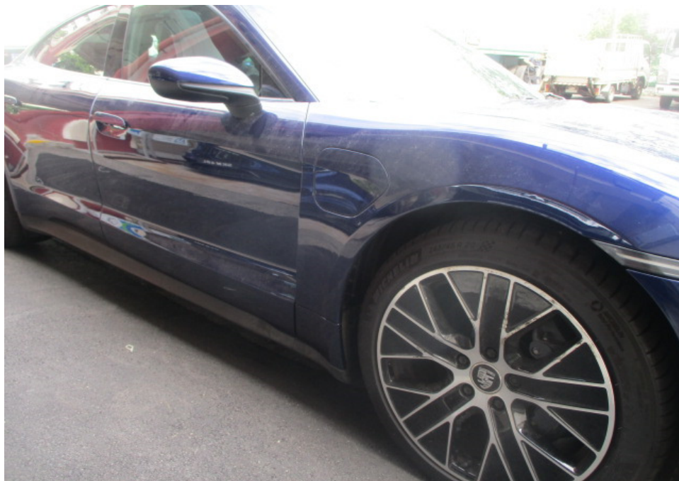
Photo 11 shows a closer view of the Motor Car's front right fender, front right wheel rim, front right door and right side wing mirror. The body parts at the right side front portion of the Motor Car were visually examined and it was observed that the repair/restoration works carried out to the damaged area of the Motor Car (refer to photograph 1 & 2 above) were reasonably adequate and in order.
