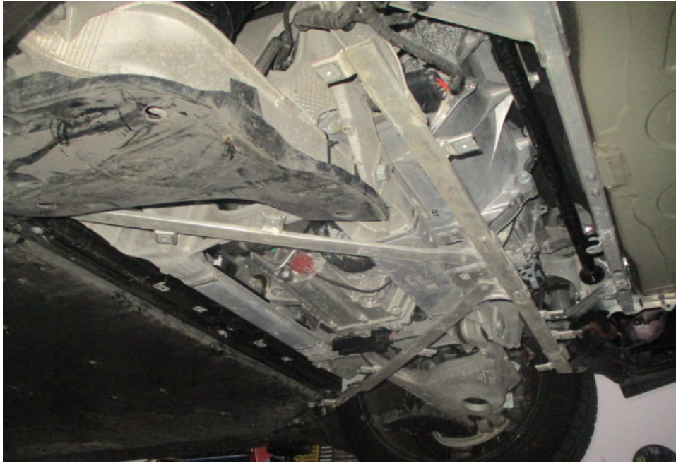
Photo 30 shows the underside rear of the Motor Car, at the location where the rear electric motor is fitted. The high voltage system of the Motor Car was visually checked, and it was observed that the various high voltage parts and components like the high voltage battery, inverter unit, converter unit, high voltage cables, electric motors and electric aircon compressor amongst others, were properly secured and without any physical damage.
