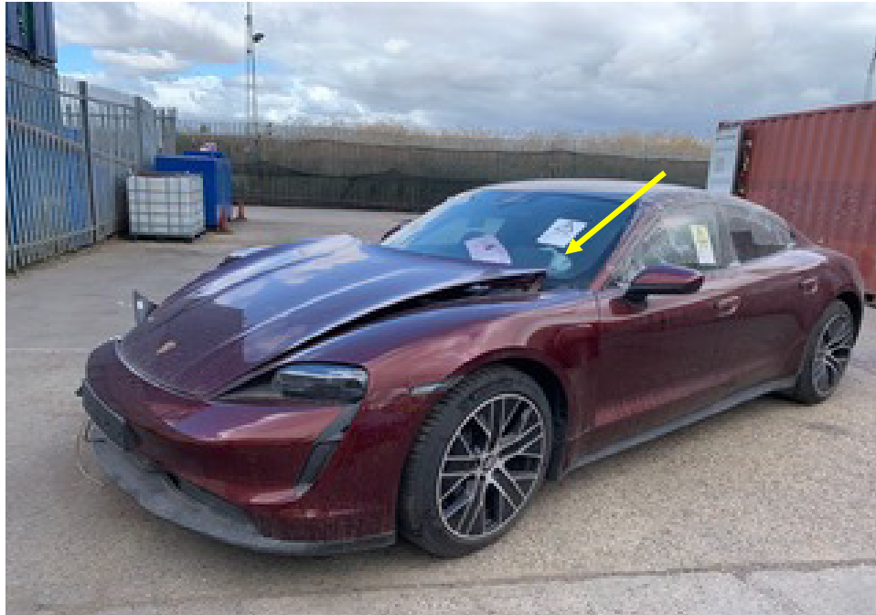
Photo 3 shows the front left body of the Motor Car (photograph provided to me). The left side portion of the Motor Car was observed to be unaffected. The front left passenger airbag was deployed (arrowed).
