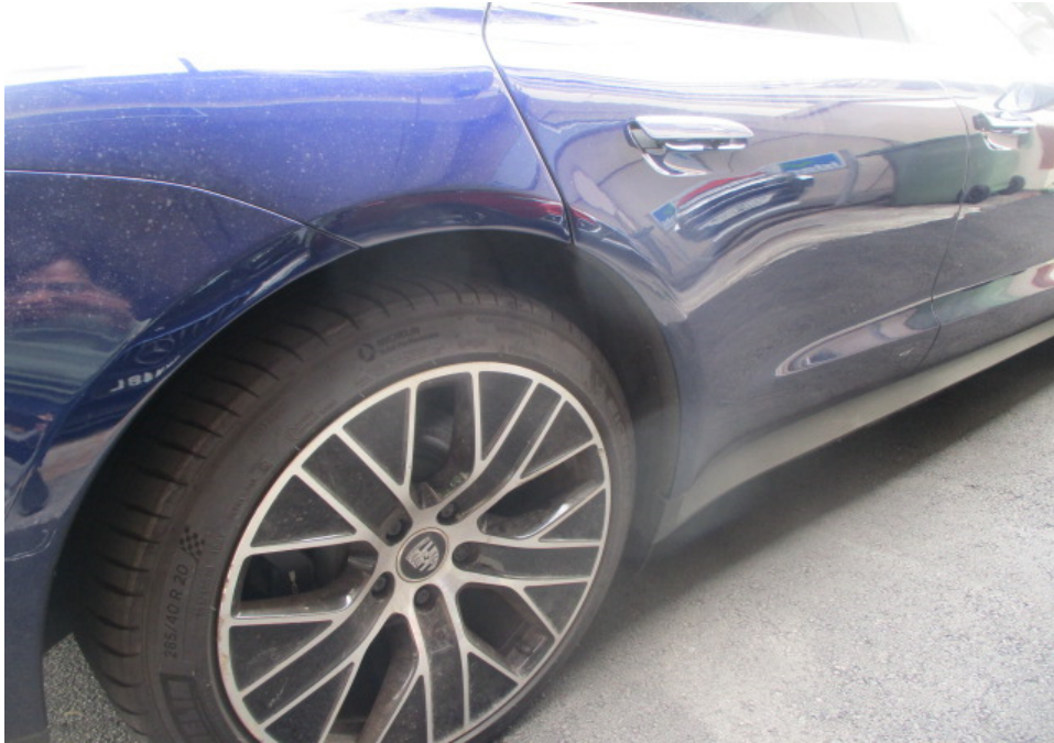
Photo 16 shows a closer view of the Motor Car's rear bumper, rear right fender, rear right wheel rim and rear right door. The body parts at the right side rear portion of the Motor Car were visually examined and it was observed that the repair/restoration works carried out to the damaged area of the Motor Car (refer to photograph 4 & 5 above) were reasonably adequate and in order.
