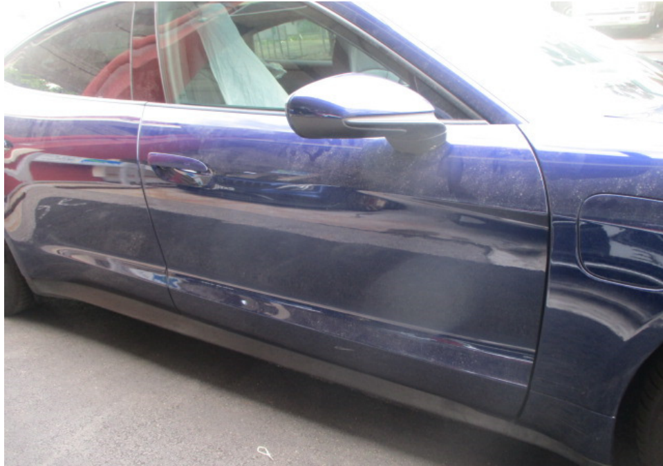
Photo 12 shows a closer view of the Motor Car's front right door, rear right door, right side wing mirror and right side rocker panel garnish. The body parts at the right side front portion of the Motor Car were visually examined and it was observed that the repair/restoration works carried out to the damaged area of the Motor Car (refer to photograph 1 & 2 above) were reasonably adequate and in order.
