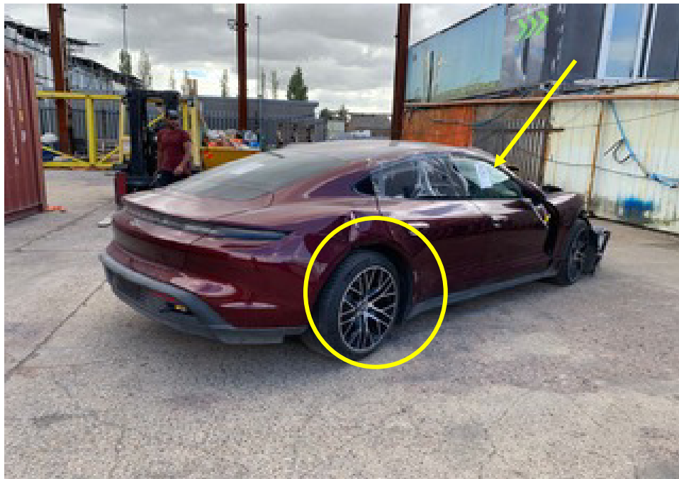
Photo 4 shows the rear right body of the Motor Car (photograph provided to me). Apart for the right side front portion, the photographs provided had also showed damage at the right side rear portion (circled). The Motor Car's right curtain airbag (arrowed) was deployed.
