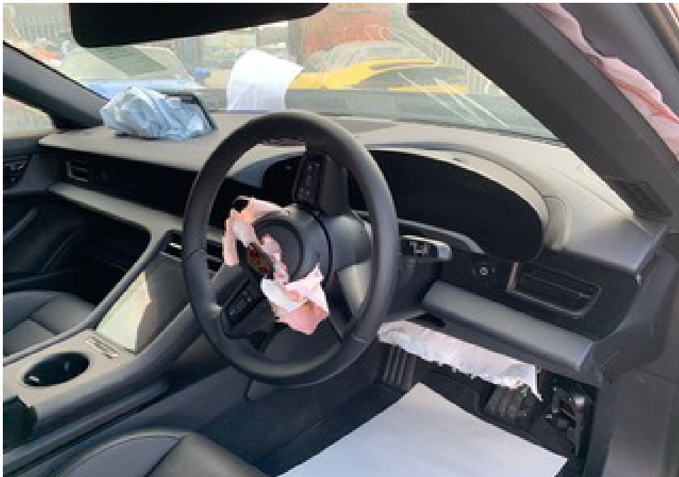
Photo 7 shows the interior compartment of the Motor Car (photograph provided to me). The various parts and components within the interior compartment were all intact and unaffected. The driver's airbag, driver's knee airbag and front left passenger airbag were deployed as seen from the photographs that were provided to me.
