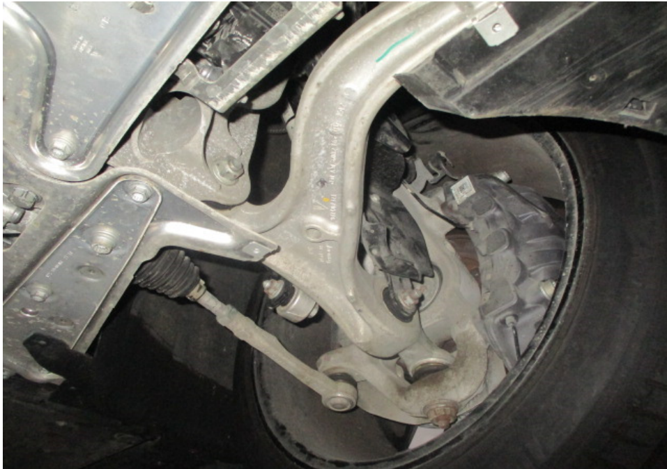
Photo 28 shows the various undercarriage components at the front left wheel of the Motor Car. The mechanical components, control arms and linkages were all found to be intact and secured in an appropriate manner.
