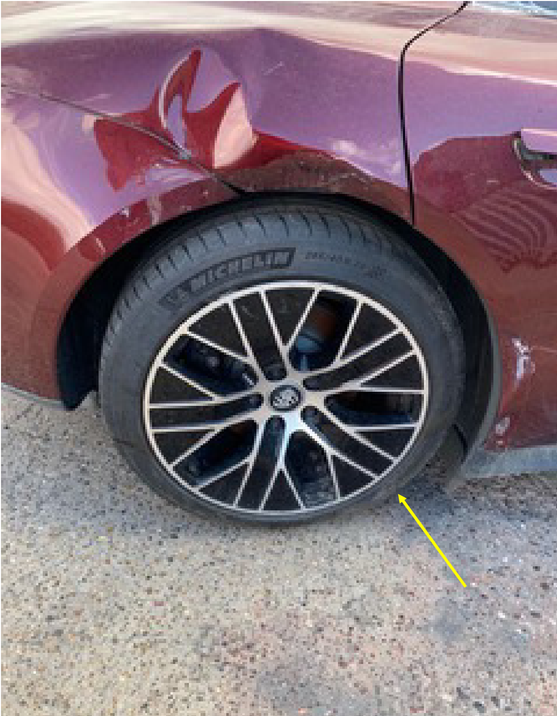
Photo 5 shows a closer view of the damage at the right side rear portion of the Motor Car (photograph provided to me). The rear right door, rear right fender and rear bumper were amongst the body parts that were observed to have been damaged. The Motor Car's rear right wheel (arrowed) was also observed to be shifted inwards, suggesting damage to the undercarriage parts at the rear right wheel of the Motor Car. Undercarriage parts that may possibly be damaged include the rear right lower arm, rear right knuckle arm, rear right upper arm and rear right shock absorber amongst others.
