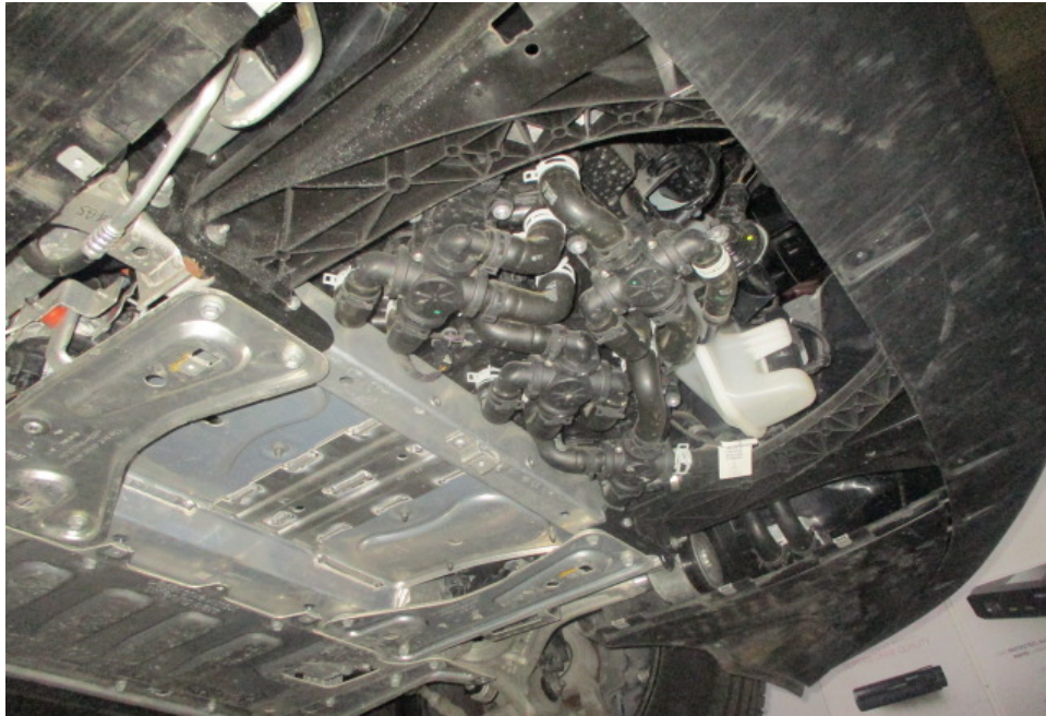
Photo 32 shows the underside front of the Motor Car, at the location where the front electric motor, is fitted. The high voltage system of the Motor Car was visually checked, and it was observed that the various high voltage parts and components like the high voltage battery, inverter unit, converter unit, high voltage cables, electric motors and electric aircon compressor amongst others, were properly secured and without any physical damage.
