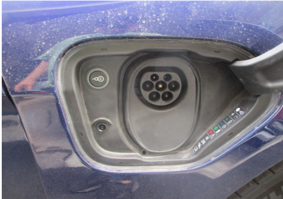
Photo 20 shows the high voltage charging port located at the front right fender of the Motor Car at the time of my inspection. A JS 1772 (Type 2) for alternating current (AC) charging was fitted on the front right fender of the Motor Car. No physical damage was observed to the charging head.
