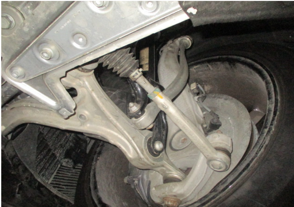
Photo 29 shows the various undercarriage components at the front right wheel of the Motor Car. The mechanical components, control arms and linkages were all found to be intact and secured in an appropriate manner. I also did not observe any fluid leak and/or fluid stain on the underside of the Motor Car.
