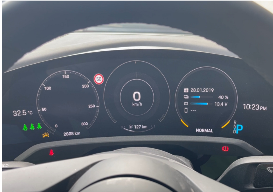
Photo 24 shows the respective warning lights no longer illuminated, indicating that there is no fault detected to the ABS, SRS, EPS, TPM and SCS systems of the Motor Car during the self-test. These electronic systems were hence in working condition at the time of my inspection.
