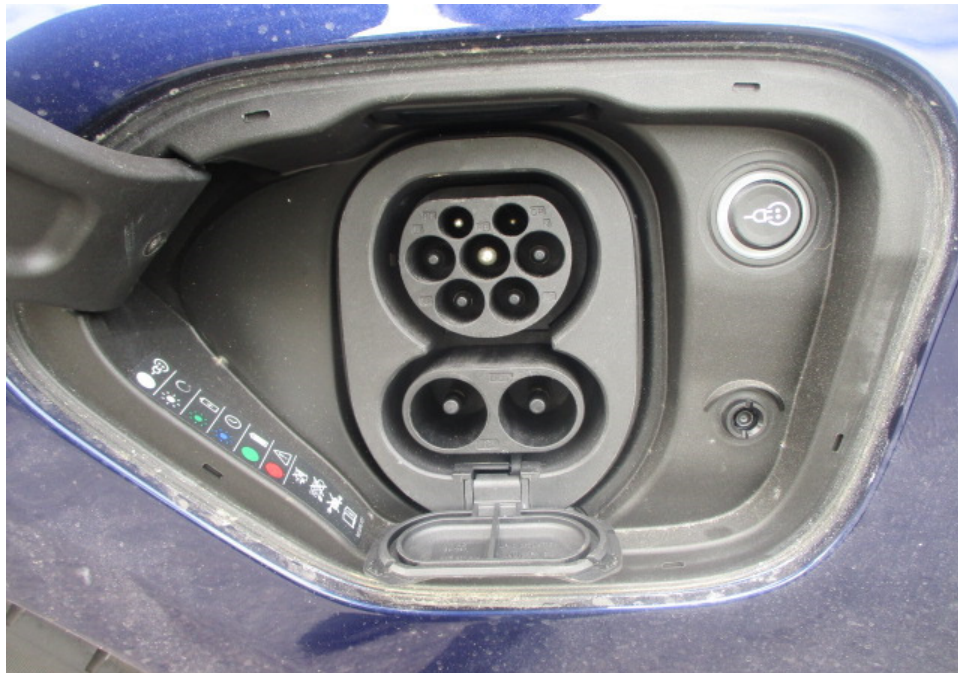
Photo 19 shows the high voltage charging port located at the front left fender of the Motor Car at the time of my inspection. A Combined Charging Standard 2 (CCS 2) for direct current (DC) charging was fitted on the front left fender of the Motor Car. No physical damage was observed to the charging head.
