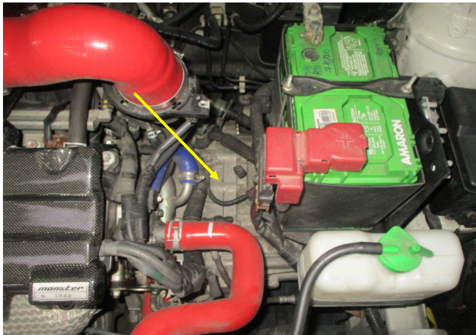
Photo 7 shows the Motor Car's transmission assembly (arrowed) as viewed from the engine compartment. The bracket supporting the left side of the Motor Car's transmission assembly is located below the battery (hidden from view). This bracket was mounted onto the left side front chassis, adjacent to the left side front wheel house of the Motor Car.
