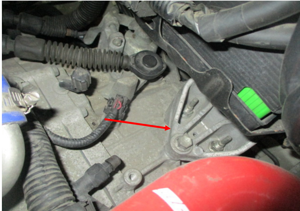
Photo 8 shows the bracket supporting the left side of the Motor Car's transmission assembly. This bracket was mounted onto the left side front chassis, adjacent to the left side front wheel house of the Motor Car. The bracket was with rubber bushings that absorbs any vibrations arising from the rotation of the transmission gears, minimising any stress to the bracket and correspondingly also minimise any stress to the engine crossmember.
