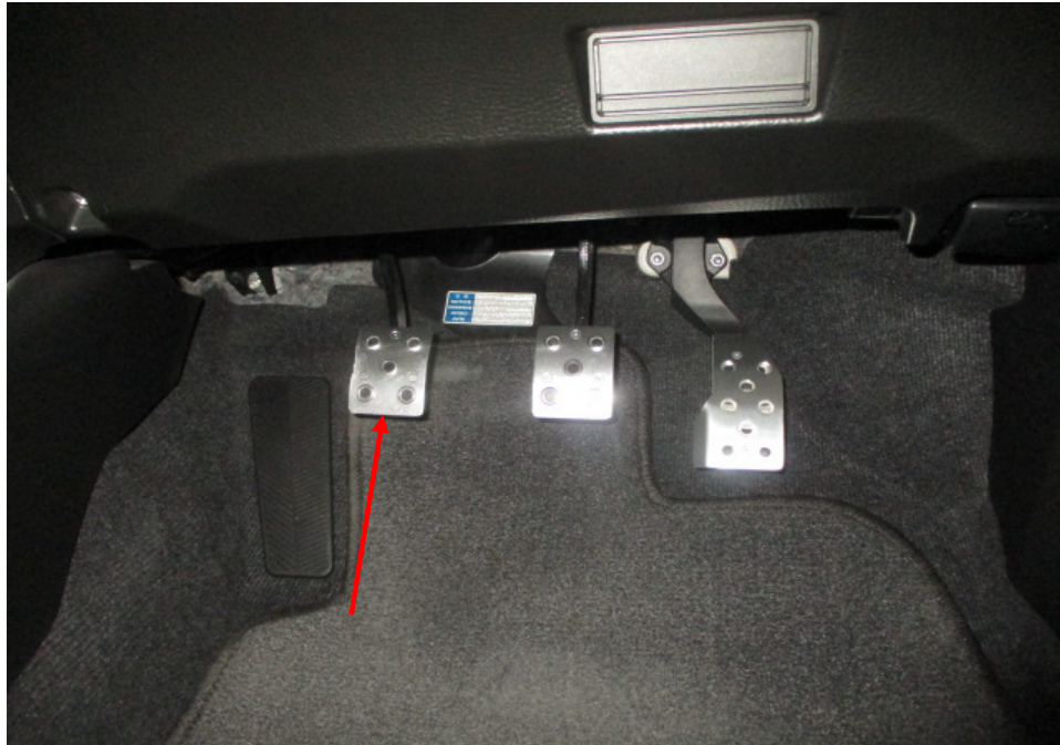
Photo 10 shows the Motor Car's clutch pedal (arrowed) for engaging and disengaging the transmission gears.
