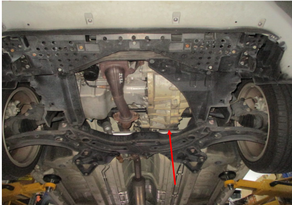
Photo 2 shows a general view of the transmission assembly (arrowed) that was fitted on the Motor Car. as viewed from the front to rear. The input side of the transmission assembly is bolted to the crankshaft side of the engine block. The left and right drive shafts were securely fitted from the main shaft, located inside the transmission assembly, to the front left wheel and front right wheel respectively. There was no crack and/or hole observed on the housing of the transmission assembly.
