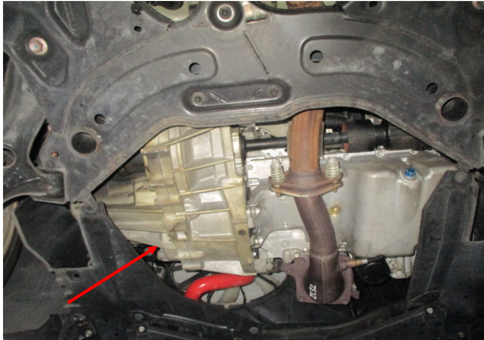
Photo 6 shows the transmission assembly (arrowed) that was fitted on the Motor Car, as viewed from the rear to front. The transmission assembly of the Motor Car was supported by 2 brackets. One bracket was at the rear of the transmission assembly (refer to photograph 4 & 5 above) while the other was at the left side of the transmission assembly (refer to photograph 7 & 8 below).
