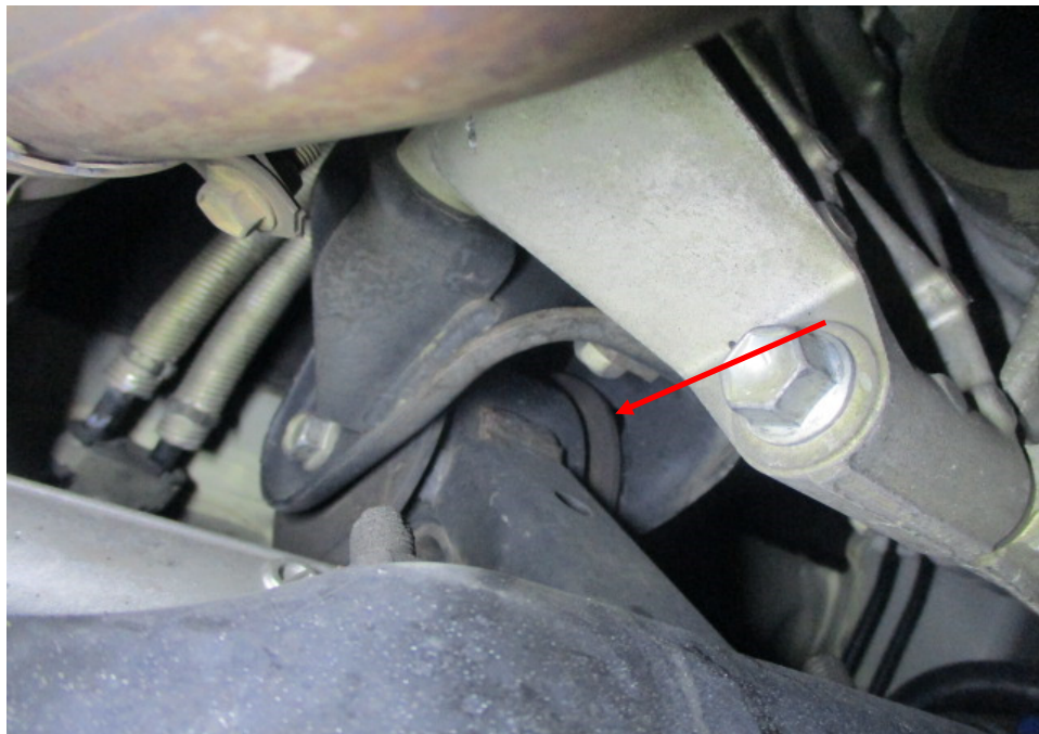
Photo 5 shows the bracket supporting the rear of the Motor Car's transmission assembly. This bracket was mounted onto the engine cross member. The bracket was with rubber bushings (arrowed) that absorbs any vibrations arising from the rotation of the transmission gears, minimising any stress to the bracket and correspondingly also minimise any stress to the engine crossmember.
