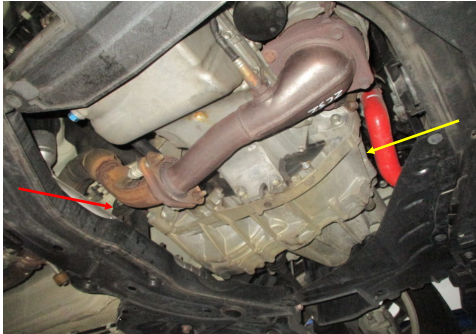
Photo 4 shows another view of the transmission assembly (yellow arrow) that was fitted on the Motor Car, as viewed from the right to left. The transmission assembly of the Motor Car was supported by 2 brackets. One bracket (red arrow) was at the rear of the transmission assembly while the other was at the left side of the transmission assembly (refer to photograph 7 & 8 below).
