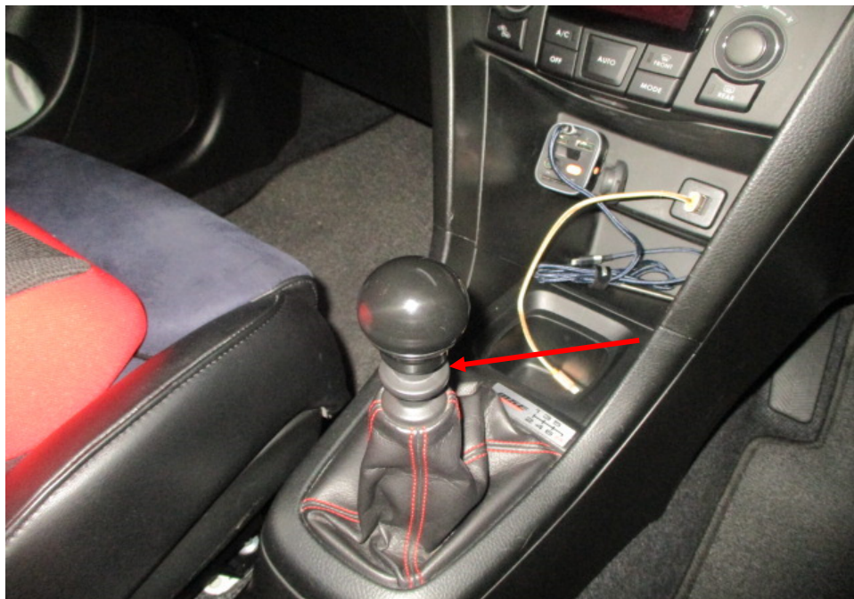
Photo 9 shows the Motor Car's manual gear shifter (arrowed) for manually selecting the transmission gear to be engaged.
